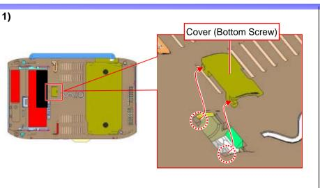
While disengaging the detent (two places), remove the Cover.
