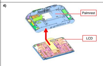
While disengaging the detent (four places), remove the Palmrest. **UX Series**
