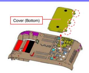
While disengaging the detent (three places), remove the Cover.
