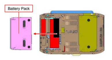
In the state of 1), remove the Battery Pack in the direction of the arrow.
