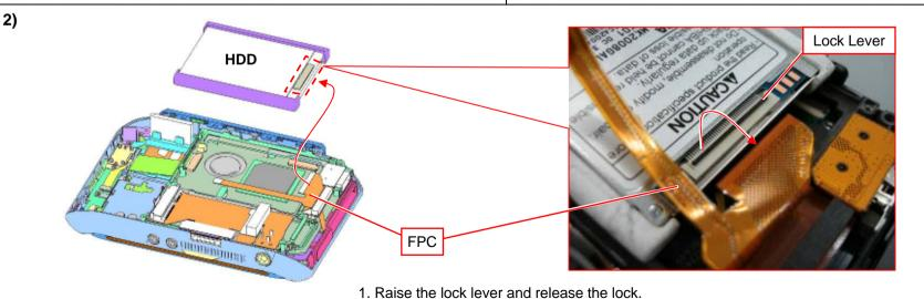
2. While disconnecting the FPC, remove the HDD.
