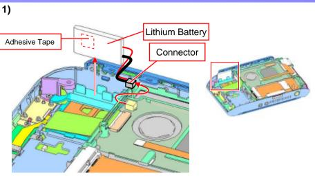
Disconnect the connector and remove the Lithium Battery.
