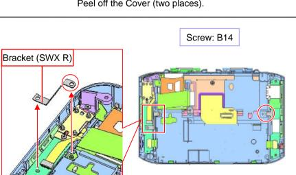
Remove the two screws and the Bracket.
