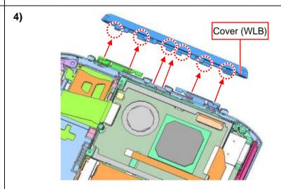
Disengage the detent (six places) and remove the Cover.
