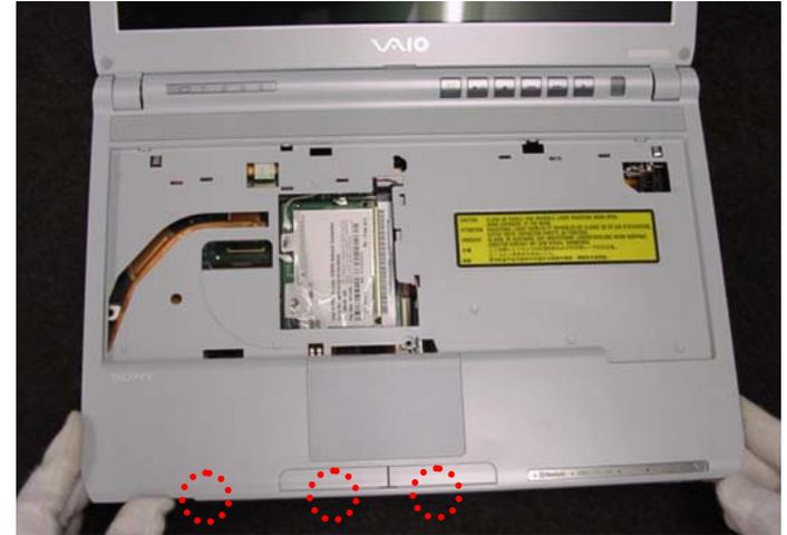
Disengage the detent (three places) at the front.
