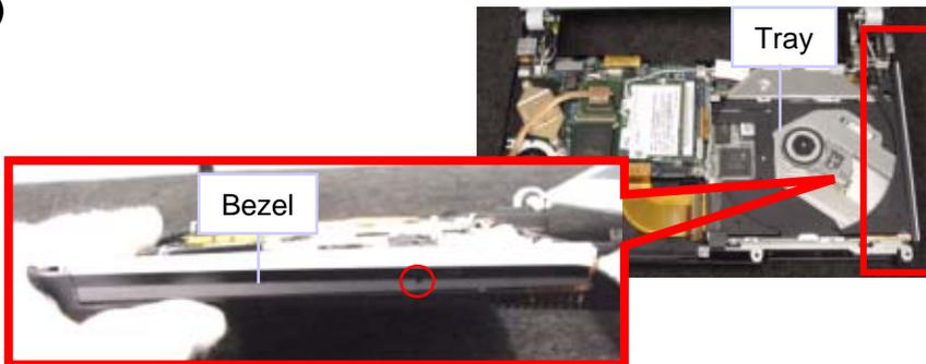
Insert a thin tool into the hole of the Bezel, push it lightly and draw out the tray.
