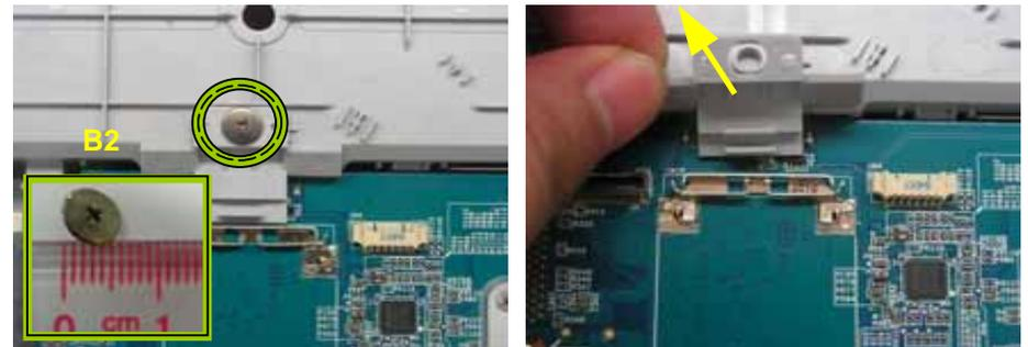
REMOVE ONE SCREW FROM THE LCD HARNESS ROUTING GUIDE. LIFT THE ROUTING GUIDE UP
