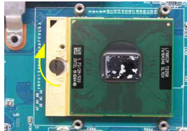
RELEASE THE CPU LOCK BY ROTATING THE LOCK CLOCKWISE WITH A FLAT-BLADE SCREWDRIVER. CAREFULLY LIFT THE CPU UP
