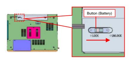
Slide the Button (Battery) to UNLOCK position.
