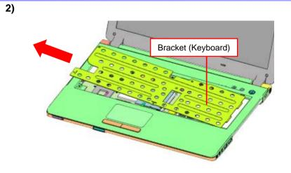
Slide the Bracket (Keyboard) in the direction of the arrow and remove it.
