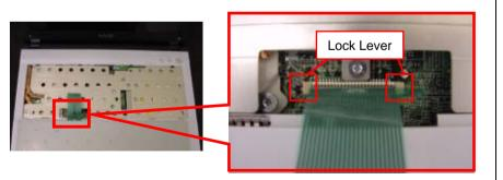
Slide the lock lever upward and release the lock.
