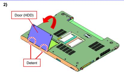
Remove the Door (HDD) toward the front.
