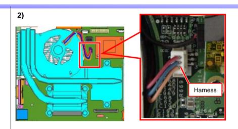
Pull out the Harness (one place) upward.
