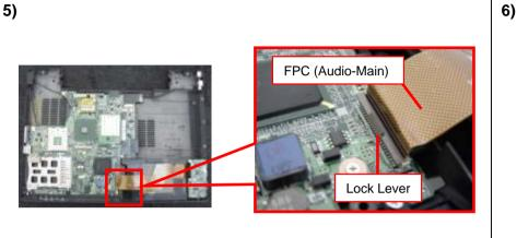
Raise the lock lever upward to release the lock, and disconnect the FPC.
