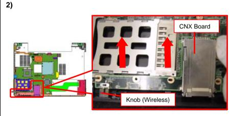
Remove the CNX Board in the direction of the arrow.
