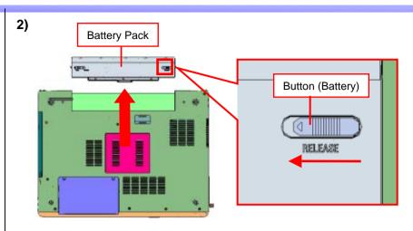
While sliding the Button (Battery) to RELEASE side, remove the Battery Pack.
