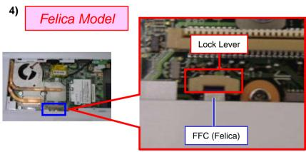
Slide the lock lever upward to release the lock, and disconnect the FFC (one place).
