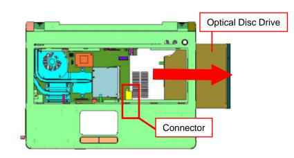
Disconnect the connector by sliding the Optical Disc Drive in the direction of the arrow, and remove the Optical Disc Drive.
