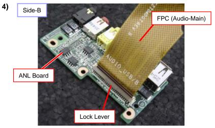
Raise the lock lever upward to release the lock, and disconnect the FPC upward.
