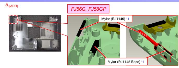
Peel off the Mylar (two place).
