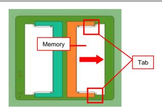
Outspread the tabs (two places) simultaneously to release the lock and pull out the Memory in the direction of the arrow.
