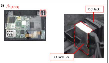
Peel off the DC Jack Foil (one place), and remove the DC Jack.
