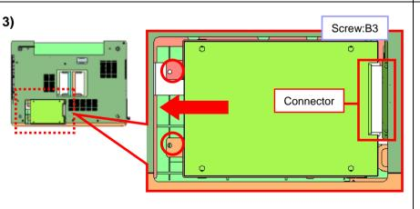
Remove the two screws, and disconnect the connector portion by sliding it in the direction of the arrow.
