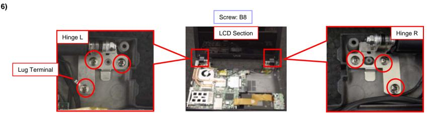
Remove the six screws, lift up the LCD Section with both hands, and remove the LCD Section.
