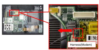
Disconnect the Harness (Modem) in the direction of the arrow.
