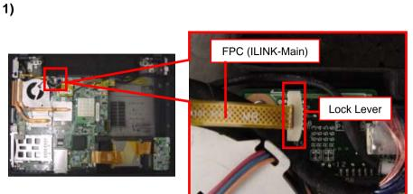
Slide the lock lever upward to release the lock, and remove the FPC (one place).
