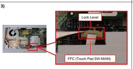
Slide the lock lever upward to release the lock, and disconnect the FFC (one place).
