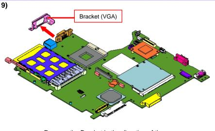
Remove the Bracket in the direction of the arrow.
