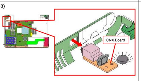
Remove the CNX Board in the direction of the arrow.
