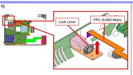
Slide the lock lever upward to release the lock, and pull out the FPC upward.
