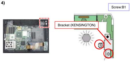
Remove the two screws, and the Bracket.
