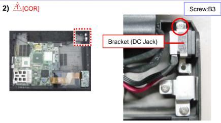
Remove the screw and the Bracket.
