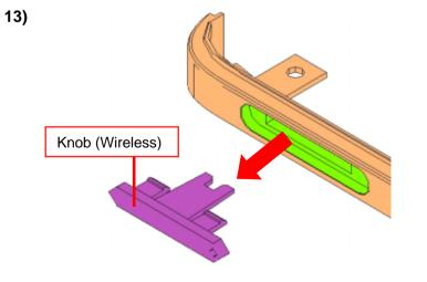
Disengage the detent (three places) from the backside of the Cover.
