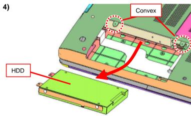
Raise the front side of the HDD, and remove it toward the front.
