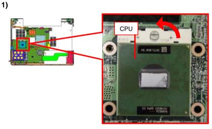
Rotate the lock screw in the counterclockwise direction with a 4 mm flat-head (-) screwdriver and release the lock.
