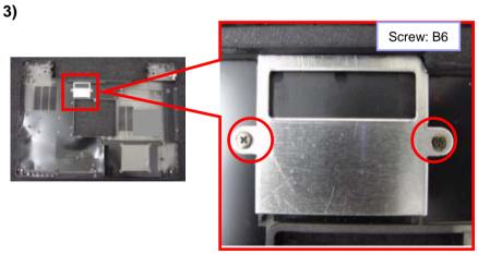
Remove the two screws, and the Plate (two places).
