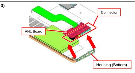
While releasing the connector portion, remove the ANL Board in the direction of the arrow.
