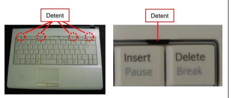
Disengage the detent (four places).
