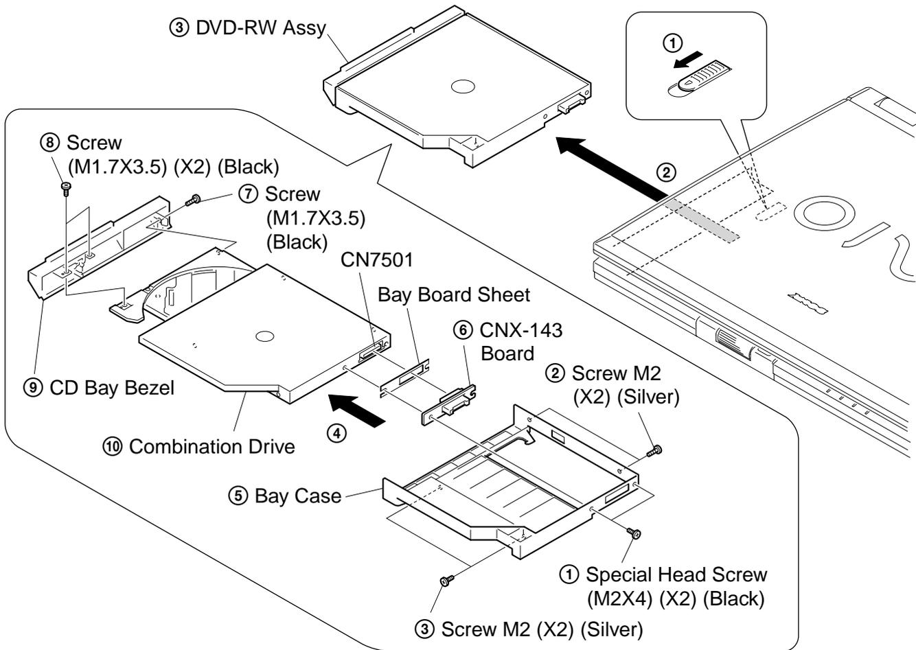
**Note :** If the DVD-RW Assy cannot be removed, there is a case that the portion (A) on the rear of the main unit is secured by screw. Remove the screw blind seal (Cap Bay) and check it.
