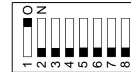
The upper position where ON indication is shown is the ON position . The lower position is the OFF position.
