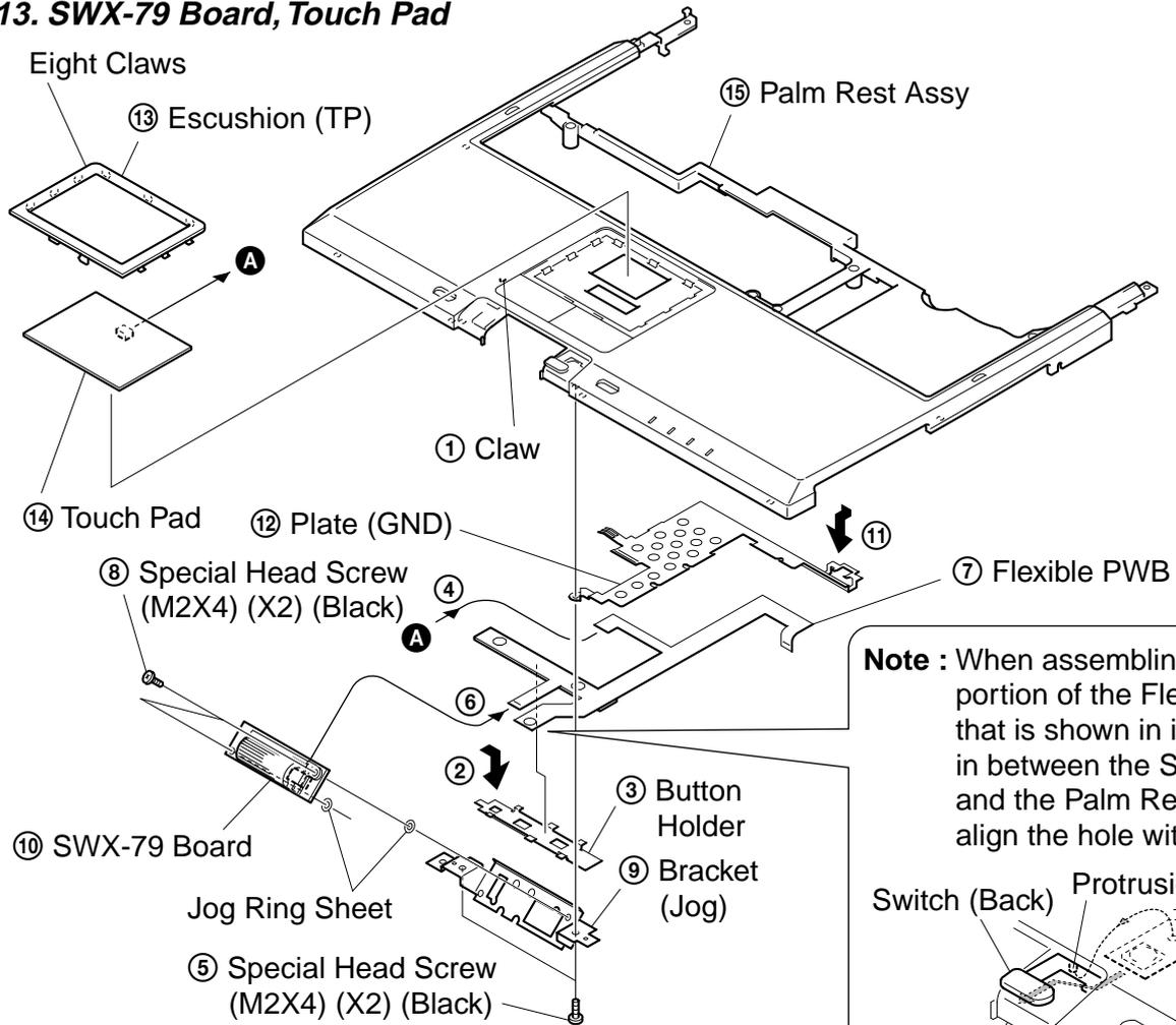
**Note :** When assembling, insert the portion of the Flexible PWB that is shown in illustration, in between the Switch (Back) and the Palm Rest Assy and align the hole with protrusion
