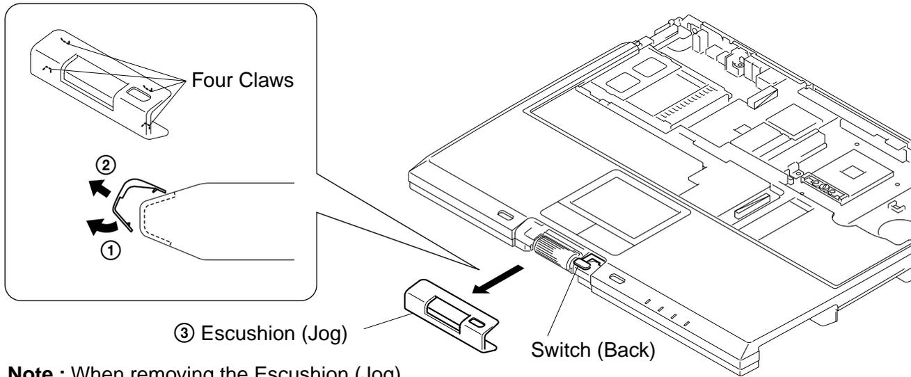
**Note :** When removing the Escushion (Jog), be careful not to damage the Switch (Back).
