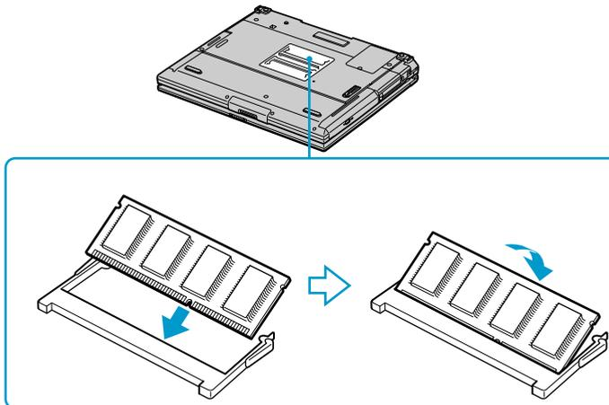
1 Slide the memory module into the slot. 2 Press the module into place until it clicks.
