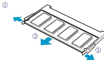
① Pull the tabs in the direction of the arrows. The memory module is released.
