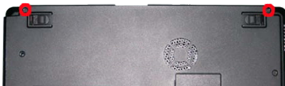
Fig. 20 Removing the screws retaining the LCD Module
