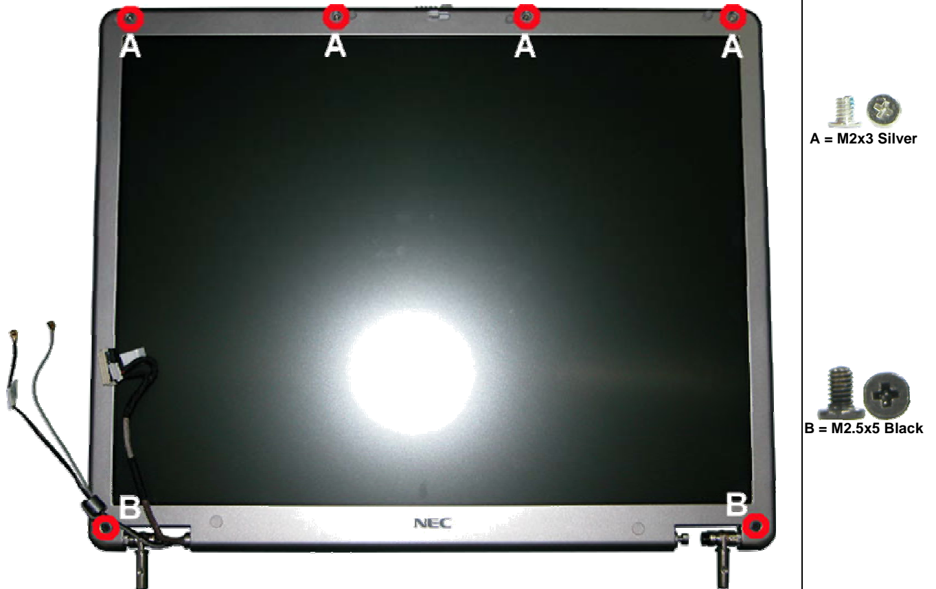
Fig. 23 Removing the rubber covers & screws on the LCD Module
