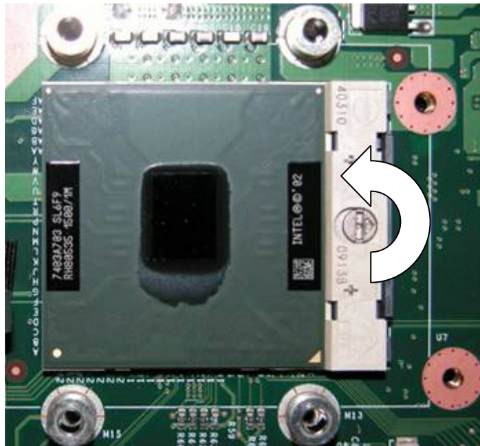
Fig. 18 Unlocking the CPU
