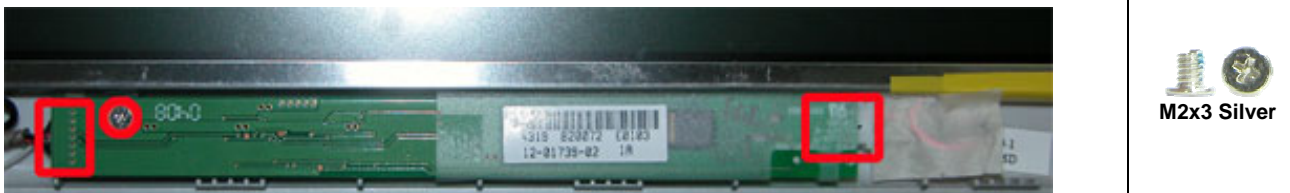
Fig. 24 Removing the Inverter Board
