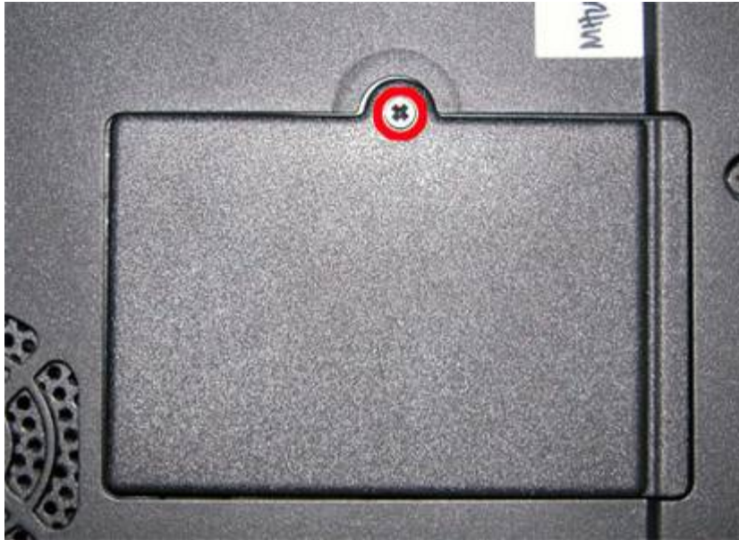
Fig. 2 Removing the screw retaining the memory module slot cover
