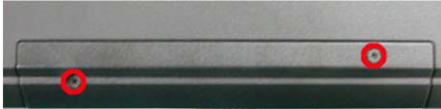
Fig. 4 Removing the Hard disk drive cover
