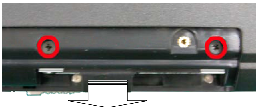
Fig. 5 Screw retaining the HDD module
