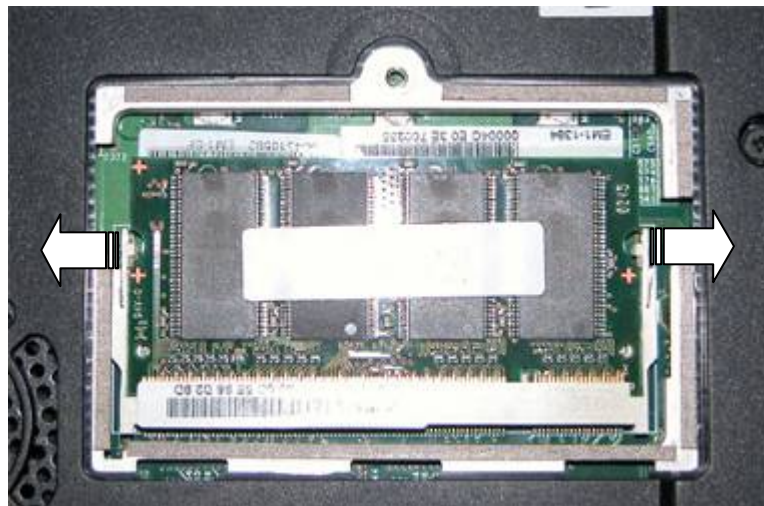
Fig. 3 Removing the memory module
