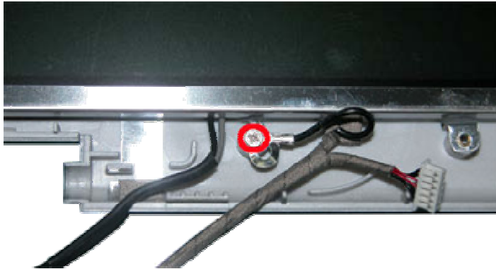
Fig. 25 Removing the screw on LCD cable
