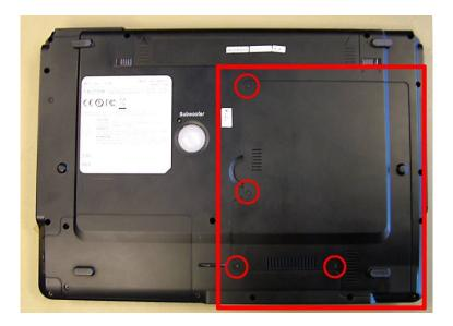
Note: The CPU cover on the EasyNote MV35, MV51 and MV61 is secured with 7 screws.
