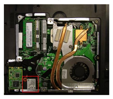
3. Disconnect the modem cable and take out the modem.
