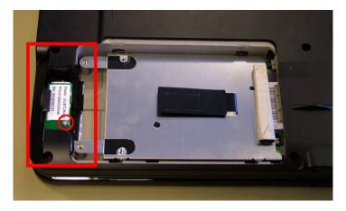
4. Lift the Bluetooth module and disconnect the flat cable.
