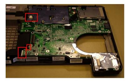
9. Remove the three screws securing the mainboard.
