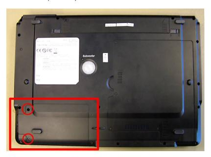
3. Remove the screw holding the Bluetooth module.
