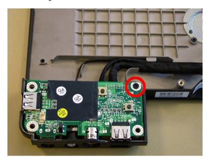
3. Lift the board and disconnect both cables.
