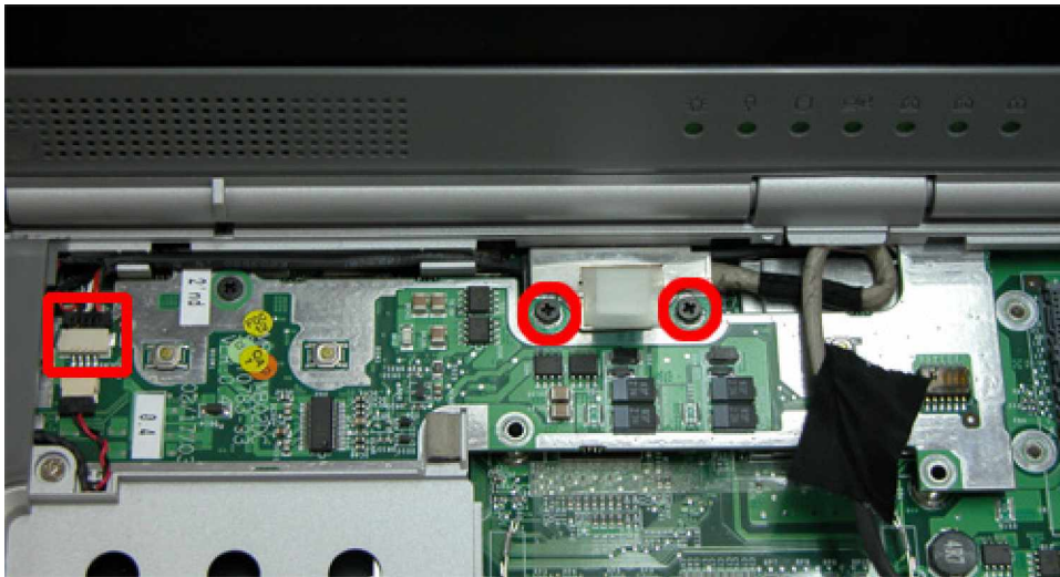
Fig. 18 Disconnecting the LCD & speaker connectors
