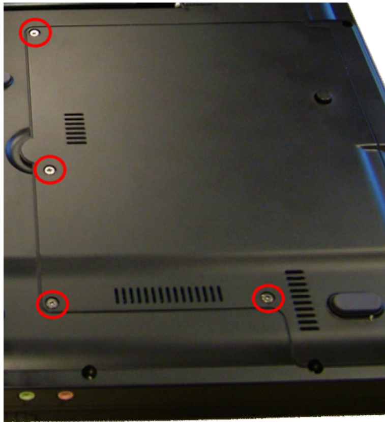
Fig. 3 Removing the main hatch.
