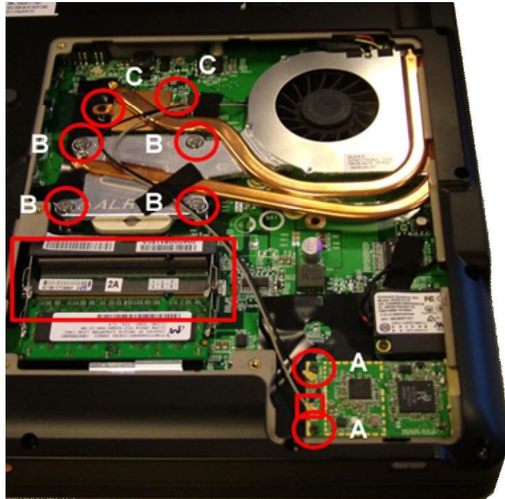
Fig. 4 Removing the memory module(s), mini-PCI and heatsink.
