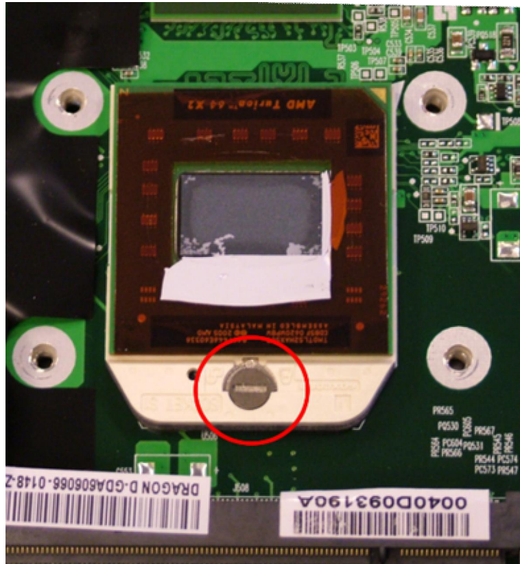
Fig. 5 Unlocking the CPU.
