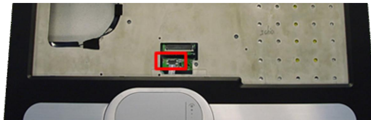
Fig. 9 Disconnecting touchpad flat cable
