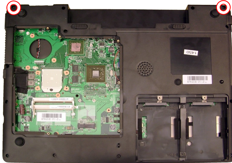
Fig. 40 Location of screws.
