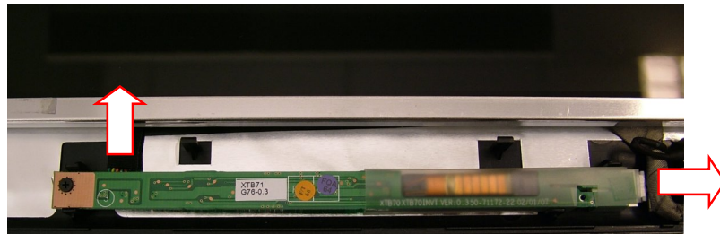
Fig. 43 Disconnecting cables from inverter board.
