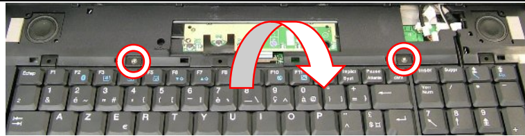
Fig. 12 Location of keyboard screws.
