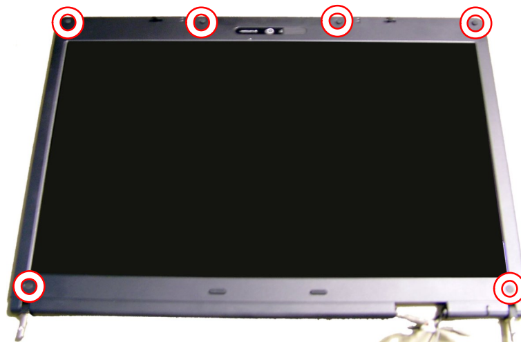
Fig. 41 Location of stoppers/screws securing LCD bezel.
