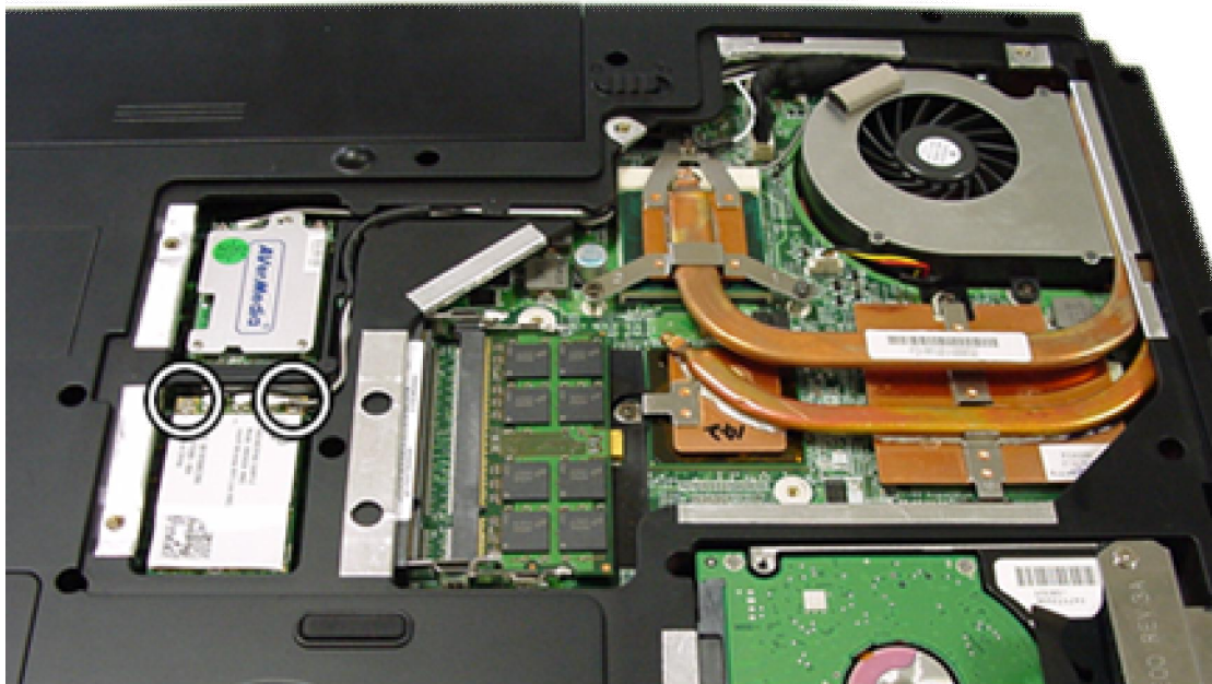
Fig. 14 Removing the wireless card.
