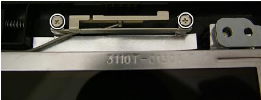
Fig. 24 One of the wireless antenna clips.
