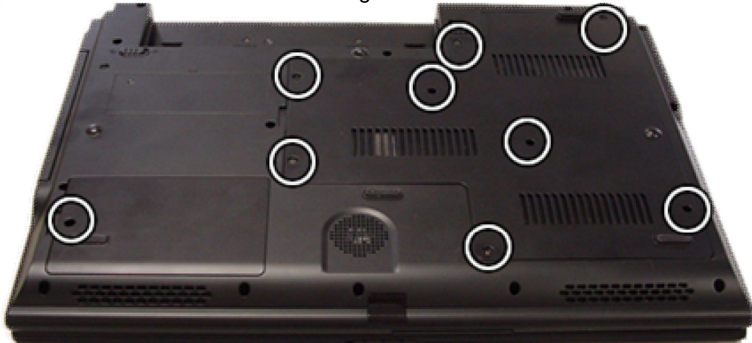
Fig. 11 The bottom base screws.
