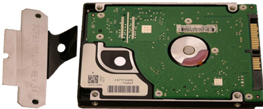
Fig. 4 The HDD and its bracket.
