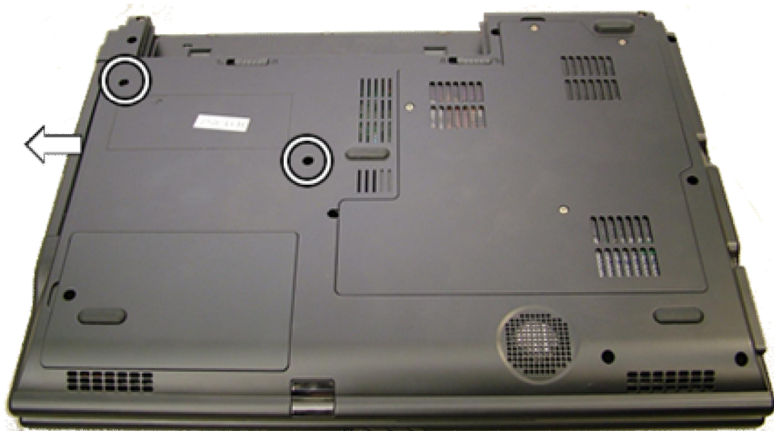
Fig. 7 The optical drive screws.
