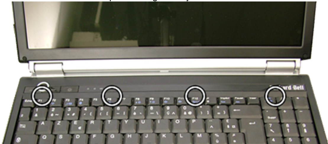
Fig. 17 The keyboard clips.
