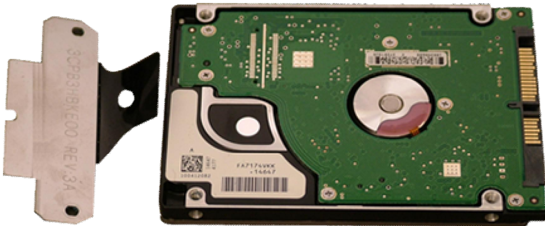
Fig. 6 The HDD and its bracket.
