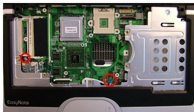
Fig. 16 Glide pad flat cable and the microphone cable.
