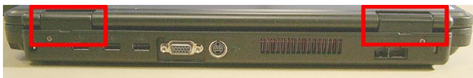
Fig. 7 Lifting the hinge/keyboard covers.
