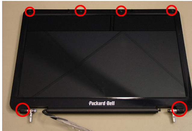
Fig. 27 Location of rubber stoppers on the LCD assembly.
