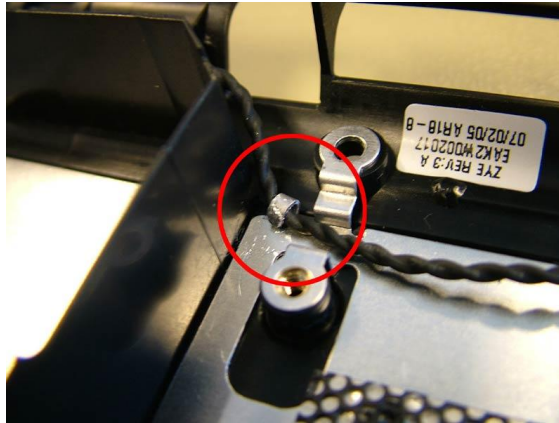
Fig. 23 Metal clip securing the speaker cable.
