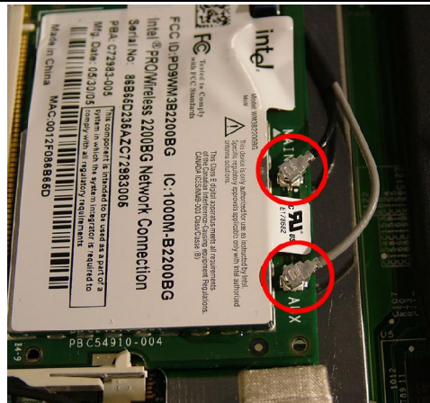
Fig. 11 The 2 antenna connectors: MAIN and AUX.
