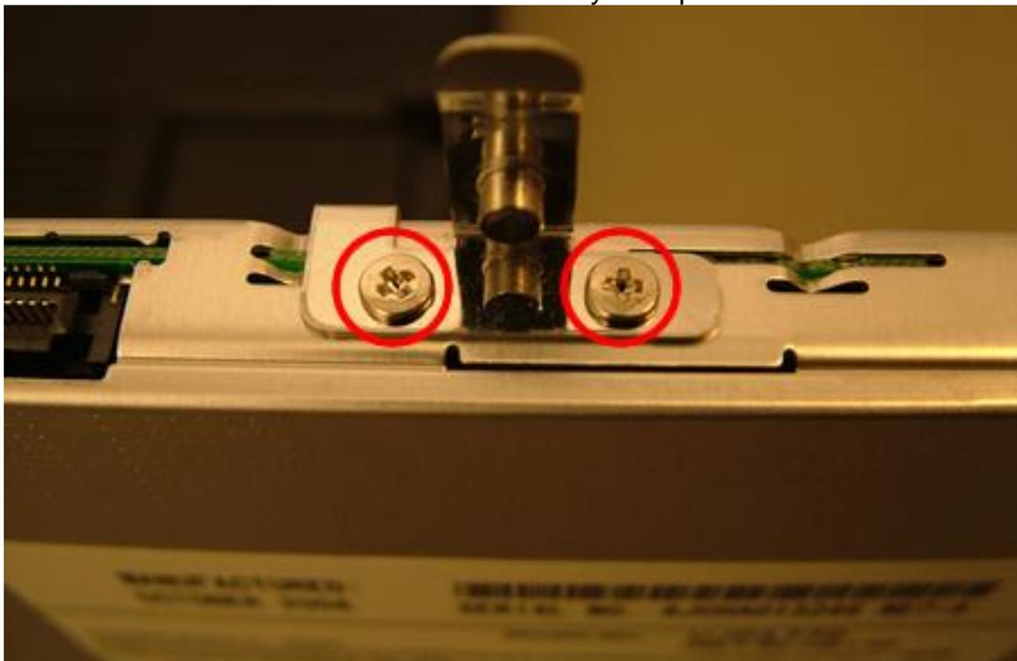
**Fig. 8** The optical drive bracket.
