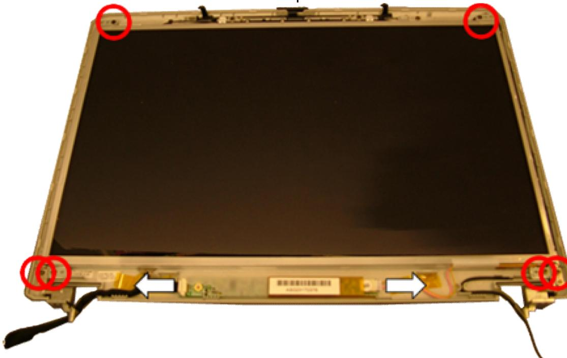
**Fig. 24** *LCD panel assembly after top cover removal.*
