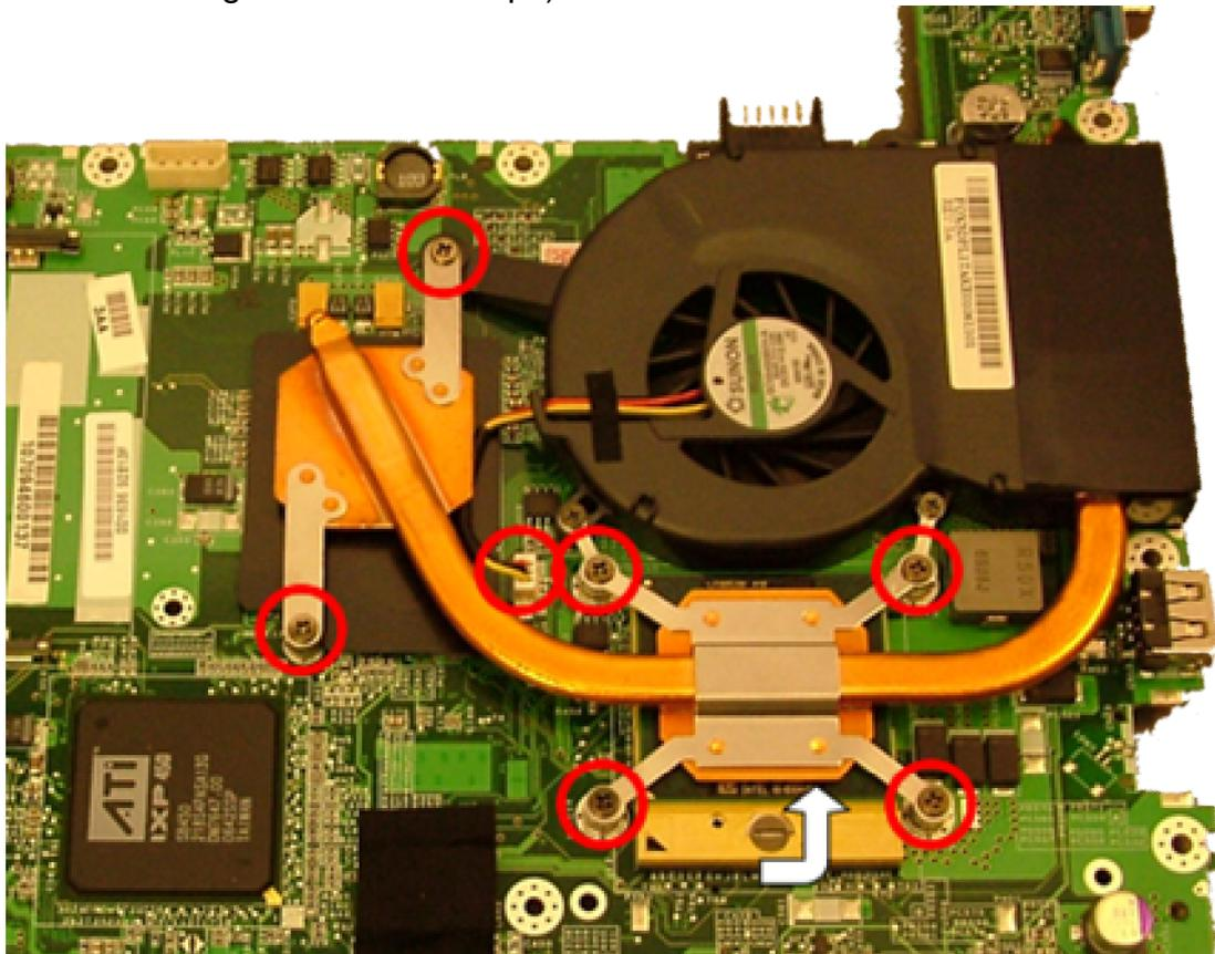
**Fig. 20** *The heatsinks for the CPU and north-bridge.*
