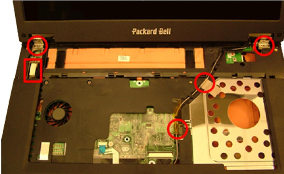
**Fig. 14** *The WLAN antenna and hinge screws.*
