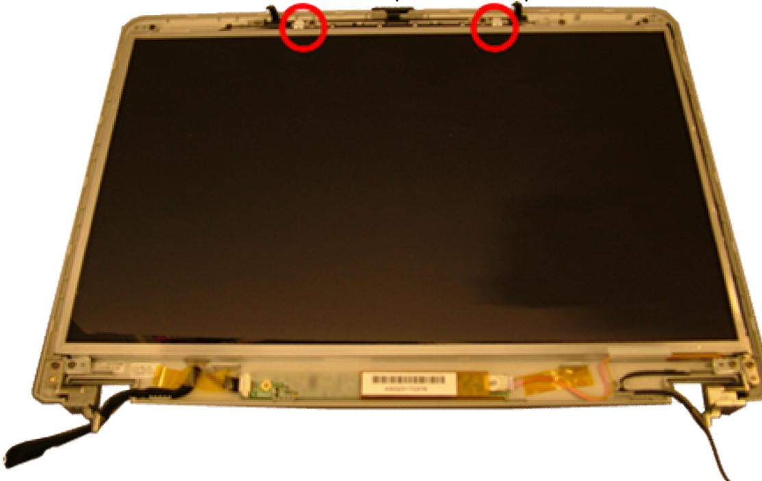
Fig. 26 *The wireless LAN antenna.*
