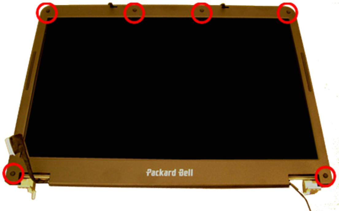
**Fig. 23** *The LCD panel assembly.*
