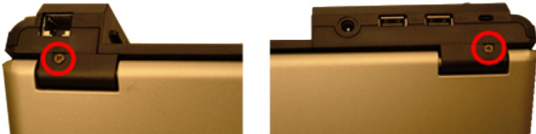
Fig. 10 Hinge cover screw.
