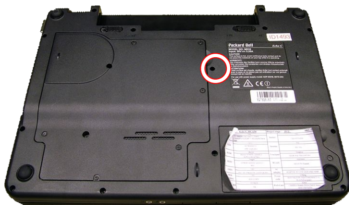
Fig. 11 Removing screw securing optical disk drive.
