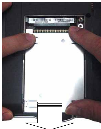
Fig. 3 Disconnecting the hard disk drive
