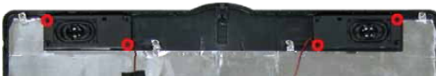
Fig. 28 Removing the Speakers
