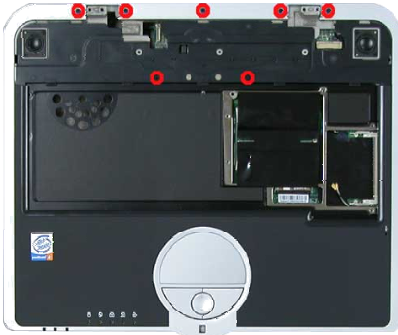
Fig. 33 Removing the top cover screws
