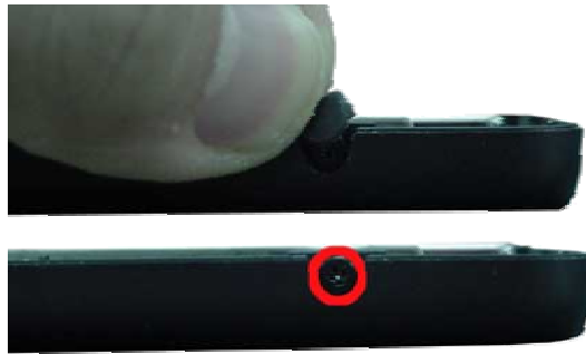
Fig. 26 Removing the Side Rubber Covers
