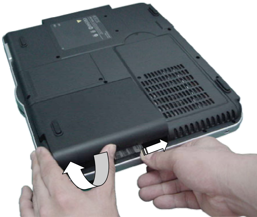
Fig. 1 Removing the battery
