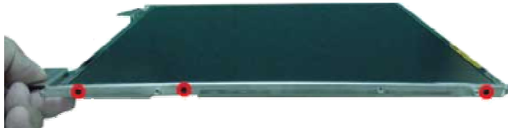
Fig. 27 Removing the LCD Panel hinges
