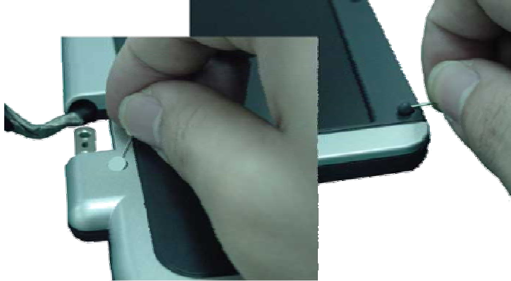
Fig. 16 Removing the rubber covers on the LCD Module
