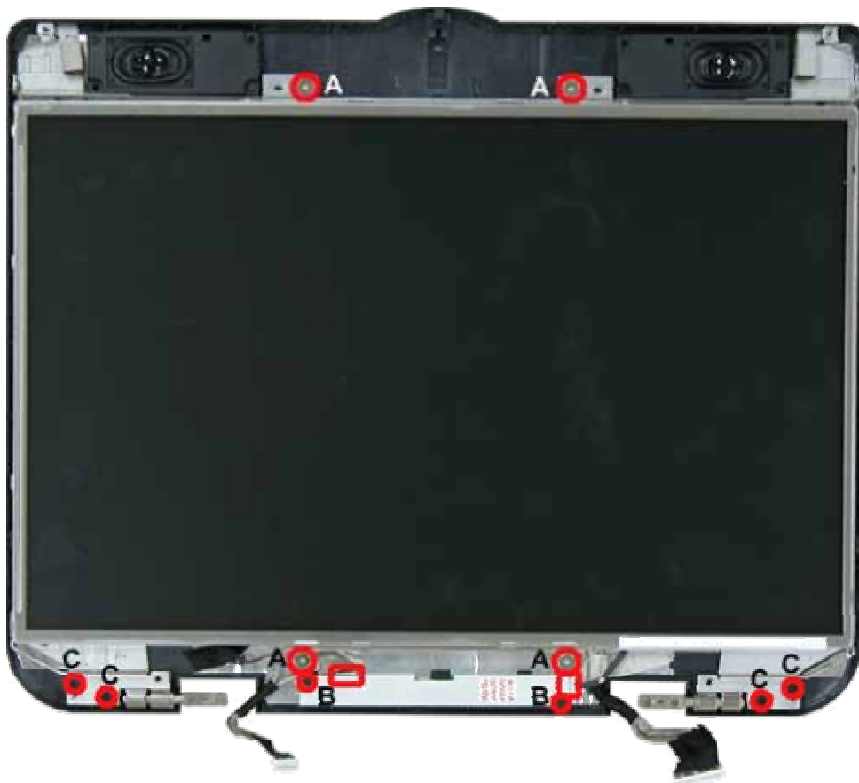
Fig. 25 Removing the LCD panel screws
