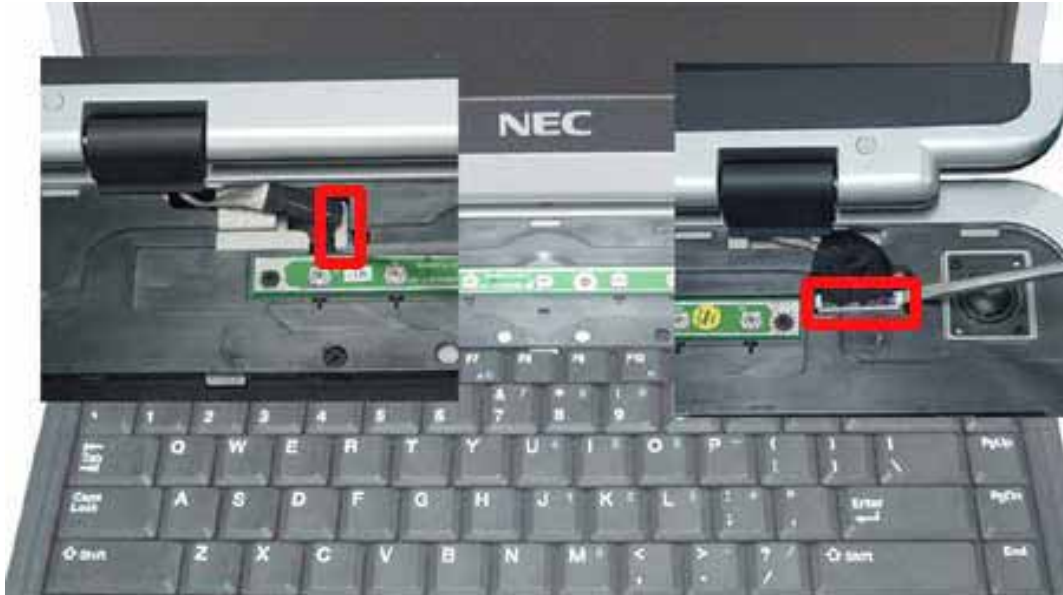
Fig. 13 Disconnecting LCD Connector
