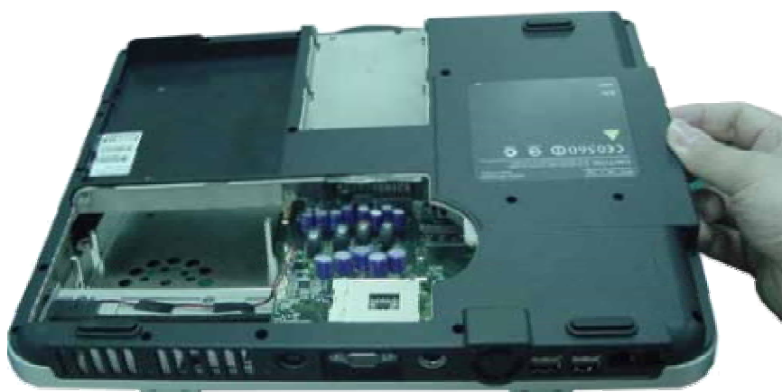
Fig. 36 Removing the Bottom Cover
