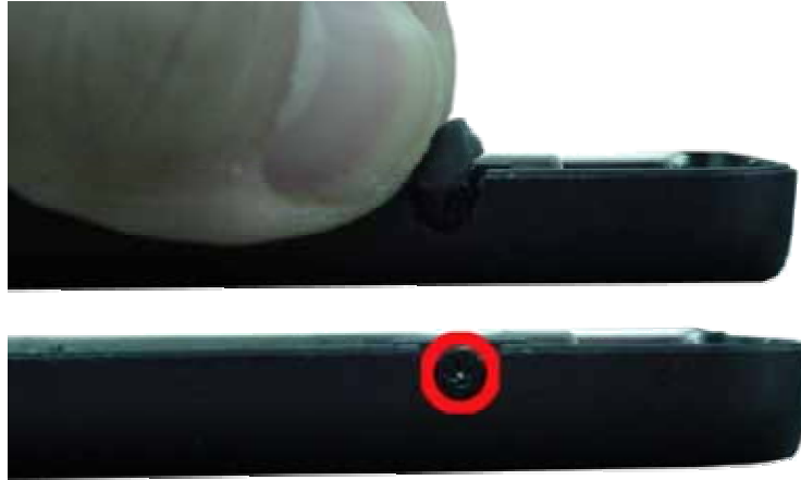
Fig. 20 Remove Side Rubber Cover
