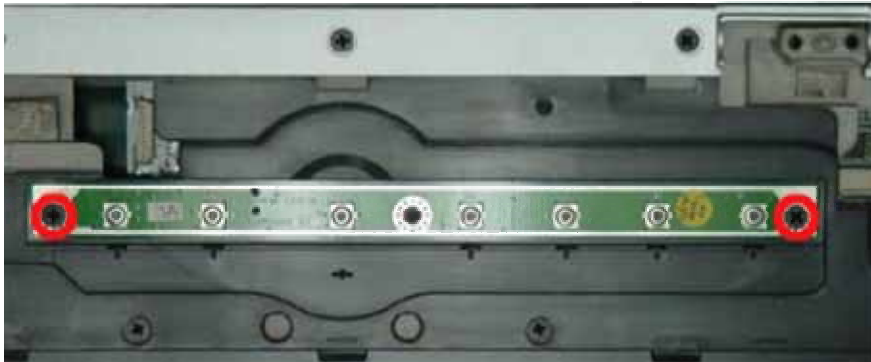
Fig. 32 Removing the Quick Key Board
