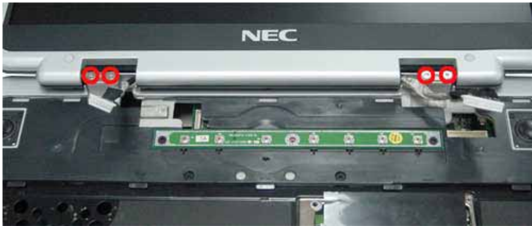
Fig. 15 Releasing the LCD Hinges
