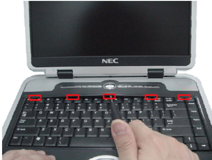
Fig. 8 Removing the Keyboard Cover
