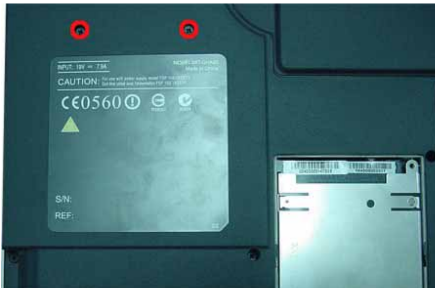
Fig. 5 Releasing the optical drive
