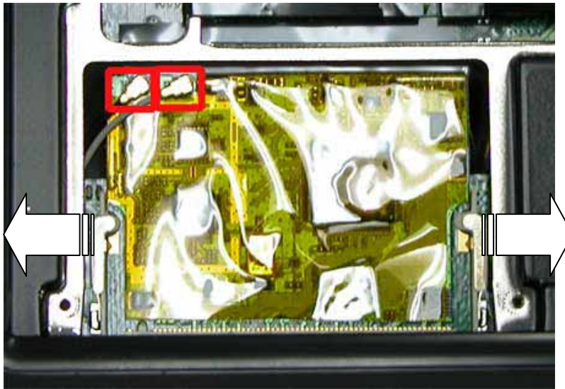
Fig. 41 Removing the WLAN Module
