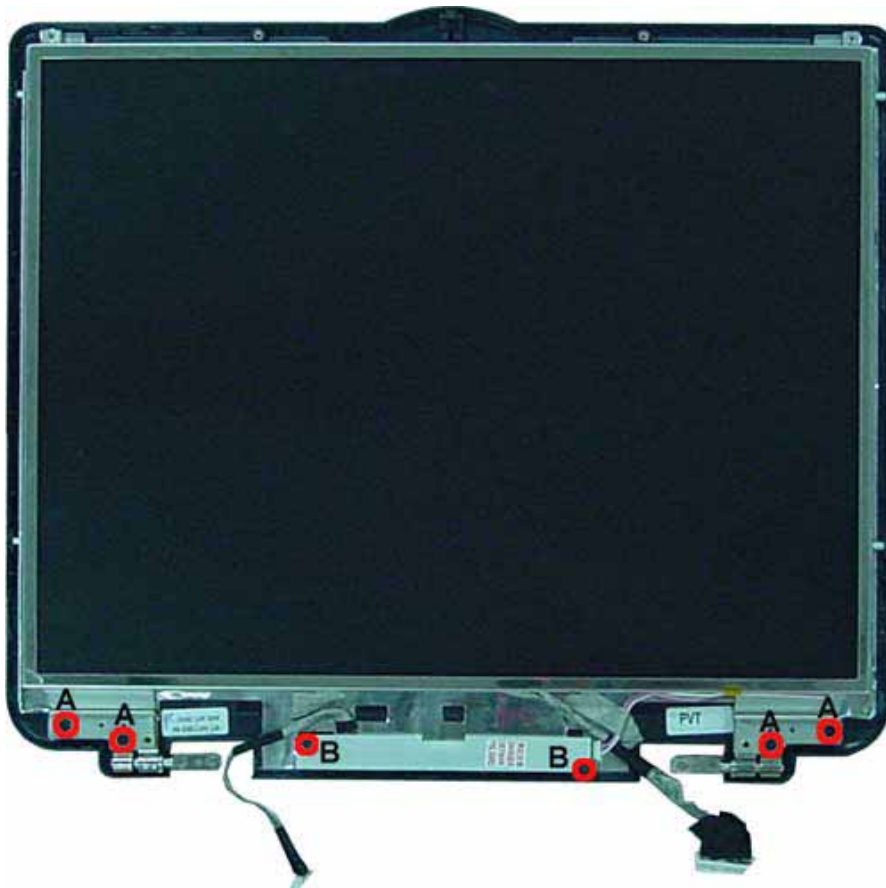
Fig. 19 Removing the LCD panel screws
