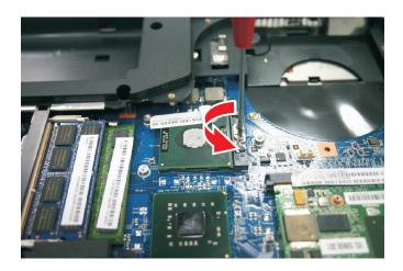
6 Remove the old processor from the system board.
