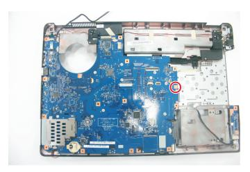
22 Carefully lift the right side of the system board and slide it out of the base panel.
