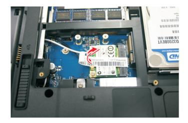
4 Unplug the antenna cables. Note which color cable corresponds to each of the connectors.
