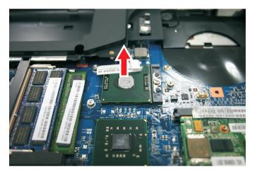
Install the new processor onto the system board making sure that Pin 1 on the processor (indicated by the silk-screened arrow on the corner of the processor) aligns with Pin 1 on the processor socket (indicated by the absence of a pin hole in the processor socket), then use a flat-blade screwdriver to turn the processor lock screw 1/4-turn clockwise.
