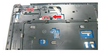
11 Disconnect the left speaker cable from REAR2 connector and release it from the latch.
