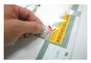
16 Disconnect the LCD cable from the connector.
