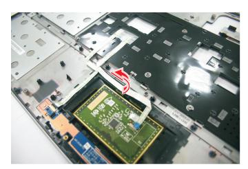
$10\,$  Note the orientation of the touchpad board for later reference in installing the new touchpad board.
