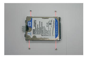
7 Remove the hard drive from the bracket.
