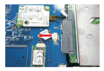
8 The Bluetooth module is glued to the system board. Carefully pry loose the Bluetooth module from the system board using a flat blade screw driver or a plastic scribe.
