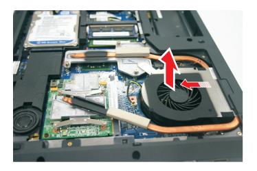
6 Lay the thermal module down in an upright position to avoid tainting your work space with thermal grease.
