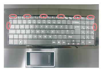
5 Carefully lift up and turn over the keyboard and place it on top of the palm rest.
