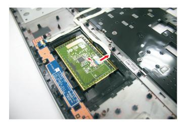
9 Remove the touchpad board cable from the palm rest.
