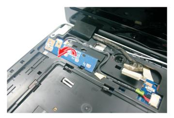
7 Disconnect the cable from the power button board and remove it from the system.
