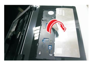
6 Disconnect the keyboard cable and remove the old keyboard.
