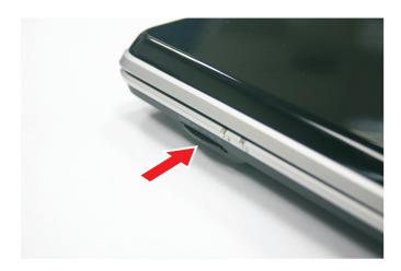
b Pull the memory card out of its slot.
