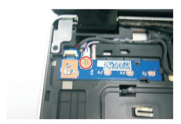
6 Carefully remove the power button board and turn in over to access the cable.
