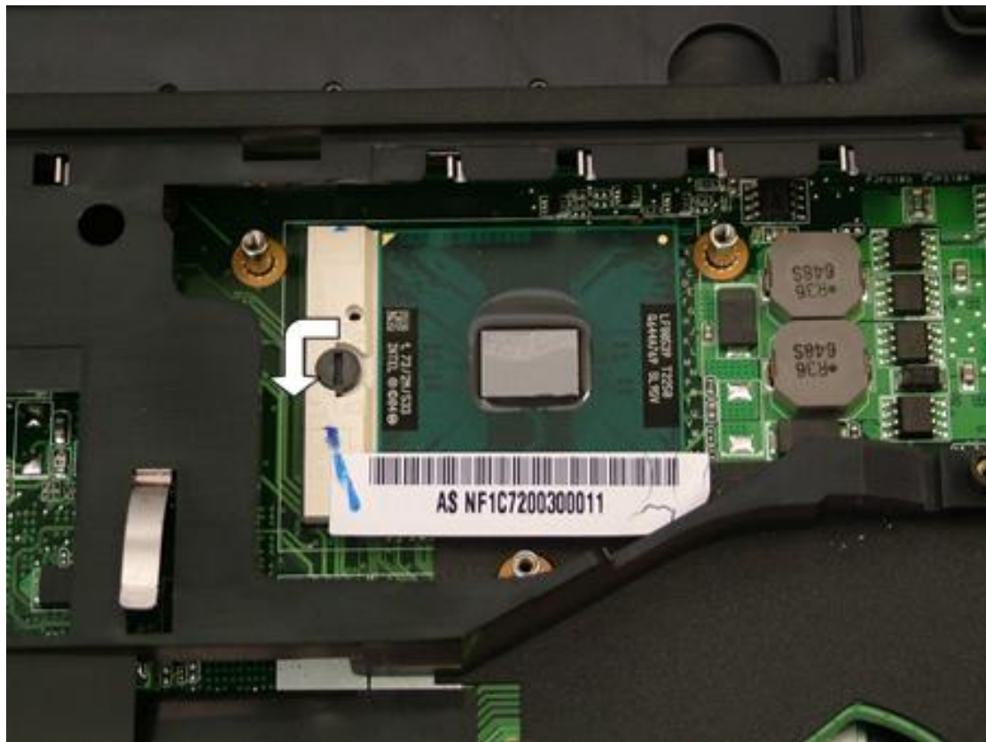
Fig. 12 Unlocking the CPU.
