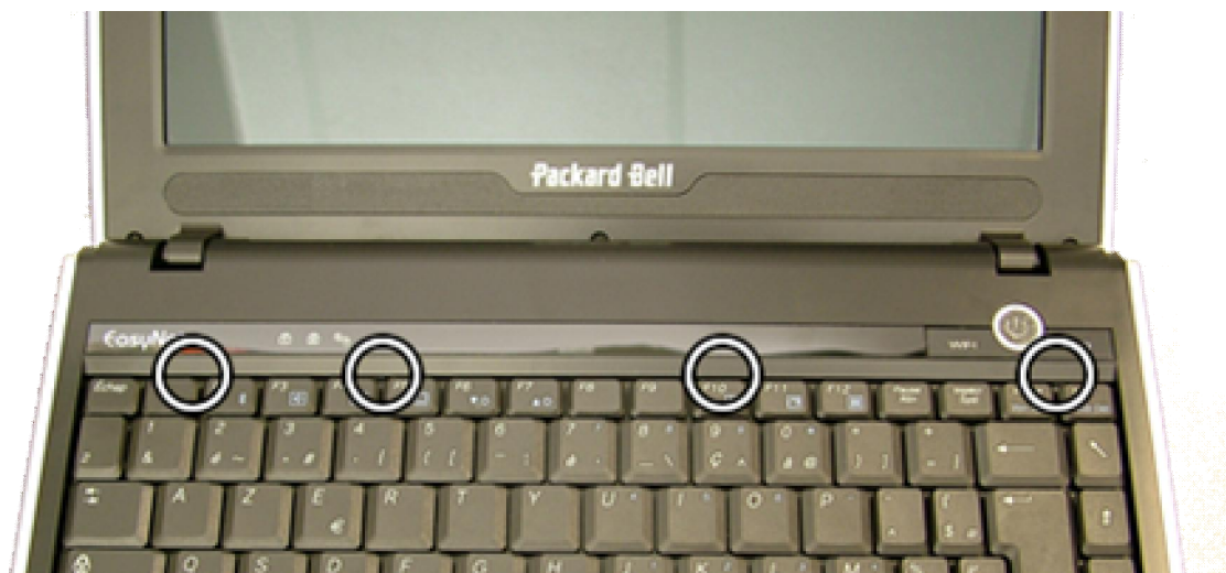
Fig. 13 The keyboard clips.
