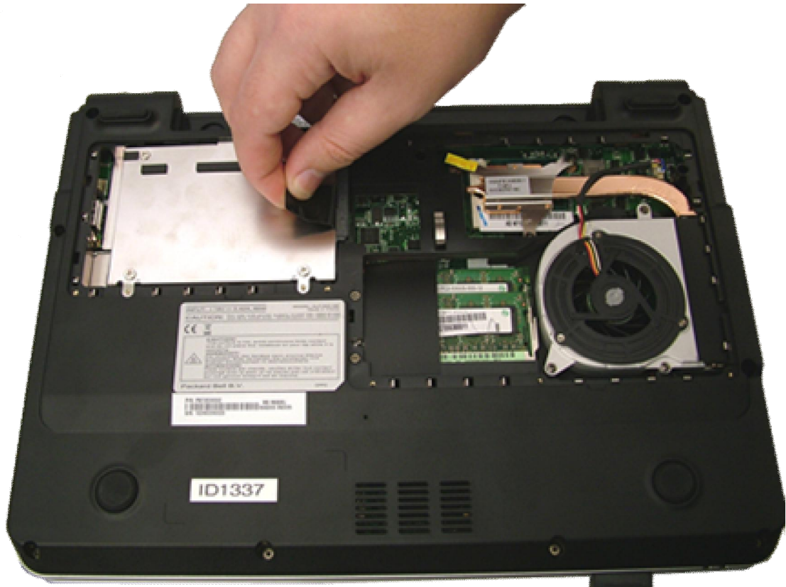
Fig. 5 Lifting out the hard disk drive.
