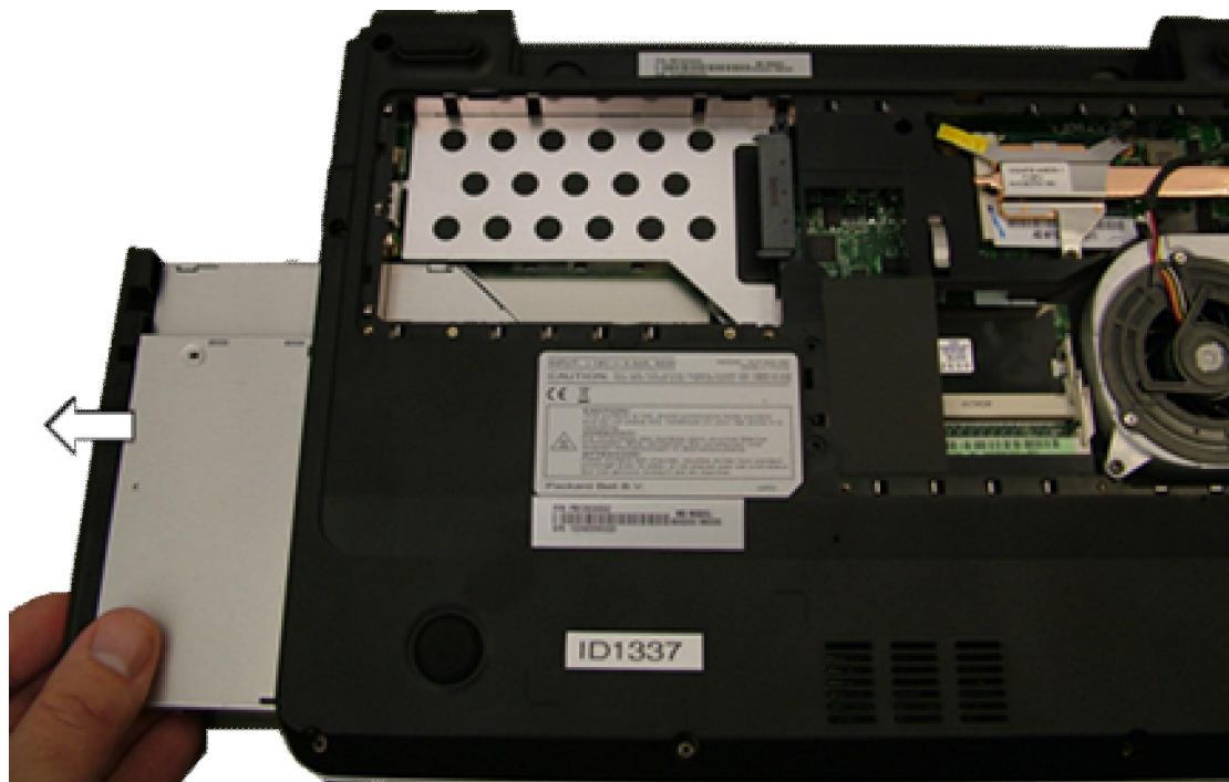
Fig. 8 Taking out the optical drive.
