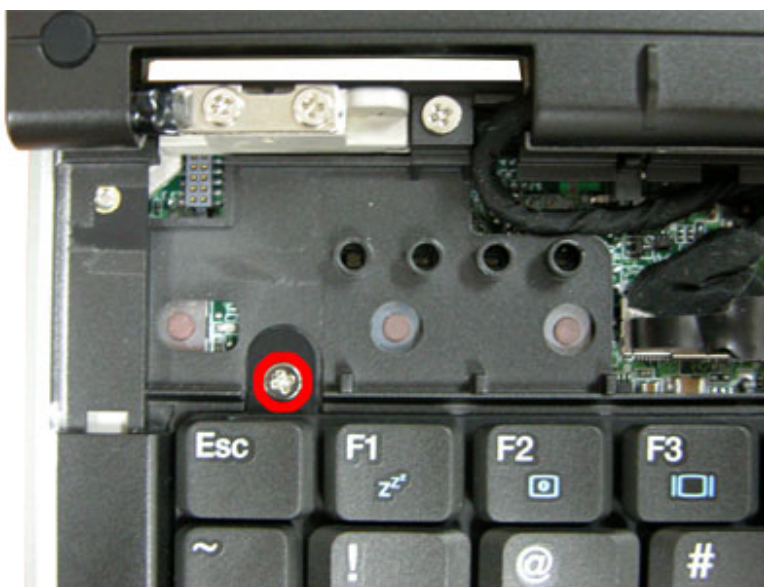
Fig. 16 Screw holding Keyboard
