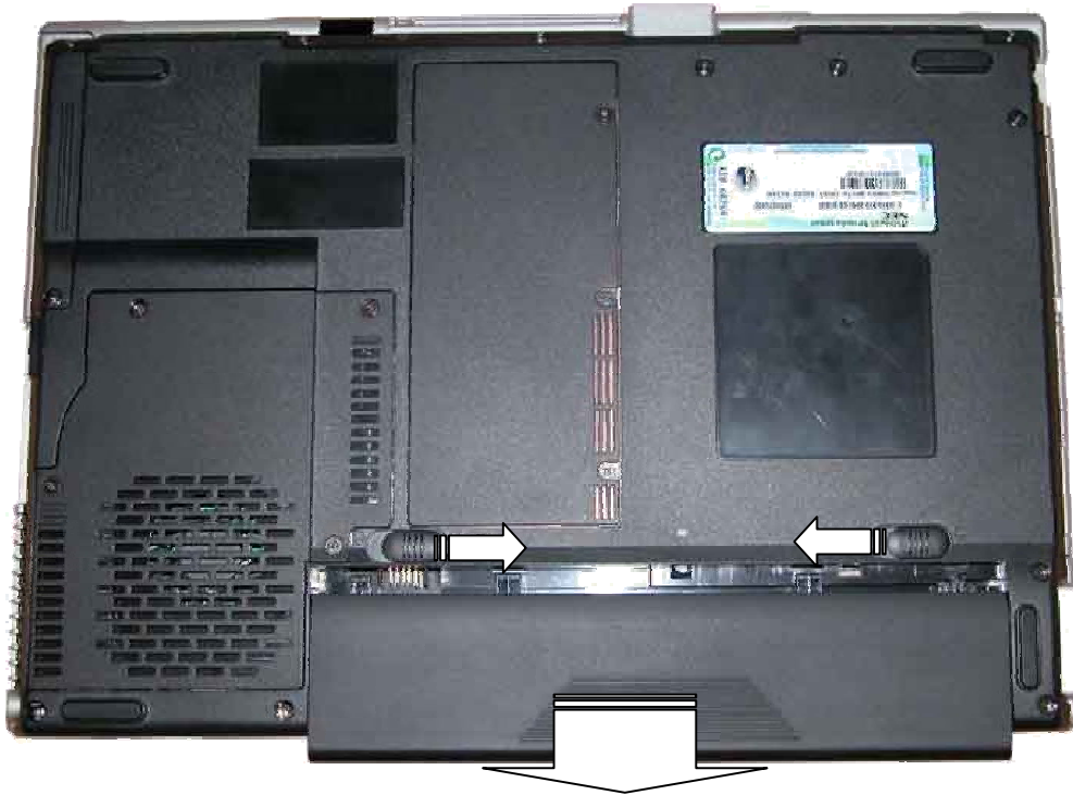
Fig. 1 Removing the battery
