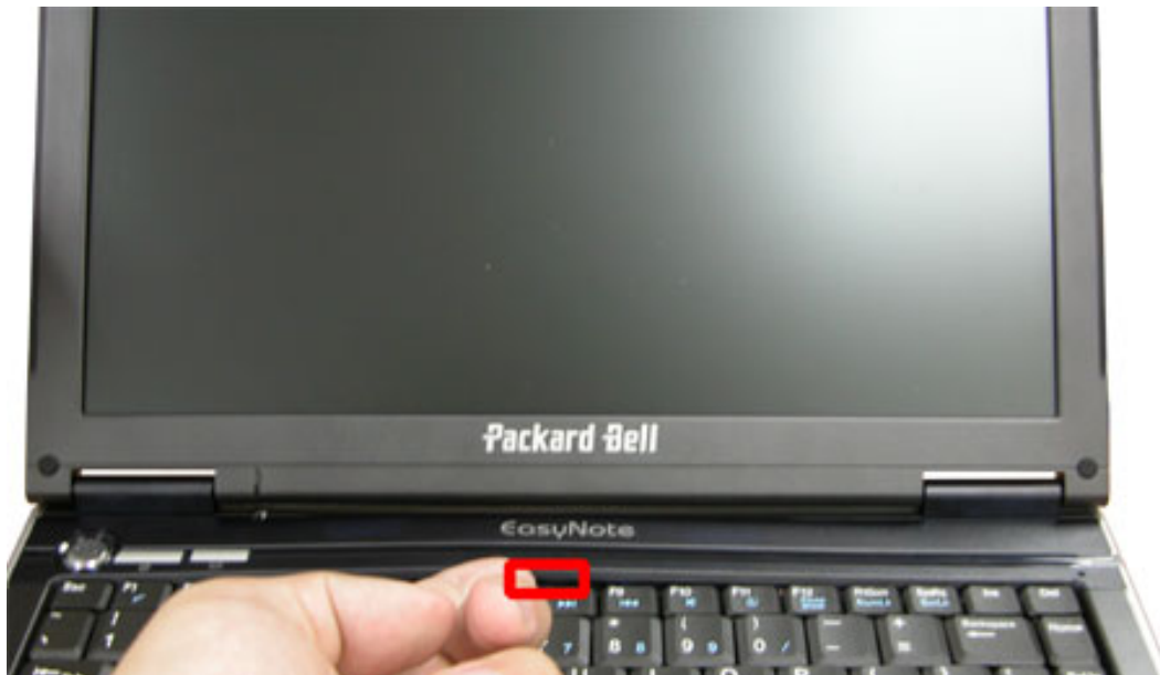
Fig. 14 Lifting up the Keyboard Cover
