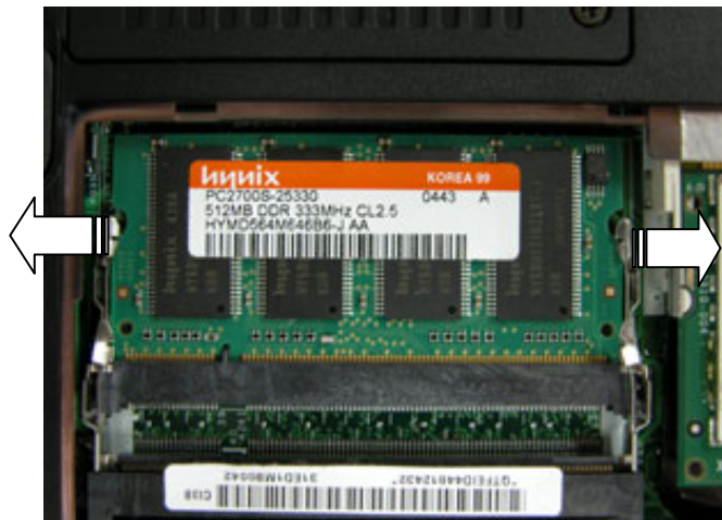
Fig. 3 Removing the memory module
