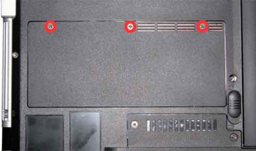
Fig. 2 Removing the screws retaining the memory module slot cover
