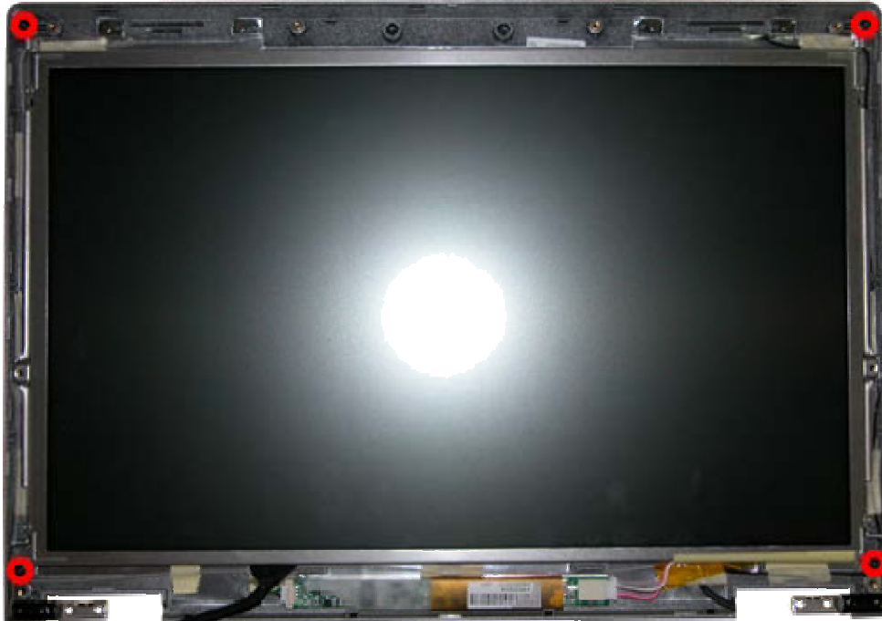
Fig. 22 Unscrew LCD Penal
