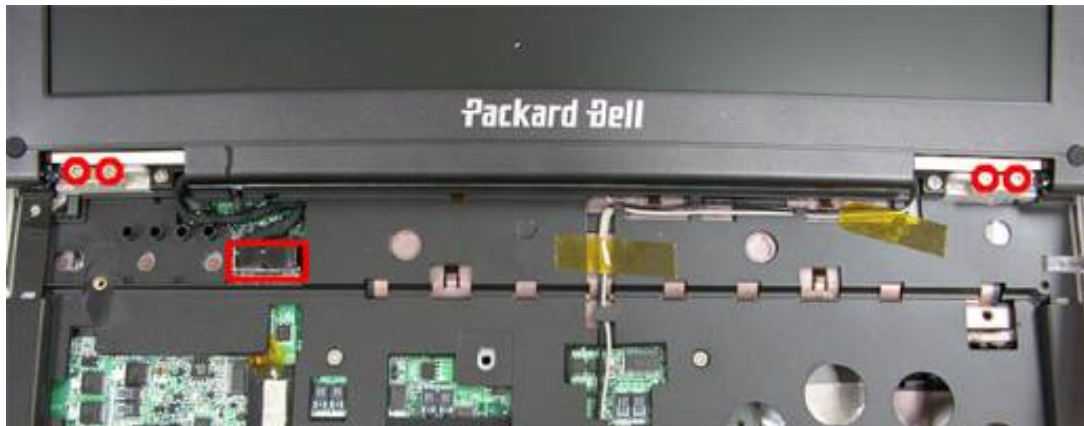
Fig. 19 Removing the screws retaining the LCD module
