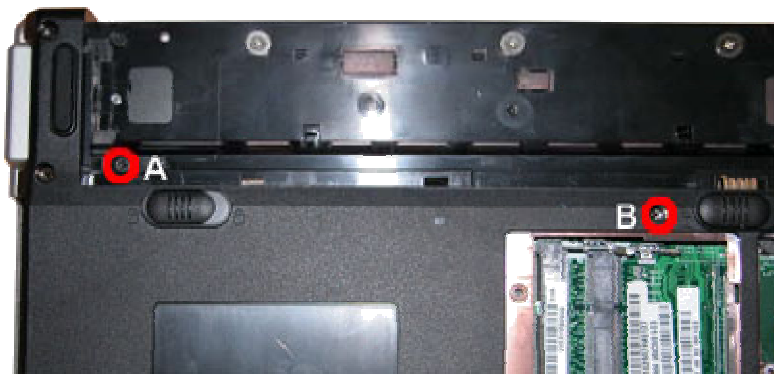
Fig. 15 Unscrewing Keyboard screws
