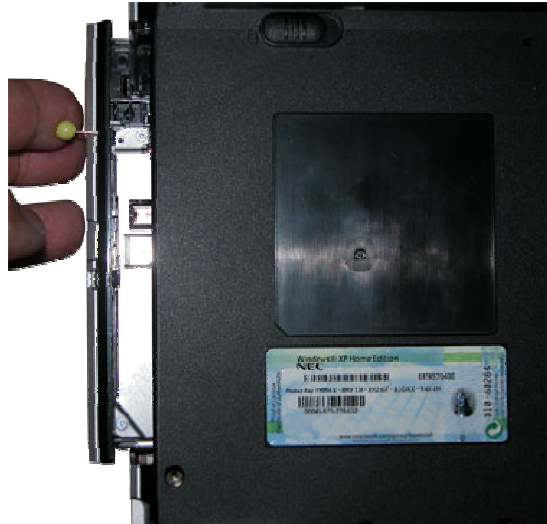
Fig. 8 Eject the optical drive
