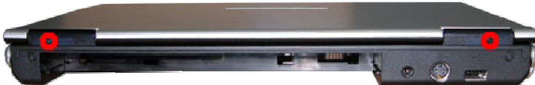
Fig. 13 Releasing the keyboard cover
