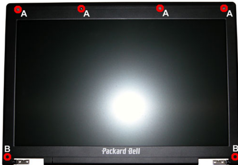
Fig. 20 Removing the rubber covers & screws on the LCD Module
