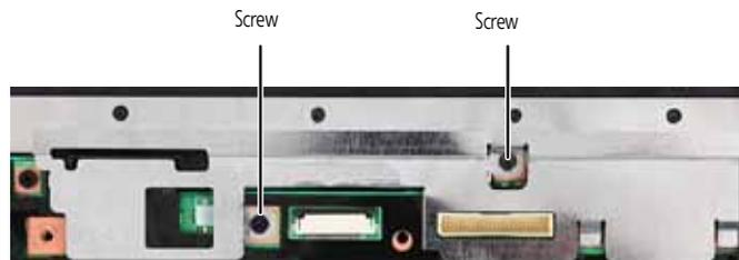
19 Remove the system board screws.
