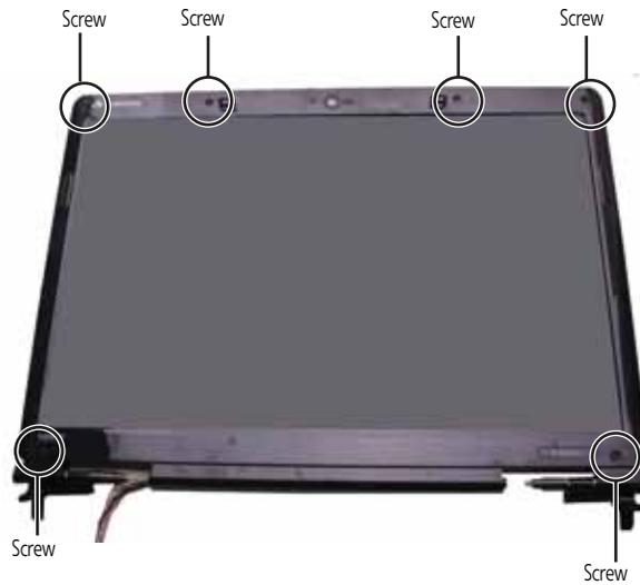
**8** Carefully separate the front and back of the LCD panel assembly.
