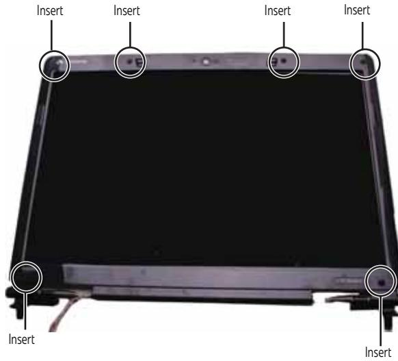
**7** Remove the screws from the front of the LCD panel assembly.
