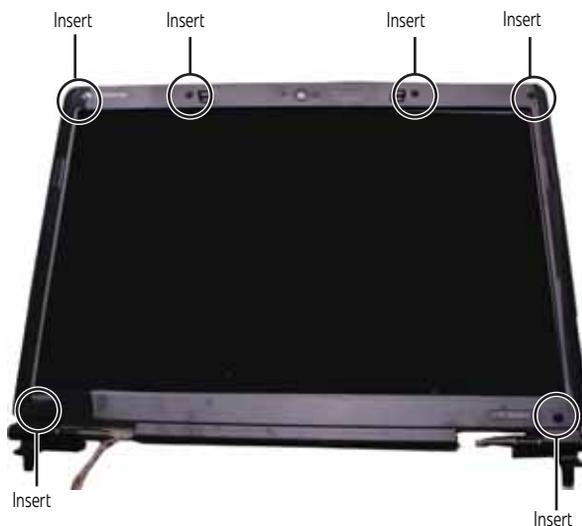
**5** Remove the screws from the front of the LCD panel assembly.
