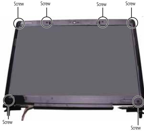
**6** Carefully separate the front and back of the LCD panel assembly.
