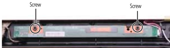
**8** Lift the inverter from the LCD panel assembly, then turn it over.
