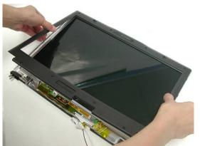
3. Remove 6 screws [M2.5  $^{\star}$  6(L)] on LCD module.
