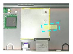
2. Disconnect the MAIN & AUX Antenna and open the two latches to pop the MINI PCI MODULE up then pull it out.
