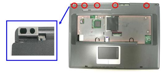
8. Remove the speaker cable & touchpad cable on top case.
