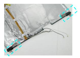
9. Remove 3 tapes and take away the CCD module from LCD back cover.
