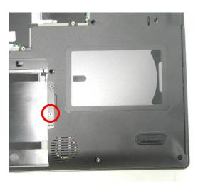
2. Put the screw driver here and push the ODD drive out from the NB.
