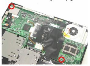
5. Remove the motherboard from the bottom case.
