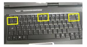
3. Lay the keyboard down over the touch pad module. Do not remove the keyboard yet. The keyboard FPC is still attached.
