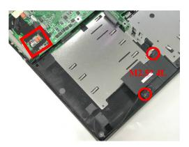
2. Remove 3 tapes and disconnect the CIR connecter then take away the CIR board.
