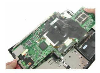
6. Remove 2 screws [M2 \* 4(L)] and remove the FAN module.
