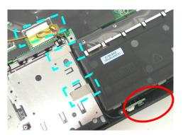
3. Remove 1 yellow tape and disconnect the FAN cable.
