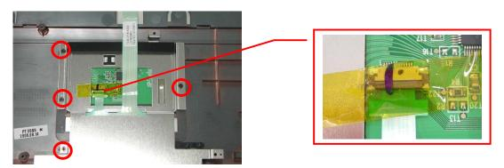
2. Separate the Touch pad board from the Touch pad bracket.
