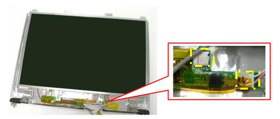
5. Remove 1 yellow tape and take away the LCD module from the LCD back cover.
