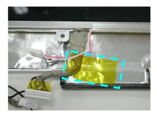
6. Turn over the LCD panel and remove 1 yellow tape then disconnect the coaxial FPC on the LCD panel.
