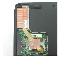
2. Remove 4 screws [M2 \*4(L)] by order and take the CPU heat sink module away.
