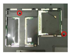
2. Turn over the NB and push the 3 latches in with a pair of tweezers or a single-slotted screwdriver and lift the keyboard up.
