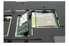
2. Remove the Memory module by opening the latches which will pop the module up to a  $45^{\circ}$  angle and then pulling out the module.
