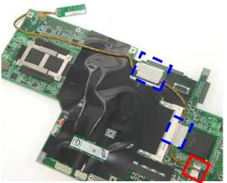
2. Remove 2 screws [M2 \* 4(W)] and disconnect the cable then take away the modem module.
