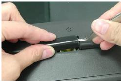
Remove 1 screws [M2 \* 4(L)] and disconnect the Coaxial cable & Inverter cable with tweezers.
