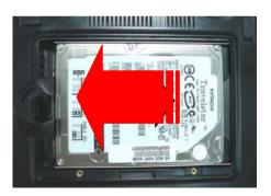
Disassembling HDD Module
