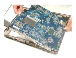
4. Remove 1 screw [M2 \* 4(L)] and remove DC-IN bracket.
