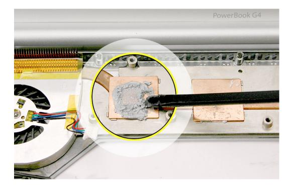
**Note:** X23 thermal grease (included with the logic board) is used for all three heatsink mating surfaces.
