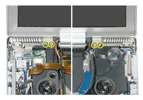
4. Lift off the display panel and clutch barrel assembly.
