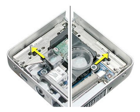
3. On the clutch, push the limit stop feet all the way back, on both sides.
