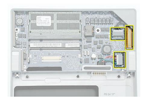
2. Turn the computer over. Disconnect the cables shown.
