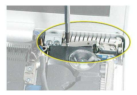
9. Then, use a sturdy hex nut driver to press the torsion bar down flat (this places tension on the pop-up spring pin) and install the second screw. Do this for both sides.
