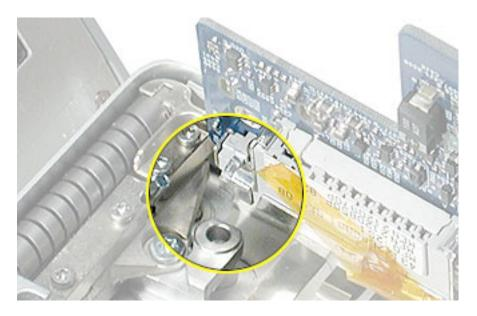
Warning: To avoid flexing the logic board, hold the board vertically along the wide sides. Do not hold the board by the ends or by the narrow neck at the blower cutout, or horizontally, as the board's weight can cause excessive flex.
