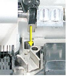
6. Install and tighten the screws for the clutch cleats, on both sides.
