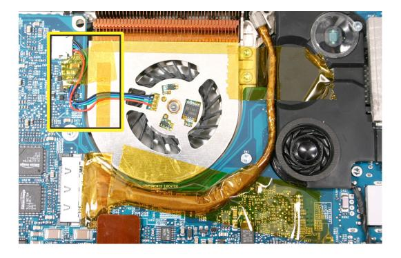
6. Verify that the LVDS cable is secured flat with Kapton tape and is not on the fan cover.
