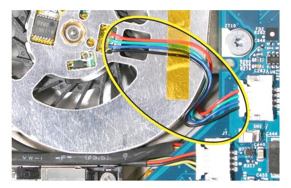
17. Verify that the right fan cables are secured flat on the fan cover with Kapton tape and do not cross over each other. Secure the excess cable off the fan cover and onto the logic board with Kapton tape, as shown.
