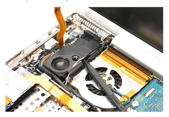
2. After removing the PC card cage, disconnect the AirPort Extreme and Bluetooth antennas from the AirPort Extreme w/ Bluetooth card.
