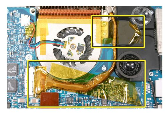
15. Verify that no cables ride up onto the fan covers. Tuck all cables that pass by the fan into the space, shown, and secure in place with Kapton tape.
