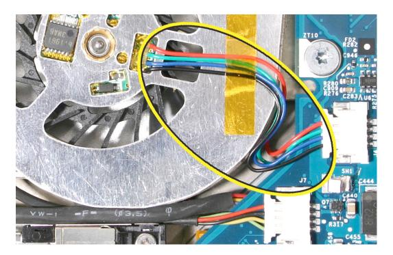
5. Verify that the right fan cables are secured flat on the fan cover with Kapton tape and do not cross over each other. Secure the excess cable off the fan cover and onto the logic board with Kapton tape, as shown.
