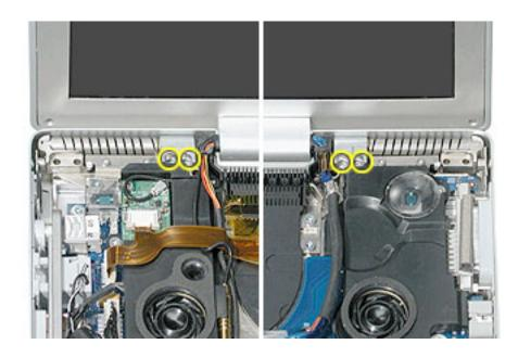
7. Hold the display at a 90-degree angle and install the end cap screws on both sides.
