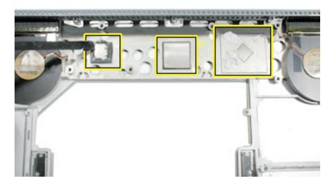
3. Center and install a new thermal pad onto the heatsink at the CPU mating surface, as shown below.
