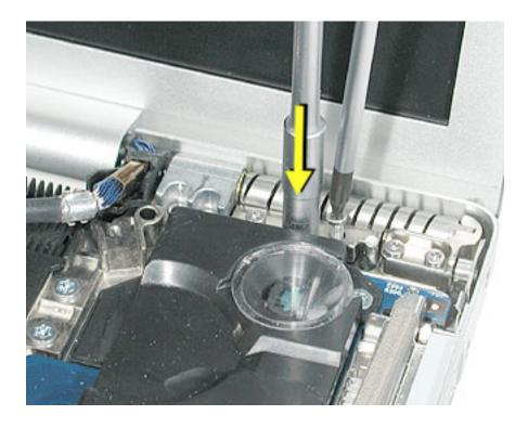
10. Replace the wire bracket screws on both sides.
