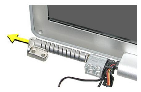
6. Remove the two screws and torsion bar on each side.
