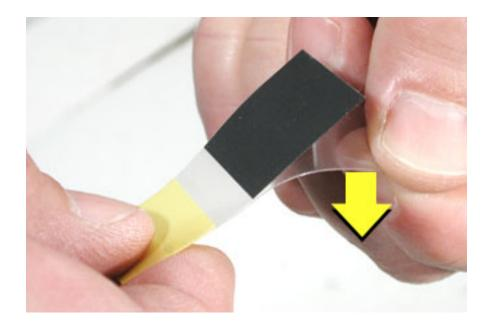
Center that side over the mating surface (raised surface) and evenly apply it, without air pockets, by lightly pressing. Remove any remaining backing. (The picture shown is for illustration only.)
