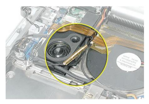
2. Carefully disconnect the Bluetooth cable connector.
