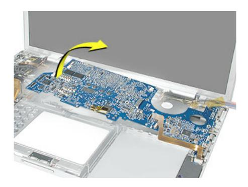
6. Carefully coax the port end of the board out of the port openings.
