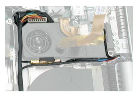
13. Verify that the LVDS cable's bead fits into the metal channel and that the cable is secured into the channel along the right speaker. Then, reconnect the LVDS cable.
