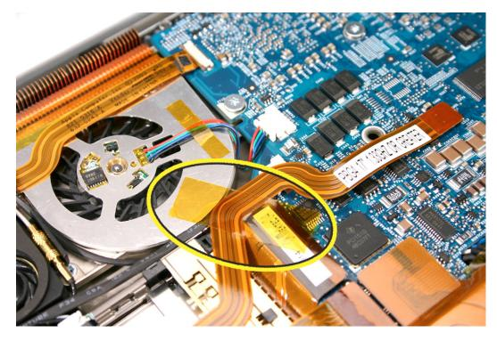
16. Verify that the left fan cables are secured flat on the fan cover with Kapton tape and do not cross over each other. Tuck the excess cable down into the space between the logic board and the fan, as shown.
