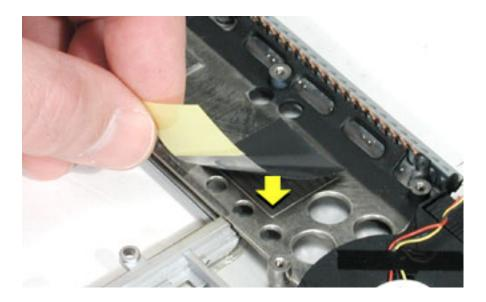
**Important:** With an razor knife, trim any excess thermal pad material, if any, that extends beyond the mating surface, to prevent it from touching holes in the heatsink.
