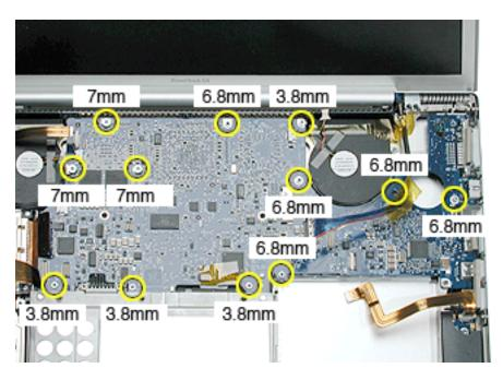
4. Insert a black stick just under the left edge of the logic board and apply slow upward pressure until the thermal material releases.
