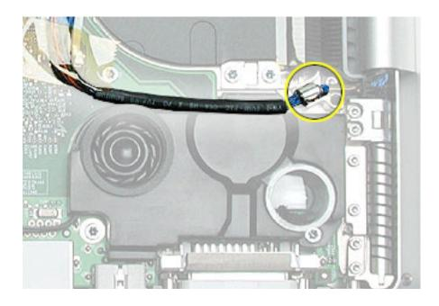
14. Verify that the LVDS cable is secured flat with Kapton tape and is not on the fan cover.
