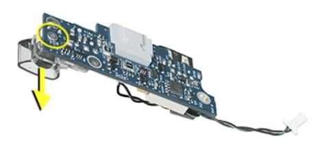
5. Install the replacement DC-in board, and reassemble the computer.
