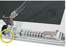
4. Lower the display panel assembly straight down onto the bottom case assembly.
