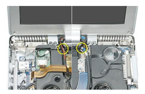
2. Move the display to a 90-degree angle and remove the two screws for the end caps of the clutch springs on each side.
