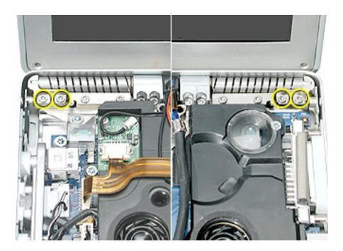
3. Remove the two clutch cleat screws on each side of the clutch barrel.
