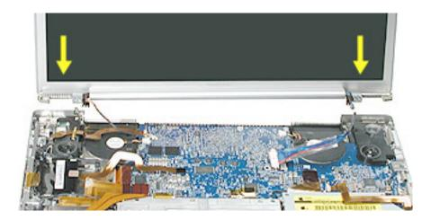
5. Verify that the limit stop feet, fit into the holes in front of the pop-up spring pins, on both sides.
