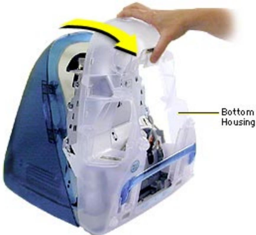
2. Press down on the tab at the top of the housing and pull the bottom housing toward you.
