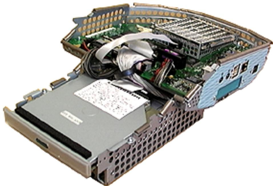
4. Place the logic board/mass storage unit on an ESD mat.
