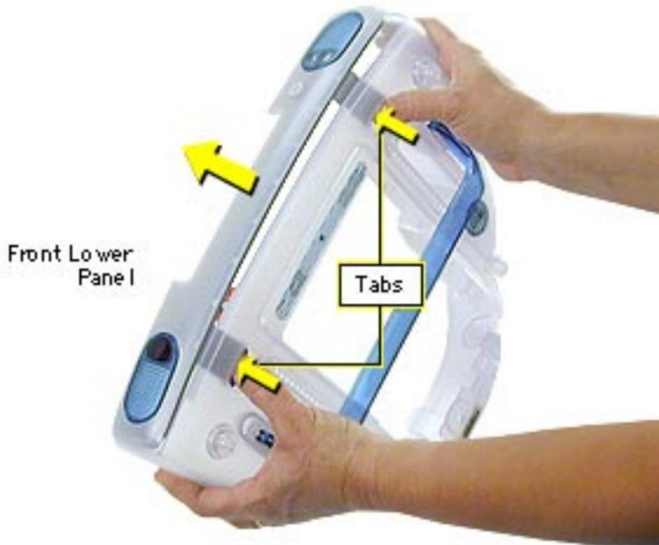
4. Push in on the front lower panel tabs to remove the front lower panel from the bottom housing.
