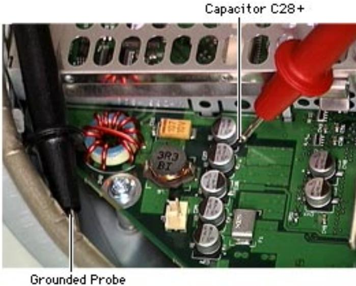
**Testing for Power at the Logic Board**
