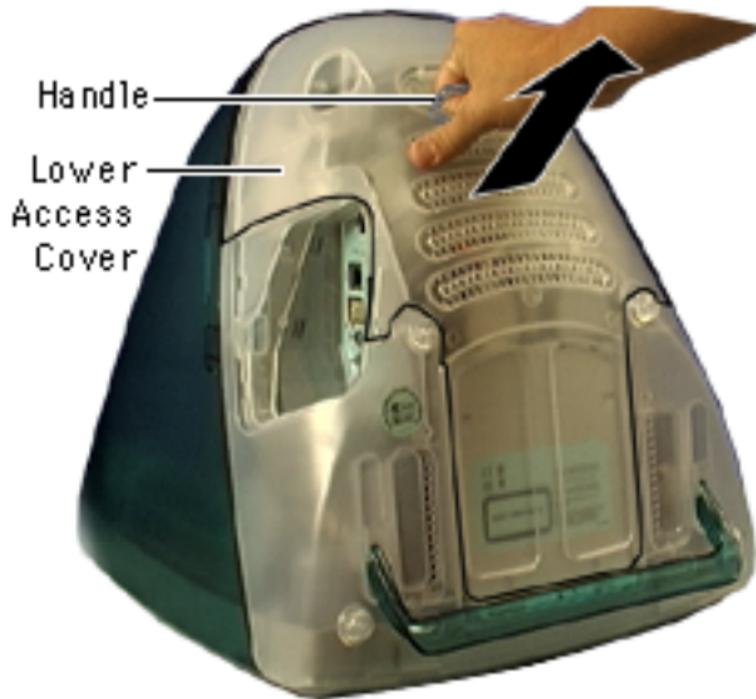
2. Using the handle, quickly jerk the lower access cover up and towards you.
