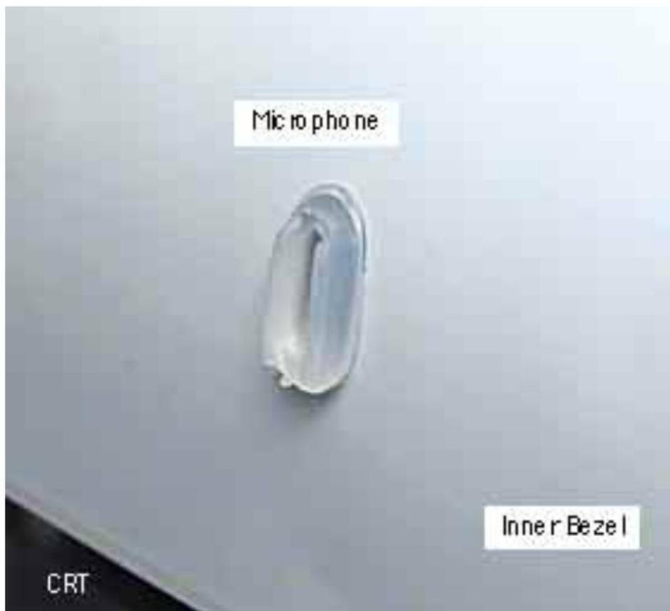
3. Check that the microphone protrudes through the inner bezel hole.
