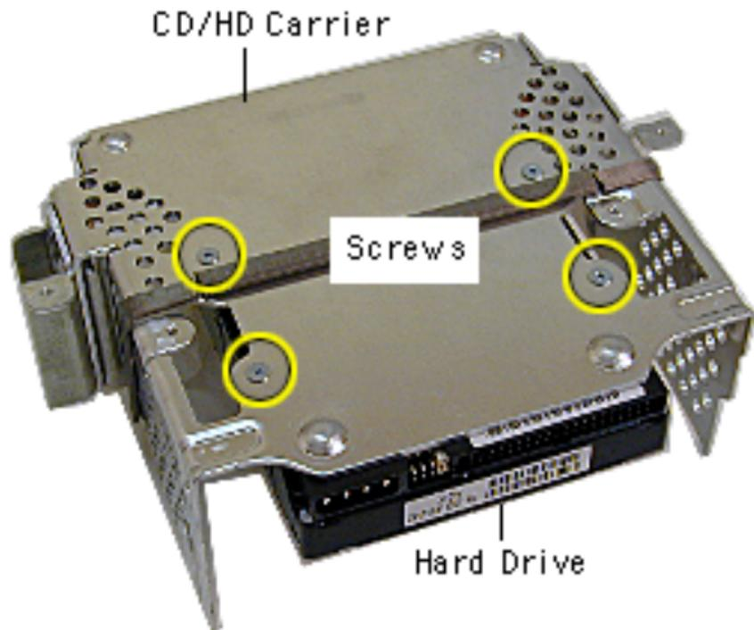
**Note:** The hard drive carrier shown was removed from the computer. However, you can easily remove the hard drive while the carrier is still screwed down to the chassis. Continue with the procedure.
