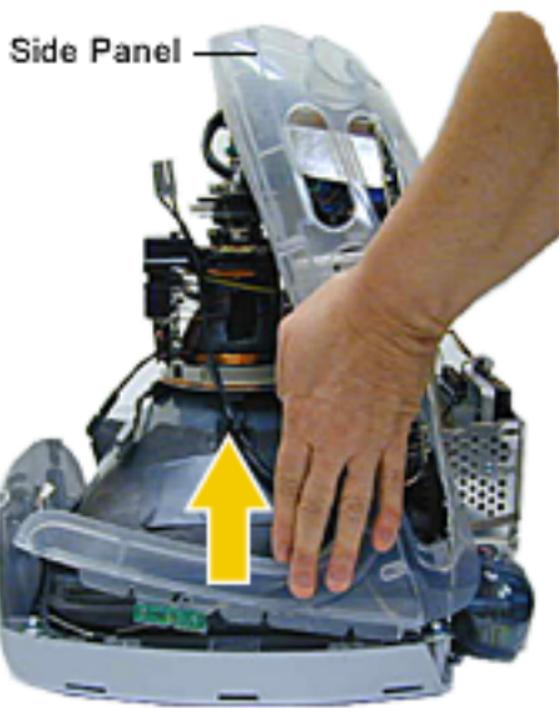
14. Holding on to the side panels, lift the power/analog/video board (which is attached to the side panels and divider panel) from the inner bezel.
