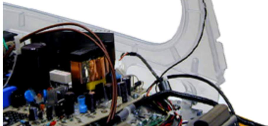
6. Carefully remove the antenna wire from each side panel.
