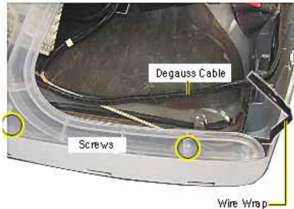
1. Undo the wire wraps in the top corners or the CRT.
