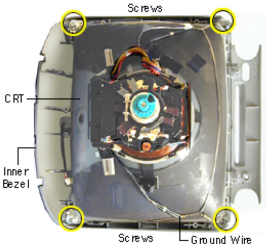
1. Remove the four CRT screws.
