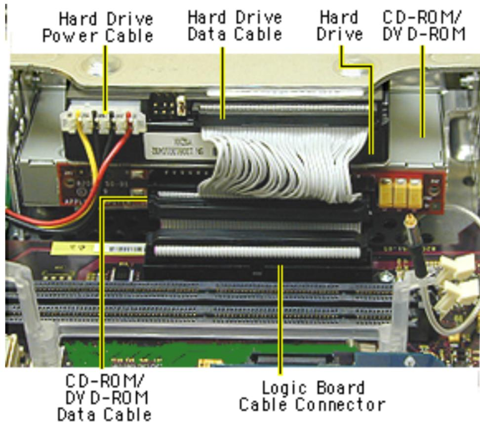
1. Disconnect the following cables on the back of the hard drive:
