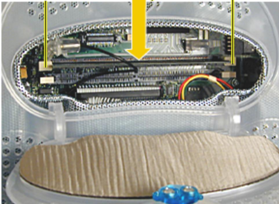
5. Align the notches on the memory module with the small notches inside the slot.
