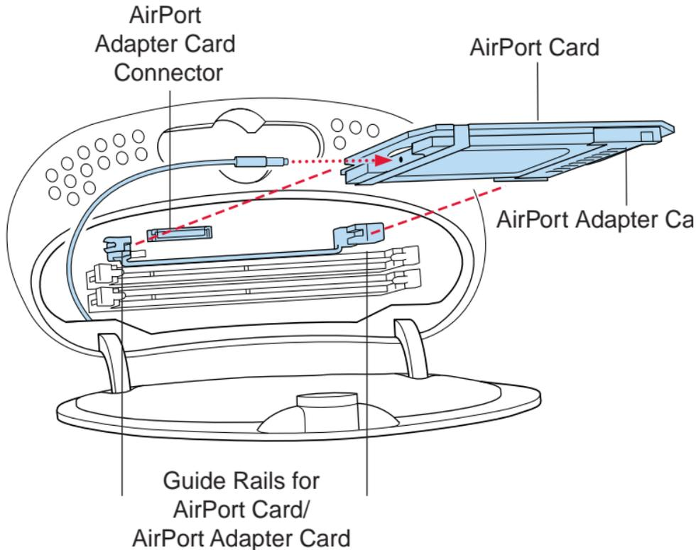
8. Align the edges of the AirPort Card with the guides on the AirPort Card slot. Insert the AirPort Card into the adapter Card connector.
