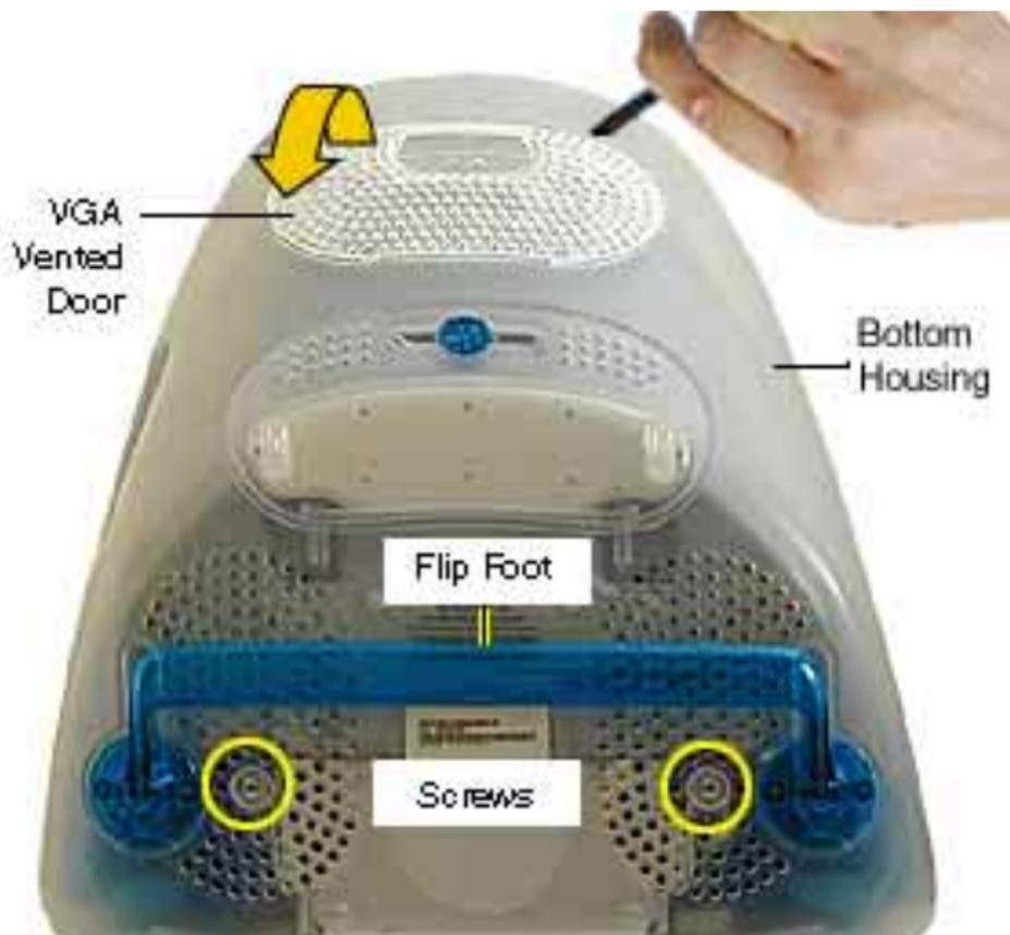
1. Using a plastic flatblade screwdriver, remove the VGA vented cover.
