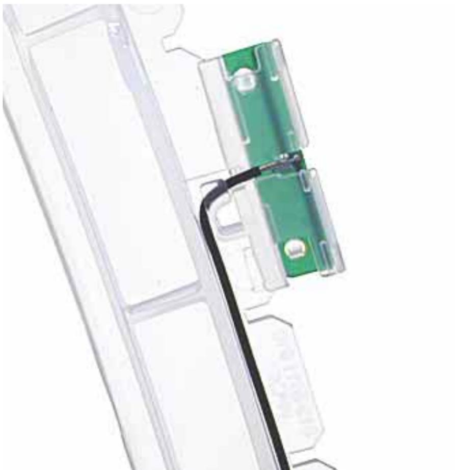
2. **Important:** Note how the antenna wire is routed through the side panel before removing. A close-up view of the right panel antenna is shown here.
