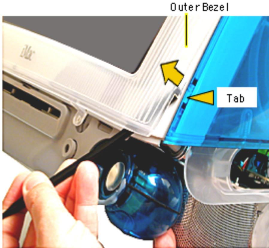
**Note:** The bezel tabs fit tightly into the rear housing. A good, hard pull upward is required to release all the tabs.
