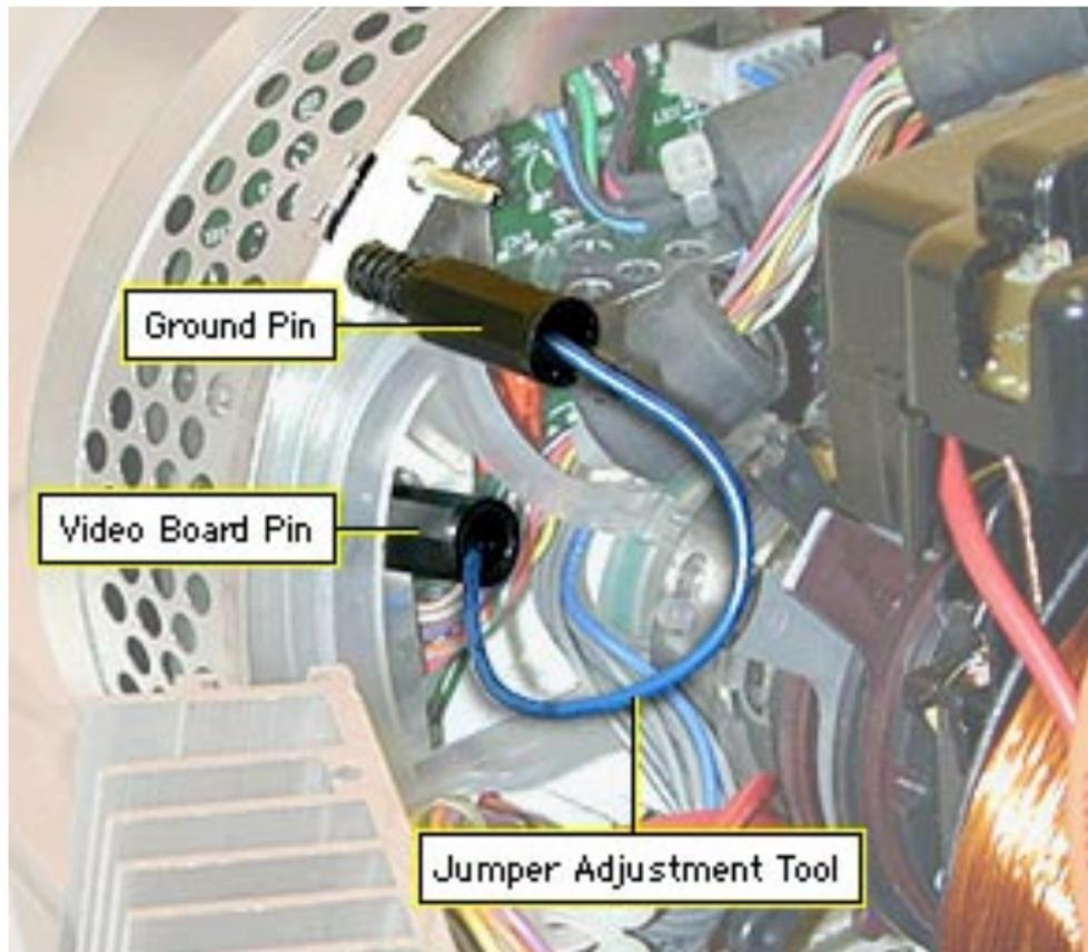
3. Connect the jumper adjustment tool (922-4165) to the video board pin. Refer to the “Jumper Adjustment Tool” procedure mentioned earlier in this section.
