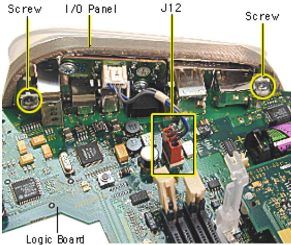
1. Disconnect the cable at J12, going from the logic board to the I/O panel.
