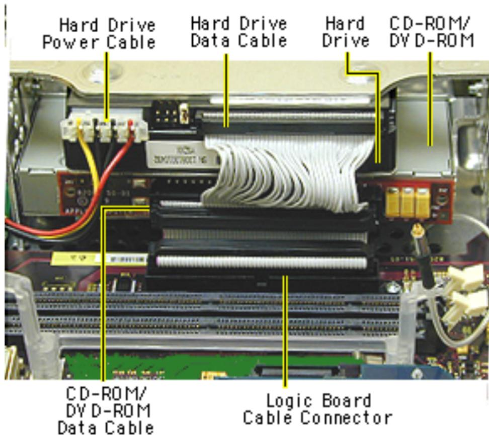
2. Disconnect the following cables from the back of the CD/HD carrier:
