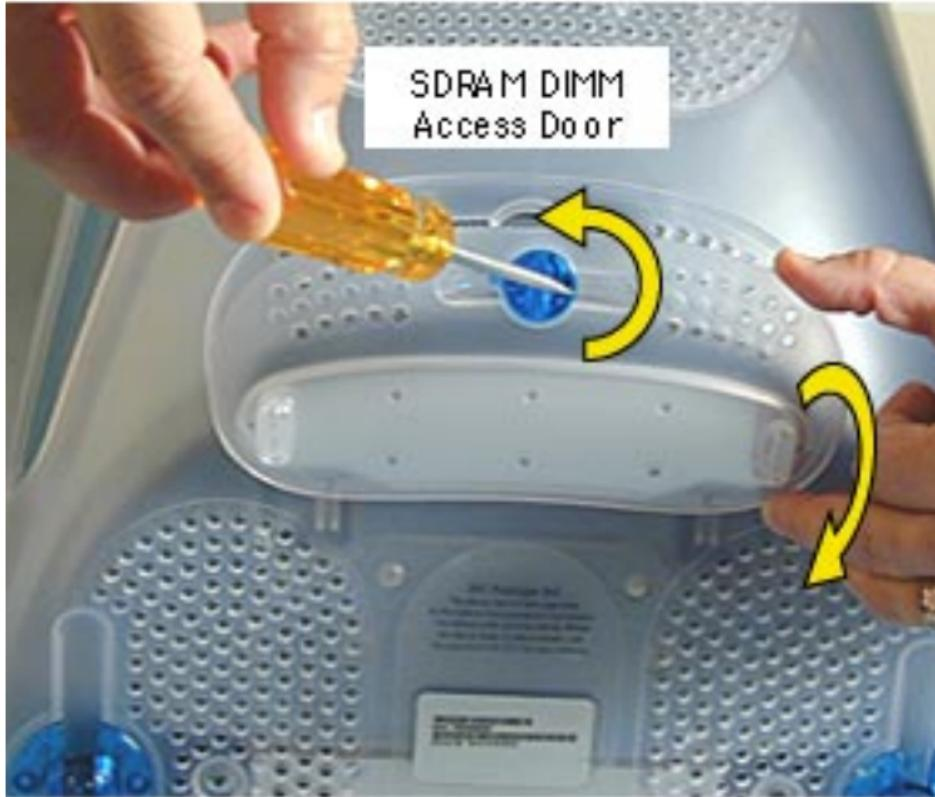
1. With a flatblade screwdriver or coin, turn the colored latch counterclockwise on the access door.
