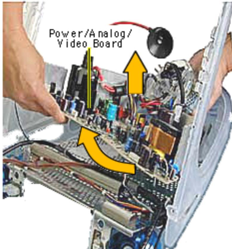
16. Lift the board from the flyback transformer side to clear the power plug from the side panel.
