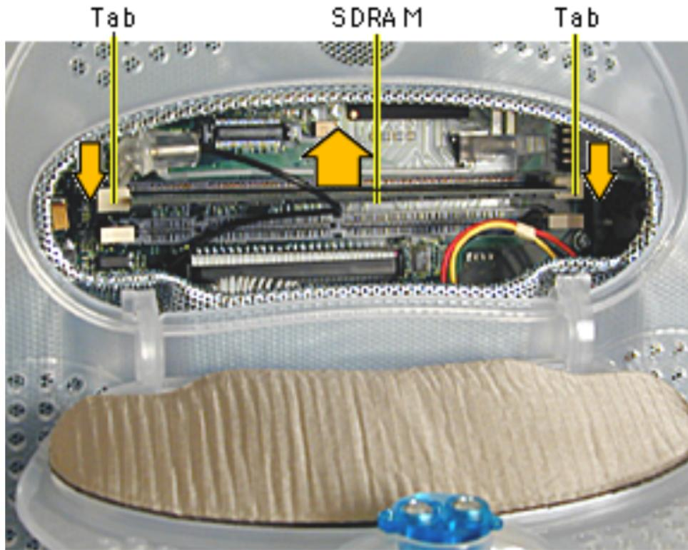
3. Push down on the plastic tabs to release the SDRAM module(s).
