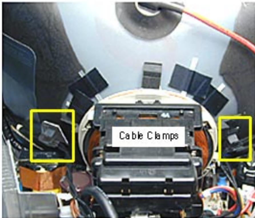
6. Open the CRT cable clamps. Remove the wires from the cable clamps.
