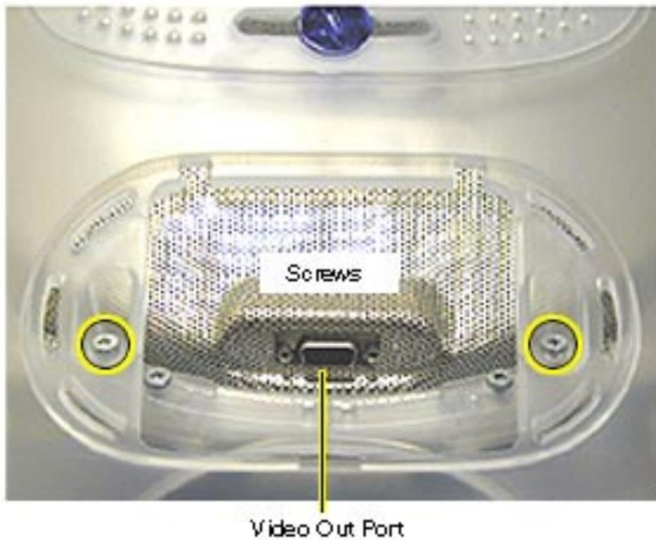
4. Remove the two outer screws located near the video out port.
