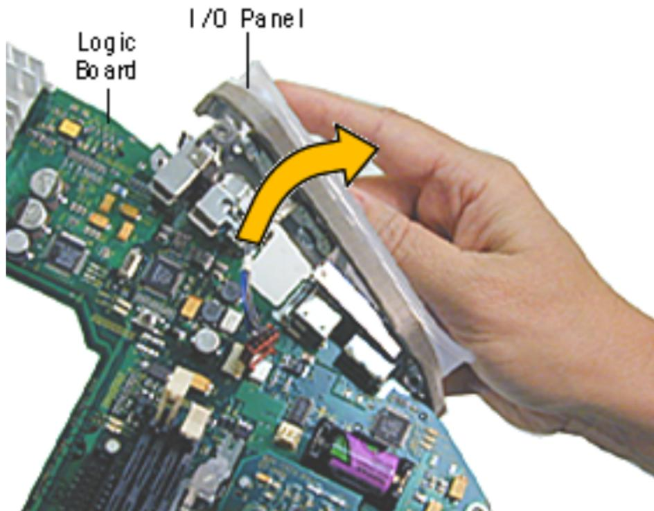
4. Rotate the logic board face up again and carefully slide the I/O panel off the logic board.
