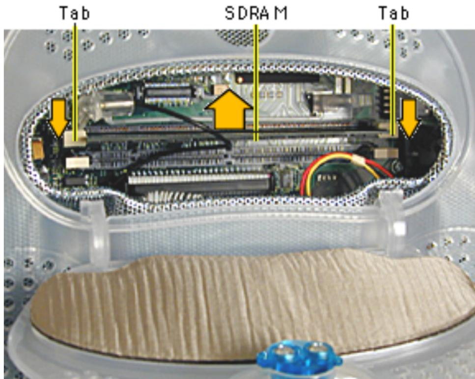
4. Push the ejector tabs on the slots outward and down so they are in the open position.
