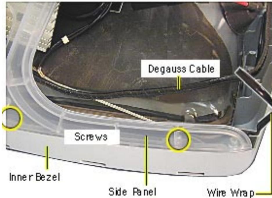
4. Lift the degauss cable out of the way to access the side panel screws.
