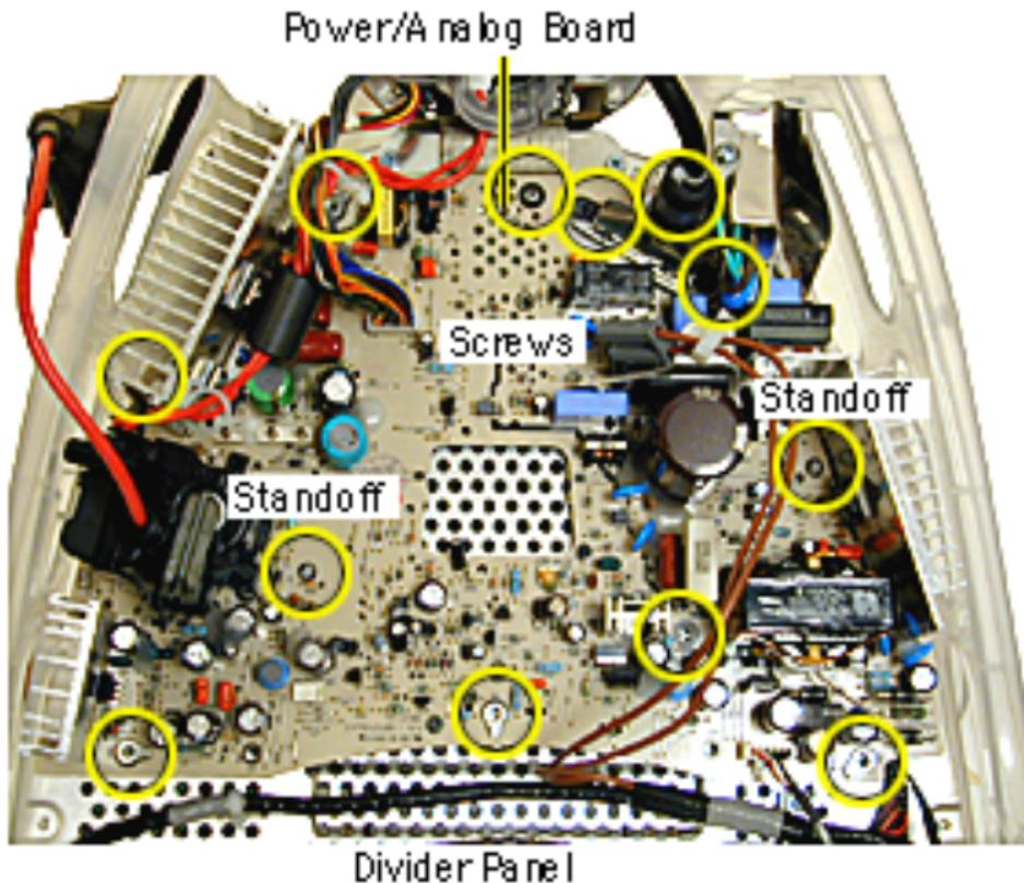
15. Remove the ten screws and pinch the two standoffs with a needlenose pliers to lift the power/analog board off the divider panel.
