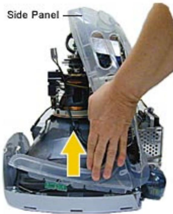
14. Holding on to the side panels, lift the power/analog/video board (which is attached to the side panels and divider panel) from the inner bezel.
