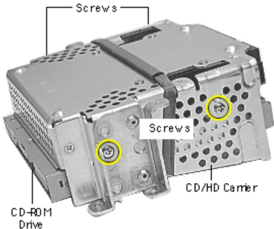
1. Using a Phillips screwdriver, remove the CD/HD carrier mounting screws (two on each side).
