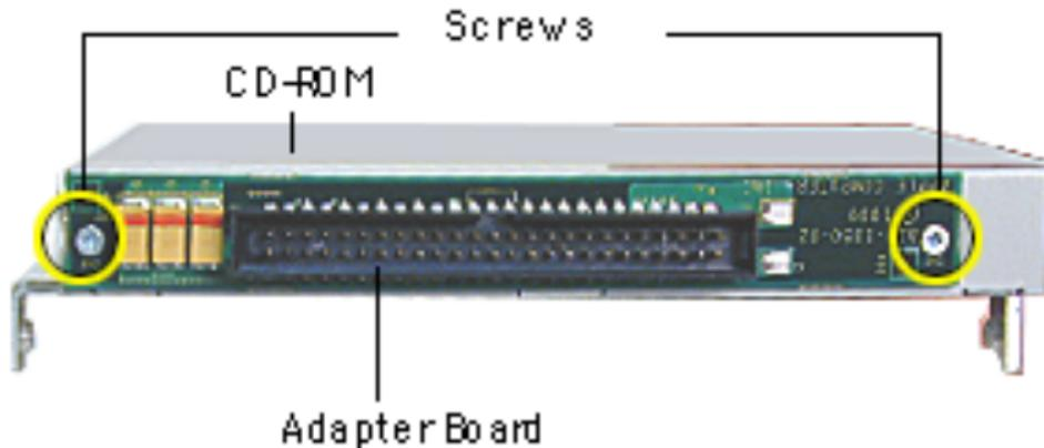
1. Using a jeweler's screwdriver, remove the two screws on the CD/DVD adapter board.
