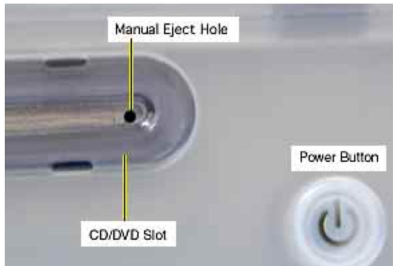
If the CD/DVD discs still won't eject after pressing the manual eject button, remove the bottom housing, and then replace the bottom housing ensuring that the center tab of the bottom housing is properly aligned.
