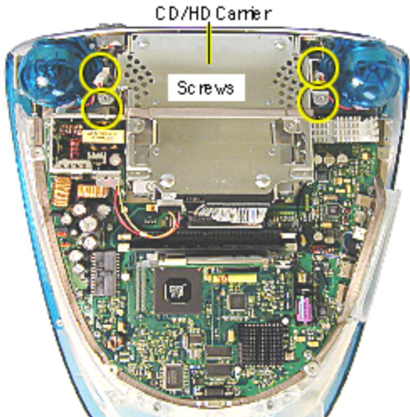
1. Remove the four screws connecting the CD/HD drive carrier to the metal chassis (also known as the divider panel).
