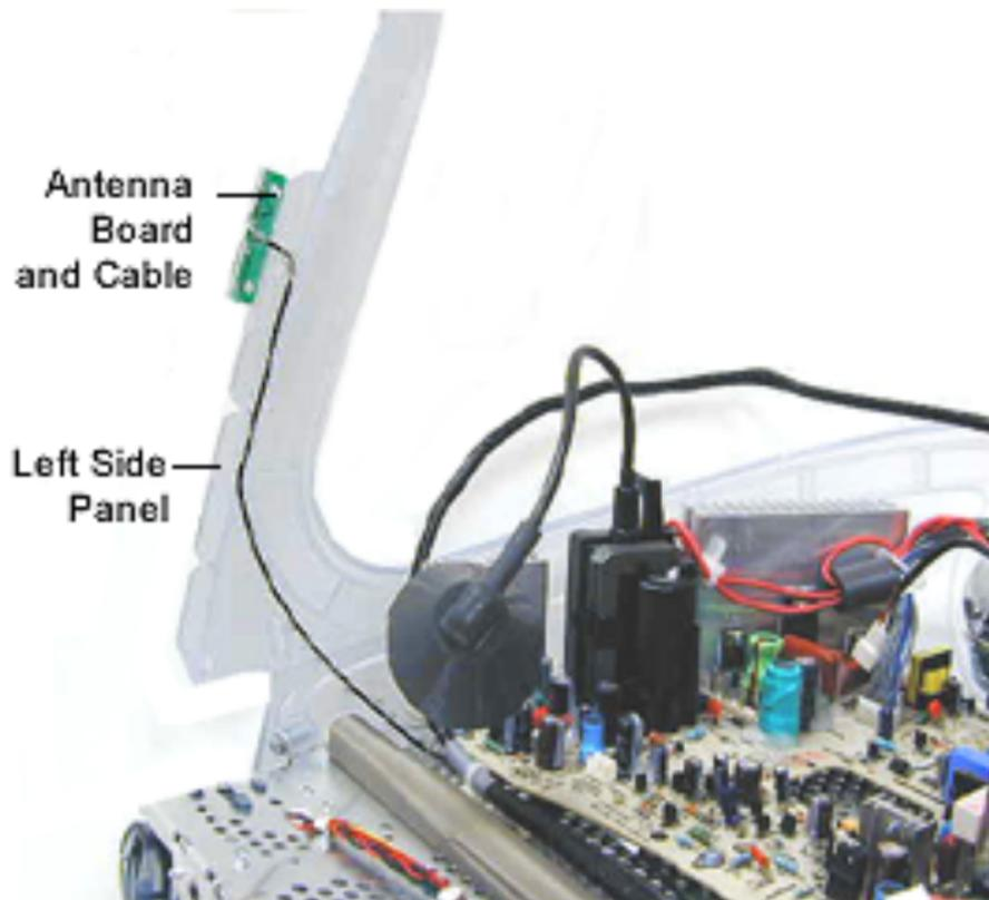
3. Carefully remove the antenna from the left side panel. Refer to the next page for a close up of the antenna in the left side panel.
