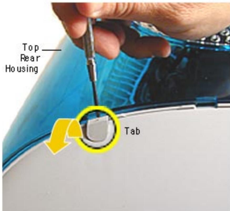
2. Pry the tabs off, and remove the two screws under each tab.
