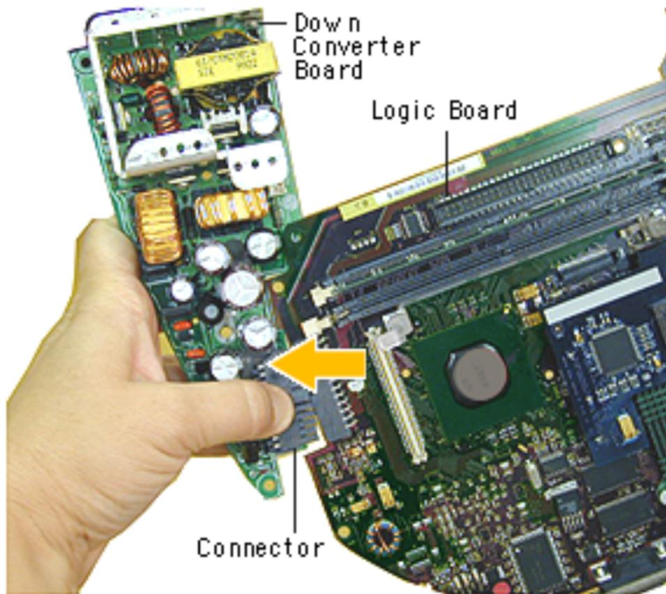
6. Holding onto the down converter, press down on the black connector to separate the down converter board from the logic board.
