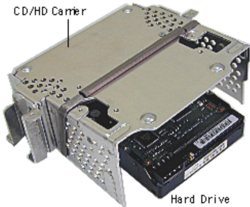
3. Slide the hard drive out of the CD/HD carrier.
