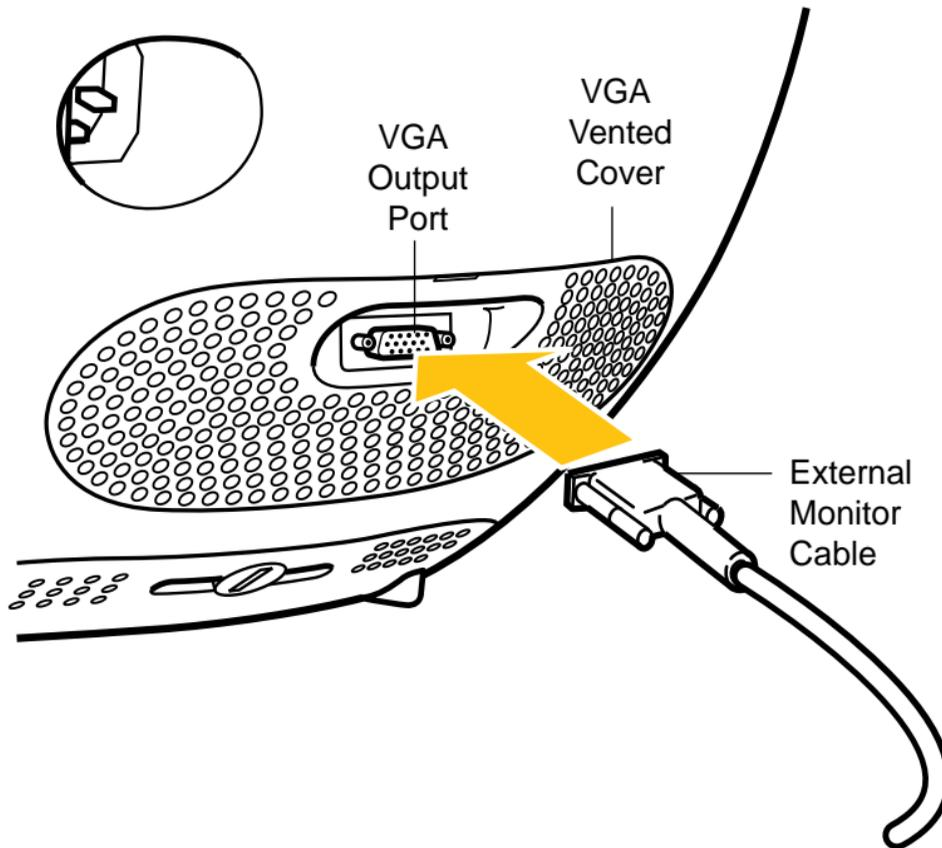
2. Plug the external monitor cable into the VGA output port on the back of the computer.
