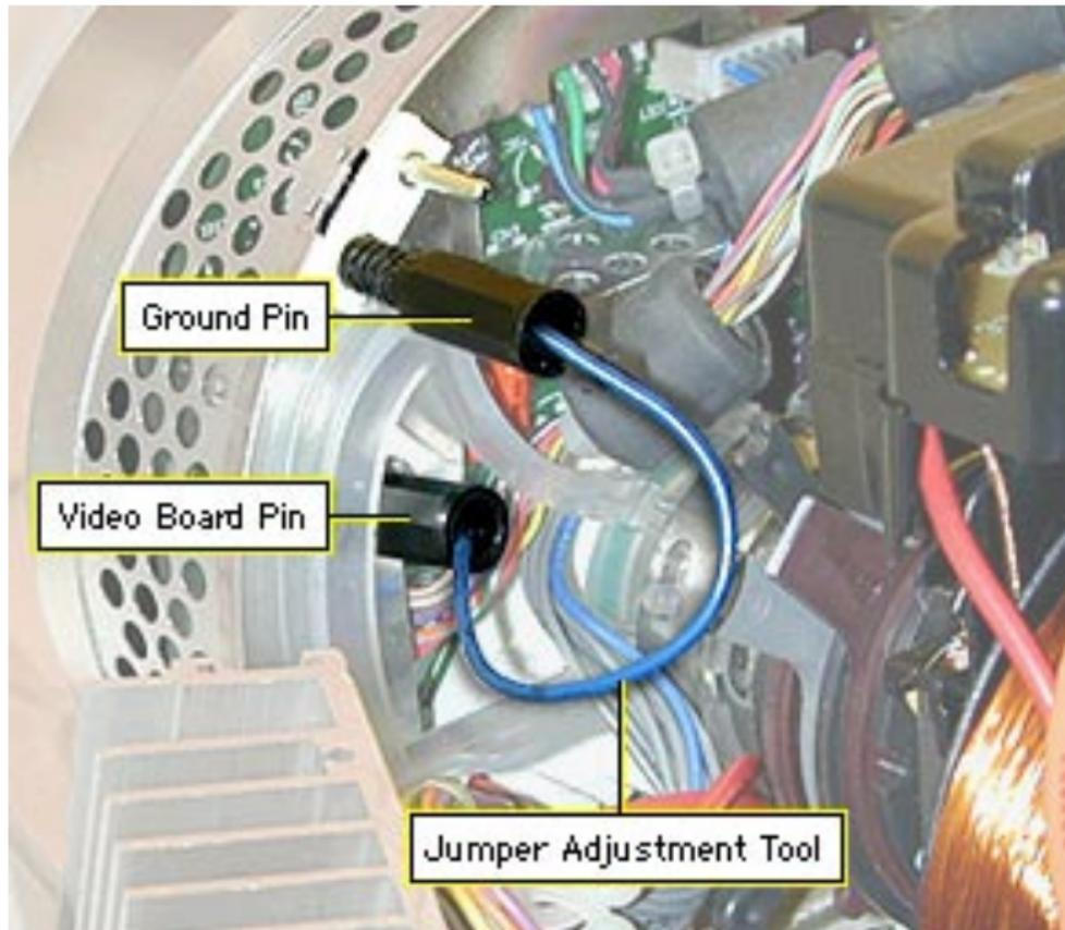
3. Connect one end of the jumper adjustment tool (922-4165) to the video board pin.
