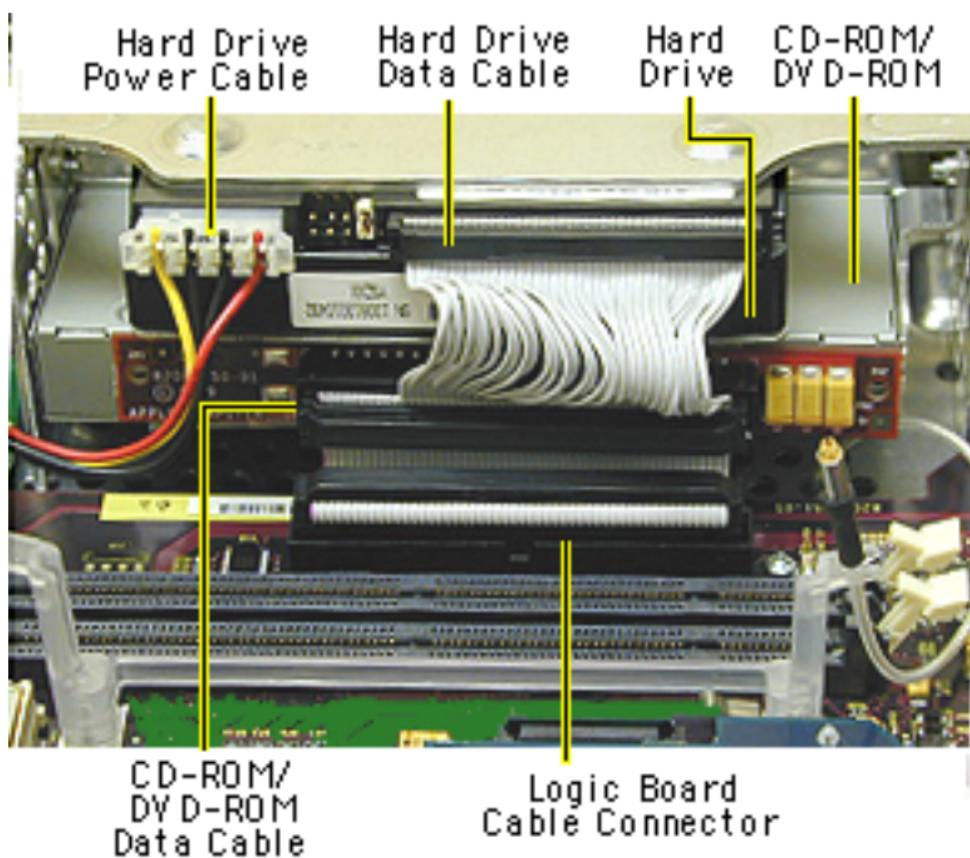
1. Disconnect the following cables on the back of the hard drive:
