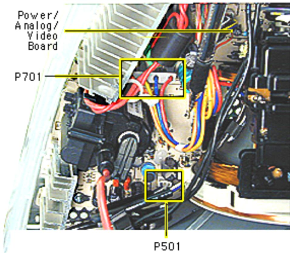
8. Disconnect P501 and P701 on the power/analog/video board. The cables are located near the high voltage capacitor.
