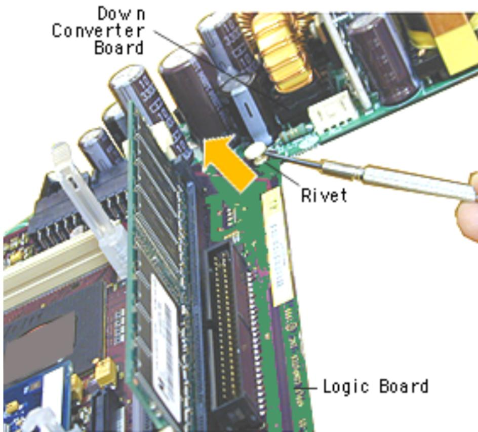
5. Using a flatblade screwdriver, pry the rivet off the logic board.
