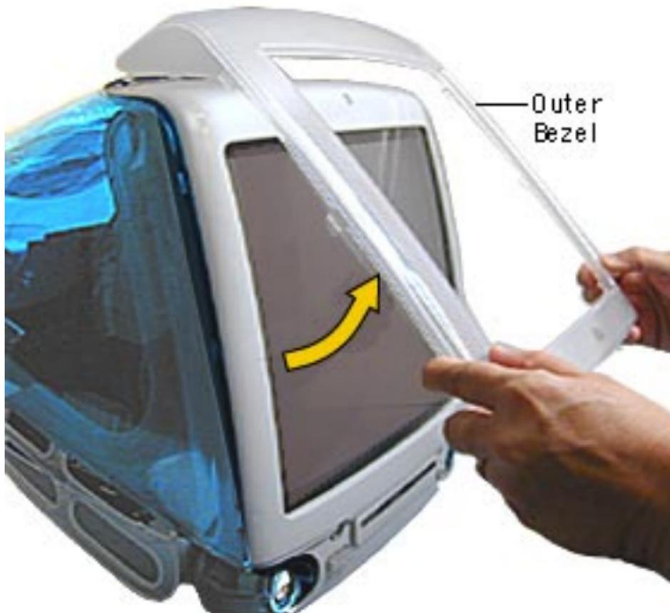
6. As the tabs start to release, pull hard on the front outer bezel to release the tabs completely.
