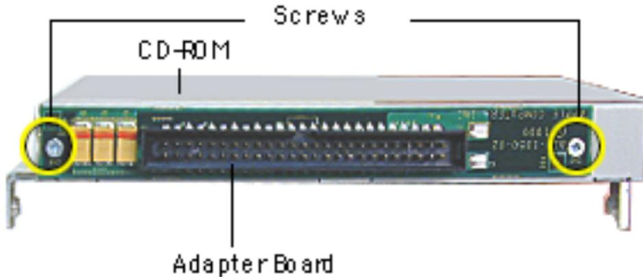
6. On the back of the CD-ROM, Use a jeweler's screwdriver to remove the two screws on the adapter board.
