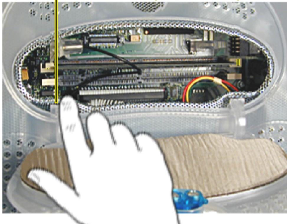
3. Touch the EMI cover that is visible inside the recessed latch area before touching any components on the main logic board. This protects the computer from damage caused by electrostatic discharge
