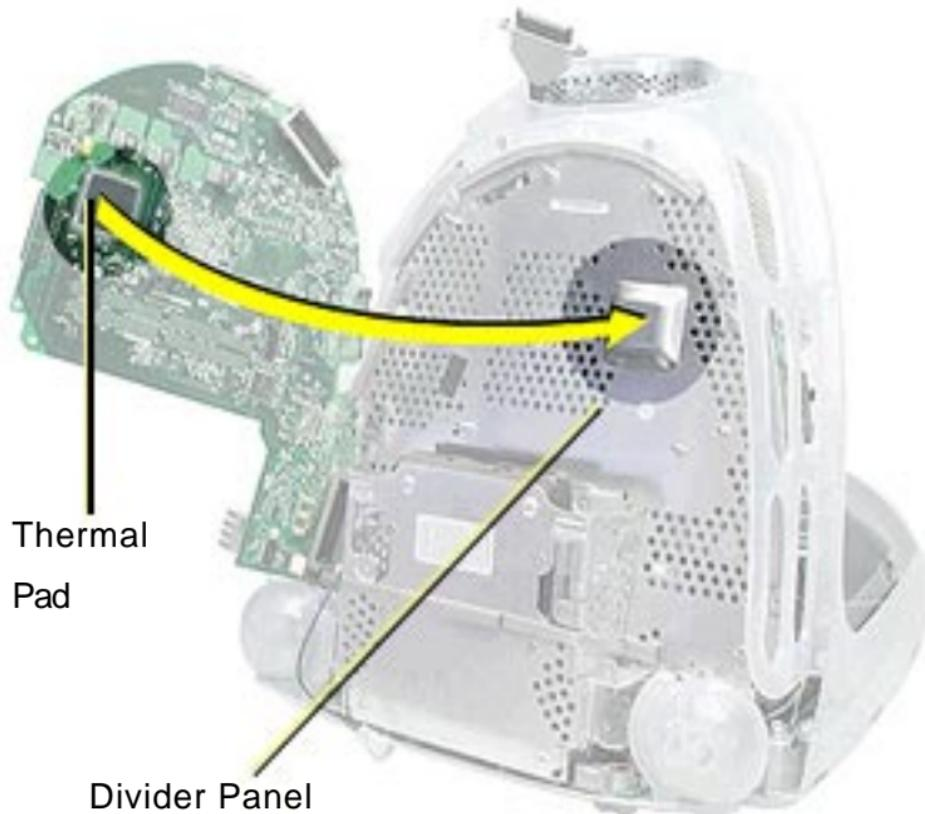
5. Install the logic board back on to the divider panel.
