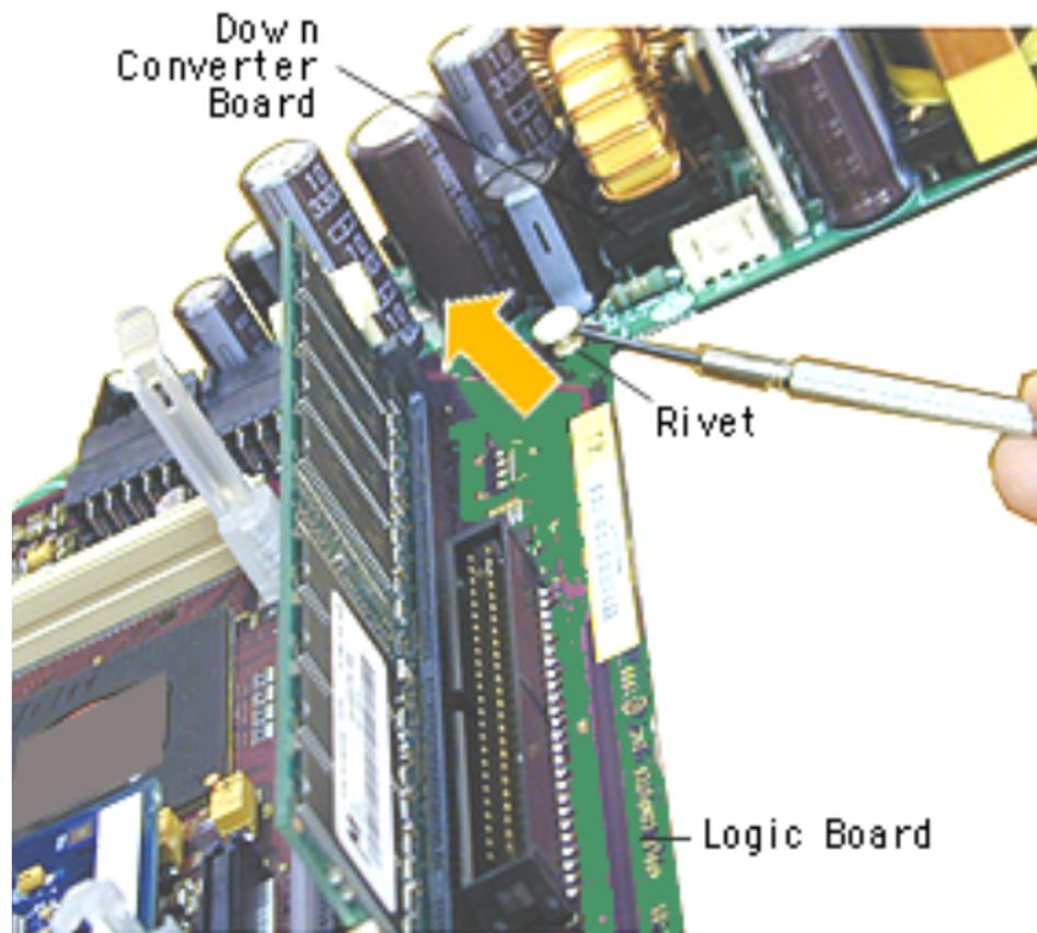
5. Using a flatblade screwdriver, pry the plastic rivet off the board.
