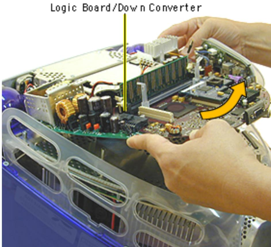
4. Gently lift the down converter board and logic board out of the computer.
