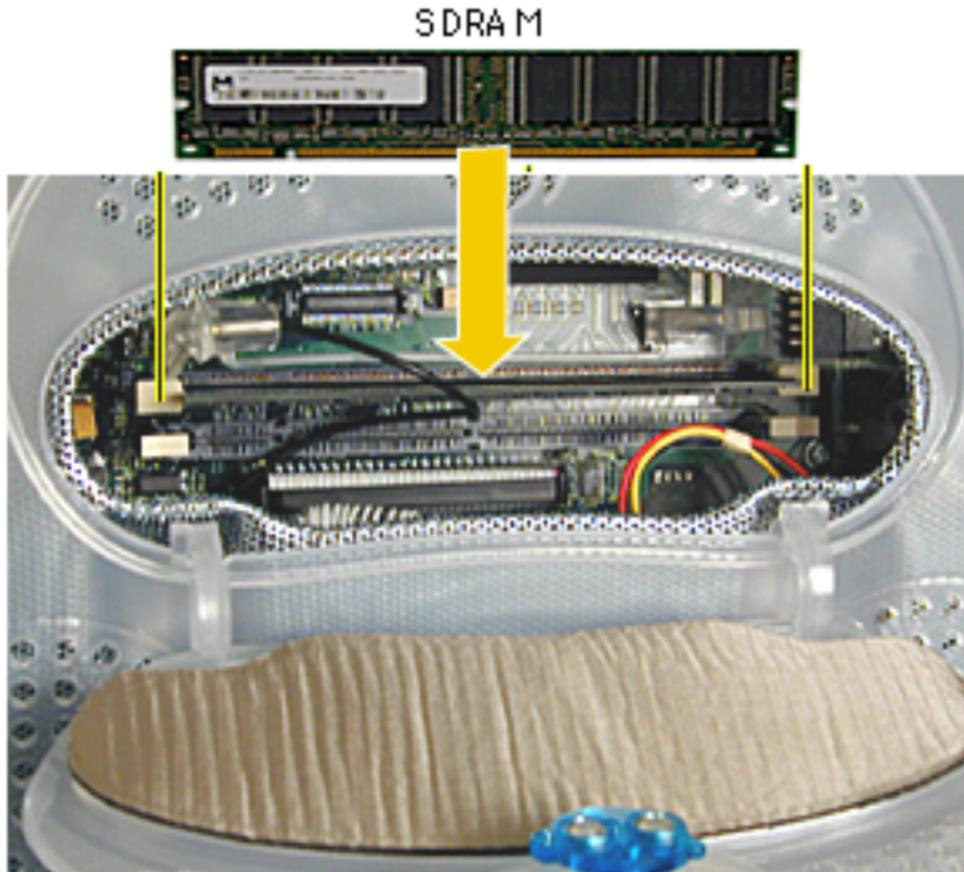
5. Align the notches on the memory module with the small notches inside the slot.
