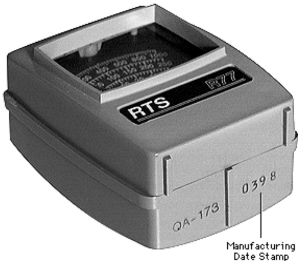
If you suspect the light meter is giving false readings, verify the readings with a known-good light meter or photometer. Also check the age of the R77 light meter by its four-digit manufacturing date stamp (such as 0398 for March 1998).
