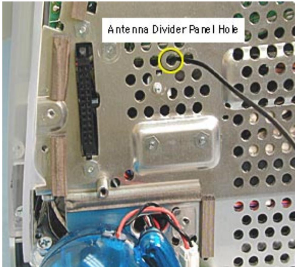
5. Before removing the antenna from the divider panel, mark the hole (with a pen tip) that the antenna passes through so you know which hole the antenna goes into when replacing the antenna.
