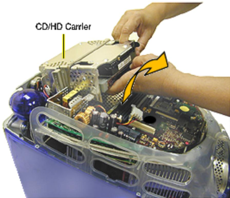
3. Tilt the CD/HD carrier forward and lift the carrier out of the computer.
