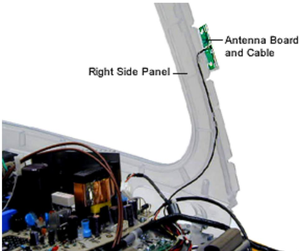
6. Carefully remove the antenna wire from each side panel.
