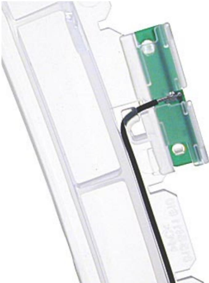
2. **Important:** Note how the antenna wire is routed through the side panel before removing. A close-up view of the right panel antenna is shown here.
