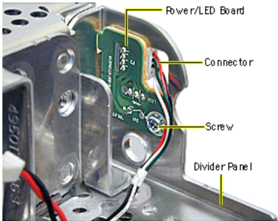
1. Turn the divider panel over and remove the speaker to access the power/LED board screw.
