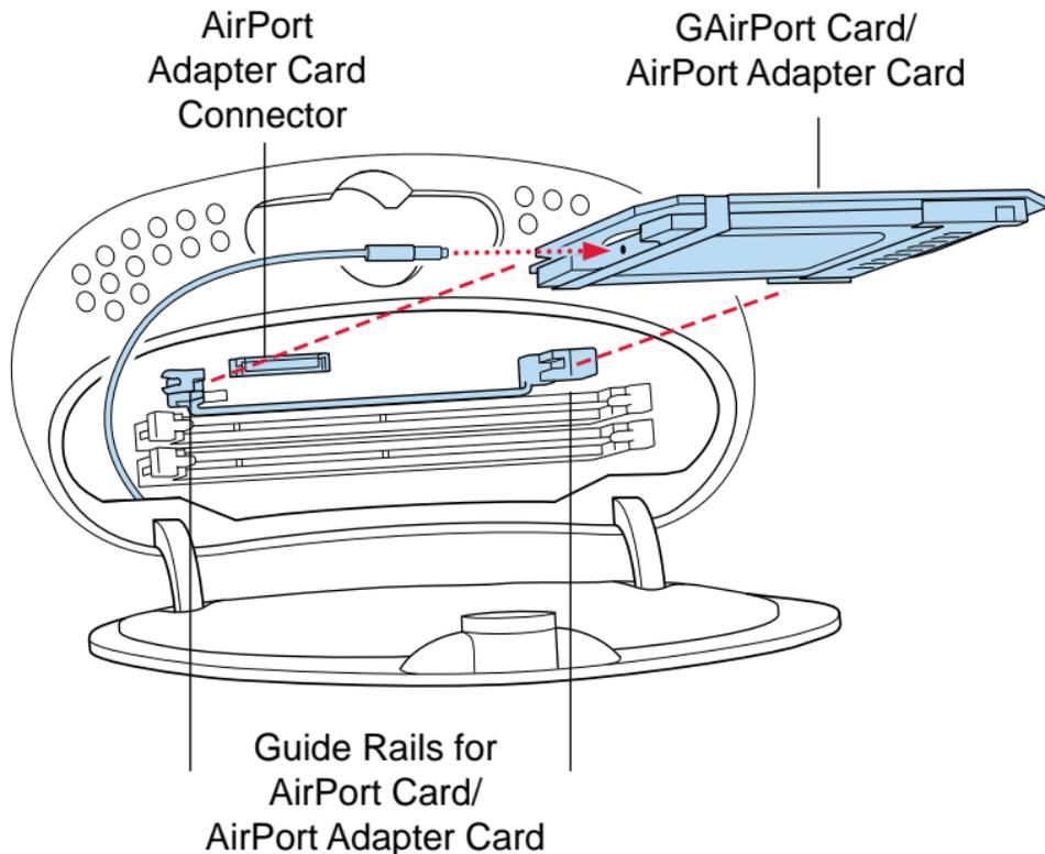
8. Align the edges of the AirPort Card with the guides on the AirPort Card slot. Insert the AirPort Card into the adapter Card connector.
