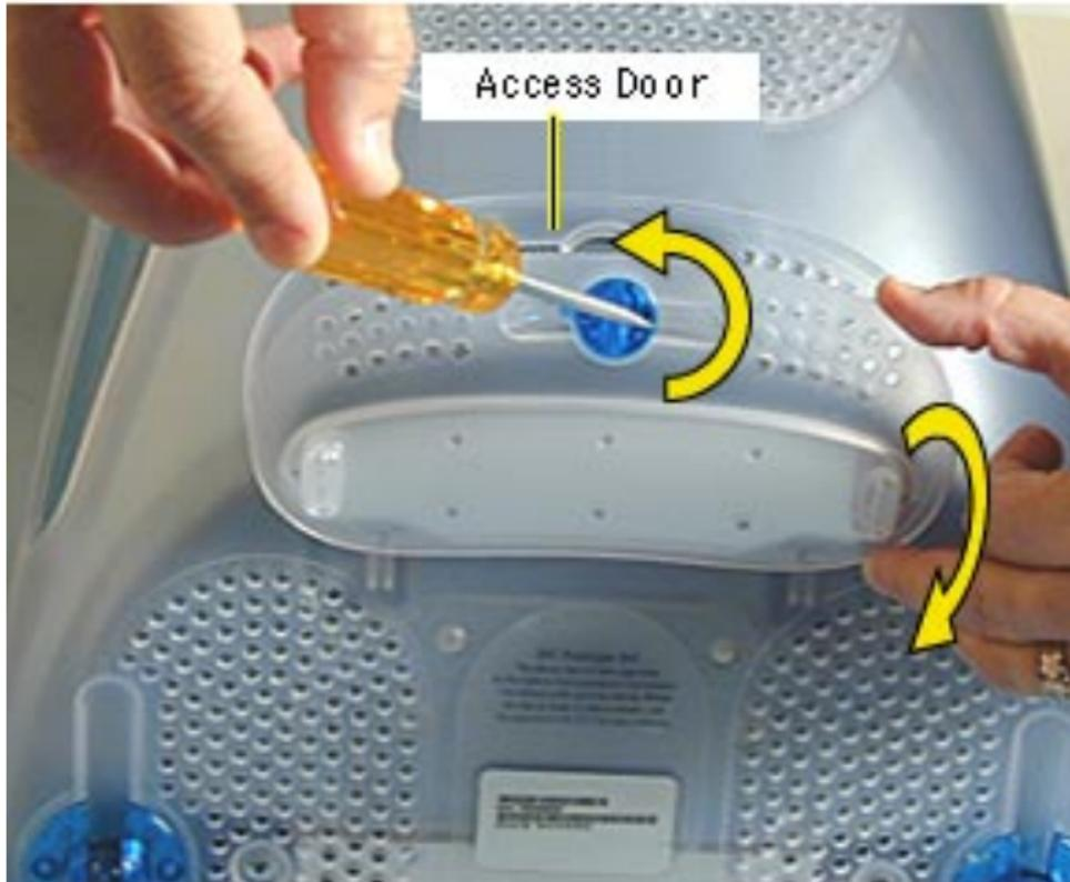
1. With a flatblade screwdriver or coin, turn the colored latch to open the access door.
