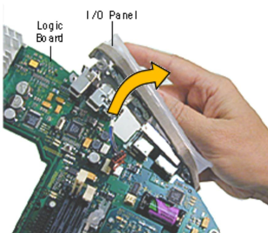
4. Rotate the logic board right side up again. Carefully slide the I/O panel off the logic board.
