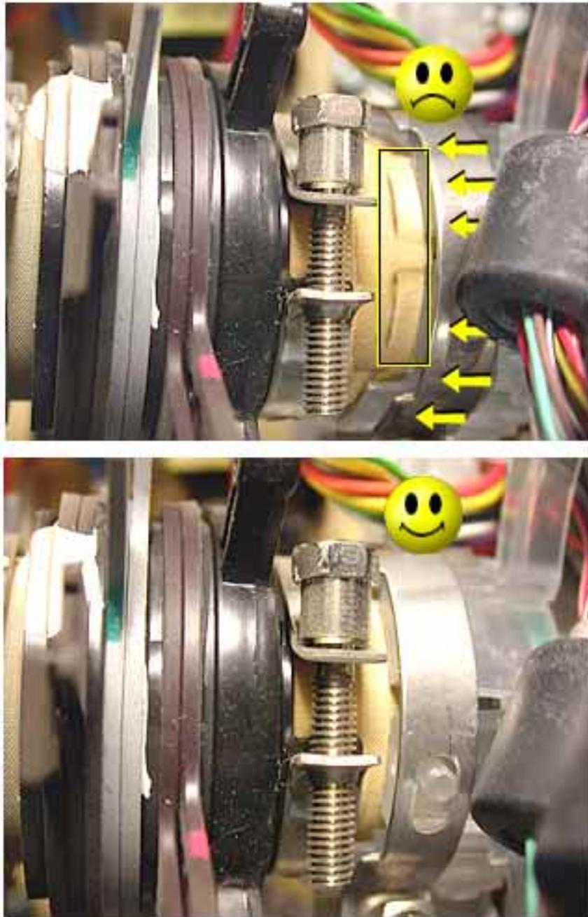
**Figure 2 Video Board Improperly and Properly Seated**
