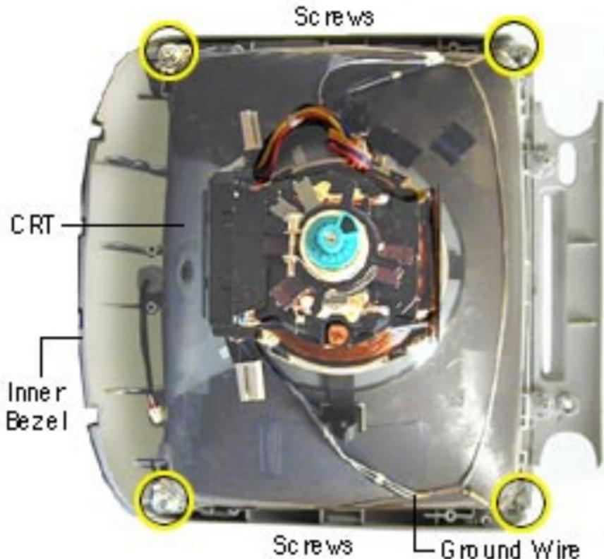
1. Remove the four CRT screws.
