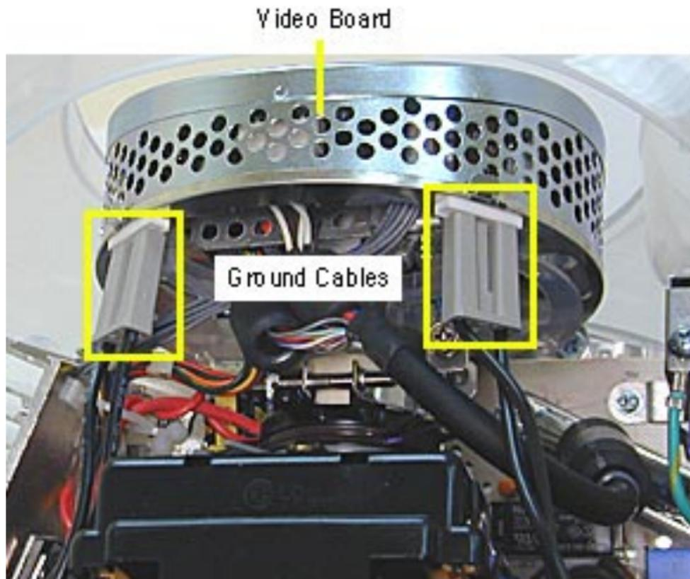
2. With the power off, remove the left ground cable from the video board.
