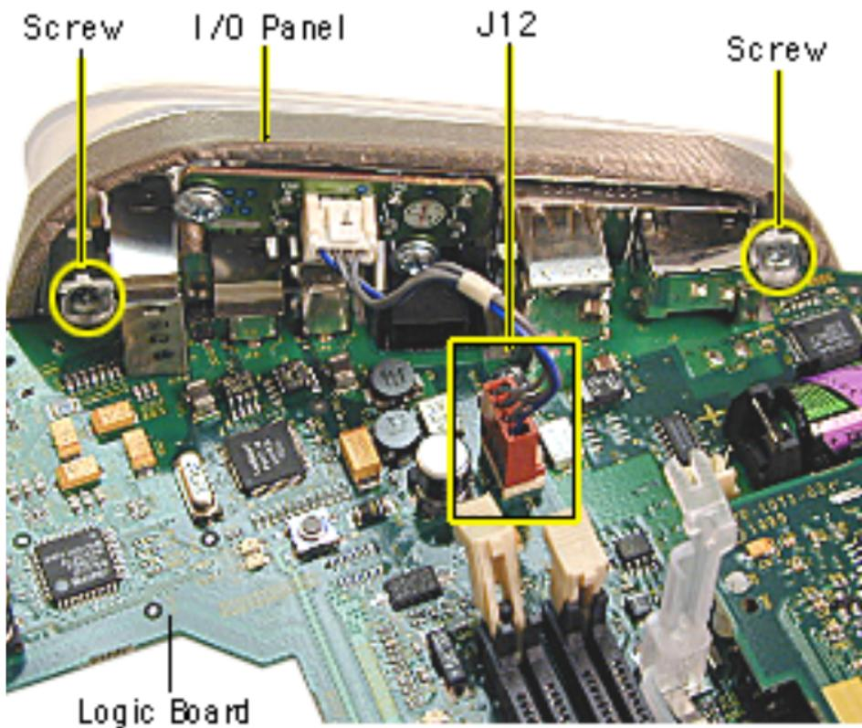
1. With the logic board facing right side up, disconnect the cable at J12.
