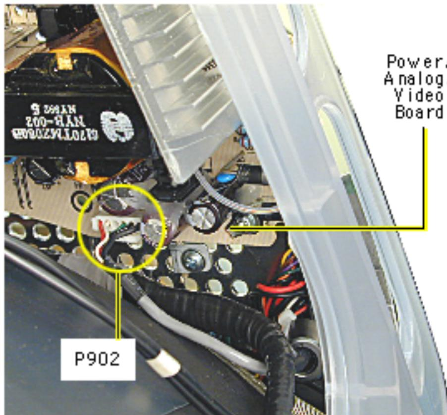
10. At the very bottom of the power/analog/video board, near the bottom of the CRT, disconnect P902, which is part of the audio/headphone/LED/speaker cable assembly.
