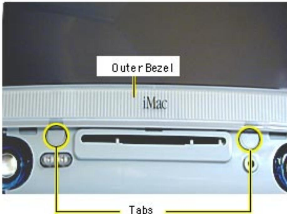
1. With a jeweler's screwdriver, carefully remove the two tabs on the front outer bezel. Refer to the next graphic for a close-up of the tab removal.
