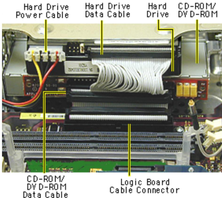
**Note:** Remove SDRAM to make cable removal easier.
