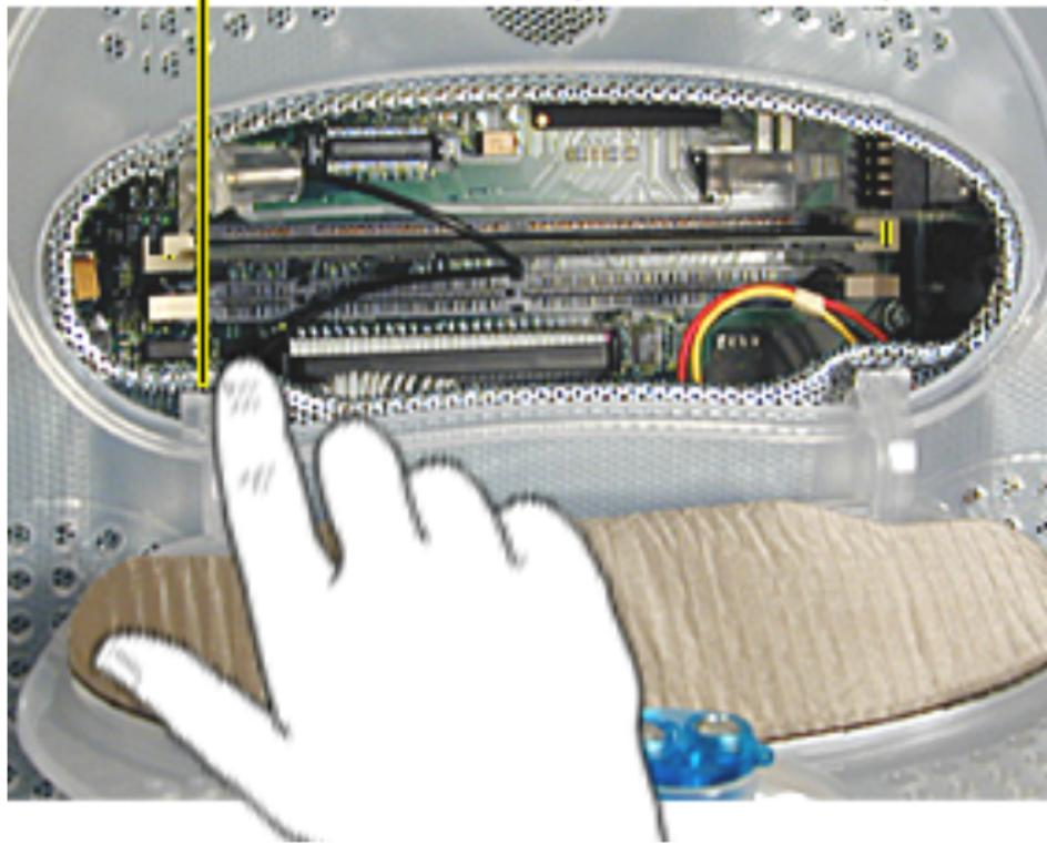
3. Touch the metal EMI shield inside the recessed latch area before touching any components on the main logic board.
