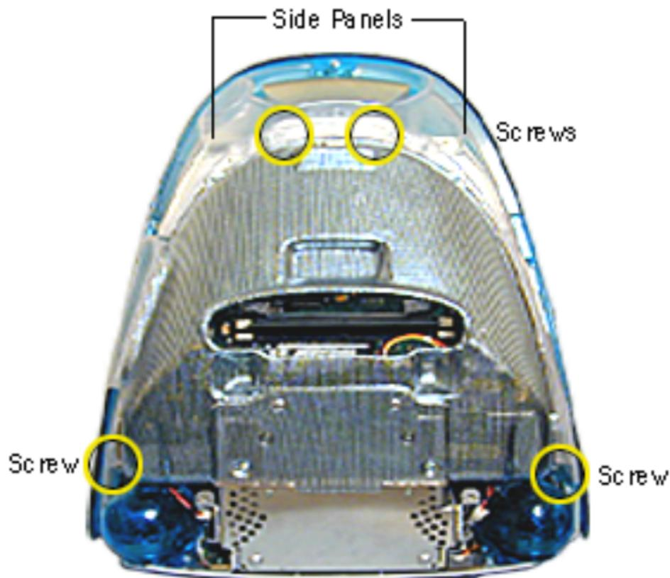
3. On the rear of the side panels, remove four screws. These screws connect the side panels to the divider panel (the metal chassis).
