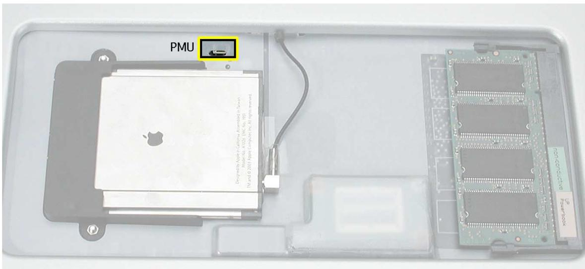
4. WAIT ten seconds before connecting the power cord and powering the computer on. If the computer powers on, go to the next step. If the computer does not power on, there is something else wrong with the computer, refer to the symptom/cure, “No Power” in this chapter.
