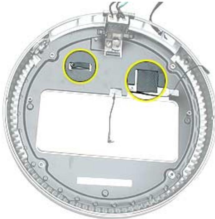
**Warning:** Whenever the logic board is separated from the bottom housing, you must install new thermal pads to two surfaces on the bottom housing. Failure to apply these pads whenever the logic board is separated from the bottom housing could cause these parts to overheat and could damage internal components.
