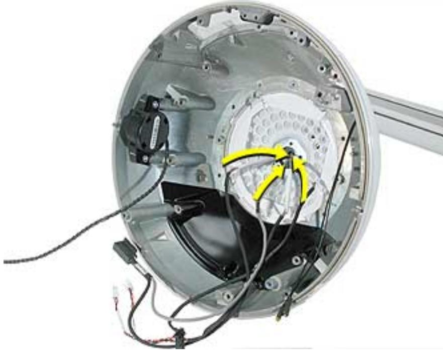
3. Pull the outer shell (with Faraday attached) away from the neck. **Note:** There is no need to remove the outer shell from the Faraday unless you are replacing the antenna or the outer shell. If you are removing the shell from the Faraday cage, go on to the next step.
