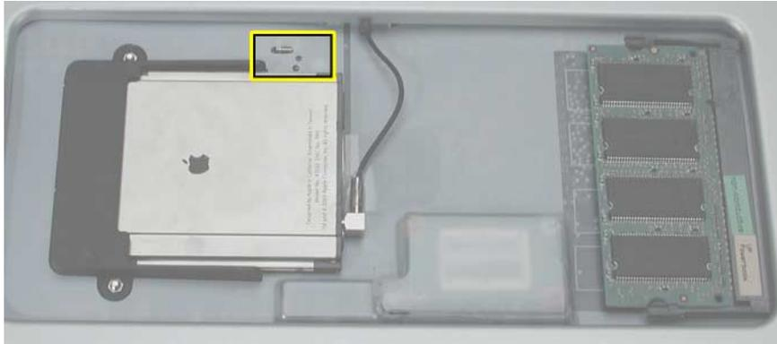
These test points provide an easy troubleshooting tool for common problems. To use each test point, put the positive probe of your voltmeter on the test point, and the negative probe on the ground pad.
