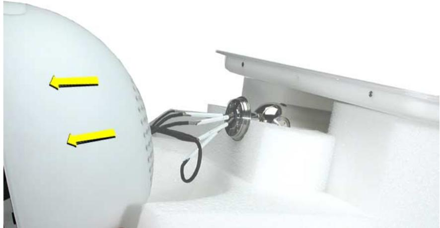
4. **Note:** Perform this step only if you are replacing the antenna or the outer shell. Remove one screw in the base of the Faraday cage to separate the shell from the Faraday cage.
