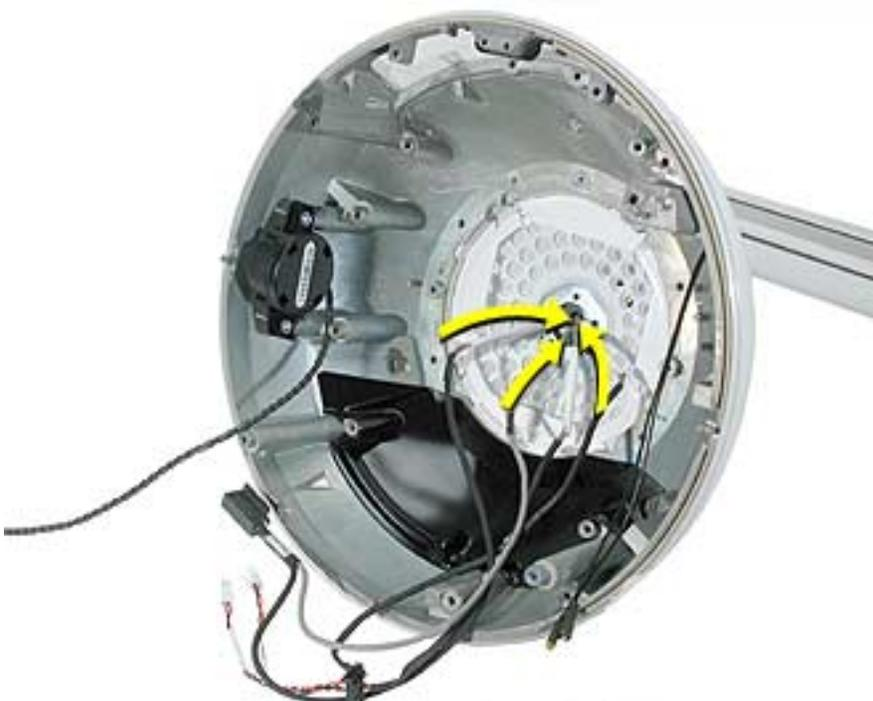
3. Next, carefully separate the outer plastic housing from the neck.
