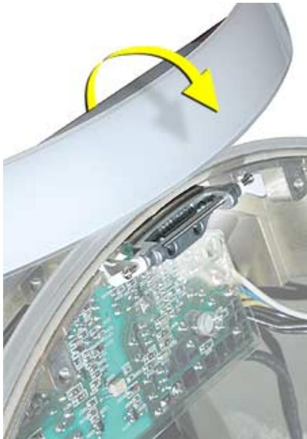
6. Slide the door and hinge off the chassis.
