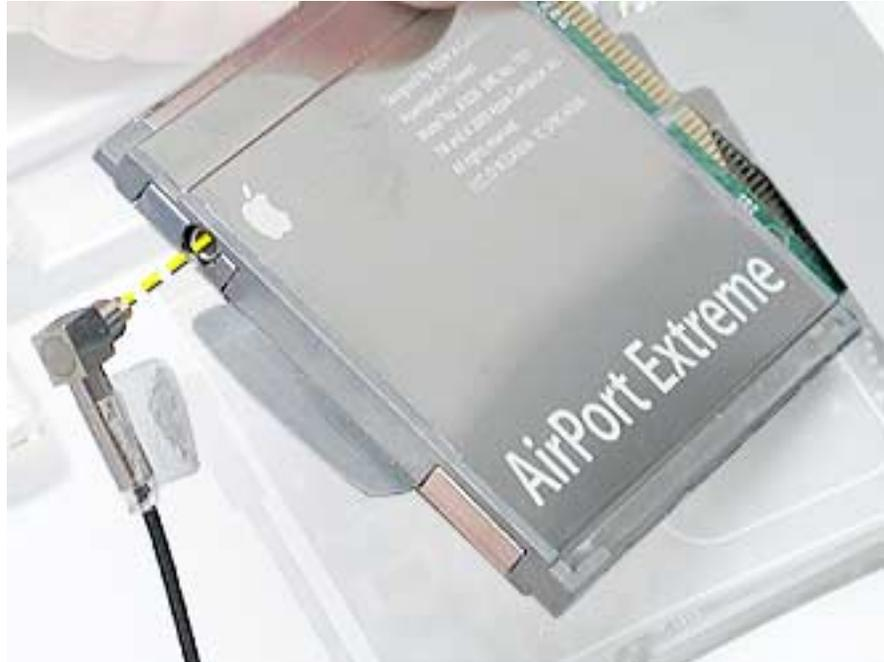
2. Insert the card into the AirPort Extreme slot. Push the card until you hear it click into the slot.
