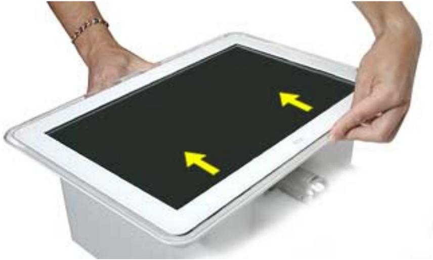
3. **Caution:** The power on LED cable (labelled A below) is fragile. When disconnecting display cables, be sure to raise the TOP SIDE of the display only. Carefully raise the TOP SIDE of the display and disconnect the inverter cable (B) and remove the TMDS cables (C) from the metal cable clip. **Note:** Enlarge the page to view the graphic at a larger size.
