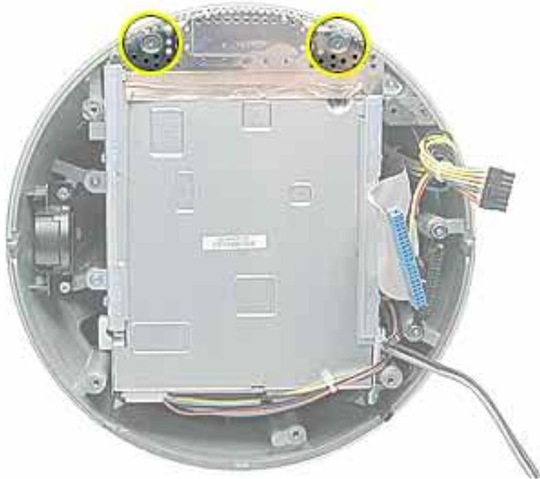
3. Remove four screws attaching the drive carrier to the metal chassis (also known as the Faraday cage).
