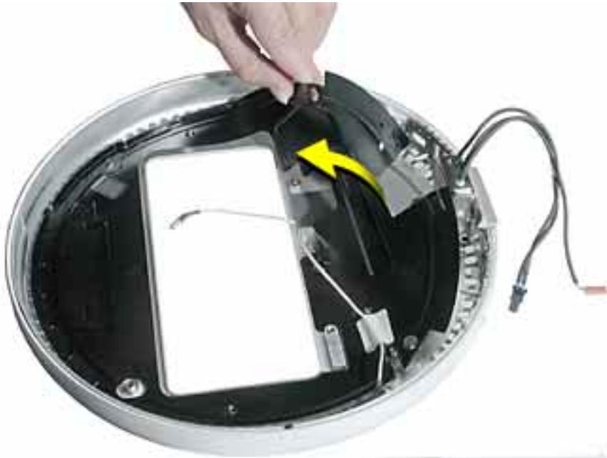
2. Remove two screws and lift the AC line filter from the bottom housing. **Note:** The AC line port cover plug may fall out of the bottom housing when you remove the AC line filter. Place the plug back into the bottom housing before reinstalling the AC line filter.
