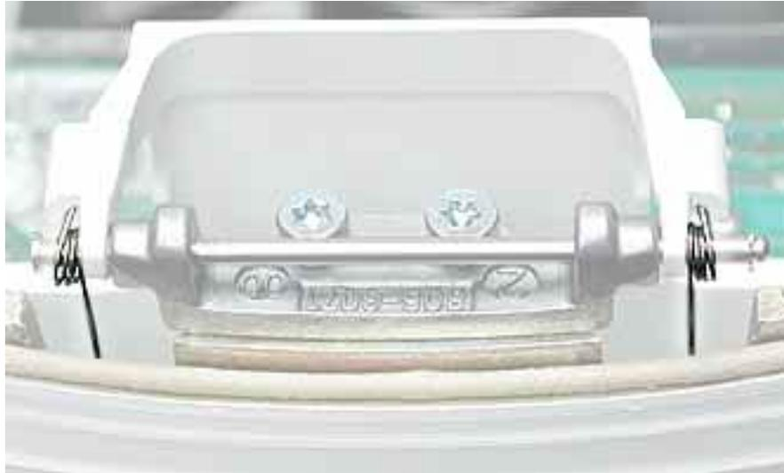
4. Remove the door hinge screws.
