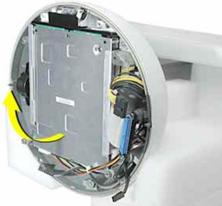
6. Peel the white wrapper up to access the screws connecting the hard drive to the carrier. Remove four screws and the hard drive.
