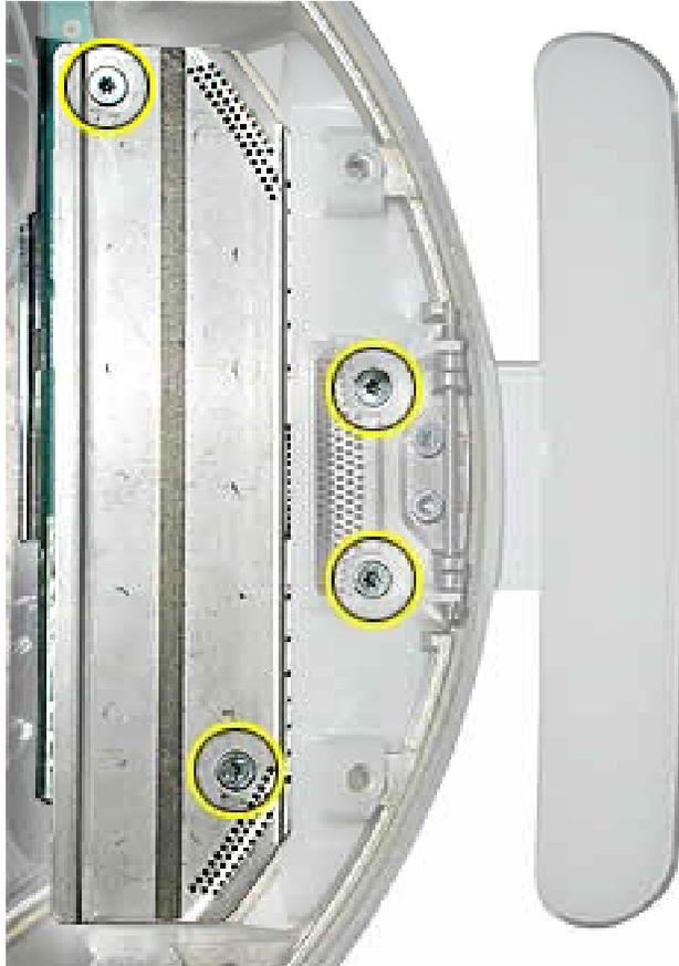
3. Remove the power supply and metal shield from the chassis (Faraday cage).
