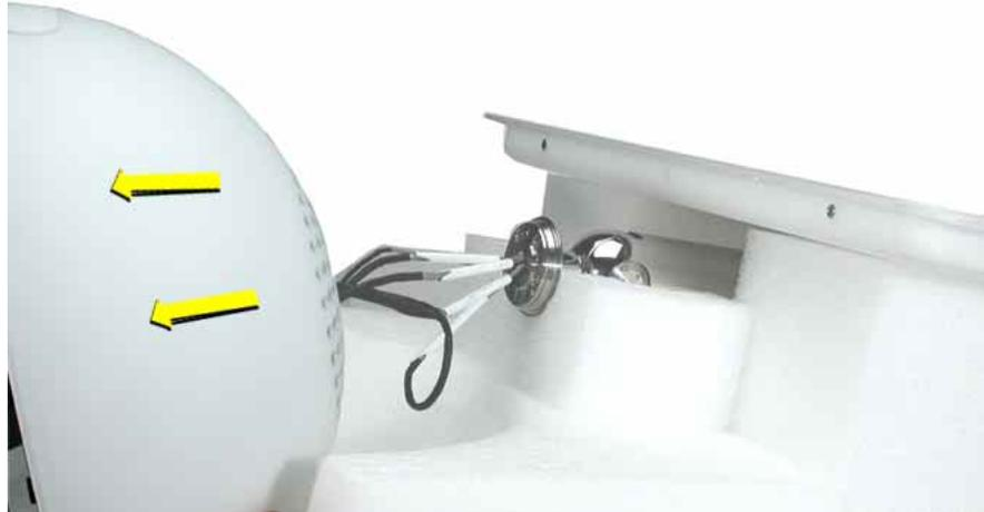
4. **Note:** : Perform this step only if you are replacing the antenna or the outer shell. Remove the three screws in the base of the Faraday cage to separate the shell from the Faraday cage.
