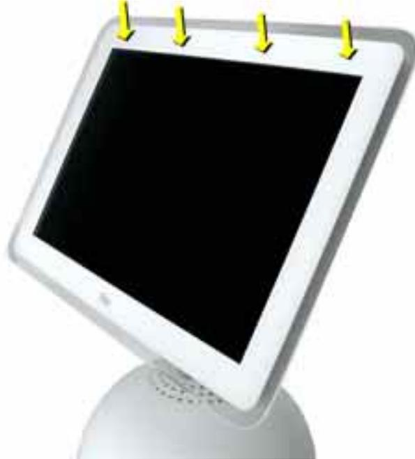
2. Holding the display, turn it over and lay the display face down on a soft cloth. Push the rear housing in the direction of the arrow. This will mate the housing and display tabs.
