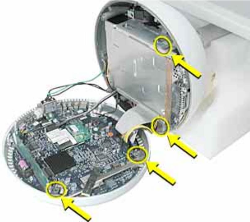
2. Squeeze a drop of thermal paste onto the thermal pipe locations circled below.
