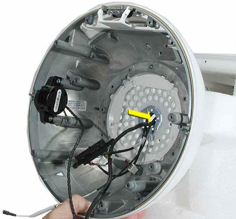
3. Next, carefully separate the outer plastic housing (with Faraday attached) from the neck.
