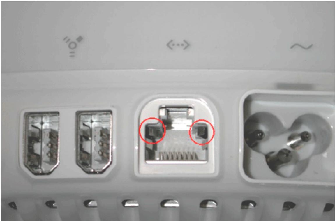
3. When inserting the Ethernet cable, try holding the cable at a slight angle and wiggle the connector to get past the metal tabs.
