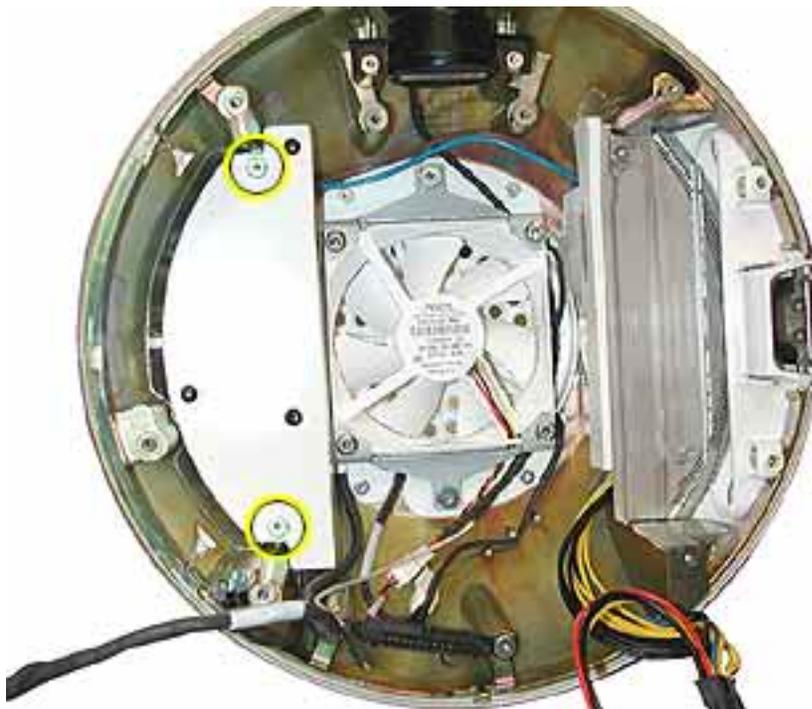
2. Open the optical drive door as shown. Support the metal plate and power supply as you remove the four screws.
