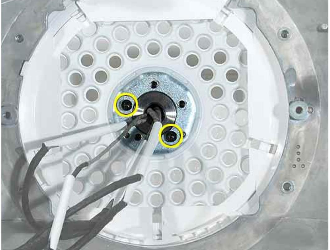
3. Pull the outer shell (with Faraday attached) away from the neck. **Note:** There is no need to remove the outer shell from the Faraday unless you are replacing the antenna or the outer shell. If you are removing the shell from the Faraday cage, go on to the next step.
