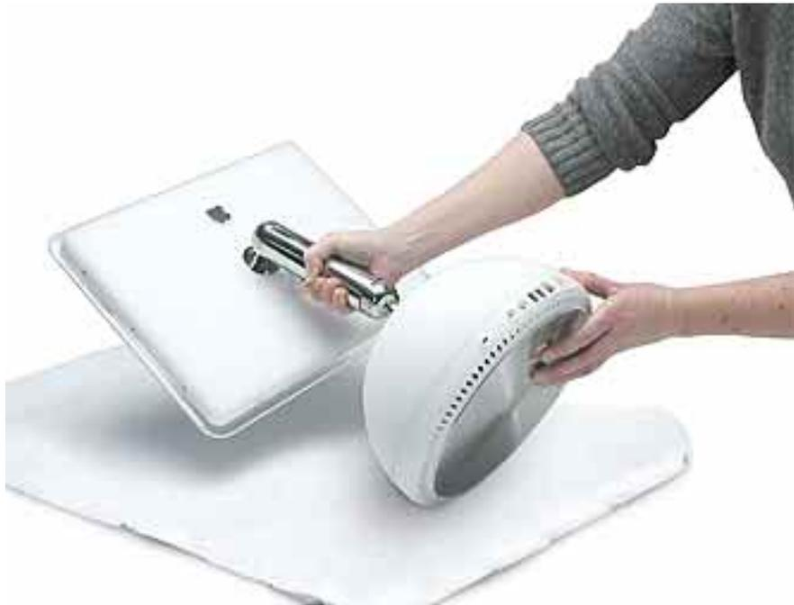
4. Loosen the four captive screws at the base of the computer and gently remove the access panel.
