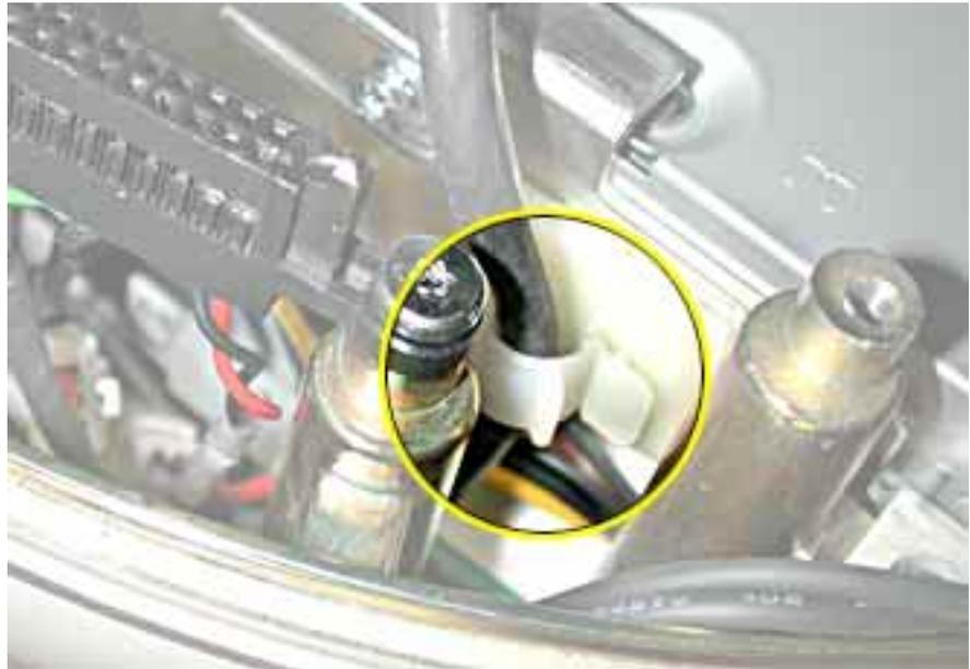
5. Grasp the carrier on both sides. Lift and pull the carrier in the direction of the arrow. Once the carrier is out, flip the carrier to the right to disconnect the power cables.
