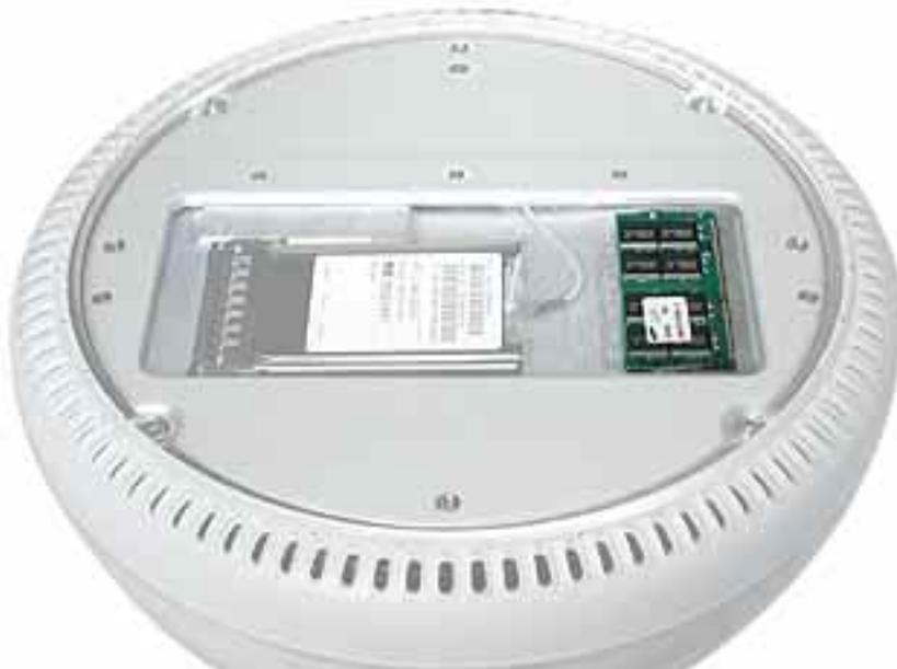
The iMac has two RAM expansion slots. The factory-installed RAM slot accepts a standard PC133 168-pin DIMM (up to 512 MB in capacity) and is accessible only by an Apple Authorized Service Provider. The user-accessible slot (shown above) accepts a standard PC133 144-pin SO-DIMM and is normally used for added RAM. Only the SO-DIMM slot is accessible by the user. A SO-DIMM for the iMac computer can contain either 64, 128, 256, or 512 MB of memory.
