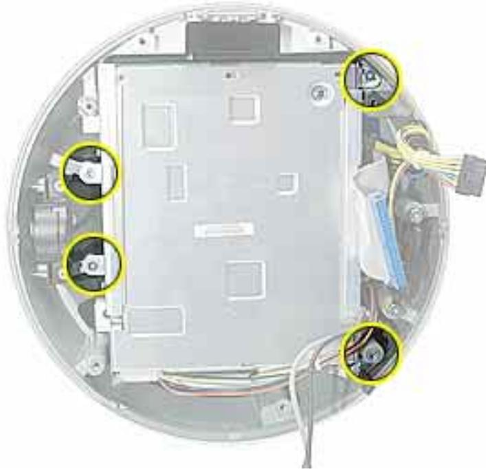
4. Remove the Airport antenna and the video cable from the plastic clip on the side of the hard drive.
