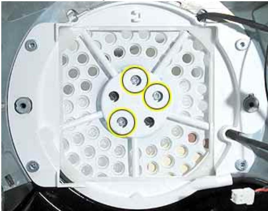
3. Lift the neck cap off the cables. The two remaining black screws hold the neck to the base. Note the orientation for neck reassembly.
