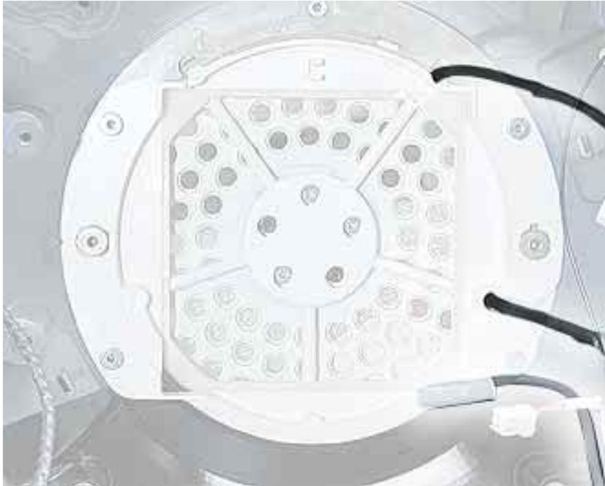
2. There are five screws on the neck cap; however, only the three silver screws need to be removed. The remaining two black screws keep the neck attached to the base.
