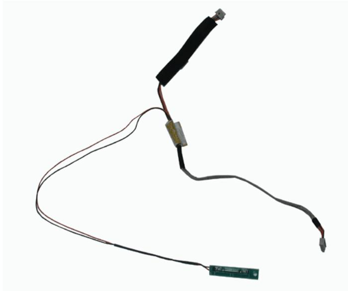
7. Install the replacement reed switch board and cable assembly, and reassemble and test the computer.
