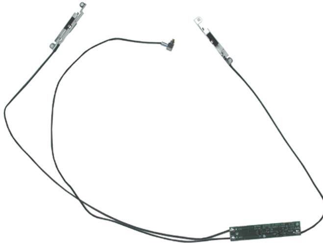
13. Install the replacement antenna board, and reassemble and test the computer.
