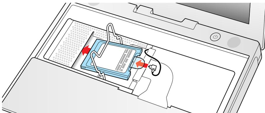
Use the wire holder to secure the AirPort Card in place by inserting its prongs into the slots in the RAM shield.
