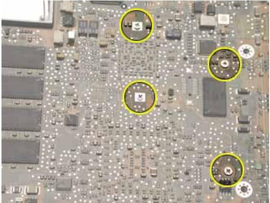
5. Turn over the computer frame, and remove the remaining screw at the heat spreader plate.
