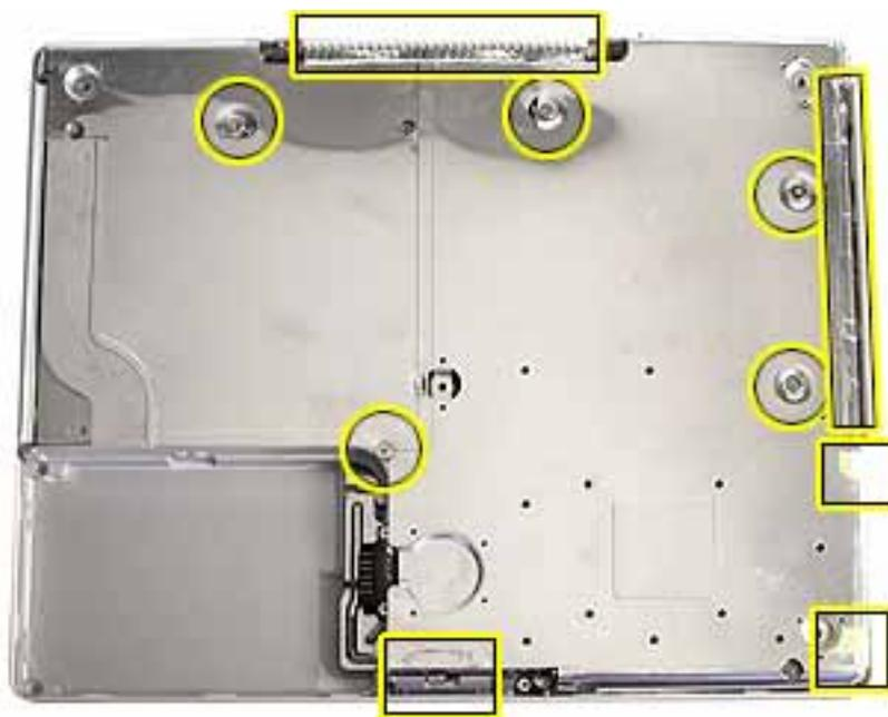
4. Peel up the tape at the computer latch. If the tape tears, replace it with new aluminum tape.
