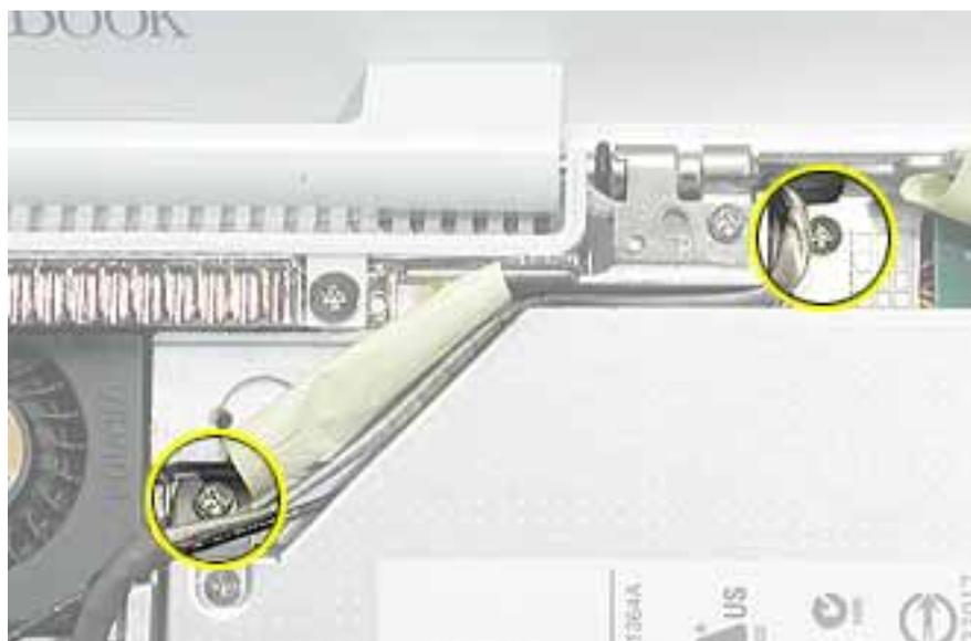
3. Lift up the ribbon cable, and remove the screw at the battery bay.
