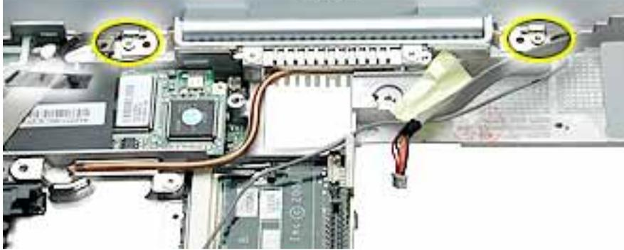
6. **Warning: When lifting the display, be careful not to strain the cables.**
