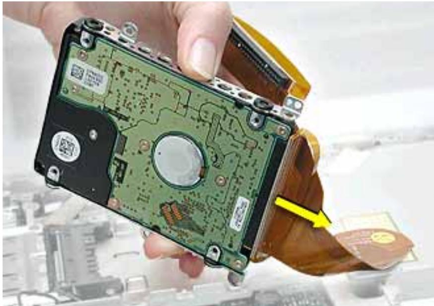
6. Holding the drive by the corners as shown, pull off the side rails (with grommets attached).
