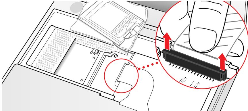
14. Install the replacement keyboard, RAM shield, and AirPort Card (if used).
