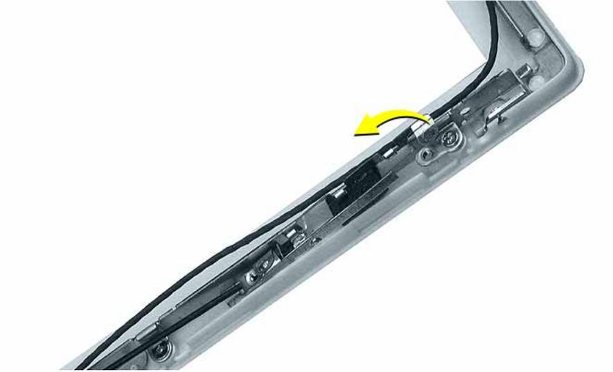
7. At the bottom of the bezel, remove the tape from the inverter board and note the routing of the two soldered cables on the left side of the antenna board.
