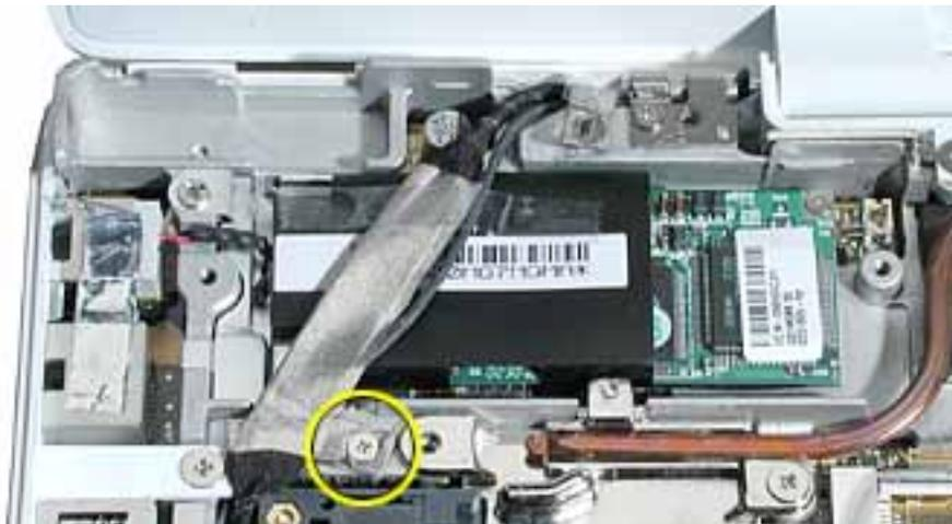
2. **Important:** Do not strain or remove the LVDS cable.
