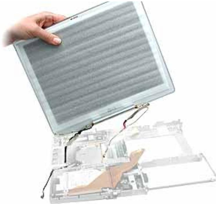
7. **Warning: While supporting the display, do not tug on the remaining cables. Make sure the cable insulation is not torn or damaged.**
