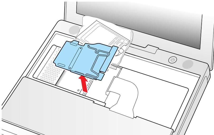
11. Locate the keyboard cable connector.
