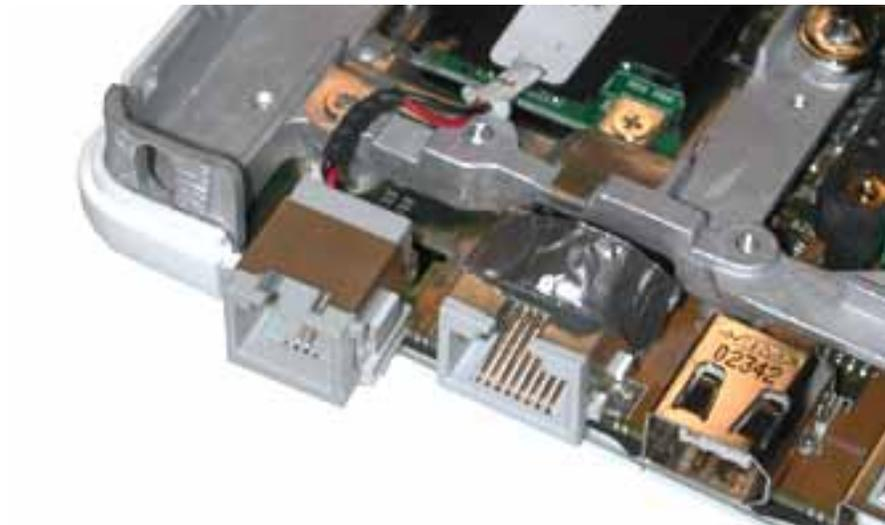
5. Install the replacement RJ11 modem cable, and reassemble and test the computer.
