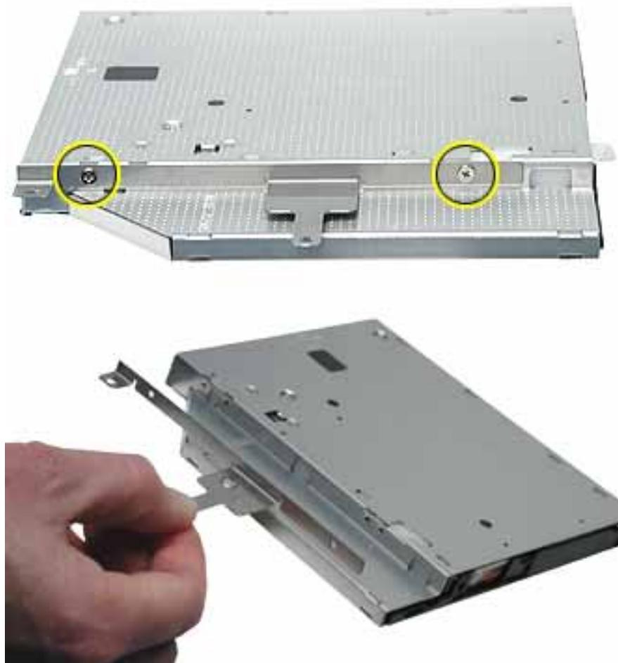
9. Install the replacement optical drive, and reassemble and test the computer.
