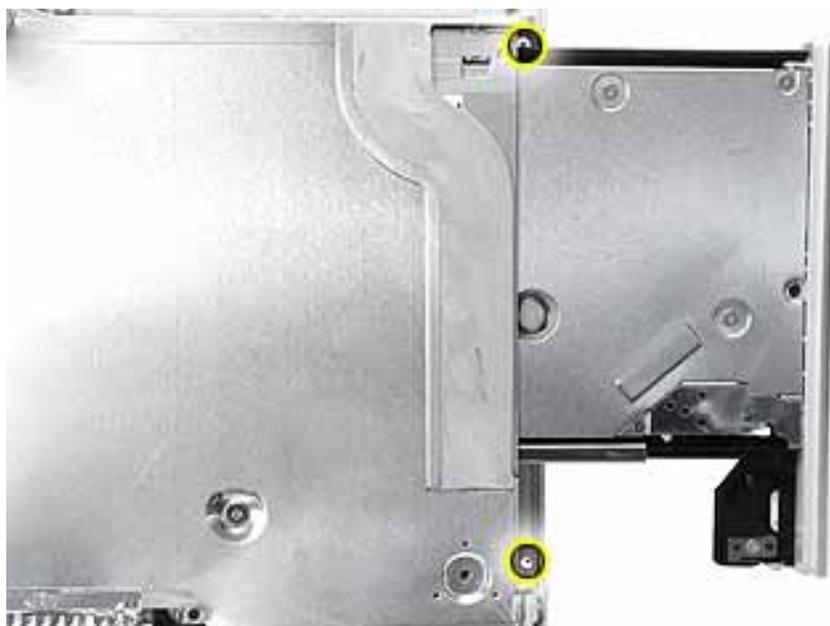
9. **Warning:** When performing this step, make sure the speaker cable and power switch cable are not strained.
