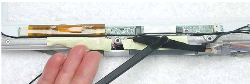
3. **Warning:** When lifting the inverter board, be careful not to pinch the cables that are routed above the board.
