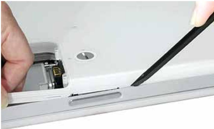
10. **Warning:** To avoid damaging the sleep light and other delicate components, do not insert the black stick too far into the computer as you free the bottom case from the computer. Use just the tip of the black stick to pry up the bottom case.
