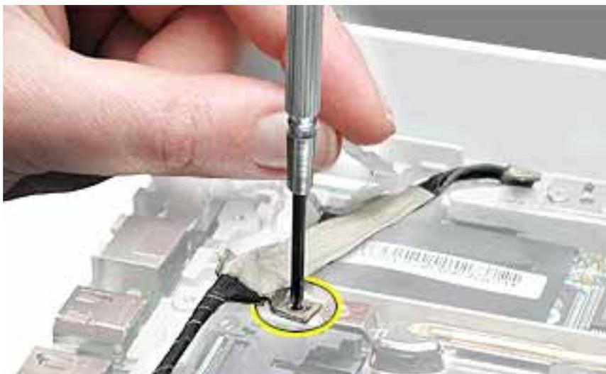
2. **Important:** Do not strain or remove the LVDS cable.
