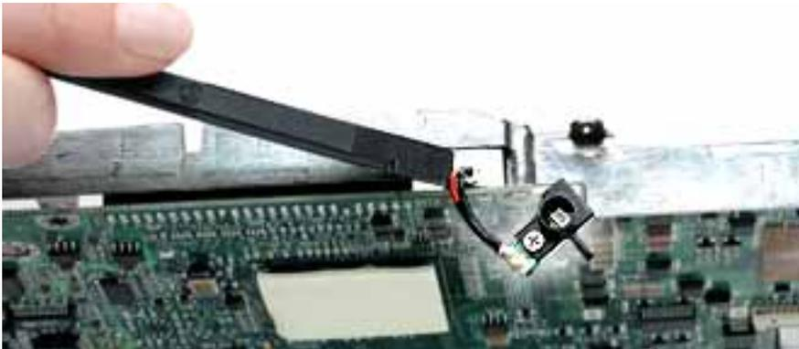
3. Remove the screw from the reset button board, and disconnect the connector from the logic board. (If tape covers the screw, remove and reserve the tape for the replacement logic board.)
