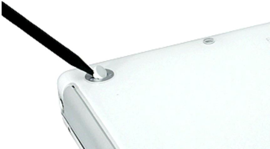
4. Remove the three identical Phillips screws from the metal sockets.
