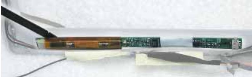
**Replacement Note:** The inverter board is held to the bezel assembly with double-sided tape on each end of the board. Use new double-sided tape when installing the replacement inverter board.
