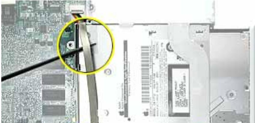
2. Remove the single screw from the DC board.
