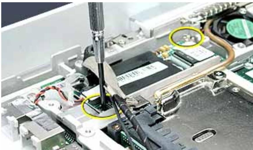
3. Tilt up the end of the modem to disconnect it from the logic board.
