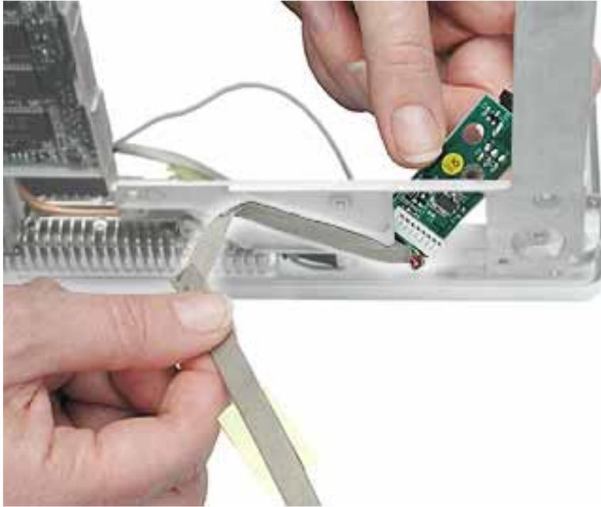
4. Install the replacement DC board, and reassemble and test the computer.
