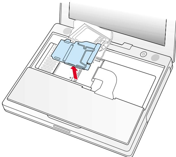
6. Locate the installed memory card and brackets that secure the card on both sides. **(Figure 9)**
