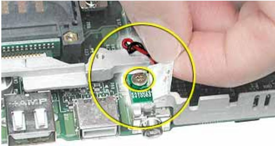
4. Remove the two screws holding the vent cover to the heat spreader.
