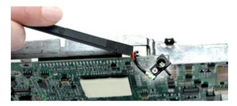
3. Remove the screw from the reset button board, and disconnect the connector from the logic board. (If tape covers the screw, remove and reserve the tape for the replacement logic board.)
