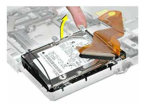
5. Warning: Handle the hard drive at the sides only. Do not touch or press anywhere else on the drive.
