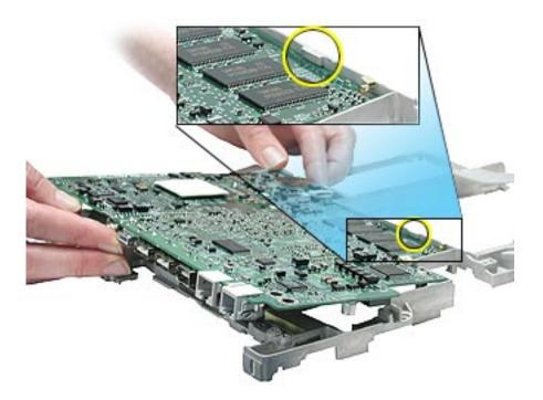
9. Install the replacement logic board, and reassemble and test the computer.
