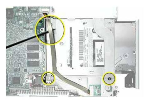
4. Tilt back the computer, and on the other side of the optical drive, loosen the tape holding the backlight cable to the optical drive. Reserve the tape for installation of the replacement drive. Do not disconnect the backlight cable.
