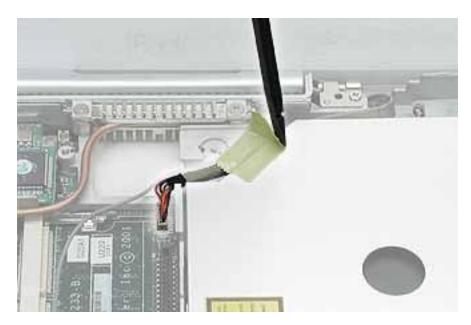
4. Remove the screw securing the flat section of the LVDS cable.
