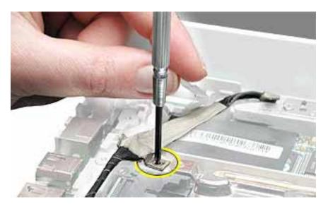
2. **Important:** Do not strain or remove the LVDS cable.
