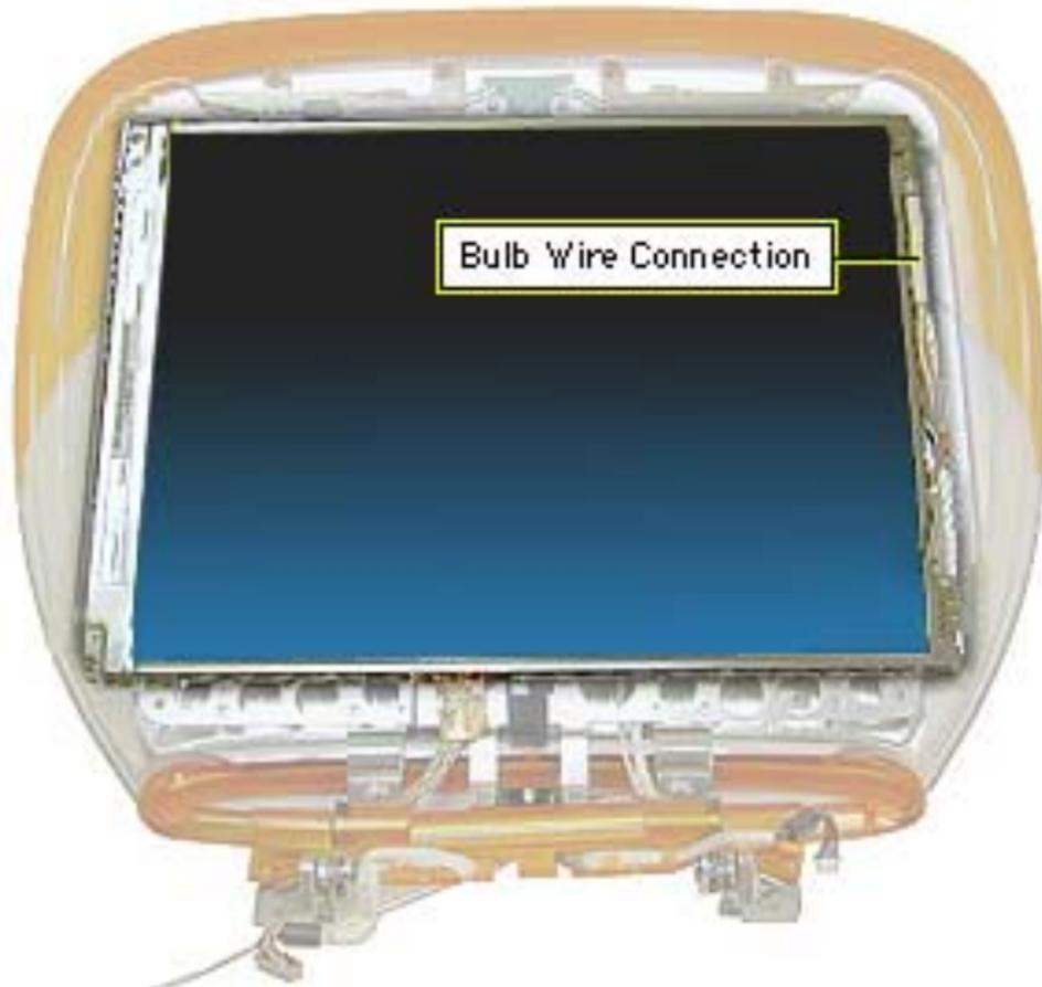
2. Remove any tape from the bulb wire connection sleeve.
