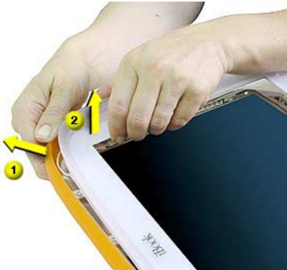
7. Work your hands around each side, separating the bezel from the display housing. At the top corners, pull the plastic of the display housing out while pulling up on the bezel.
