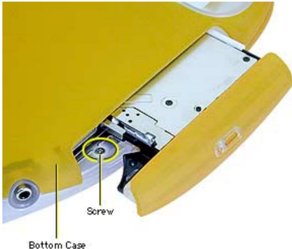
4. Press the manual disc eject button with the tip of a jeweler's screwdriver or paper clip to eject the optical drive tray.
