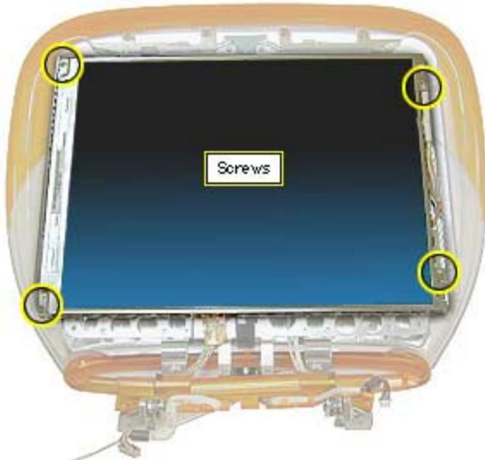
9. Remove the four Phillips screws on the corners of the display.
