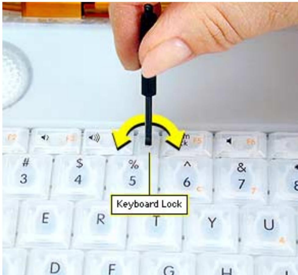
3. If the keyboard does not pop up, it may be locked. Locate the keyboard lock screw (left of the num lock key). Turn the lock a half turn in either direction until the tab slides out from under the top case.
