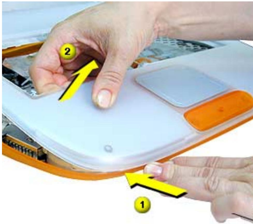
11. At the front left corner, push in on the bottom front while pulling up on the top case.
