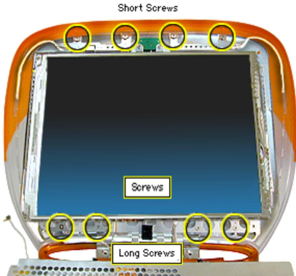
6. Loosen the four short Phillips screws on the top of the display mounting frame.
