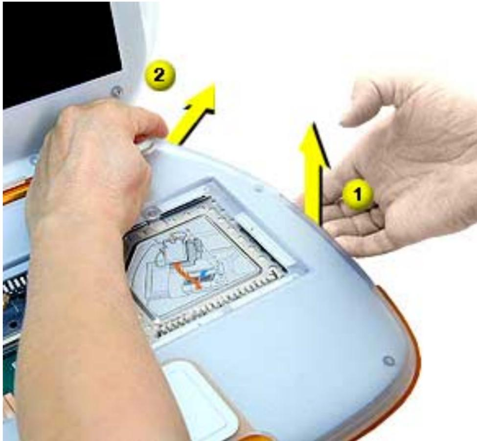
9. With the optical drive tray open, push up on the underside of the top case while pushing out on the clear lip that holds the back right edge of the top case until the case pops open.
