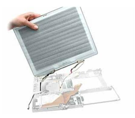
7. Warning: While supporting the display, do not tug on the remaining cables. Make sure the cable insulation is not torn or damaged.
