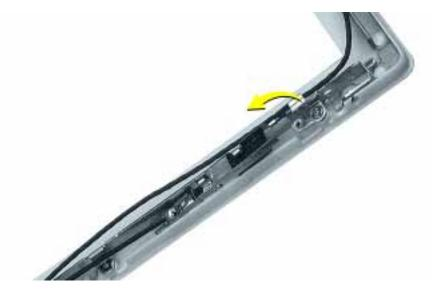
7. At the bottom of the bezel, remove the tape from the inverter board and note the routing of the two soldered cables on the left side of the antenna board.
