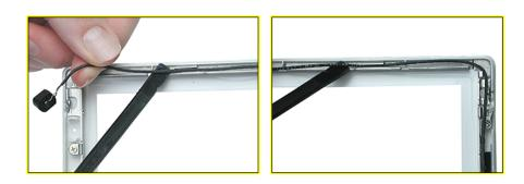
4. Free the microphone cable from the right corner of the bezel and from underneath the tape at the antenna board.
