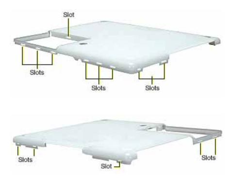
8. In the battery compartment, lift up the corner of the bottom case, and use a black stick or jeweler's flat-blade screwdriver to gently pry up the slot from the inner tabs on the frame.
