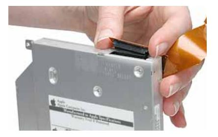
9. Remove the two screws that hold the mounting bracket to the optical drive.
