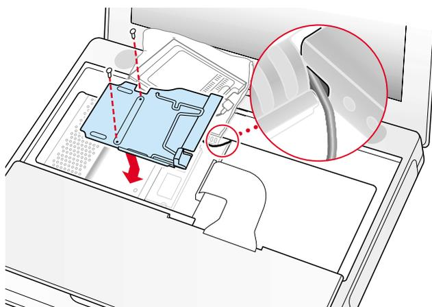
7. If you do not have an AirPort Card, flip down the wire holder over the AirPort Card antenna cable and secure it by inserting the prongs of the holder into the slots in the RAM shield (**Figure 13**).
