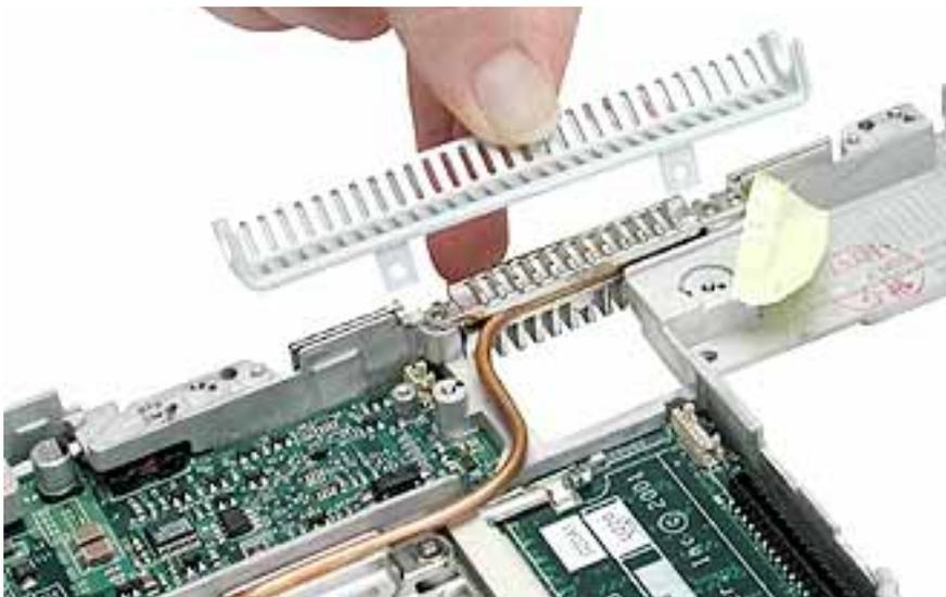
4. Turn over the computer frame and remove the two Phillips screws that secure the logic board to the heat spreader plate:
