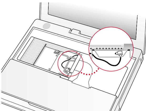
8. If you have an AirPort Card, gently slide it (with the AirPort ID number and bar code facing up) under the wire bracket and securely into the AirPort Card slot.
