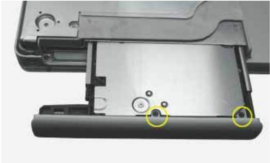
2. Press on the wide tab, and pull the door away from the drive.
