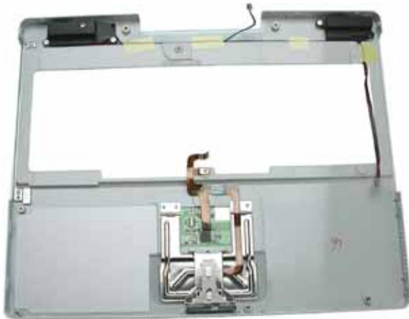
15. Install the replacement top case, and reassemble and test the computer.
