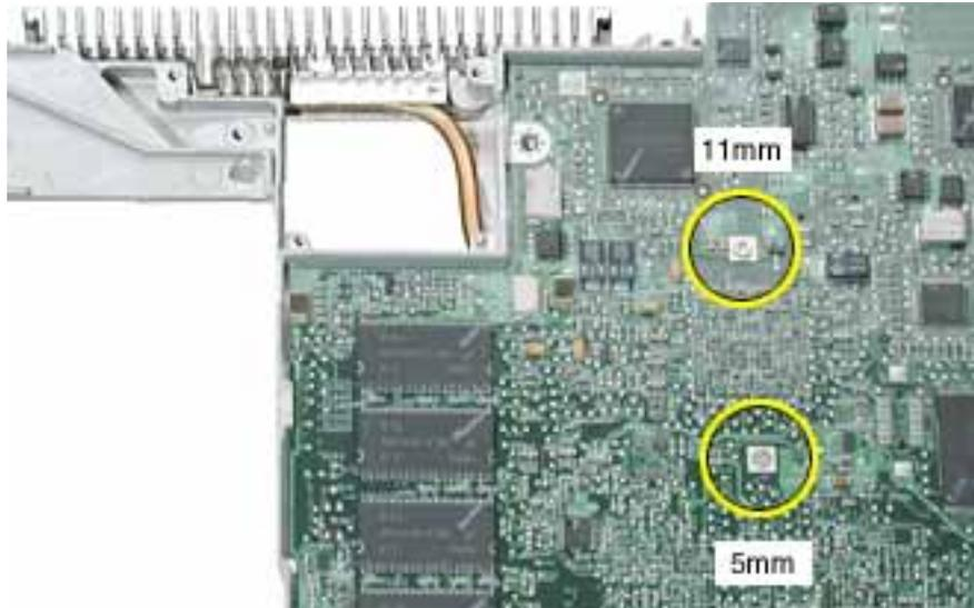
5. Turn over the computer frame, and remove the remaining screw at the heat spreader plate.
