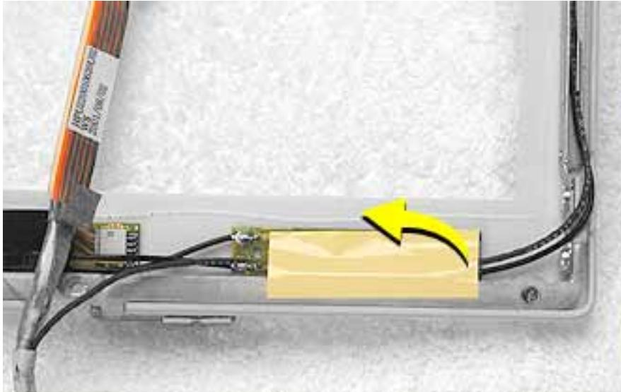
2. Note the placement of the antenna board and the routing of the cables that are soldered to and run along the bottom of the antenna board.
