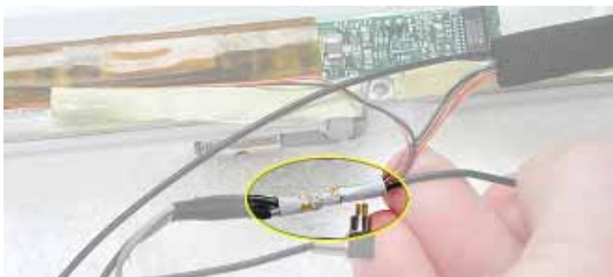
11. Use a black stick to lift out the cables from the channels.
