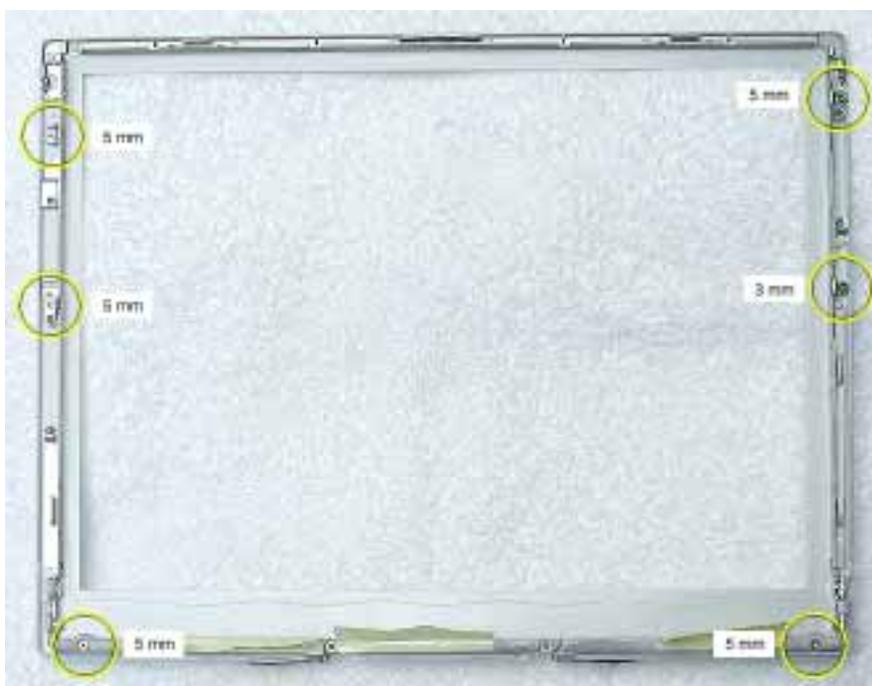
5. Lift the 3-sided bezel brace with clutch assembly off of the bezel.
