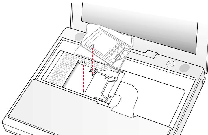
5. Lift the RAM shield out of the computer. Carefully pulling up on the wire holder may help to remove the shield (**Figure 8**).
