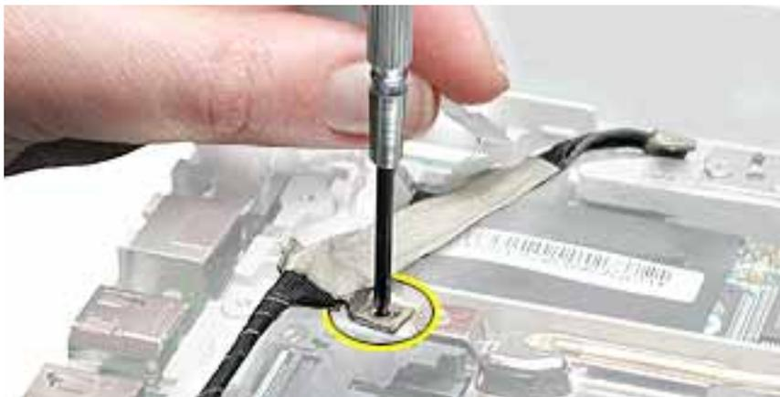
2. **Important:** Do not strain or remove the LVDS cable.
