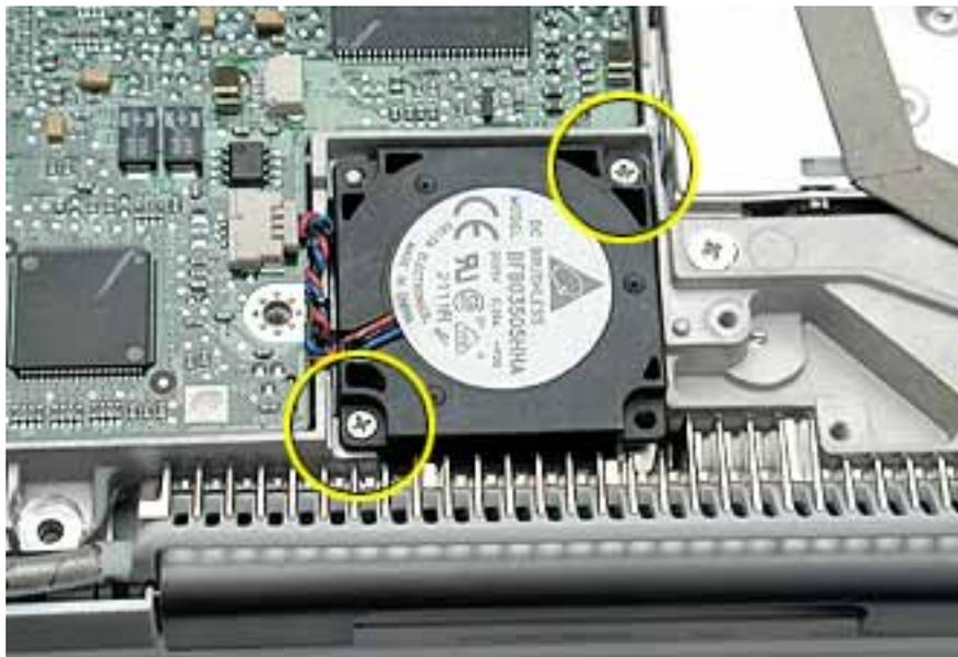
2. Lift the fan from the computer, and use a black stick to disconnect the connector from the logic board.
