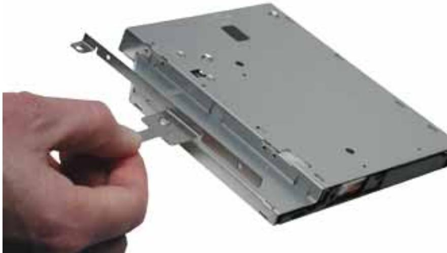
**Note:** The mounting bracket has a different shape on the 900 MHz model:
