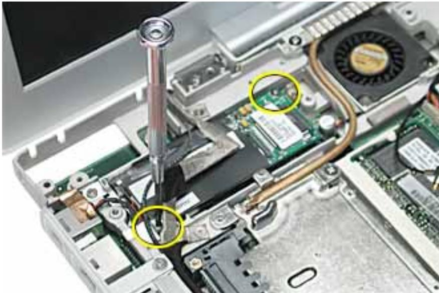
3. Without straining the LVDS cable, peel off the clear tape.
