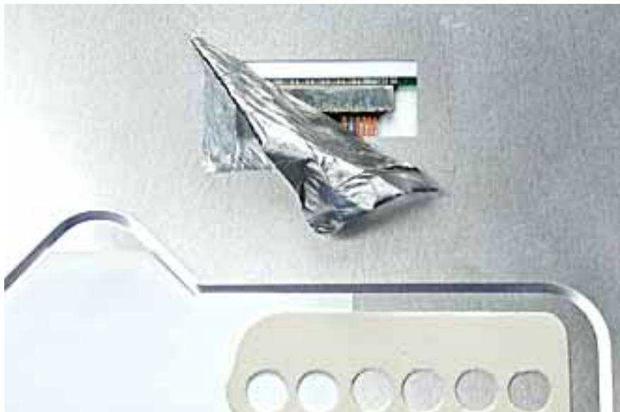
8. Peel up the tape if it covers the two screws at the clutch. Remove the two 11-mm long Phillips screws.
