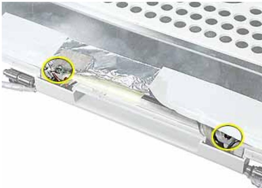
10. Loosen the remaining tape that secures the shield to the assembly. Remove the shield.
