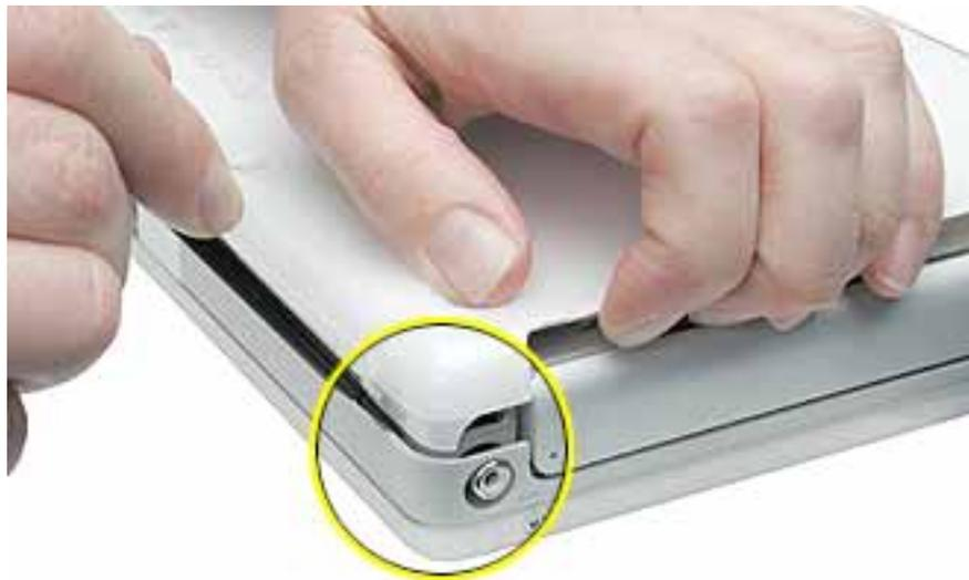
12. The bottom case fits snugly. Use moderate force to remove the remaining tabs from the slots.
