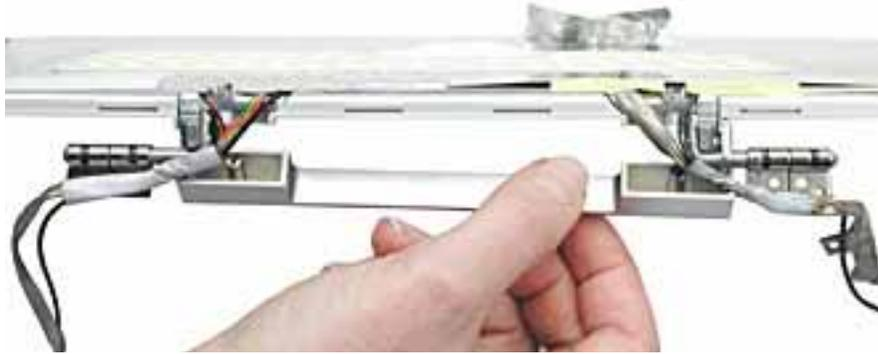
**Replacement Note:** When installing the replacement clutch cover, hold the cables and clutch cap in place as you slide the clutch cover over them.
