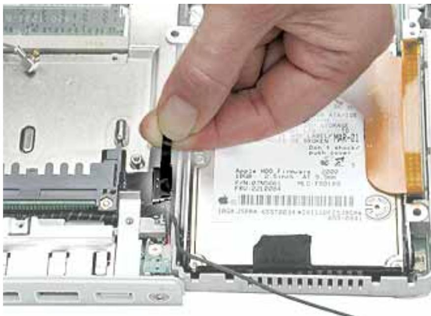
3. Remove the two screws securing the flat section of the LVDS cable.
