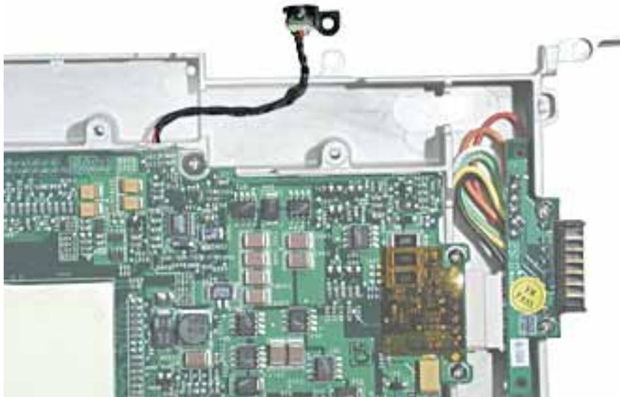
3. Turn over the computer frame and remove the two Phillips screws that secure the logic board to the heat spreader plate:
