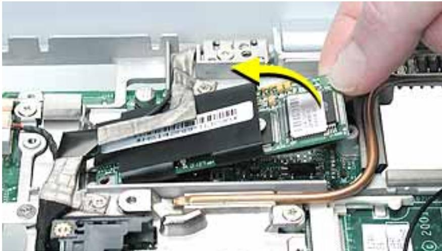
5. **Important:** Do not strain or remove the LVDS cable.
