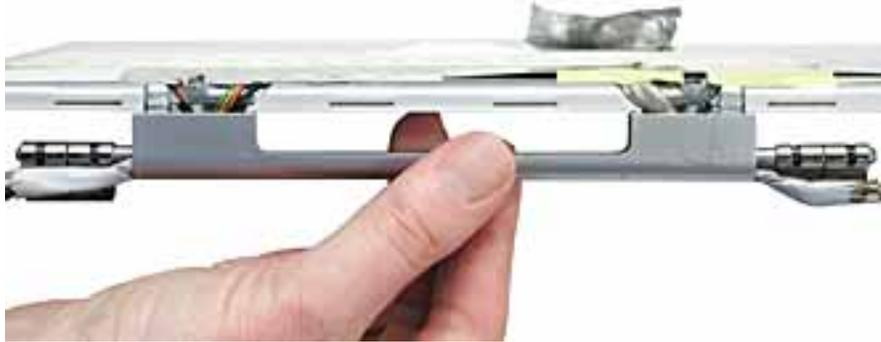
**Note:** The clutch caps are mirror images of each other. There is a right clutch cap and a left clutch cap. Note the positioning of the clutch caps on the display clutch cover. The image below shows the left clutch cap installed.
