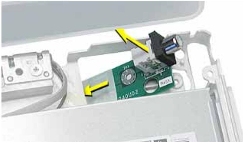
3. Disconnect the flat power cable from the connector on the logic board.
