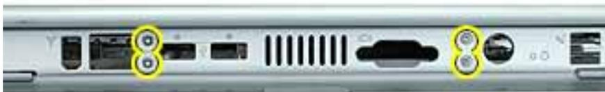
4. Turn over the computer, and remove the four identical black screws.
