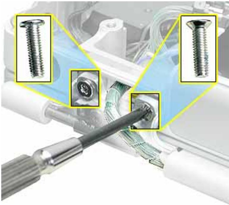
5. At the right clutch, note the routing of the inverter cable (the black and pink wires). Without straining the inverter cable, gently move it aside so you can access the two silver-colored screws.
