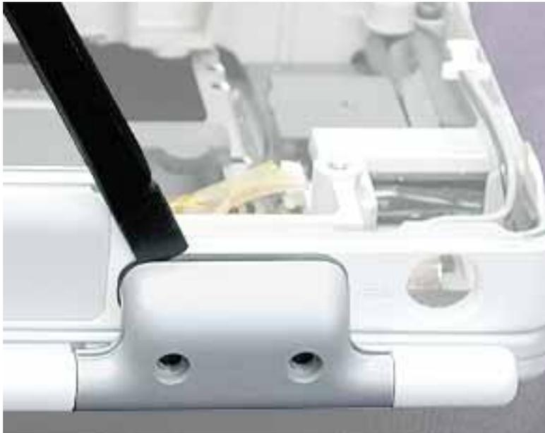
**Important:** When reassembling the computer, note that each clutch cover has a molded number centered inside it. When the computer is positioned upside down, as shown below, the left clutch cover is labeled "1"; the right clutch cover is labeled "2". Make sure the left and right clutch covers are placed correctly on the clutches.
