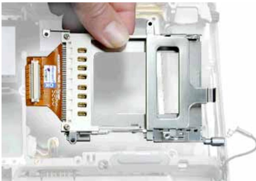
3. Install the replacement PC card cage, and reassemble and test the computer.
