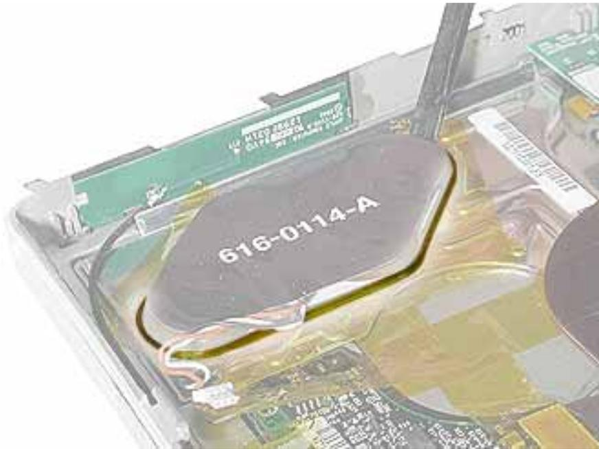
7. Install the replacement backup battery, and reassemble and test the computer.
