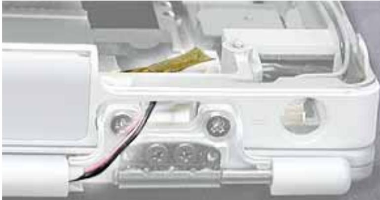
8. Disconnect the inverter cable, and lift the inner clutch mount out of the way.
