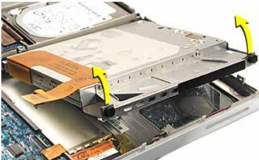
**Note:** There are four rubber stoppers (two on each side) on the drive that fit over metal posts at the corners of the drive. Remove any that may have fallen off inside the computer.
