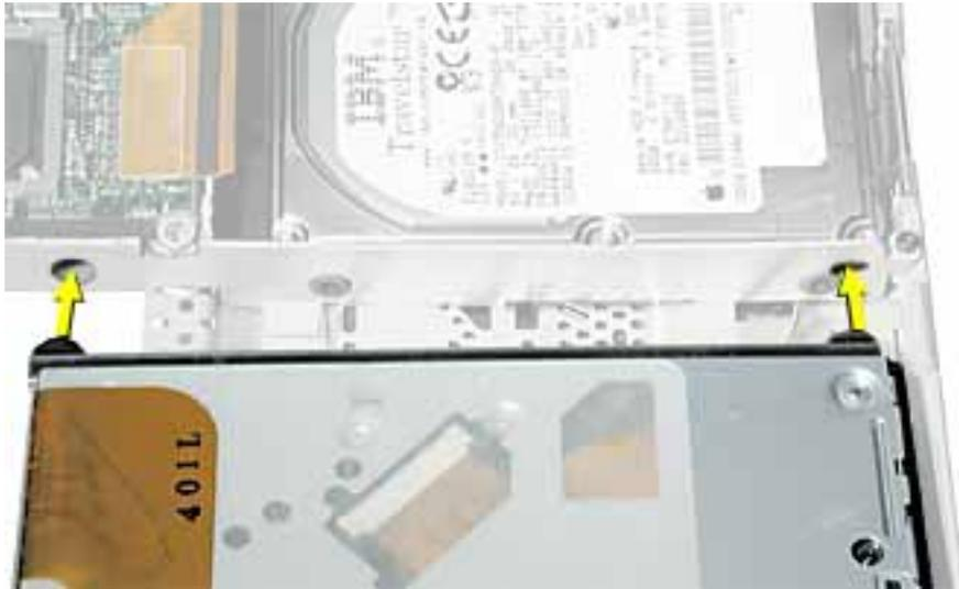
**Important:** When the rubber stoppers are inserted, push down on all four corners of the drive to verify that the drive is level and secure.
