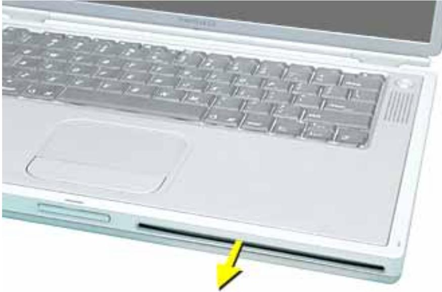
**Important:** Check the operation of the optical drive. If the drive is installed incorrectly, the optical drive mechanism might not spin correctly and will result in mechanical noise when playing a disc.
