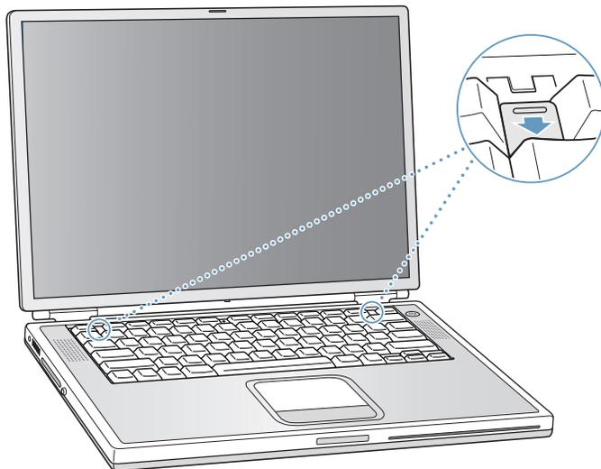
10. Flip the keyboard over and lay it on the palm rests and trackpad. (**Figure 4**)
