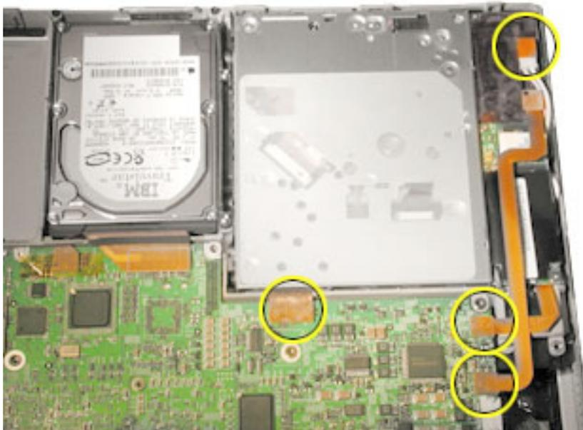
6. Disconnect the bulb wire cable from the inverter board.
