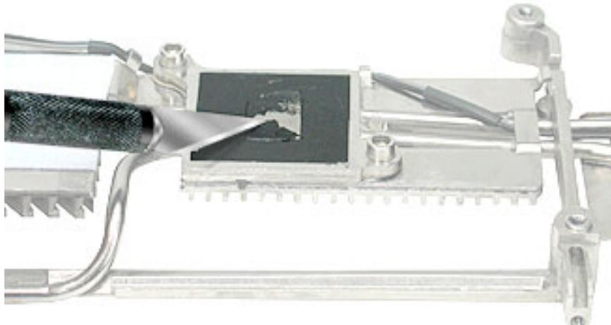
17. **Important:** If you have removed the logic board to access another part, and you will be placing the original logic board back in the computer, use a black stick to gently scrape away any residual thermal transfer material from the microprocessor chip on the logic board.
