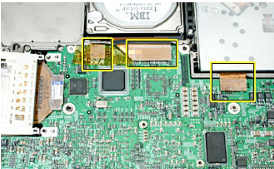
8. Remove the T8 screw on the edge of the logic board near the battery well.
