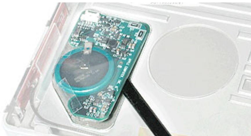
3. If there is any adhesive left on the surface of the inner top case, use a black stick to rub it away. Do not use solvents.
