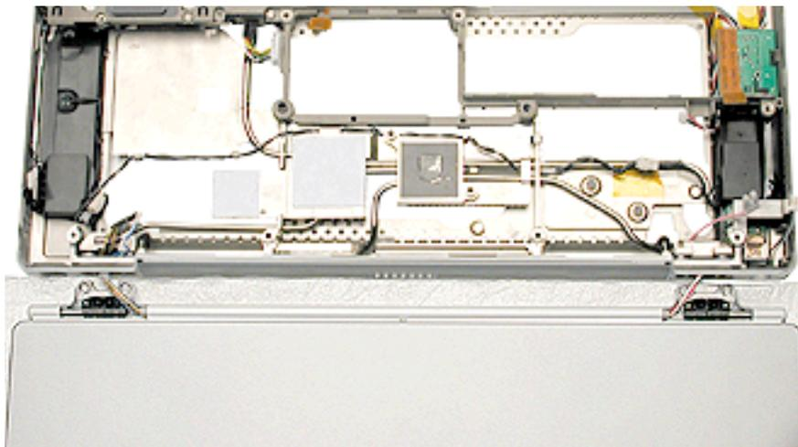
13. Remove the four rib frame screws. Three are identical black T8 screws, the fourth is a longer chrome T8 and also secures the heat exchanger alignment bracket to the end of the heat exchanger. (You might need to move aside the AirPort antenna cable to reach one of the screws.)
