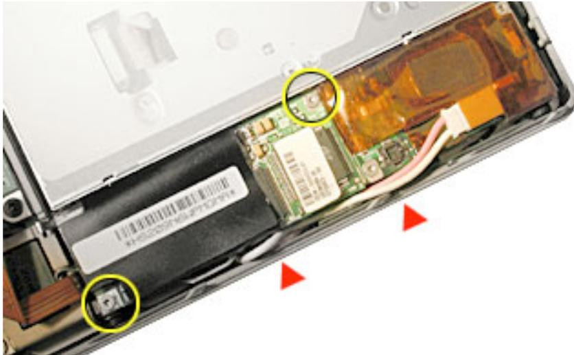
**Important:** Make sure the bottom case is installed correctly. If the slot-load area is slightly bowed, carefully pull the bottom edge of the slot until it clicks into place and becomes flush with the bottom case.
