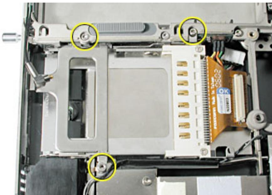
3. Check that the replacement PC card cage includes a clear plastic shim on the outer frame near the PC card eject button. If the shim is not there, transfer the shim from the old PC card cage to the replacement PC card cage.
