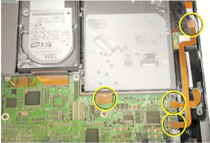
6. Remove the two T6 screws that secure the modem.
