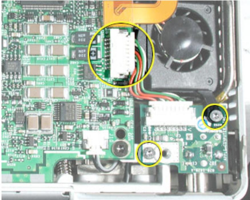
3. Guide the DC-in board out of the case.
