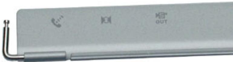
4. Install the replacement I/O door. Make sure each L-shaped pin threads through the top case, inner clutch mount, spring, and plug.
