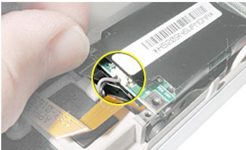
9. Use a thin tool to lift the optical drive slightly, then deroute the modem flex cable.
