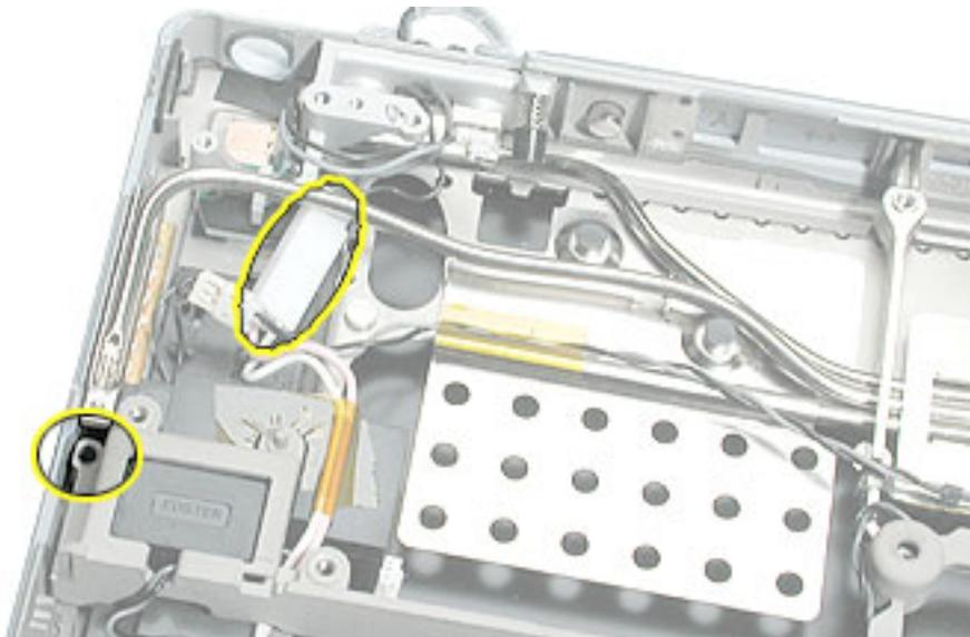
**Replacement Note:** After reconnecting the bulb wire, ensure that the bulb wire cable is safely tucked within the case edge so that it will not get pinched by the bottom case.
