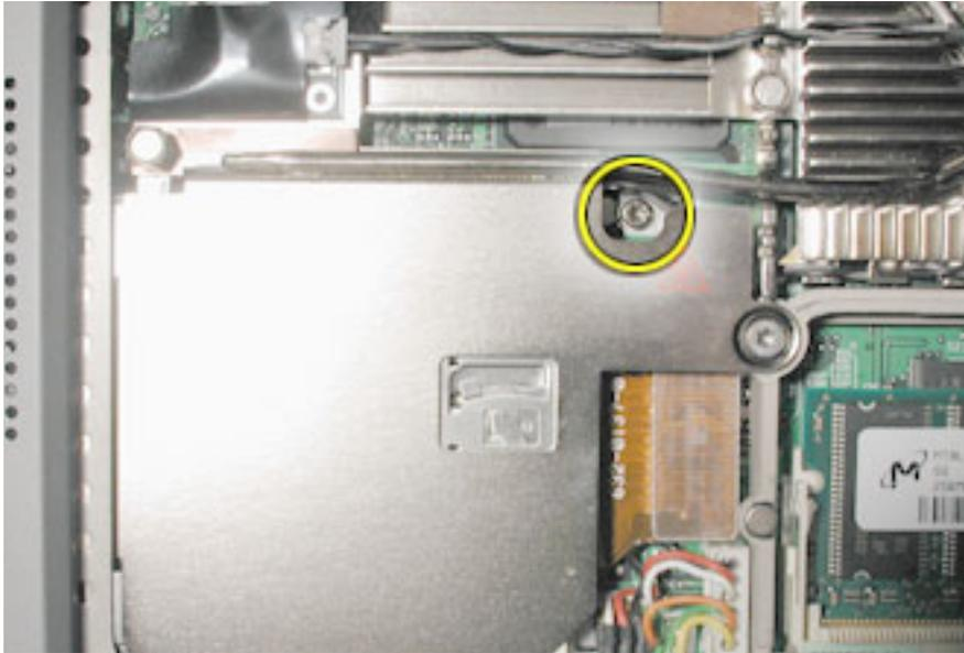
2. Disconnect the PC card flex cable connector and the keyed battery connector.
