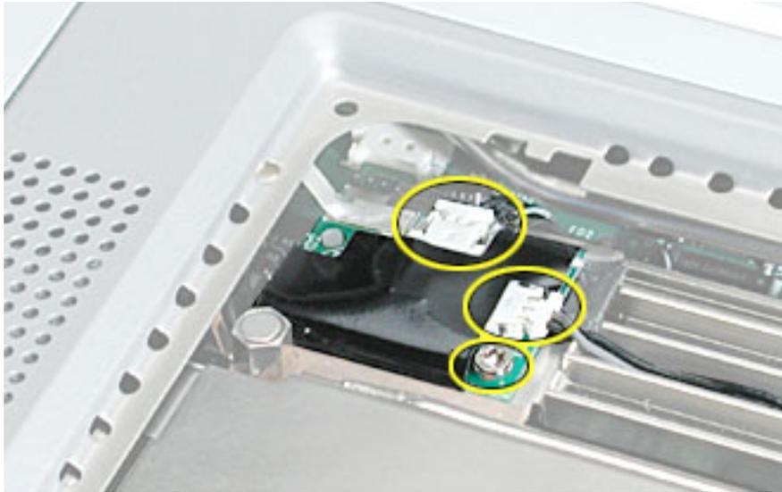
3. Guide the modem filter board out of the case.
