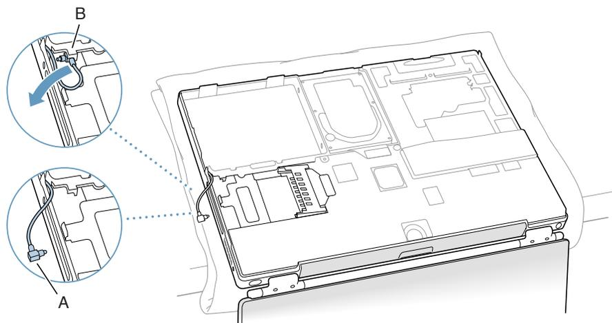
3. Position the AirPort Card (**Figure 10B**) with the AirPort ID numbers and bar code facing up. Pull up the insertion end of the AirPort Card connector (**Figure 10A**) slightly and slide the card all the way into the connector until it is securely attached.
