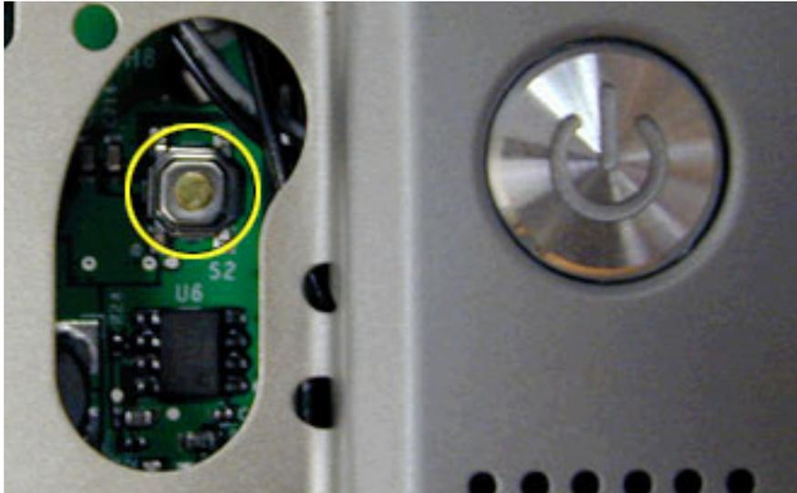
7. Verify power button cable is connected properly to logic board, if power button is not functioning correctly or damaged, replace the top case.
