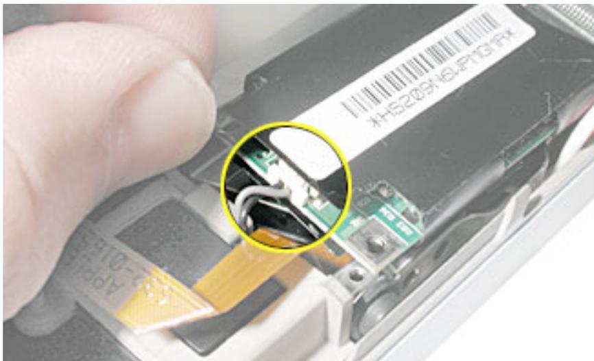
8. Use a thin tool to lift the optical drive slightly, then deroute the modem flex cable.
