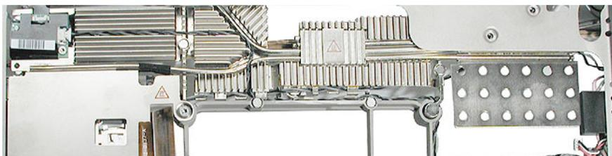
Check that the EMI clip for the optical drive's flex cable has been removed for transfer to the replacement rib frame.
