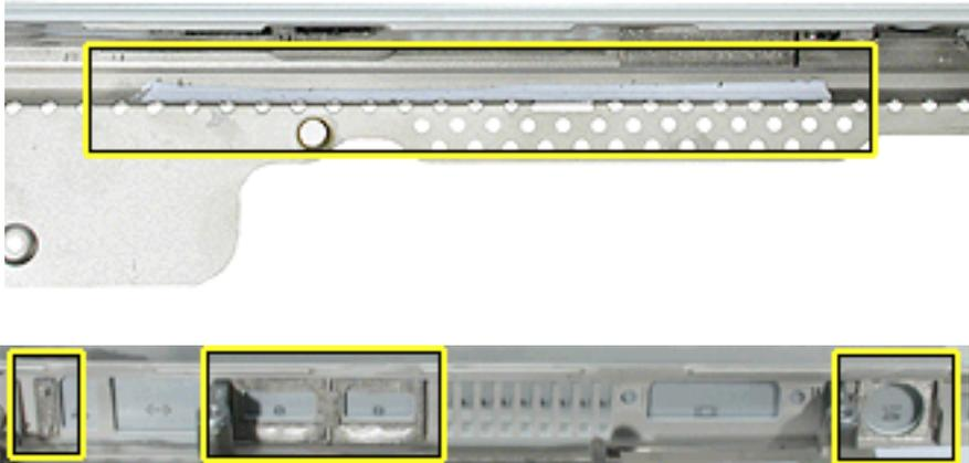
5. **Important:** Make sure you transfer the backup battery cable from the original top case to the replacement top case. The backup battery cable is tucked below the bulb wire cable along and between the speaker and top case, as shown.
