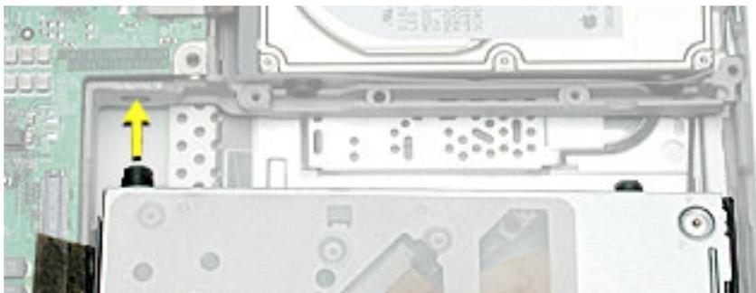
**Important:** When the rubber stoppers are inserted, push down on all four corners of the drive to verify that the drive is level and secure.
