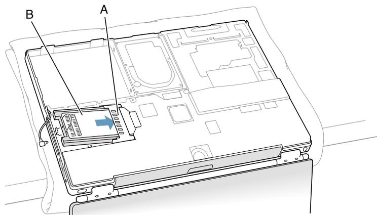
4. Plug the antenna cable connector (**Figure 11A**) into the port on the AirPort Card, located just below the plastic tab (**Figure 11B**). Make sure the connector is straight before inserting it into the port.
