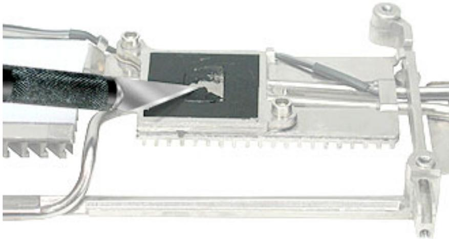
**Replacement Notes:** If replacing the heat exchanger, transfer the hex nut and screw to the replacement heat exchanger.
