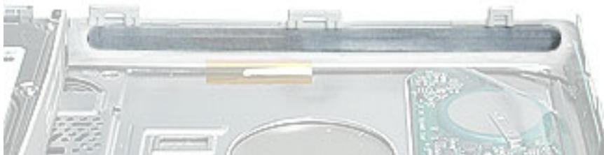
Peel off the felt strip from the inner top case. If there is any residual adhesive on the top case, rub it away.
