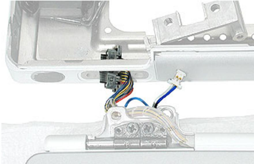
4. At the right clutch, raise the inner clutch mount and disconnect the inverter cable. Carefully slide the inverter cable out through the opening in the top case.
