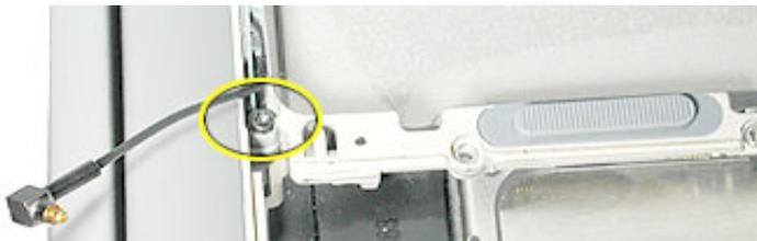
14. Lift the rib frame off of the heat exchanger. If the heat exchanger sticks to the rib frame, press gently on the heat exchanger near the two connection points shown.
