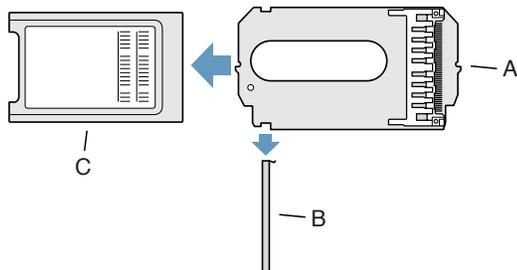
2. If necessary, pull the AirPort antenna cable connector (**Figure 9A**) from its holder (**Figure 9B**).
