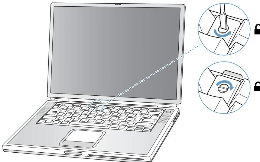
9. Release the keyboard by pulling down on the keyboard release tabs (located to the left of the F1 and F12 keys) (**Figure 3**), then lift the top portion of the keyboard up slightly, and toward the display.
