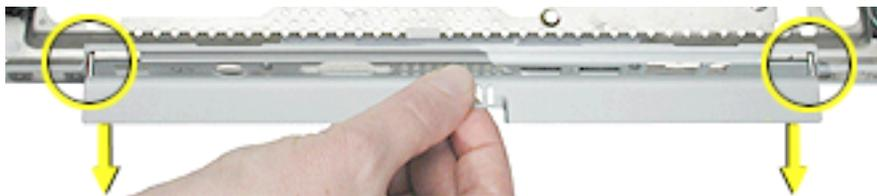
3. Remove the L-shaped pin from each end of the I/O door.
