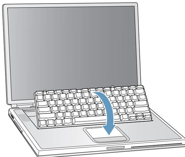
11. Touch the computer's inside framework (a dull gray conductive composite material) to discharge any static electricity, as shown (**Figure 5**).
