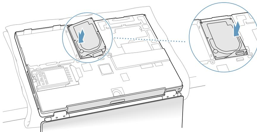
5. Replace the hard drive mounting bracket and secure with the screws. **(Figure 12)**
