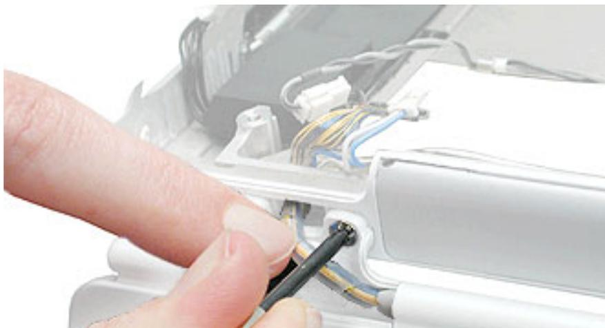
10. At the right clutch, note the routing of the inverter cable. Without straining the inverter cable, gently move it aside so you can access the two large silver-colored screws.
