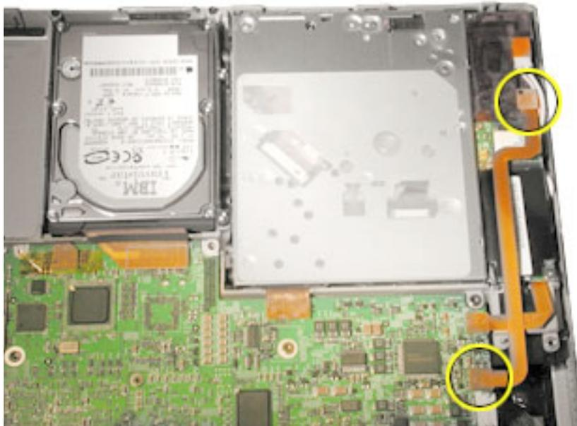
2. Disconnect the bulb wire cable from the inverter board.
