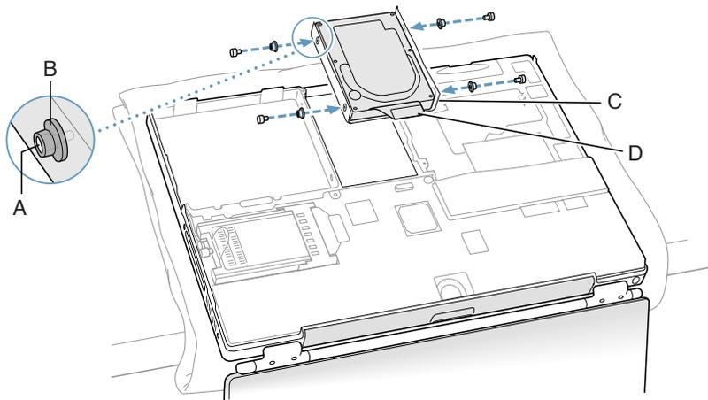
4. Insert the left side of the drive first, then the right. Use a screwdriver through the frame holes on the left side to help align the stoppers, as necessary. (**Figure 11**)
