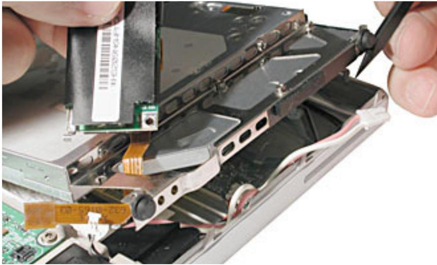
9. If the modem flex cable is not damaged, remove it and transfer it to the replacement modem.
