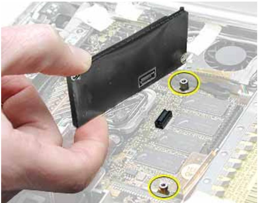
4. Install the replacement modem, and reassemble and test the computer.
