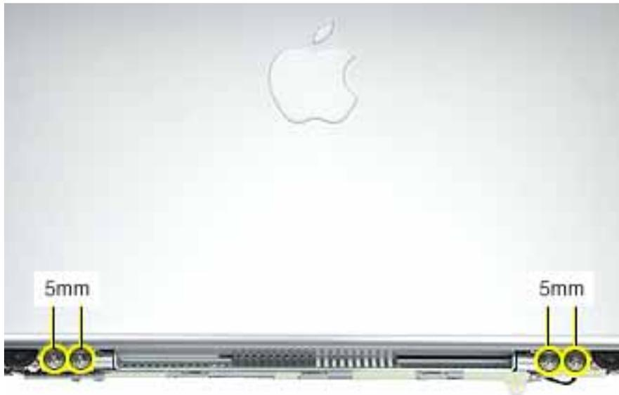
10. Remove the inner rear panel with attached speakers by routing the cables through the slots in the rear panel.
