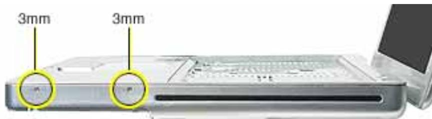
5. Remove two screws from the front left side of the top case.
