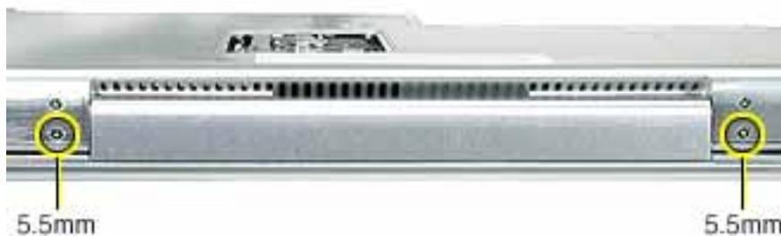
3. Open the display, and with the computer upright, remove the following 13 screws from the top case:
