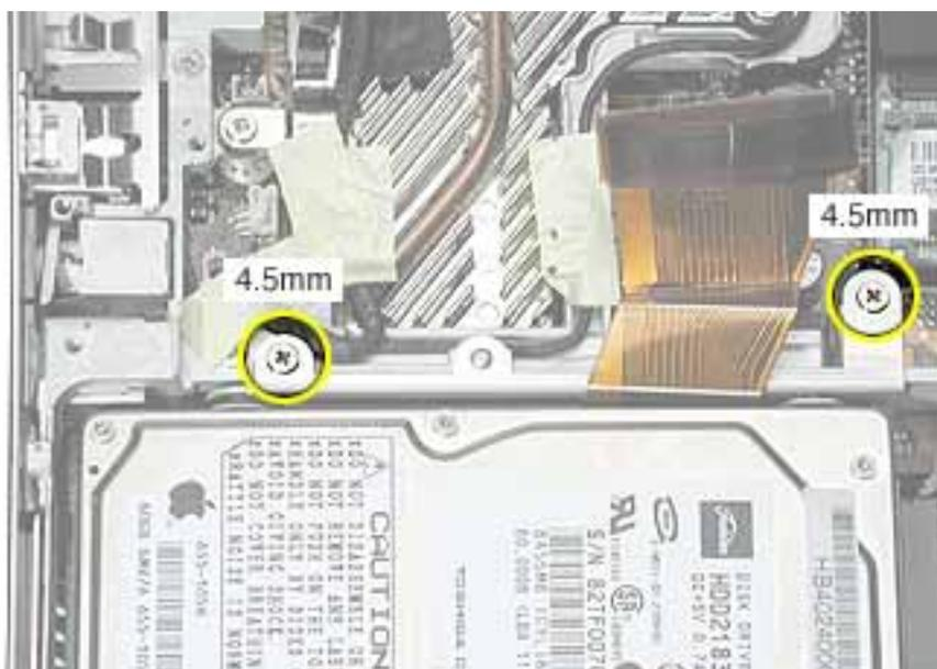
3. Use the flex cable to lift up the hard drive, bracket, and cable from the computer housing.
