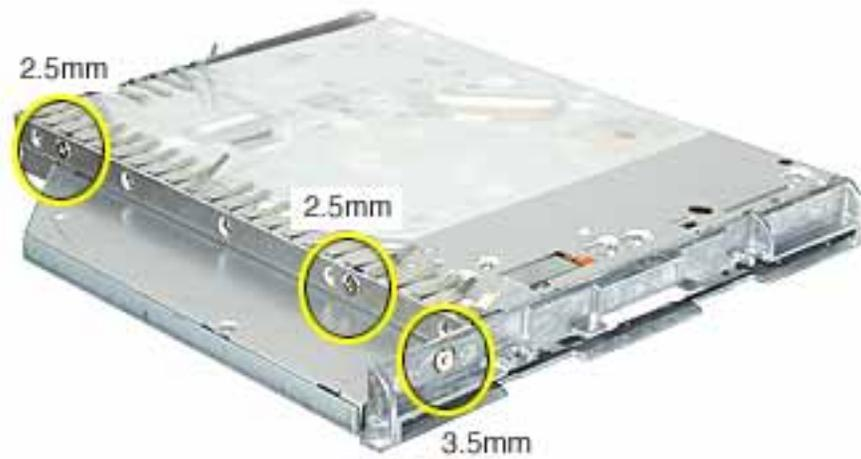
7. Remove the bottom L-shaped EMI bracket.
