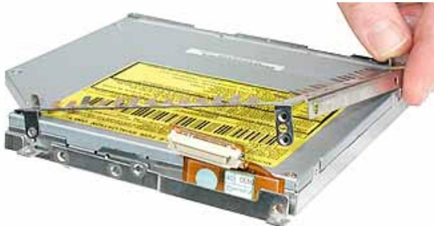
6. Turn over the drive and remove the three screws from the L-shaped EMI bracket on the bottom of the drive.
