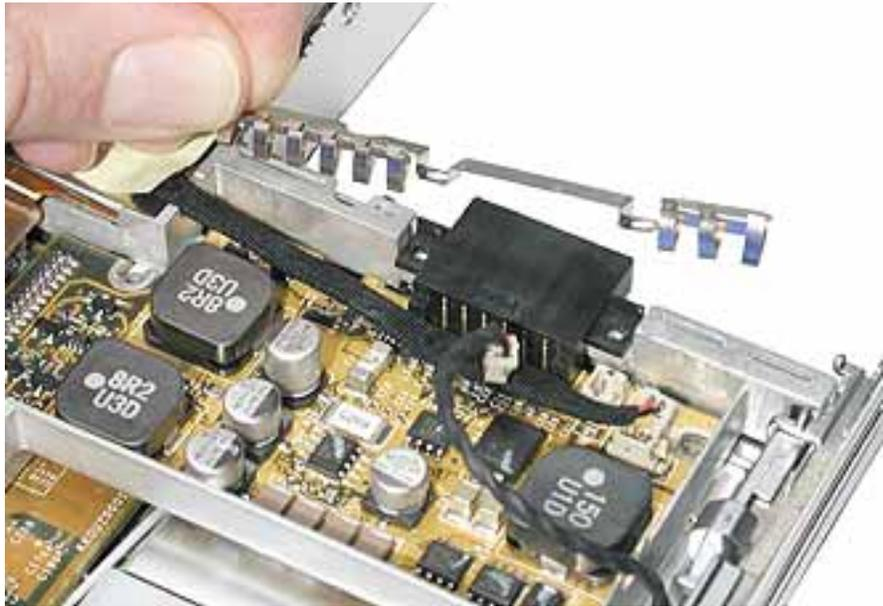
4. Use a black stick to tilt up the board from the logic board, and lift the opposite end of the board to remove it from the computer housing.
