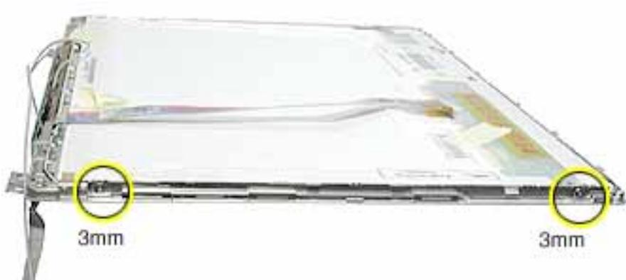
3. Lift off the long EMI clip at the base of the bezel.
