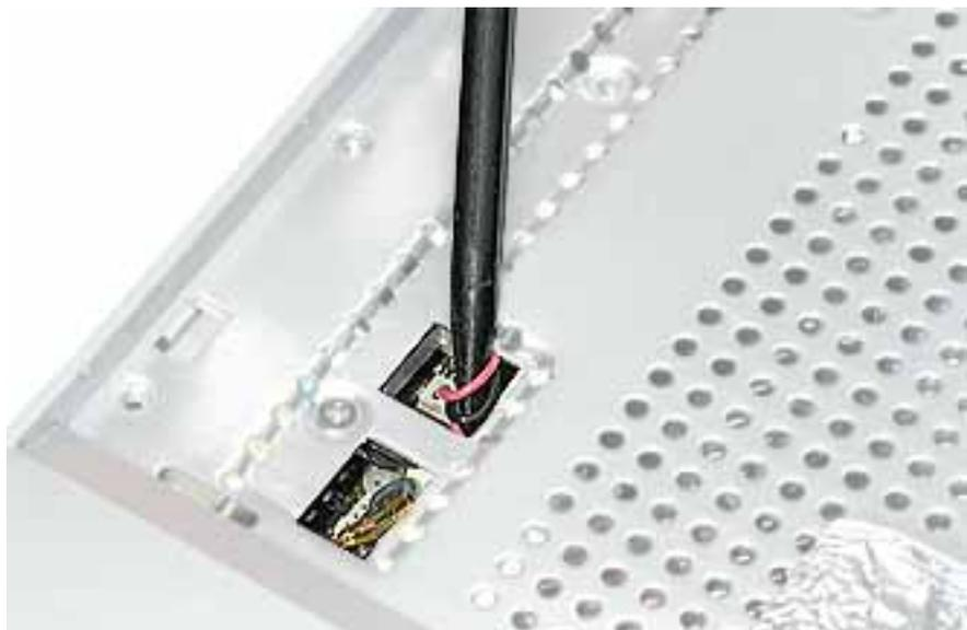
8. Remove the screw near the cables.
