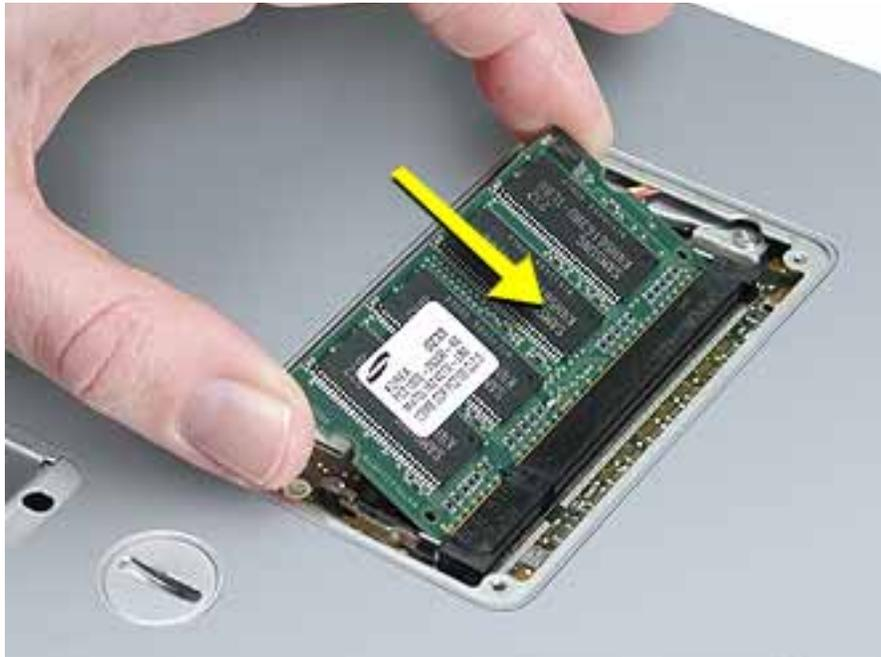
6. Make sure the memory card is fully inserted. Check that the notches in the card clear the tabs as you press down on the sides of the card to lock it into place.
