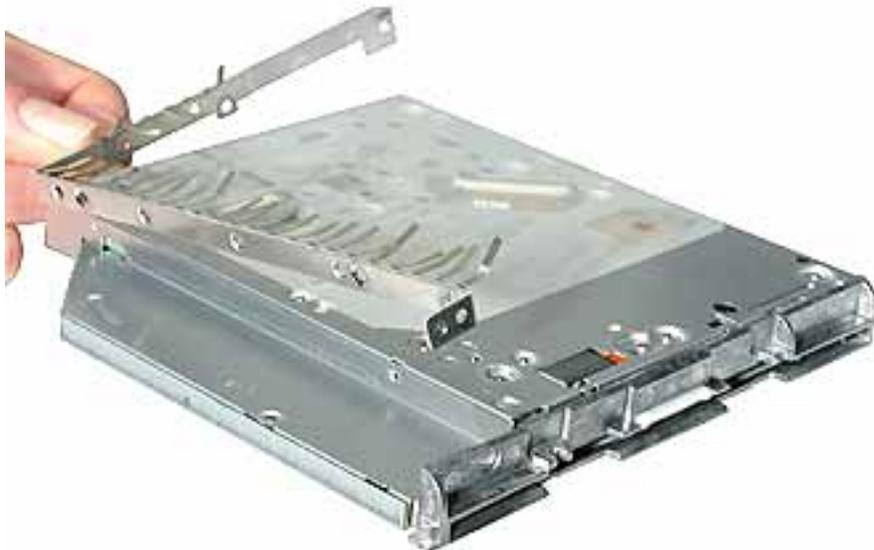
8. Use a black stick to press the tabs and remove the slot load bezel. Pull the bezel straight off the drive.
