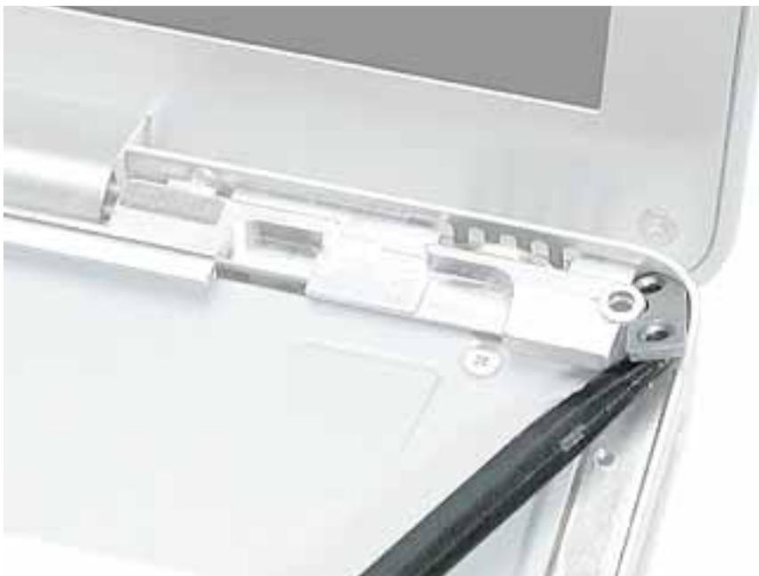
3. Remove the two screws from the slot load bezel.
