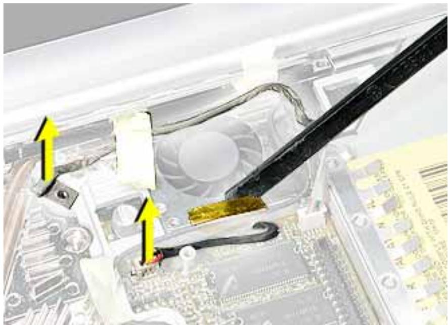
7. Holding the heatsink at the crossbar, begin to lift up the heatsink assembly, being careful where it catches on remaining tape and the chassis. Use a black stick to pry up the middle right corner of the heatsink plate.
