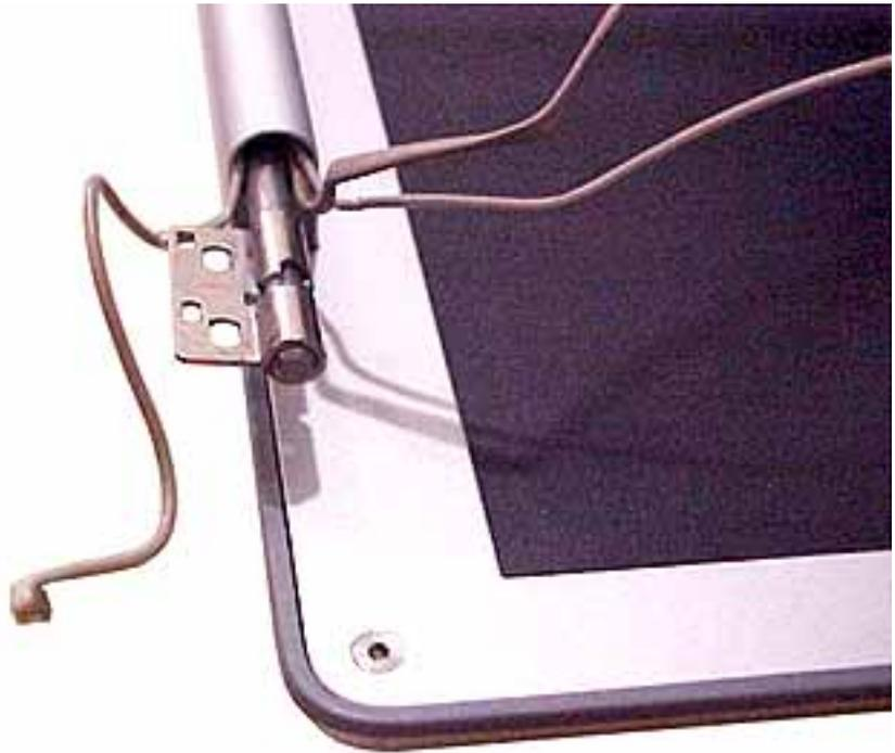
9. From the left side of the bezel, remove the three screws.
