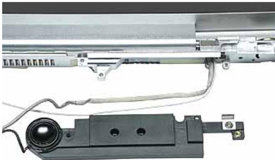
8. With the display open to a 90-degree angle, lift off the display with attached subwoofer and inner rear frame.
