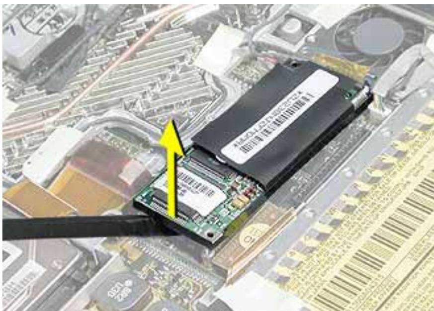
3. At the other end of the modem, disconnect the modem cable from the connector.
