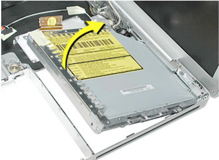
5. Remove the screws from the L-shaped EMI bracket on the top of the drive. Lift off the bracket.
