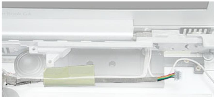
4. **Note:** The back edge of the subwoofer adheres to the rear panel.
