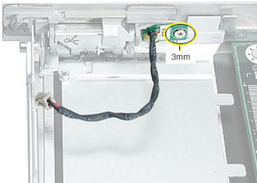
3. **Replacement Note:** Make sure the bottom case has the sleep light pipe installed before installing the replacement sleep light board.
