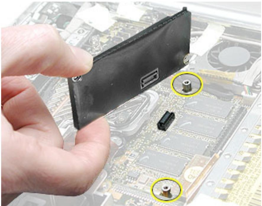
**Replacement Warning:** For the PowerBook G4 (12-inch DVI) model, make sure you reapply the transparent tape over the end of the modem so it overlaps the heatsink at the bottom of the fan, as shown.
