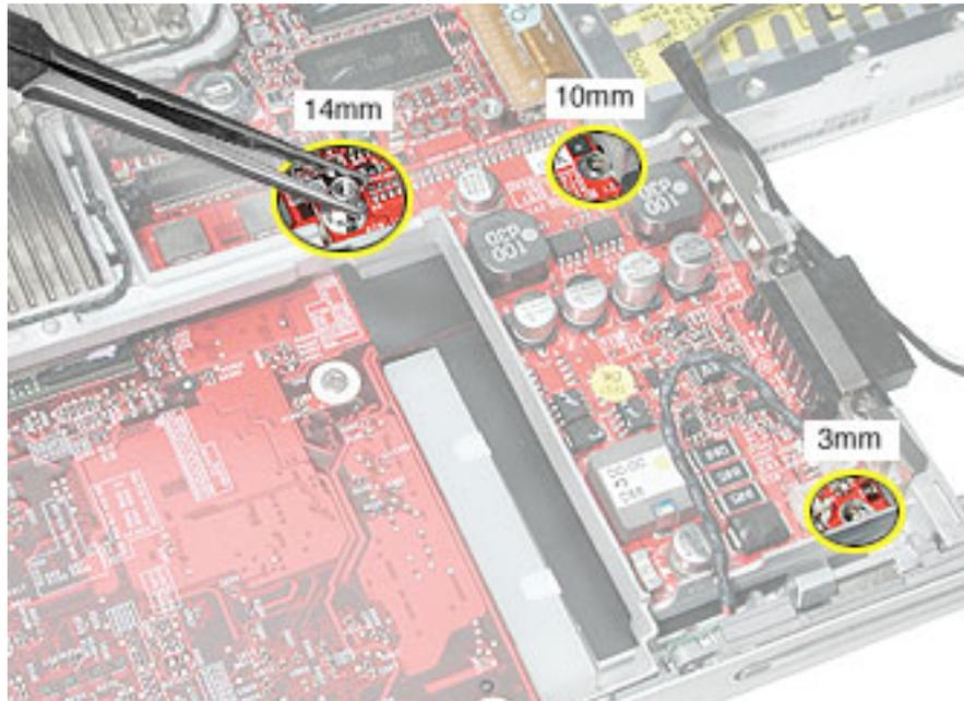
3. Remove the two screws at the battery connector.
