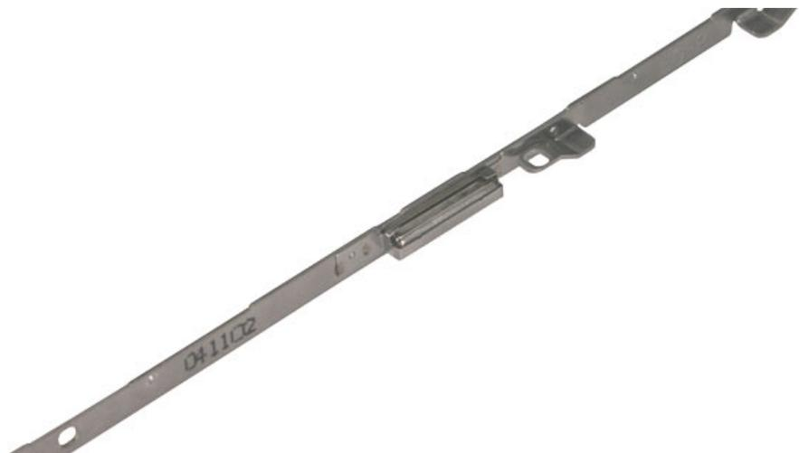
4. From the right side of the bezel, slide out the left hinge with bezel brace (no screws and no magnet on this side).
