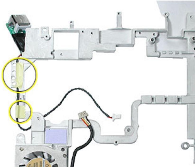
13. Remove the screws from the fan. Transfer the fan to the replacement frame. (Refer to "Fan" in this chapter.)
