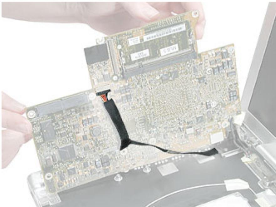
4. Remove the side EMI shield from the I/O ports.
