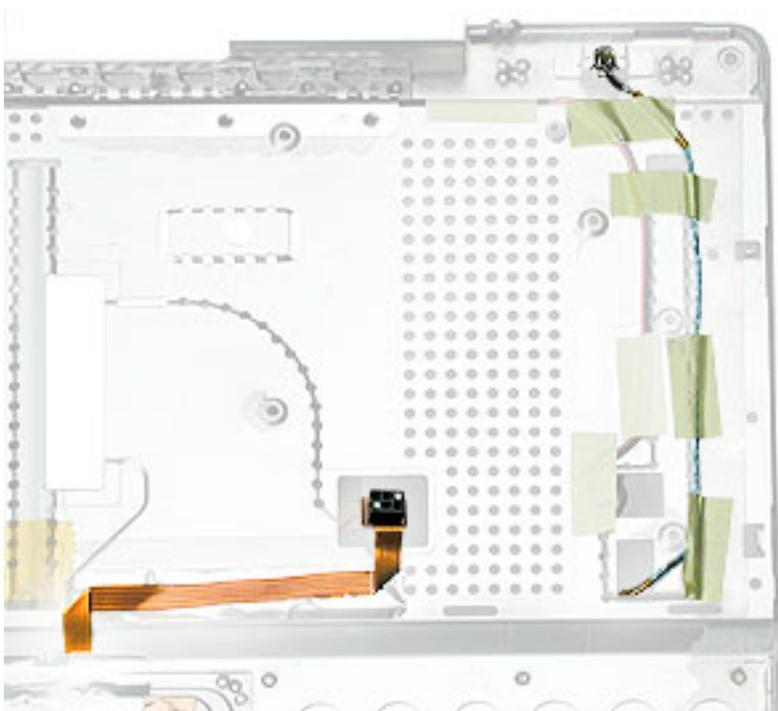
15. Install the replacement top case, and reassemble and test the computer.
