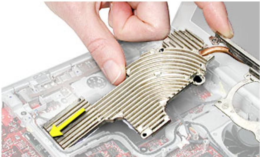
9. Install the replacement heatsink, and secure the screws using the following sequence:
