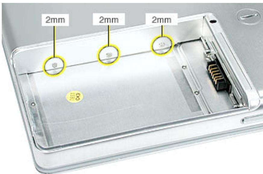
2. Remove the screws near the display hinge.
