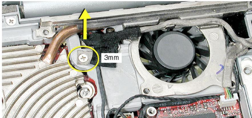
6. Use a black stick to pry up the lower right side of the heatsink plate. Holding the heatsink at the crossbar, begin to lift up the heatsink assembly, being careful where it catches on remaining tape and the chassis.
