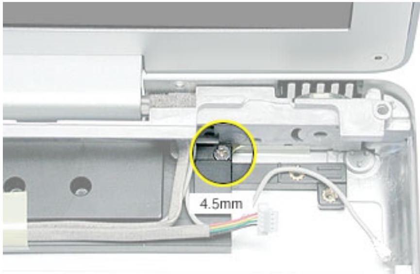
3. Remove the remaining tape from the subwoofer and the loose cable.
