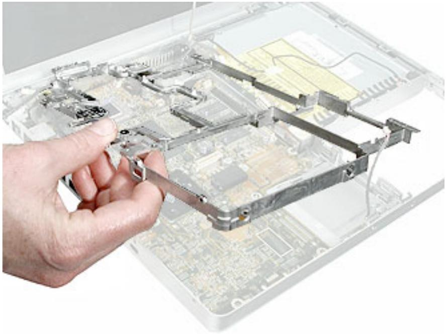
17. Remove the tape that secures the RJ11 board and cable to both sides of the frame. Transfer the RJ11 board and cable to the replacement frame.
