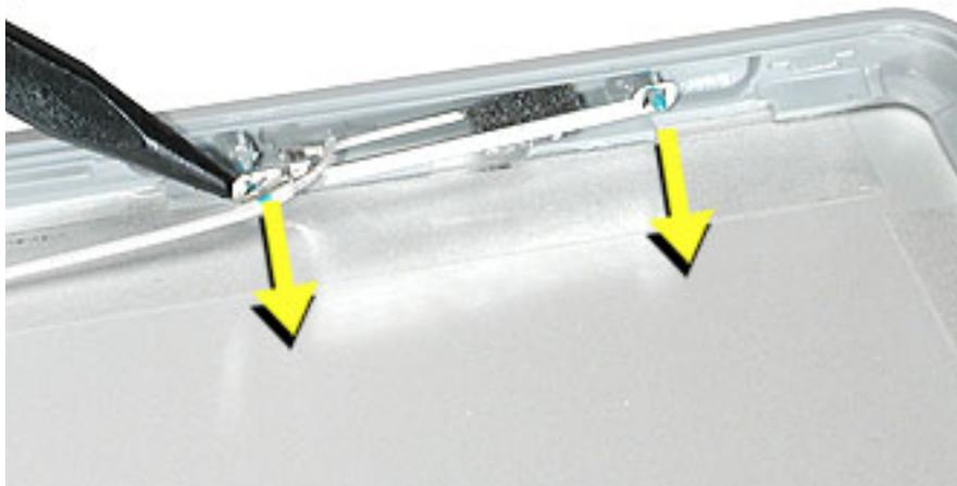
8. Placing the antenna cables and receptors aside, remove the display housing.
