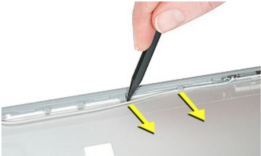
7. **Note:** The antenna receptors are held in place with glue at each post. Use a black stick at the end of each antenna receptor to gently pry it off the post.
