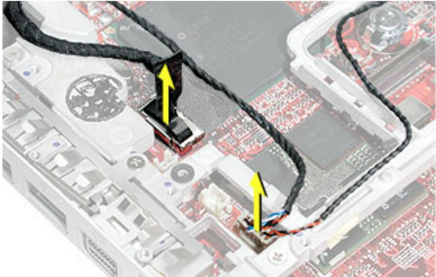
**Replacement Note:** When reinstalling the LVDS cable, tuck the pull-tab under the frame.
