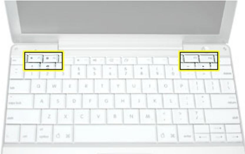
3. **Important:** Using a black stick, carefully pry up each of the four keys from the left side of each key. The keys are easily removed from the left side without damaging the keyboard.
