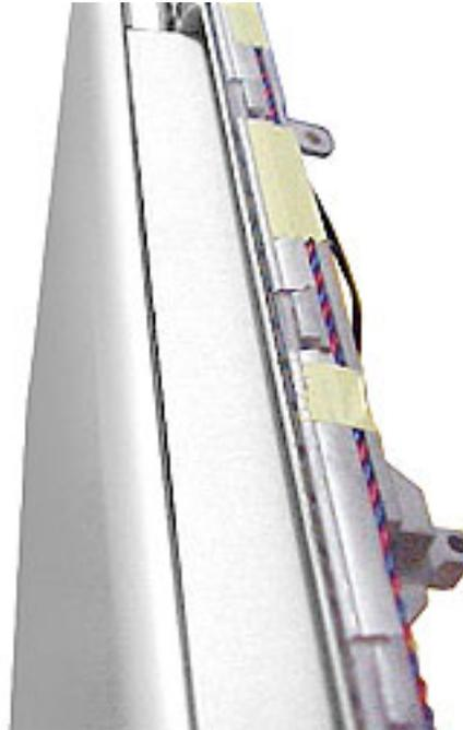
**Replacement Note:** Check that the orientation of the cables directed through the rear panel openings are as shown below:
