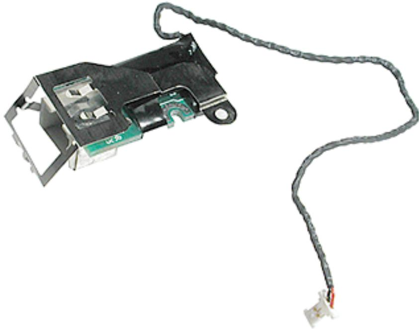
3. Secure the replacement RJ11 modem board and cable to the frame, and reassemble and test the computer.
