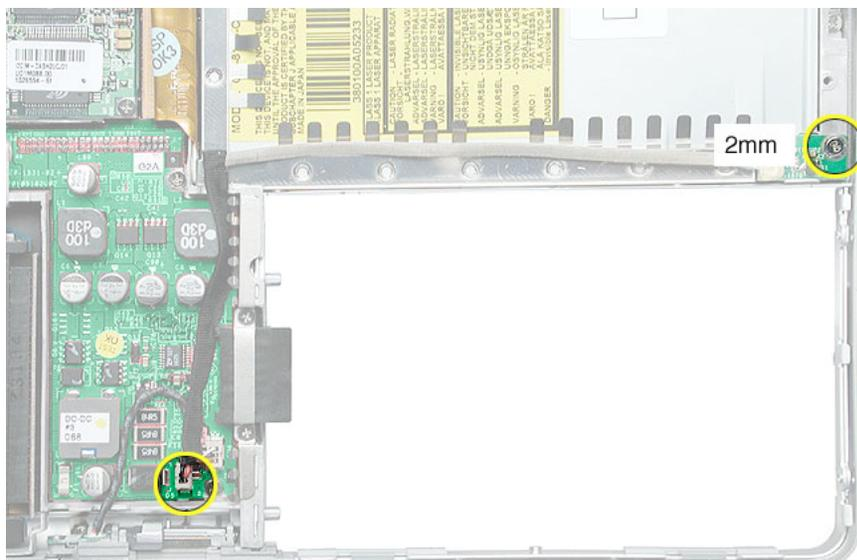
4. Install the replacement hall effect sensor board and cable, and reassemble and test the computer.
