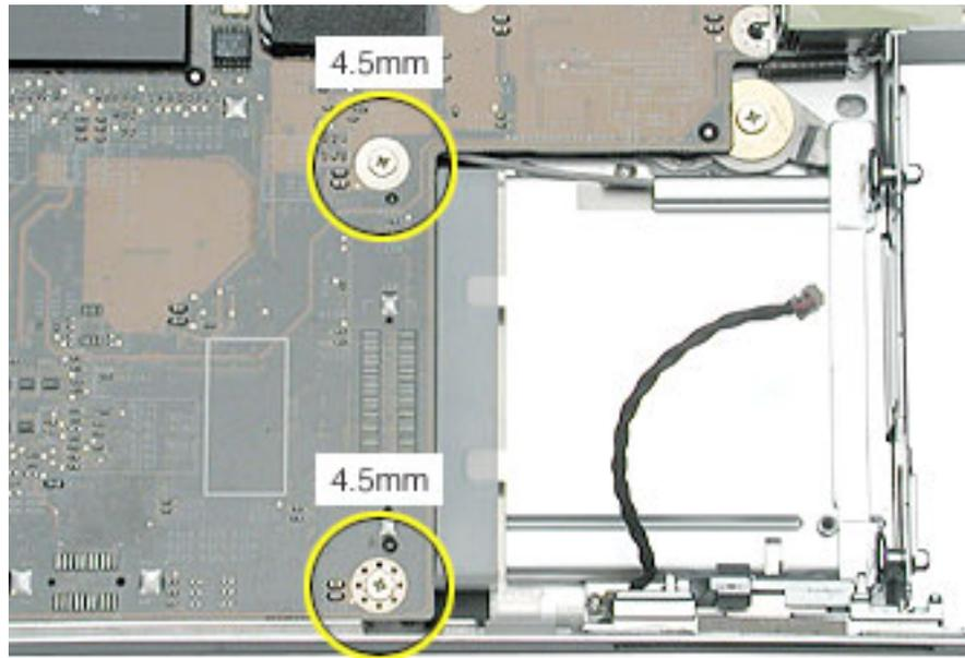
2. Holding the edges of the board tilt up the logic board.
