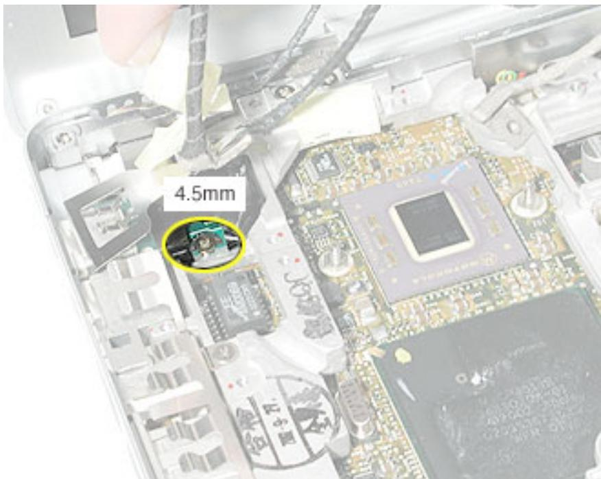
9. Tilt up the RJ11 modem cable board and remove the 6-mm long screw (not shown) that secures the frame to the logic board.
