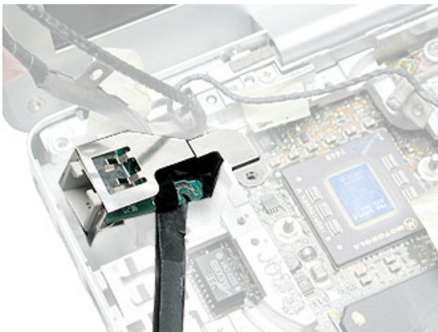
10. Remove the two screws at the I/O ports.
