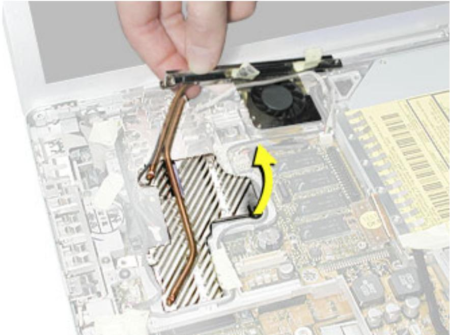
8. Route the fan cable through the slot in the computer frame.
