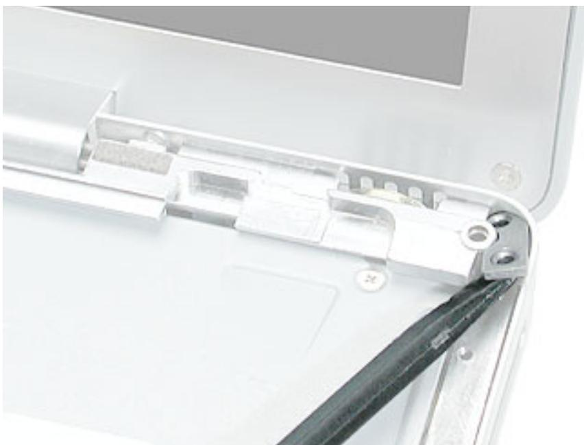
3. Remove the two screws from the slot load bezel.
