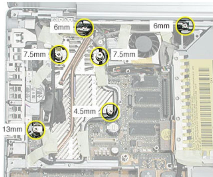
3. Remove the tape that covers the heatsink and secures the cables in place.
