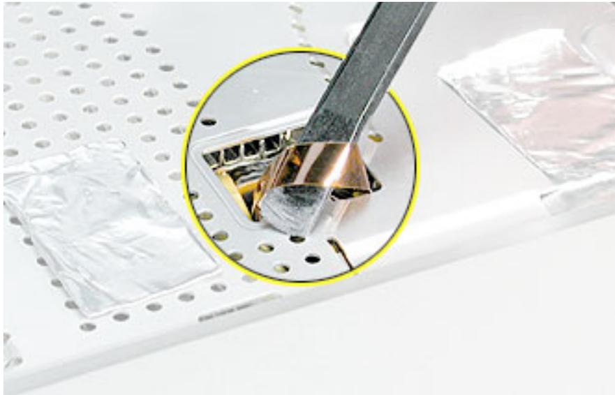
10. Raise the top case up slightly from the bottom case until you can access the cables that are connected under the top case.
