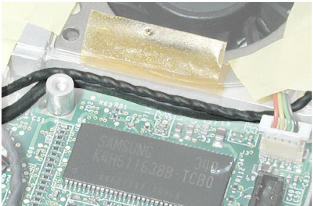
7. Peel up any remaining tape, and remove the screws from the frame and I/O port shield.
