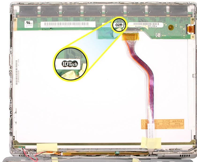
2. If the label on the LCD panel shows Samsung as the manufacturer, order replacement hinges that show a SAM-L or SAM-R designation on the outer arm of the bezel brace.
