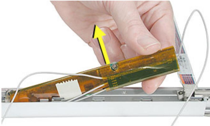
3. Peel away the tape and mylar cover that holds the inverter board and the antenna cable assembly together.
