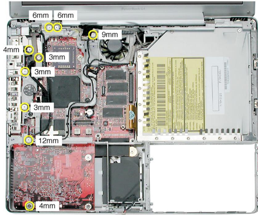
8. Tilt up the RJ11 modem cable board and remove the 6-mm long screw (normally hidden by the RJ11 board).
