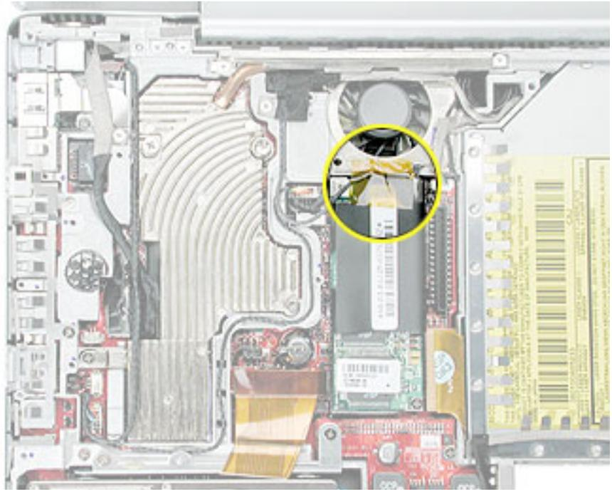
4. Install the replacement modem, and reassemble and test the computer.
