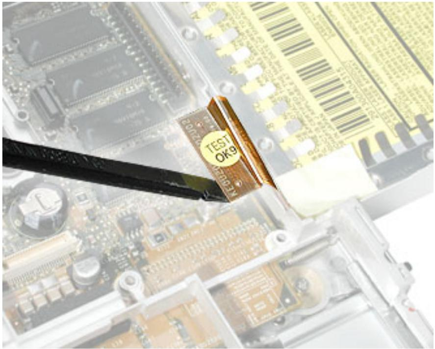
10. Lift up the frame, being careful where it catches on the optical drive flex cable or other cables.
