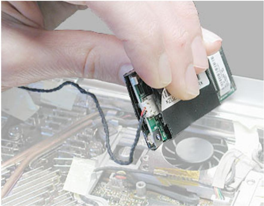
**Replacement Note:** When placing the replacement modem on the logic board, be sure to align the board over the standoffs and connector on the logic board.
