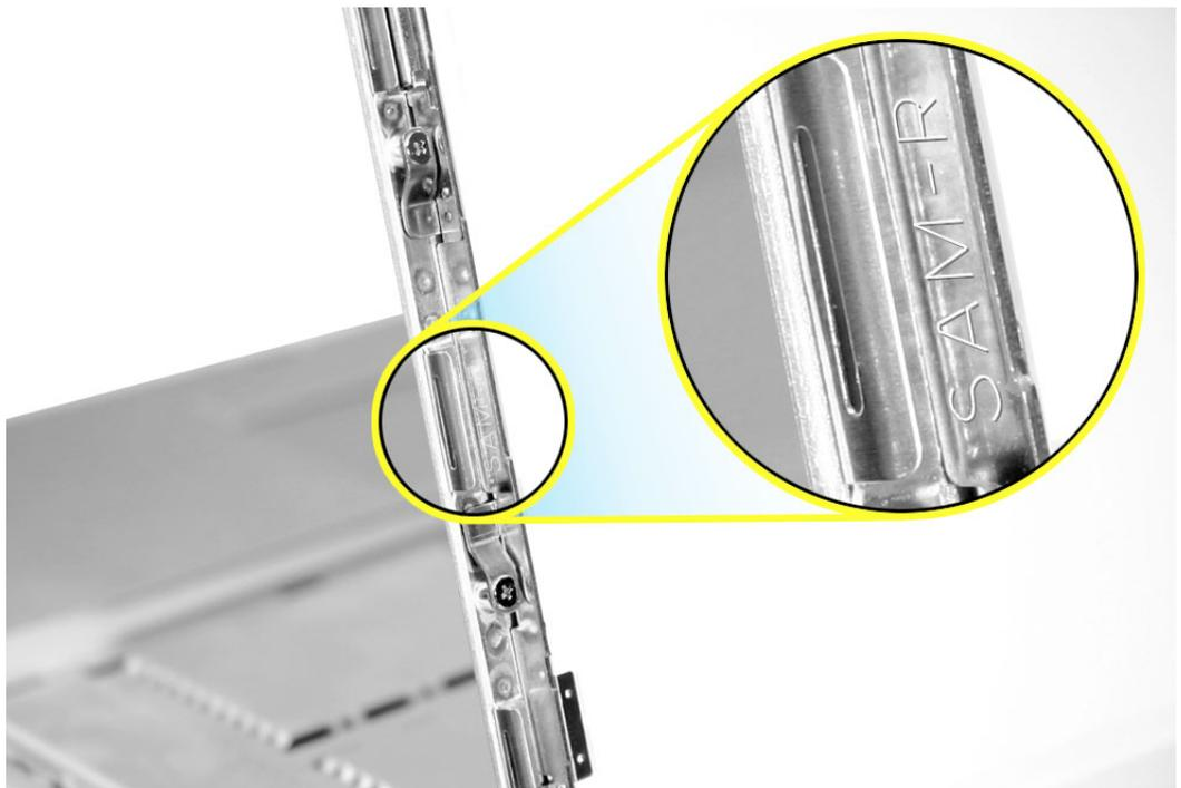
3. If the label on the LCD panel shows IDTech as the manufacturer, order replacement hinges that show an LG-L or LG-R designation on the outer arm of the bezel brace.
