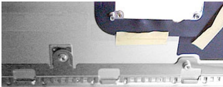
8. Remove the four screws from the display's inner rear panel. Make sure the screwdriver does not touch the speakers.
