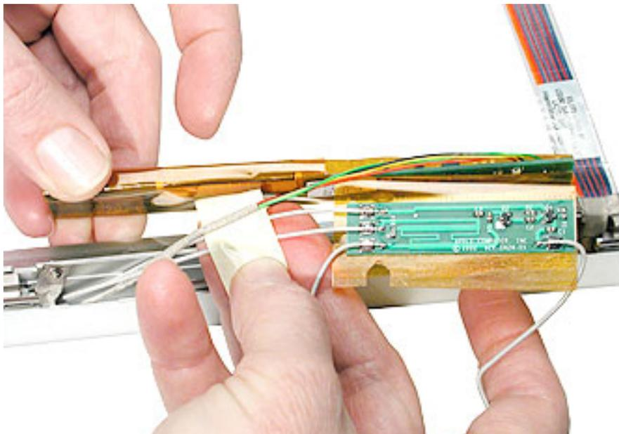
4. Separate the antenna cable assembly (board with attached antenna cables and Bluetooth cable) from the inverter board.
