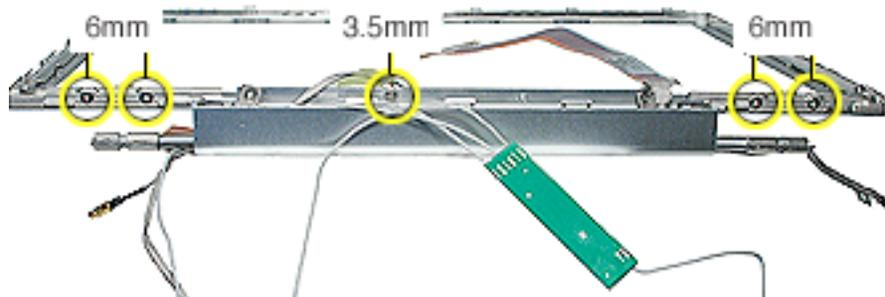
7. Separate the clutch cover from the bezel and remove the LVDS cable.
