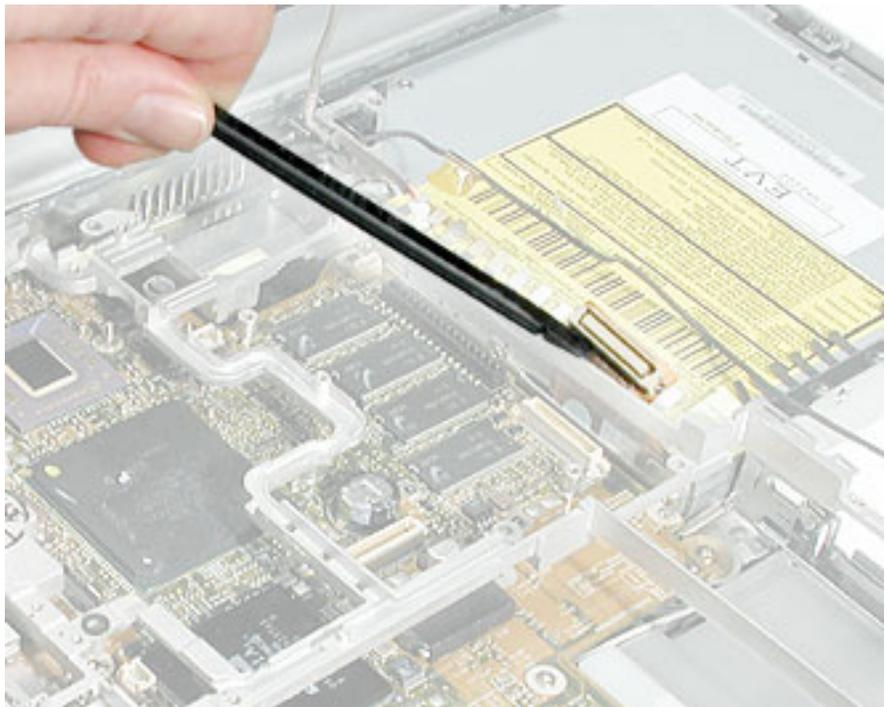
11. Lift the inner frame out of the computer assembly.
