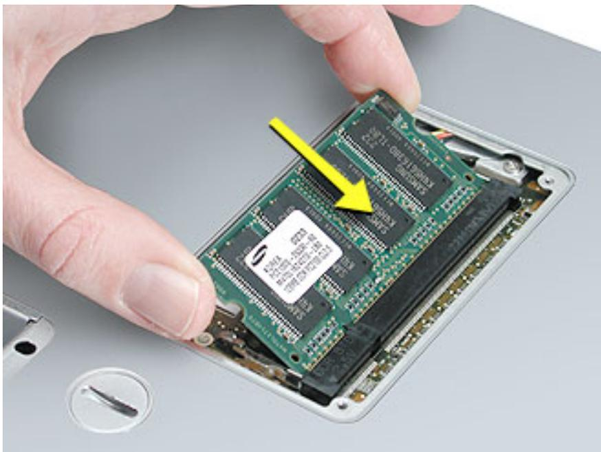
7. Make sure the memory card is fully inserted. Check that the notches in the card clear the tabs as you press down on the sides of the card to lock it into place.
