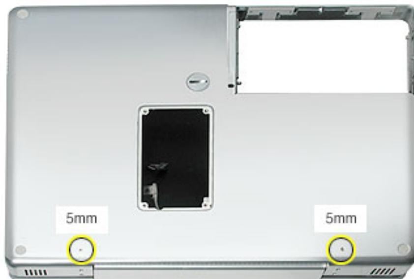
2. Remove the two screws near the display hinge.
