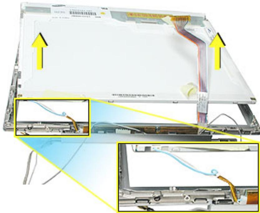
5. Install the replacement LCD panel, and reassemble and test the computer.
