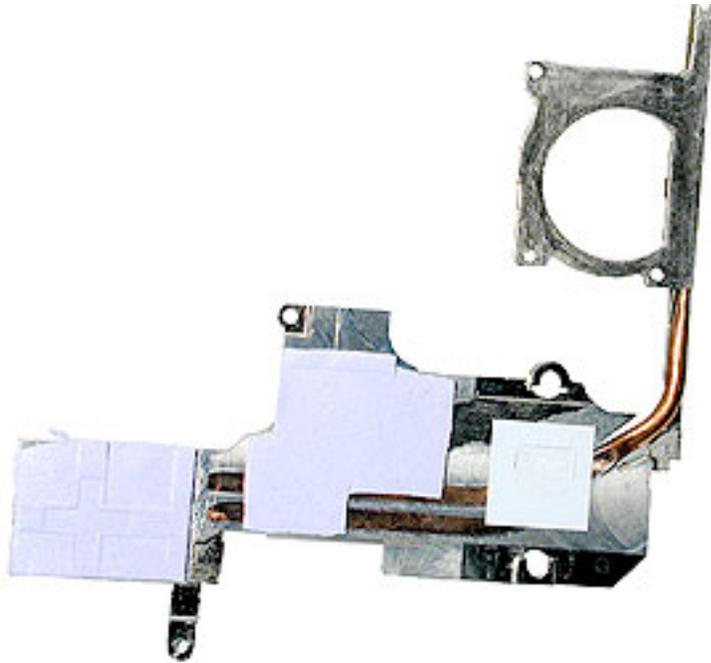
8. When installing the heatsink, first insert the lower flange of the heatsink panel under the frame.
