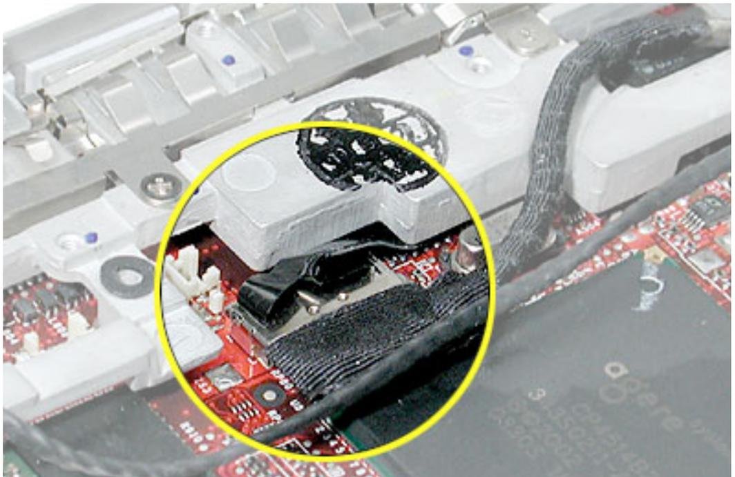
6. Near the fan, disconnect the two connectors shown
