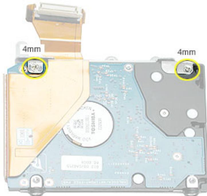
5. Peel up the flex cable from its double-sided tape.
