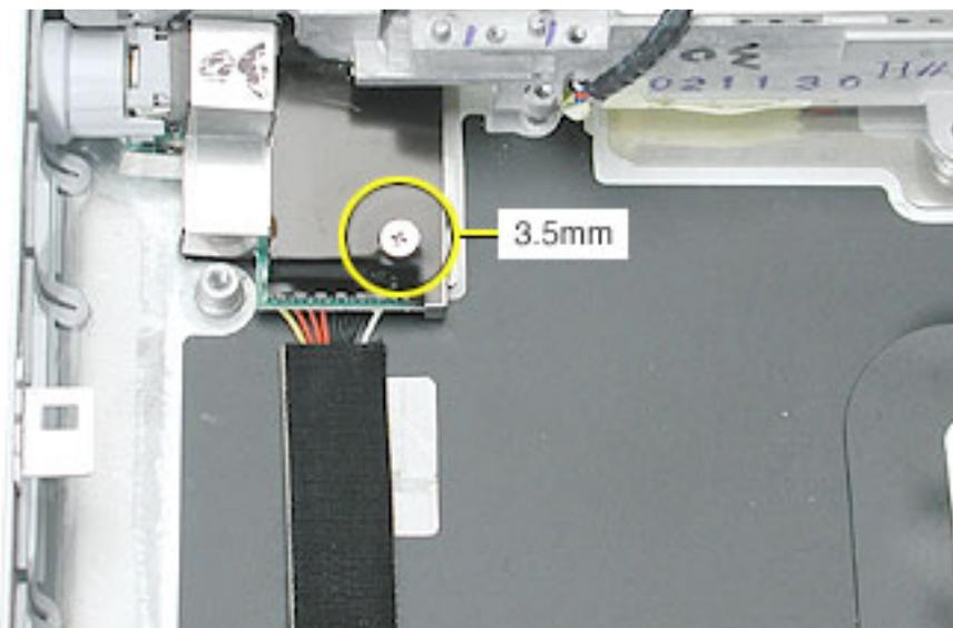
2. Pull the flat cable up from the adhesive on the bottom case.
