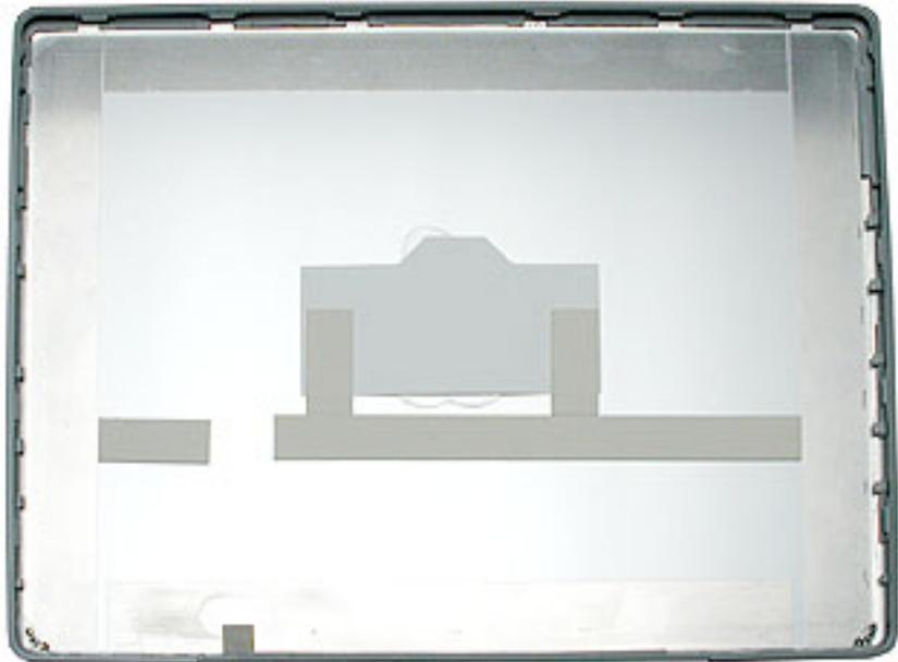
**Replacement Note:** When installing the replacement display housing, make sure the antenna cables are secure under all of the inner tabs that run along the sides and bottom of the display housing.
