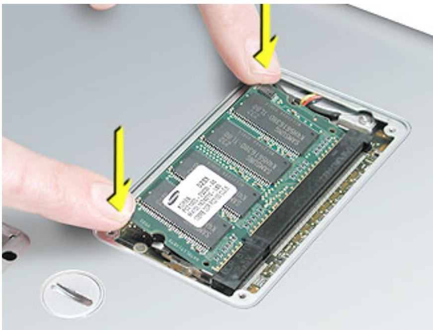
8. Install the memory door. Be careful not to overtighten the screws.
