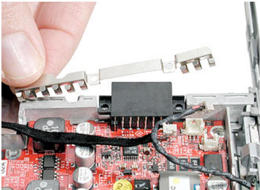
5. Place a black stick just under the top edge of the board at the modem standoff. Disconnect the DC-to-DC board from the logic board by prying up the DC-to-DC board and removing it from the computer assembly.
