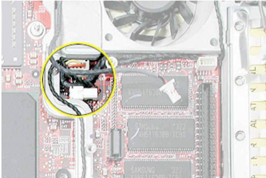
**Replacement Warning:** When reassembling the computer, notice the two black insulated cables that run along the bottom of the fan. To avoid damaging the cables, make sure that the thinner twisted cable is routed on top of the thicker fan cable and that both cables are routed between the fan and the modem standoff, as shown.
