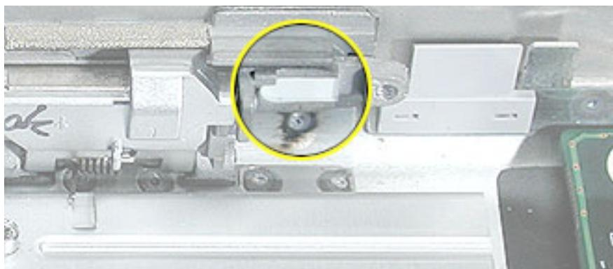
4. Install the replacement sleep light board, and reassemble and test the computer.
