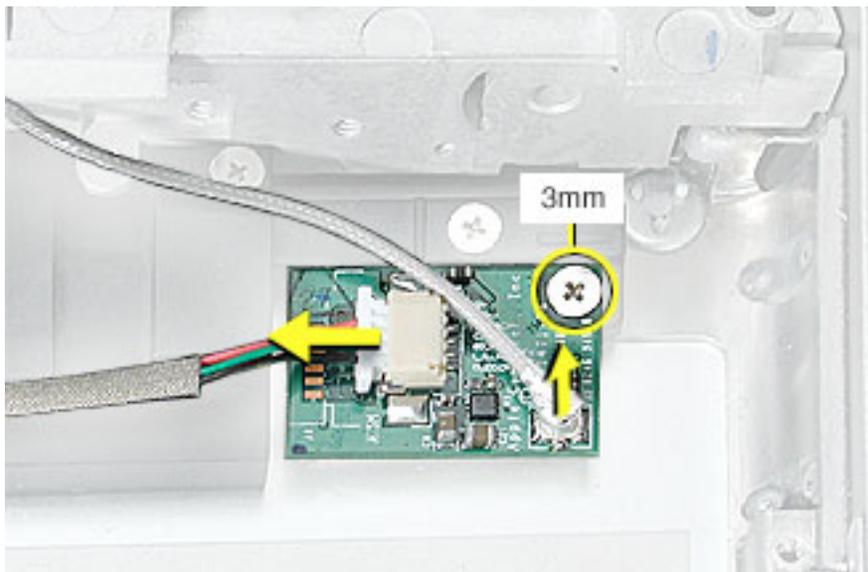
5. Remove the Bluetooth board from the bottom case.
