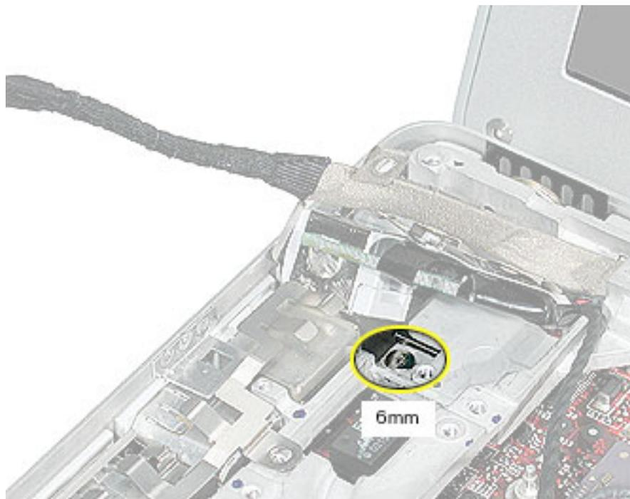
9. Disconnect the optical drive flex cable.
