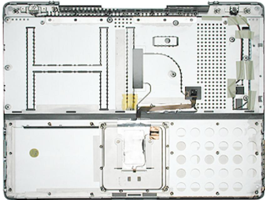
14. Before installing a replacement top case, check the cable routing of the
