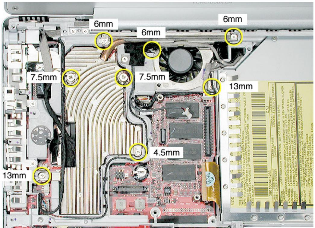
3. Near the fan, peel up the tape that secures the cables to the heatsink.
