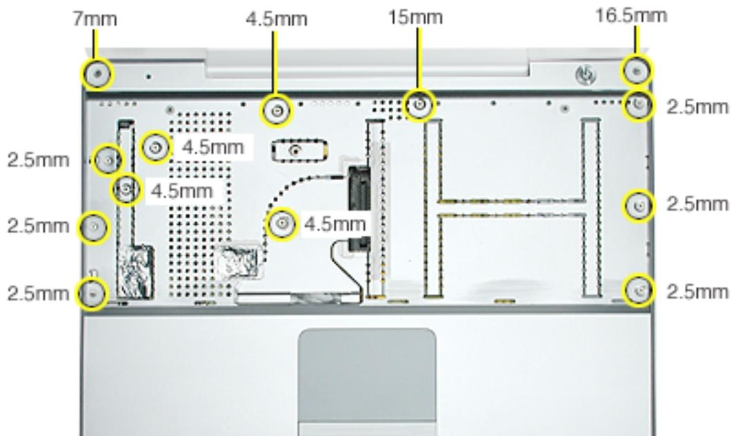
4. Carefully peel up the two pieces of foil tape that cover the microphone cable, power cable, and trackpad cable. Reserve the tape when reassembling the computer.
