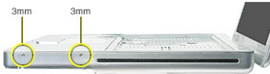
**Replacement Note:** In addition to securing the top case to the bottom case, the two 3-mm long screws help secure an inner bracket to the battery well. Make sure the bracket is installed in the bottom case before replacing the top case.
