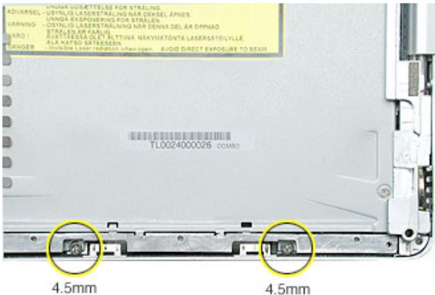
4. Tilt up the optical drive and remove it from the computer.
