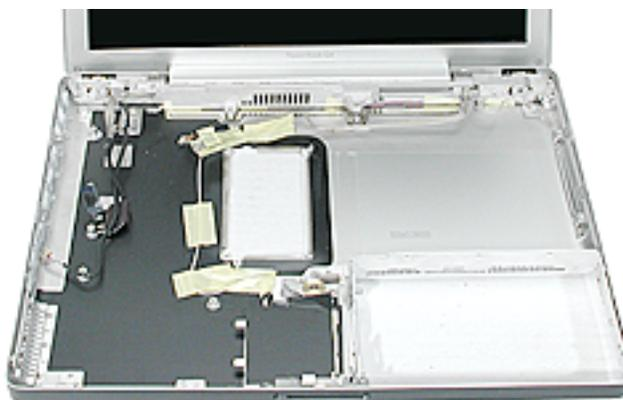
4. Note the routing of the AirPort antenna. Using a black stick, start to thread the AirPort antenna cable through the AirPort Extreme Card bay.
