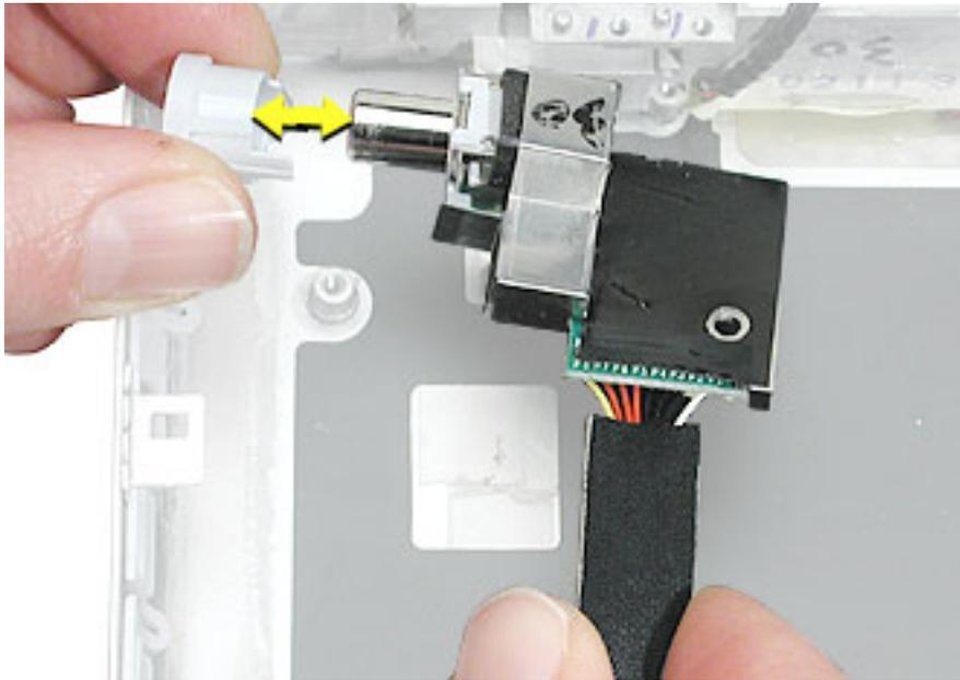
5. Install the replacement DC-in board, and reassemble and test the computer.
