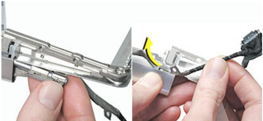
8. Remove the antenna cables and inverter from the clutch cover.
