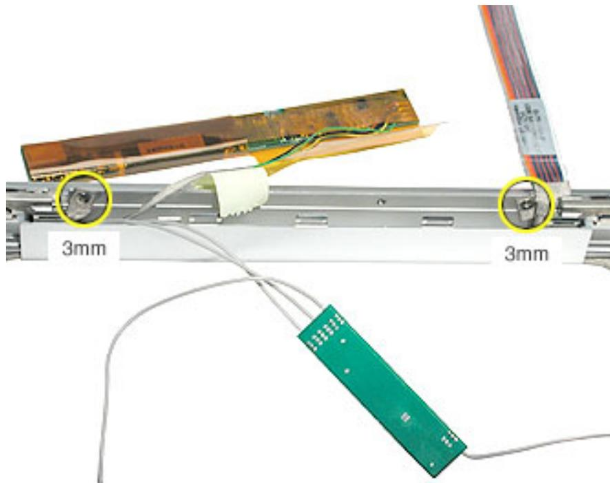
6. Remove the five screws from the bottom edge of the display bezel
