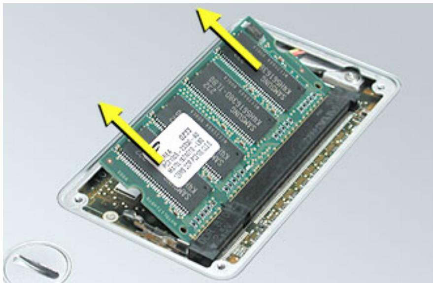
6. Insert the replacement memory card into the expansion slot at a 30-degree angle.
