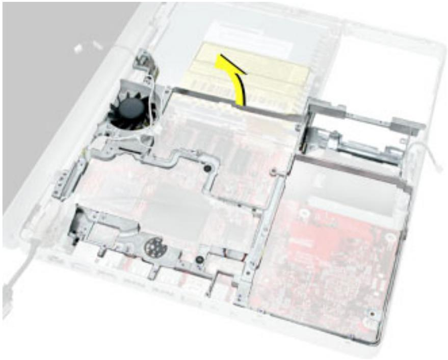
12. Remove the tape that secures the RJ11 board and cable to both sides of the frame. Transfer the RJ11 board and cable to the replacement frame.
