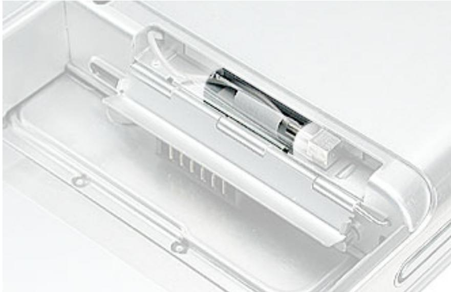
**Note:** The AirPort slot on the bottom case has a recessed inner slot designed for the clear plastic tab to tuck into.
