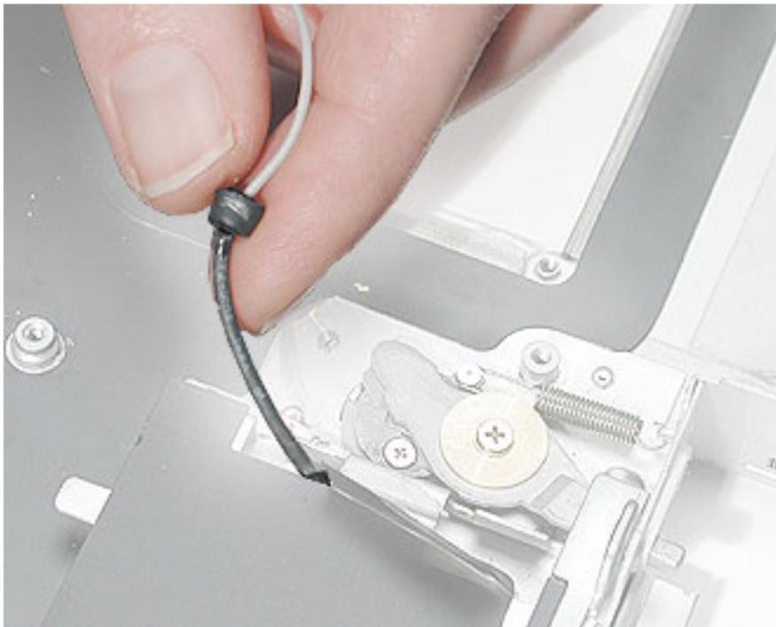
6. Support the antenna cable as you direct the antenna plug out of the opening in the card bay.
