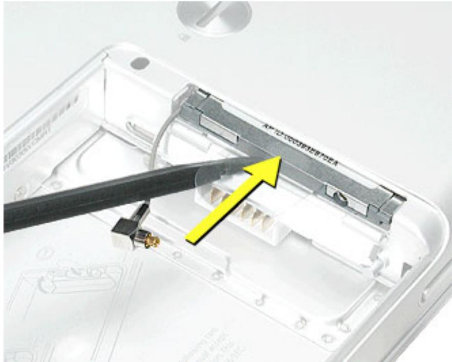
7. Connect the end of the antenna cable to the card.
