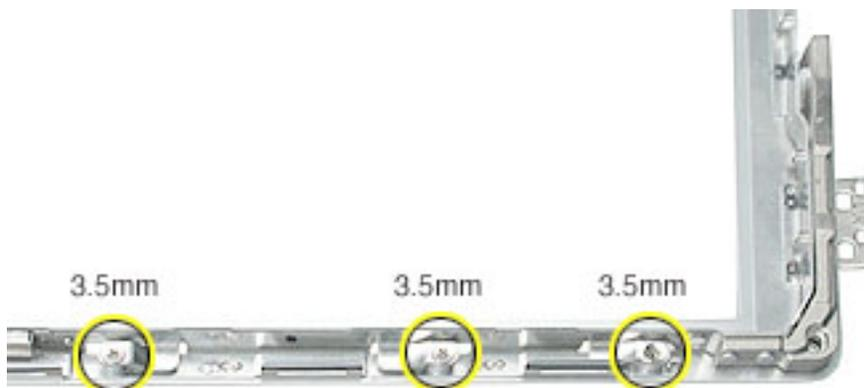
2. Remove the right hinge with bezel brace from the left side of the bezel.
