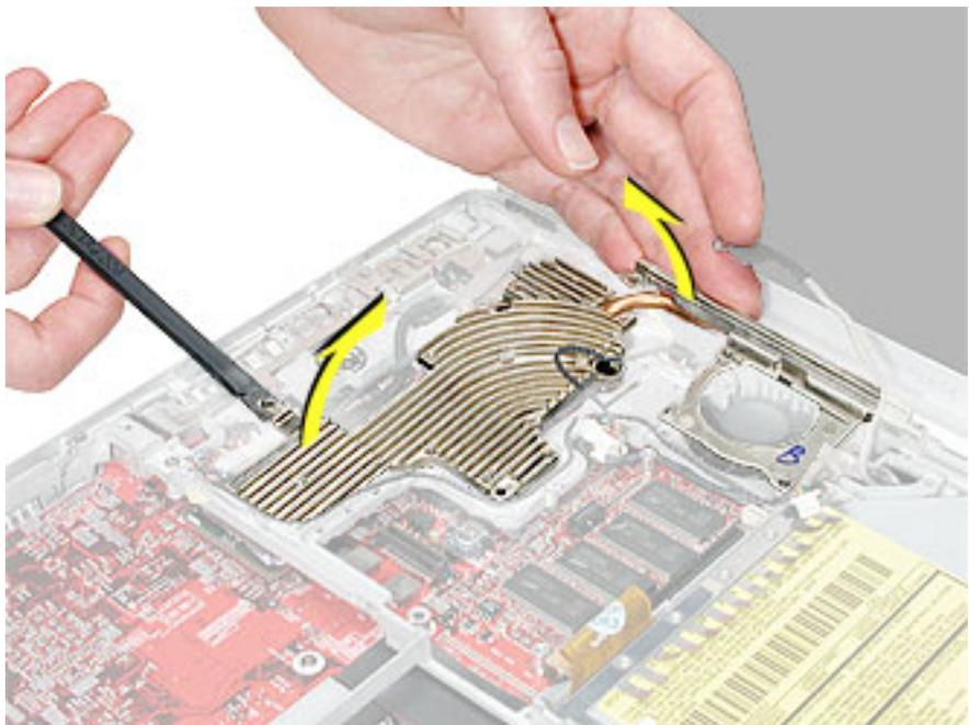
7. Check the thermal pads on the heatsink:
