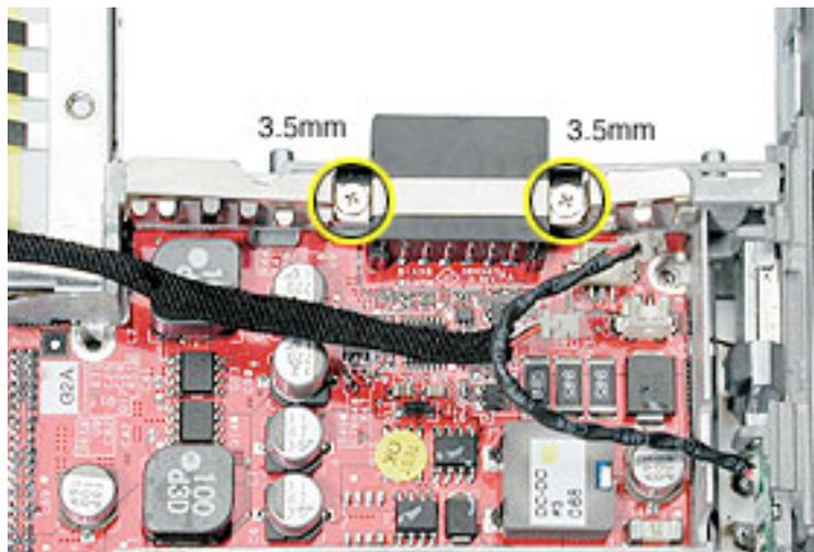
4. Lift off the EMI strip from the battery connector. Be sure to replace it when installing the replacement DC-to-DC board.
