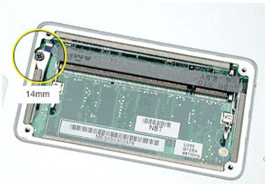
**Replacement Note:** Make sure you replace the screw and EMI shield so that the EMI shield is positioned with the finger-like projection pointing up.
