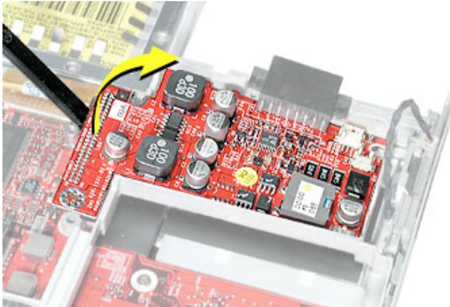
6. Install the replacement DC-to-DC board, and reassemble and test the computer.
