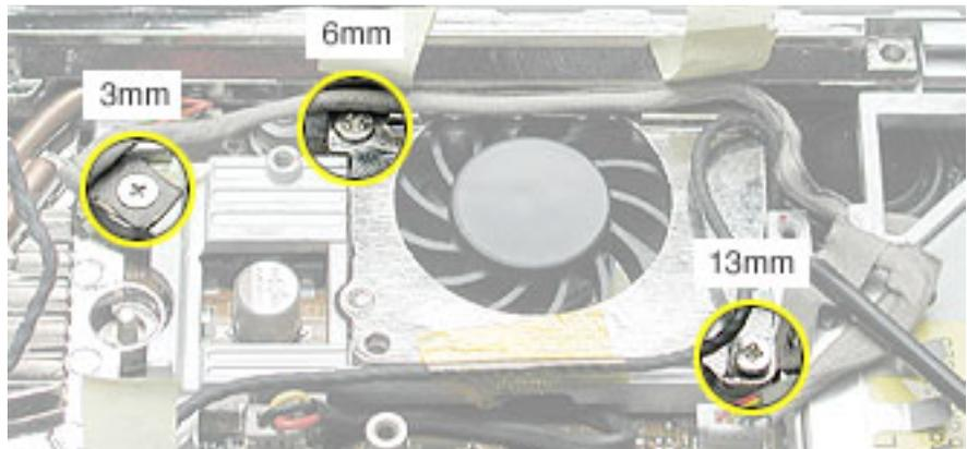
5. Peel up the yellow tape, and disconnect the inverter cable that runs along the top of the fan from the logic board.
