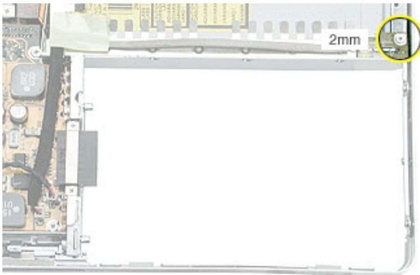
5. Install the replacement reed switch board and cable, and reassemble and test the computer.
