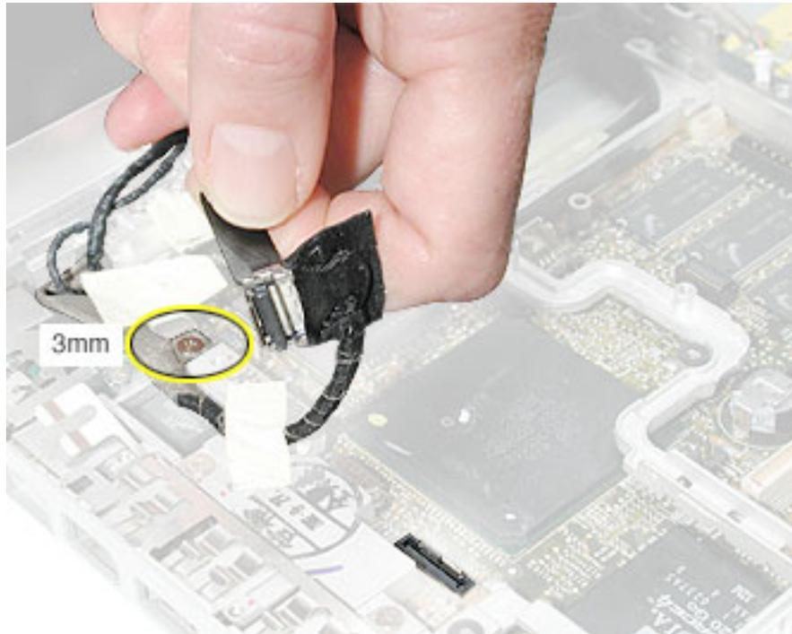
**Replacement Note:** When reinstalling the LVDS cable, tuck the pull tab under the frame.
