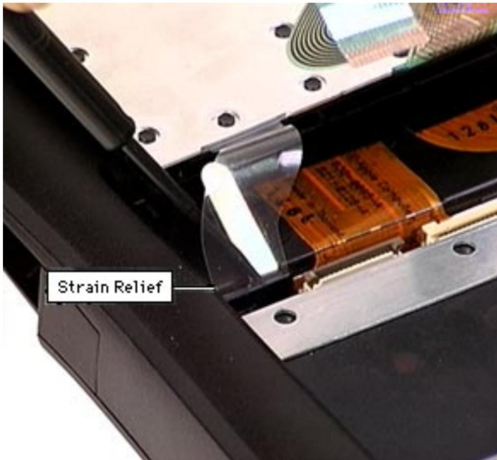
6 Use a nylon tool to bow the two strain relief cables outward, then pull the cables up to release them.
