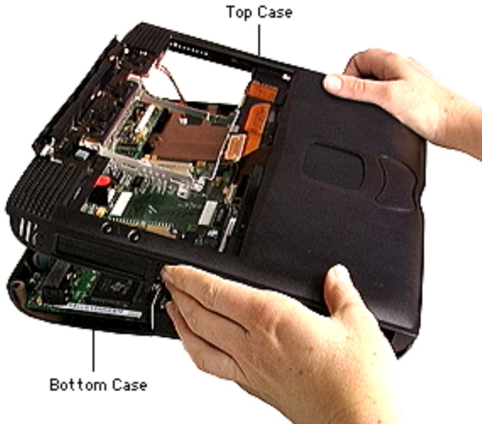
**Replacement Note:** To make sure the expansion bay flip door is aligned properly, push in on it when you replace the screw near the expansion bay flip door.
