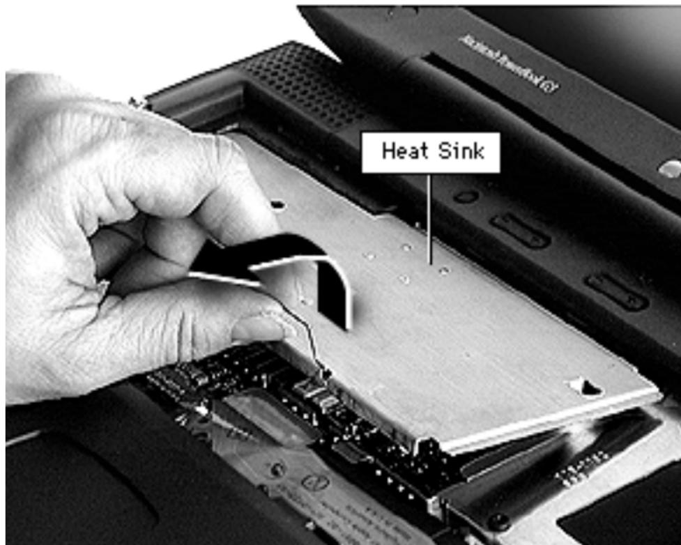
**Replacement Note:** Align the tabs to the slots before reseating the heat sink. If you have trouble fitting the tabs into the slots, press down on the clutch cover while pushing in on the heat sink. Ensure the heat sink is tightly secured.
