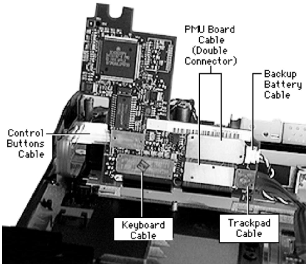
2 Lift the PMU board up and use a nylon tool or other flat-blade tool to disconnect the following cables:
