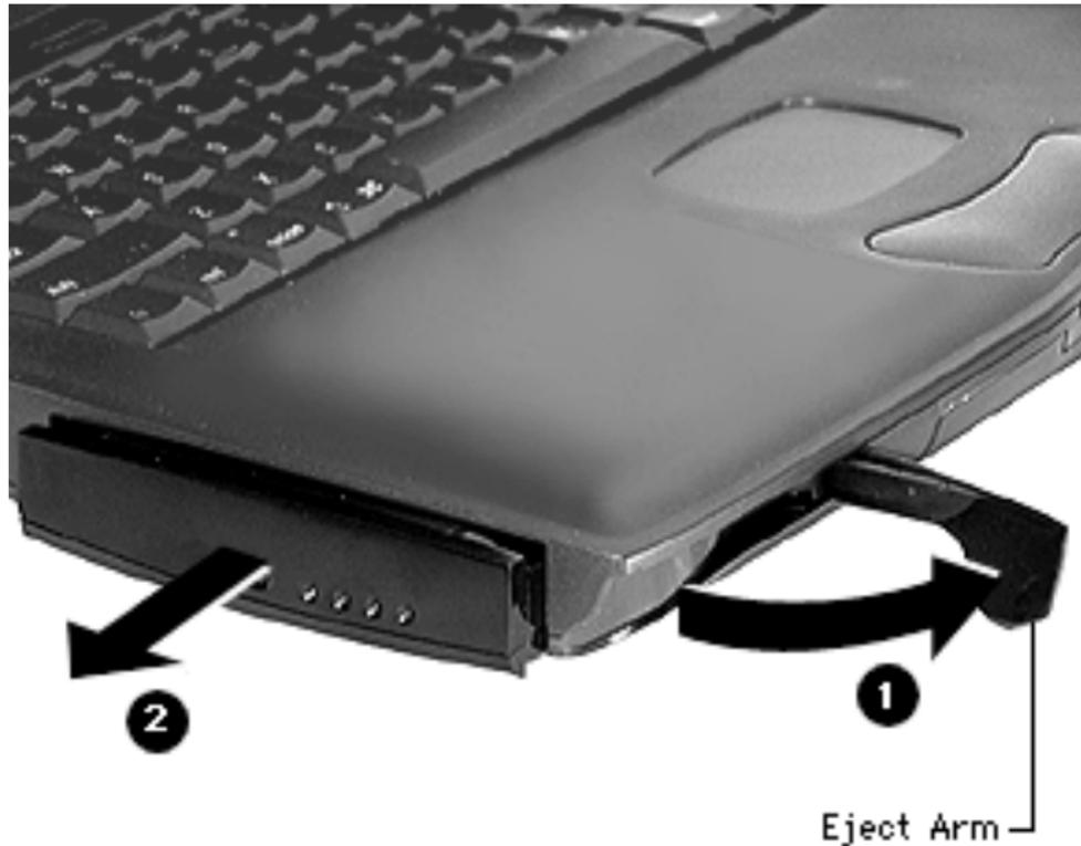
**Note:** If you do not wish to open the display all the way, open the display to a 90° angle. This will prevent the computer from tipping over when the expansion bay modules are removed.
