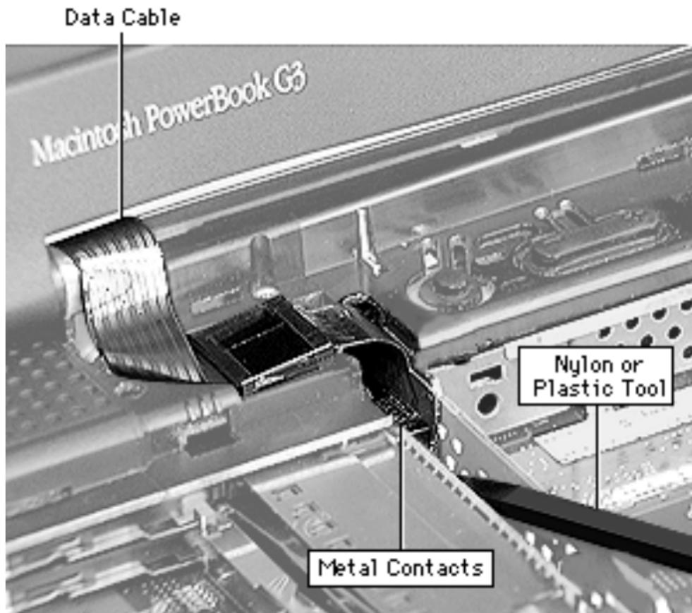
**Warning:** The cable connectors on the inverter cable and data cable have exposed metal contacts. Use only a non-metal tool to connect and disconnect these cables or you could short out the system.
