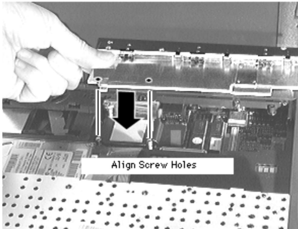
**Replacement Note:** Align the top left screw holes on the heatsink with those on the display shield. As you install the shield, be careful not to damage the fragile display cable wires.
