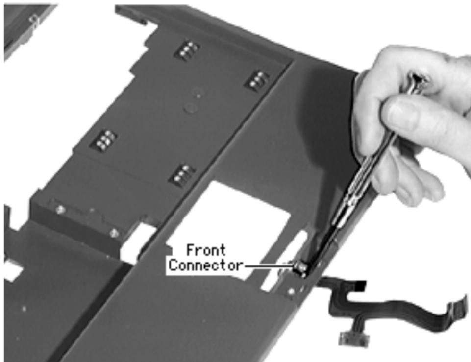
**Note:** The trackpad cable connector on the top case is secured by glue.
