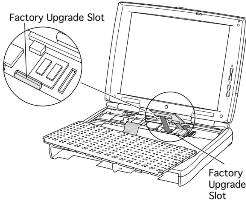
**Note:** An optional RAM card may be installed in the nearby factory upgrade slot.
