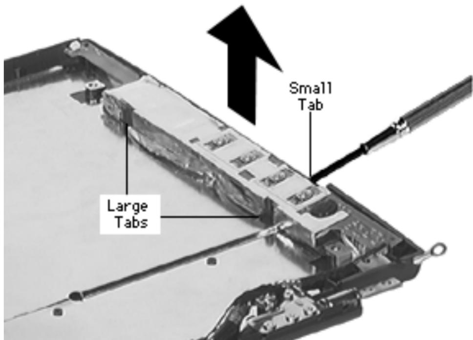
**Note:** The inverter board sits on 3 posts. It is secured by 2 large tabs and numerous small tabs
