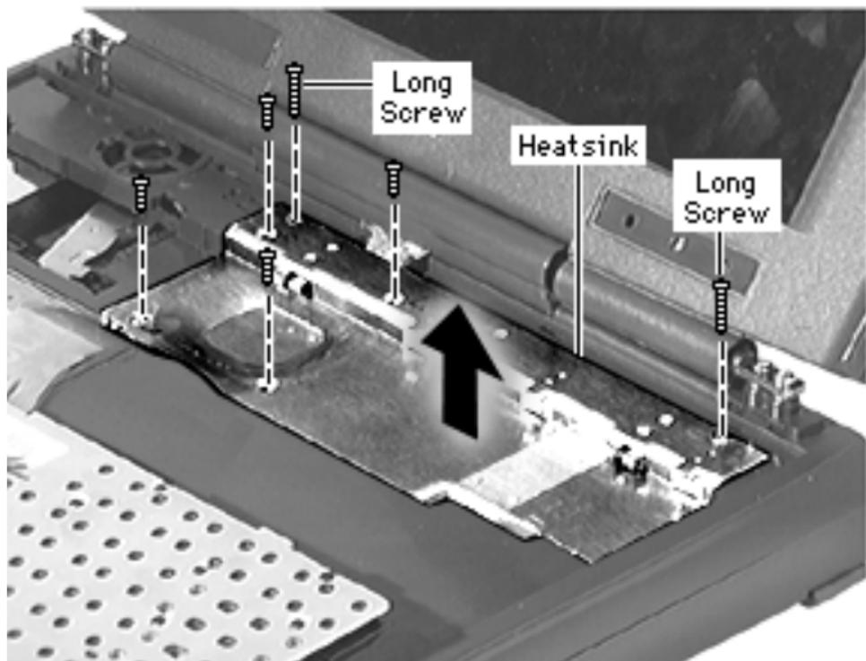
**Replacement Note:** Slide the heatsink's 2 depressed tabs under the top case and lower the heatsink into place.
