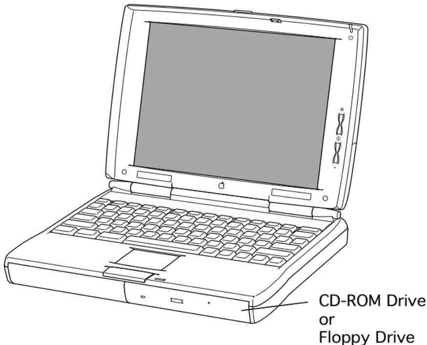
The PowerBook 1400 Series is the first PowerBook to support fully modular features. Customers can upgrade their floppy drive, CD-ROM drive, and expansion memory. Customers can also replace the removable panel on the top of the case with a clear or colored panel that came with the system.
