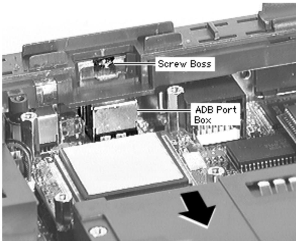
**Note:** The following step clears the top case from the logic board fence and releases each side latch.
