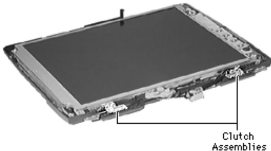
**Note:** Each clutch assembly consists of a clutch and clutch bracket. The left and right assemblies are not interchangeable.
