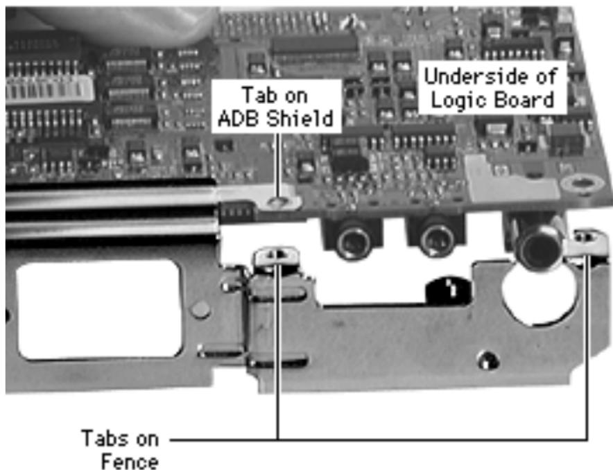
**Replacement Note:** Install the fence tabs **above the logic board**, not under the logic board. (Notice that the ADB EMI shield tabs are installed under the logic board.)
