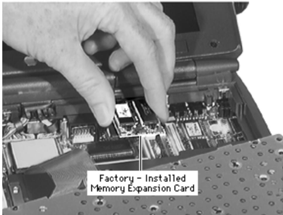
**Note:** To access any factory-installed memory expansion card, first remove the optional video expansion card. (Refer to the Upgrades chapter.)
