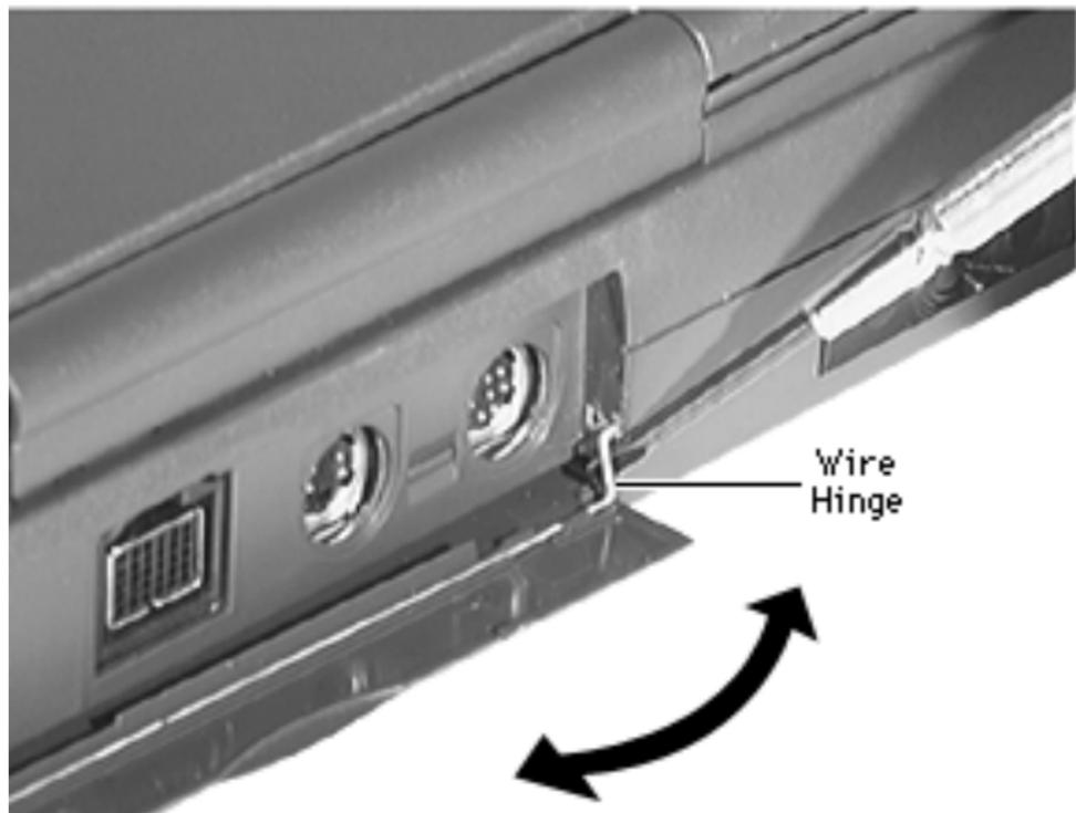
**Caution:** Remove the door carefully so you do not break the fragile tabs.
