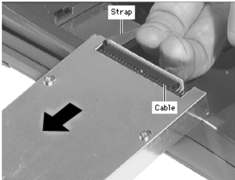
**Caution:** Pull the cable straight off to prevent damage to the pins. Handle the cable carefully; if the cable is damaged, you will need to remove the logic board in order to replace it. (See “Hard Drive Cable.”)
