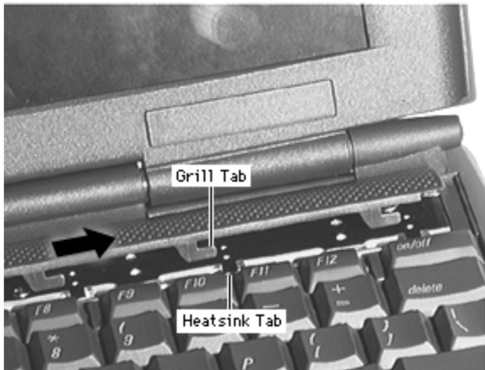
**Replacement Note:** With the downward tabs on the speaker grill slightly to the left of the heatsink tabs, slide the grill into place.
