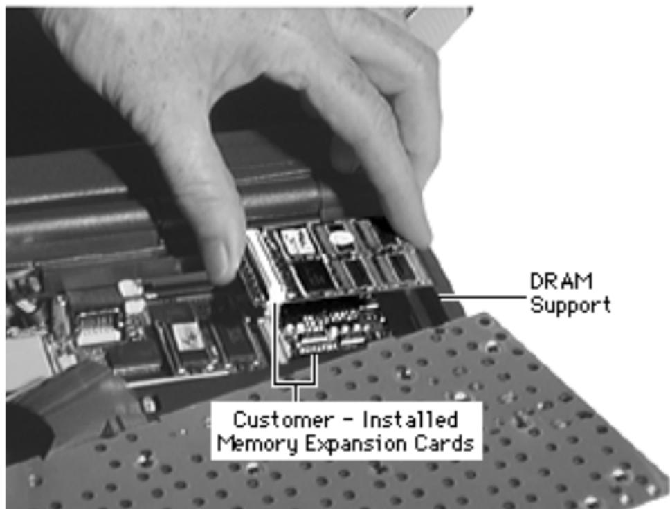
**Note:** The customer-installed memory card has connectors on the top and bottom, allowing a second card to be plugged in. The second RAM card is supported by a DRAM support on the top case.
