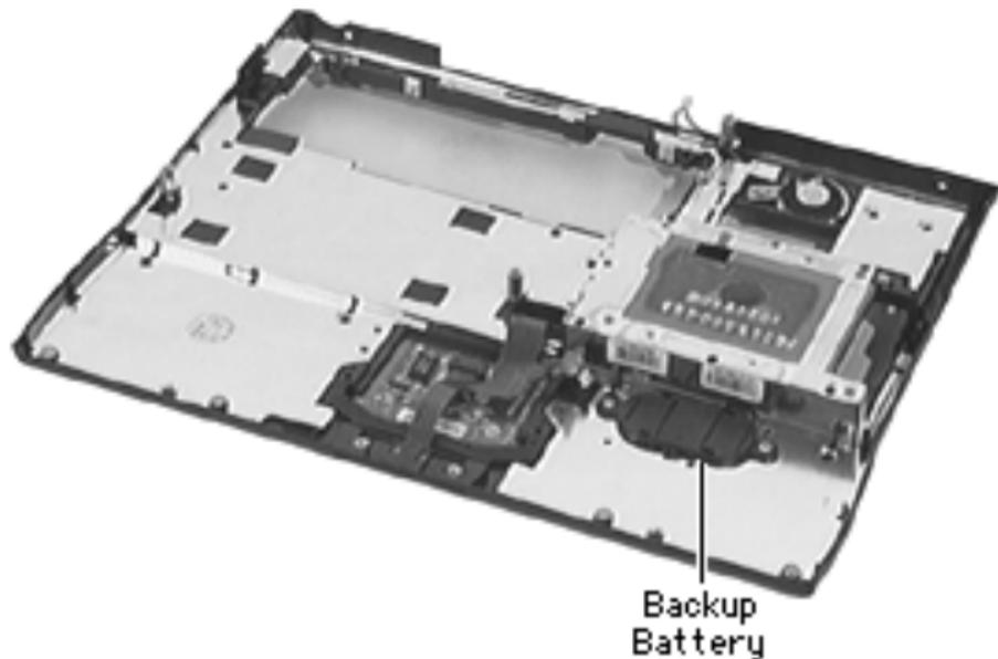
**Note:** For this procedure it is not necessary to remove the trackpad; just disconnect the trackpad cable from the backup battery.
