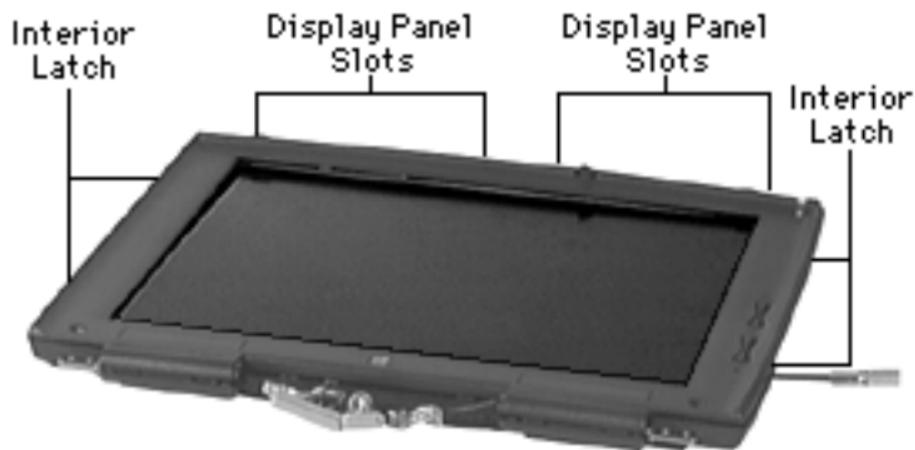
**Note:** The bezel is secured to the display housing by numerous latches, which must be disengaged.
