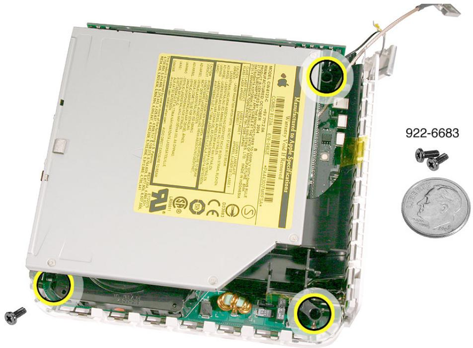
8. Lift the internal frame straight up.
