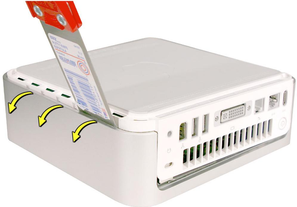
5. Be careful not to damage the EMI foam on the inside of the top cover.
