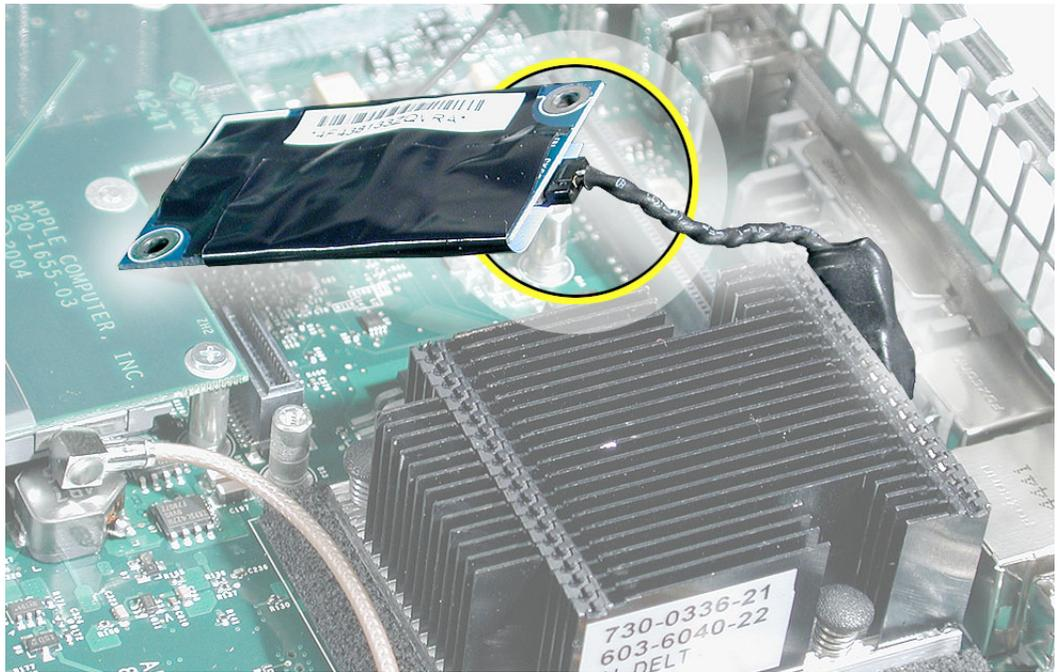
8. Connect the modem to the modem connector on the logic board, and install the two modem mounting screws.
