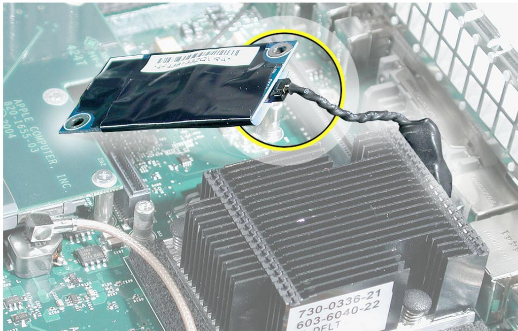
2. Using a jeweler's #0 Phillips screwdriver, replace the two modem screws.
