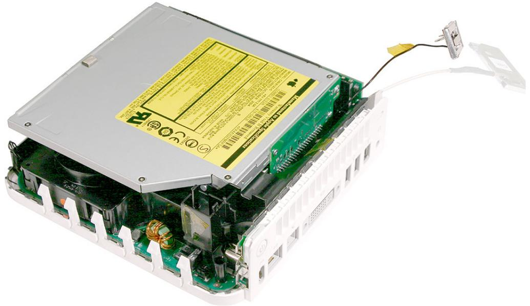
9. Free the power button cable from the kapton tape on the internal frame.
