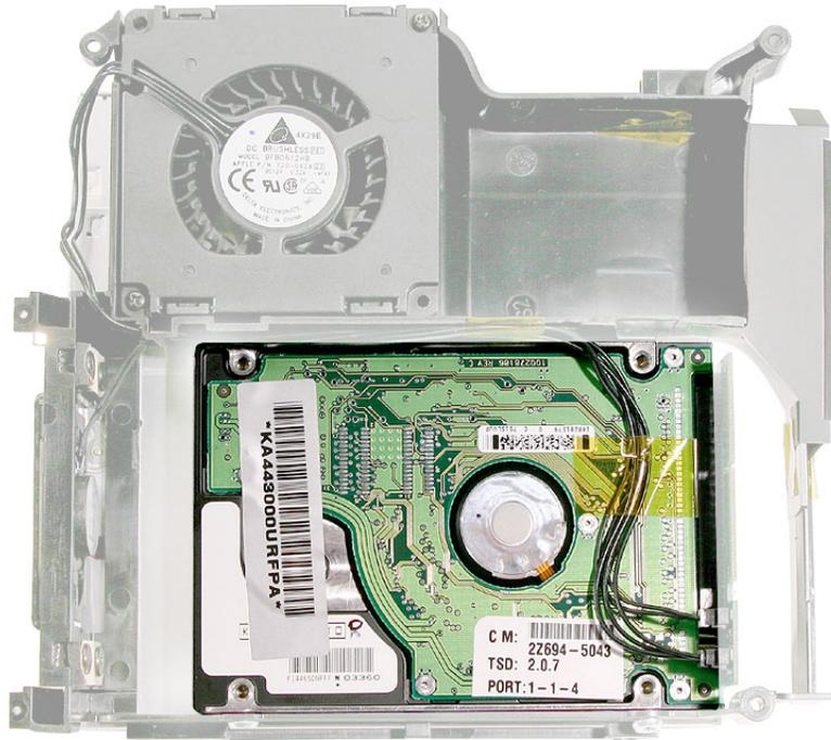
3. With a jeweler's #0 screwdriver remove the three fan screws.
