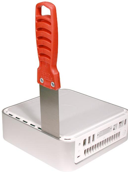
4. Gently release the internal latches by prying the tool away from the computer.
