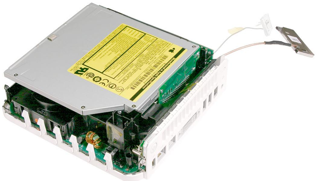
9. With a jeweler's # 0 Phillips screwdriver remove three screws on the internal frame.
