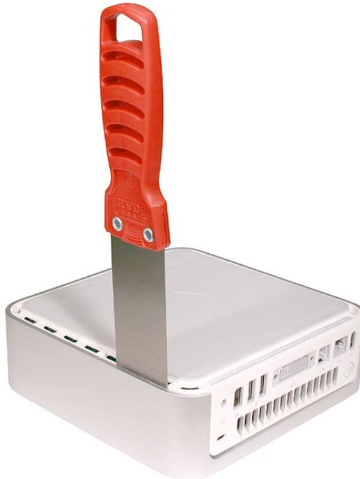
9. Gently release the internal latches by prying the tool away from the computer.
