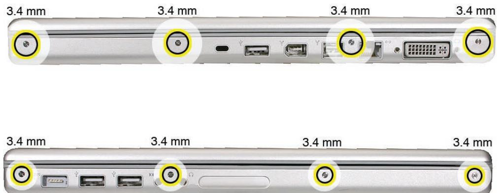
4. Remove the two screws from the back edge.
