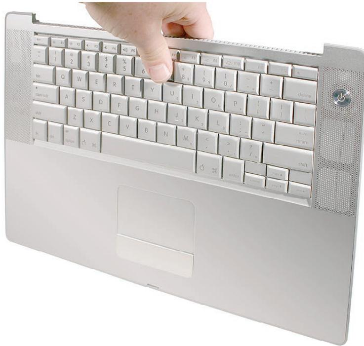
19. If needed, push through one of the top center keyboard screw holes, with the point of a black stick, to bow out the keyboard slightly.
