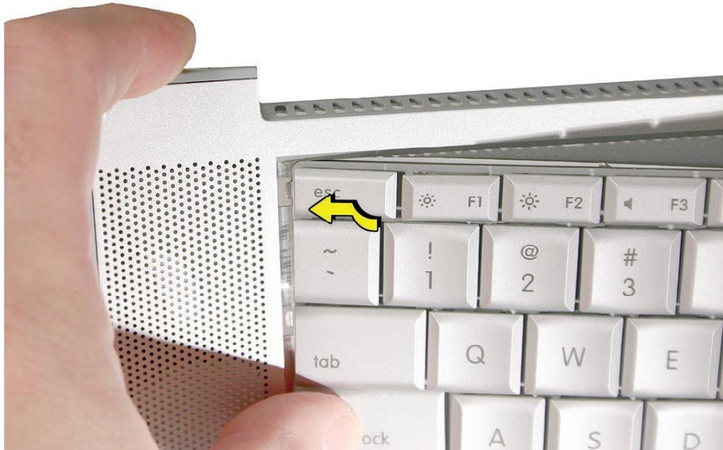
7. While supporting the keyboard in the top case, verify that the keyboard lays flat and that all the tabs have seated properly.
