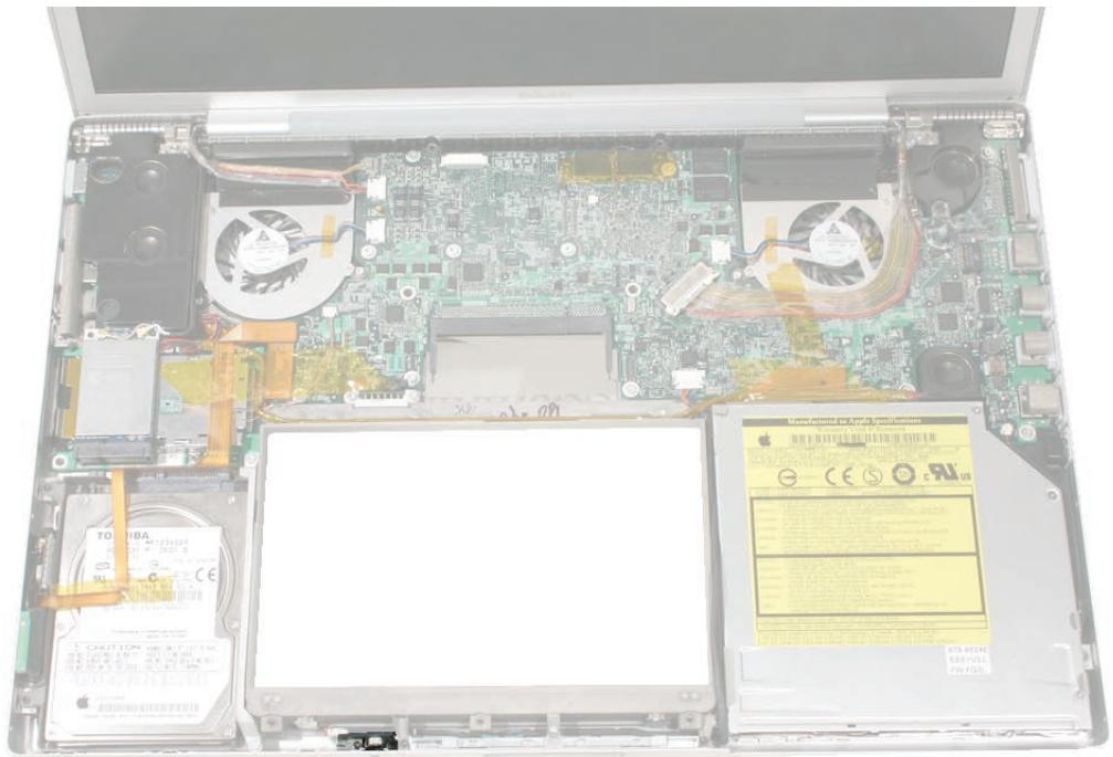
3. Disconnect the infrared board cable.
