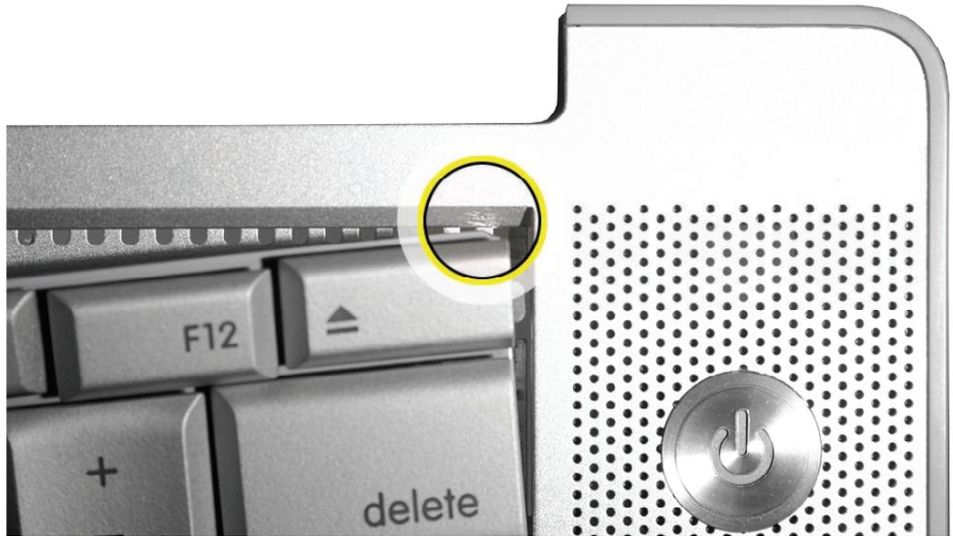
21. Use your finger to hold the bowed out keyboard. Continue to bow it out only enough for the tabs on one side of the keyboard to release cleanly. Repeat for the other side.
