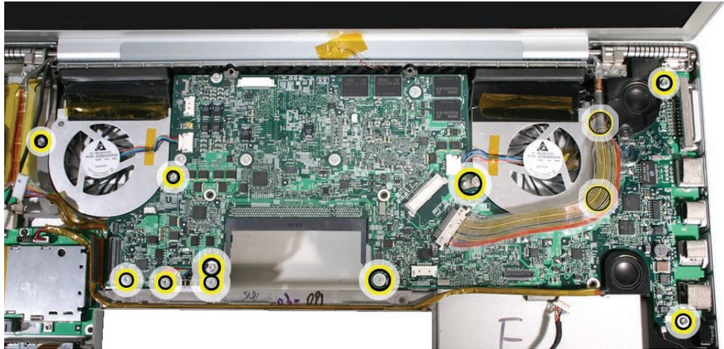
4. **Warning: Do NOT allow the logic board to flex at any time. Flexing the board can crack solder joints to components. Give special attention at the narrow neck of the fan cutout.**
