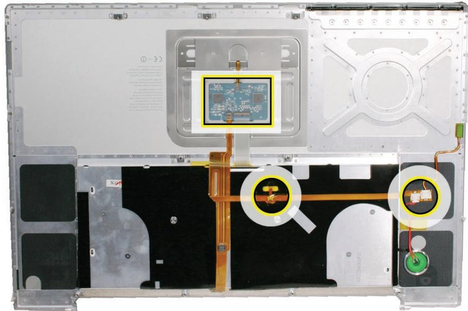
5. Check that the perimeter screw tabs and ribs are not bent.
