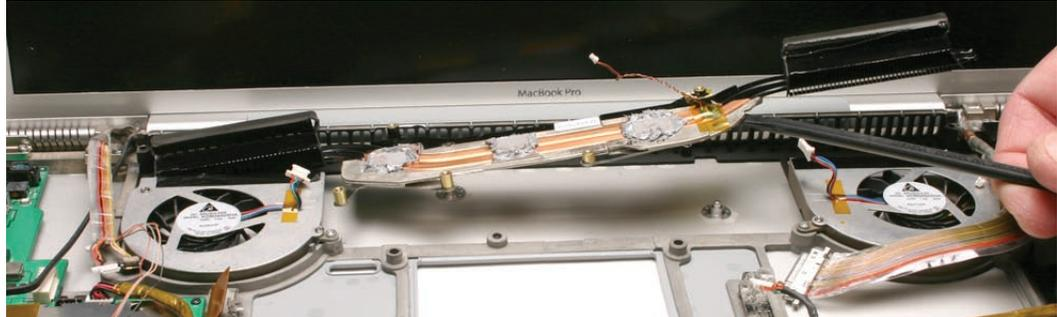
2. When installing the heatsink, make sure that it fits over the pins, shown, and lays flat.
