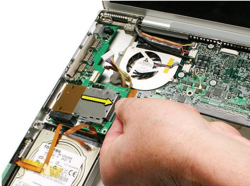
5. The ExpressCard cage assembly is attached to the left I/O board. Peel back the Mylar and remove the four screws.
