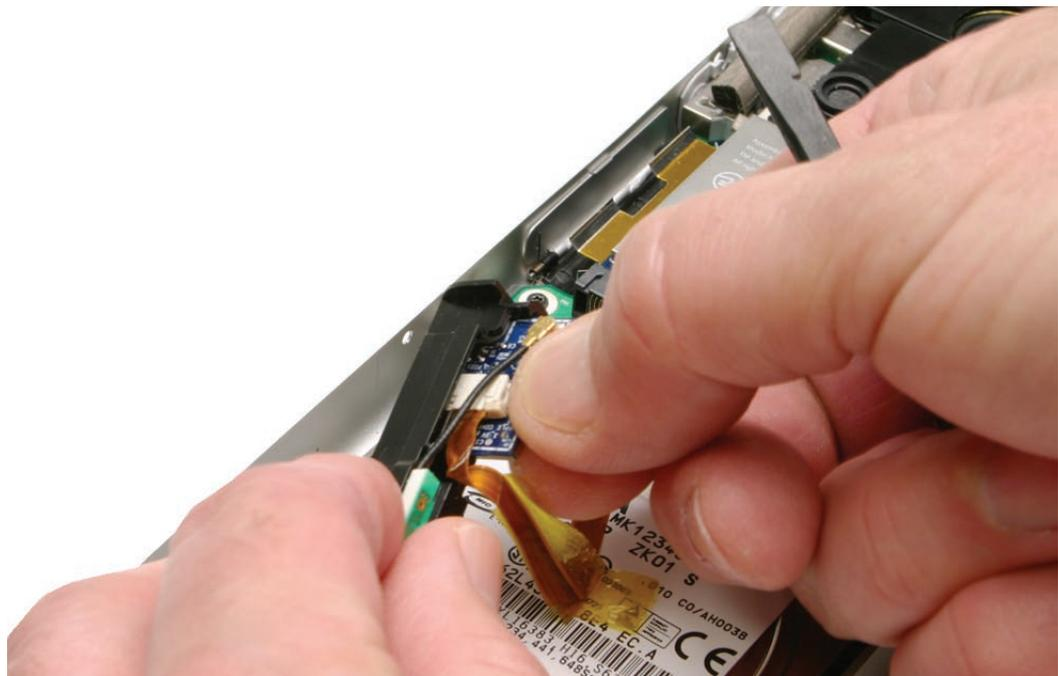
3. Lift the antenna cable connector straight off to disconnect.
