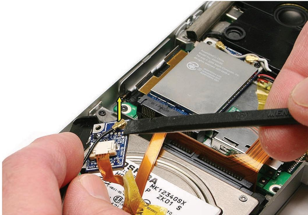
4. If replacing the bluetooth card, disconnect the flex cable by releasing the sliding lock.
