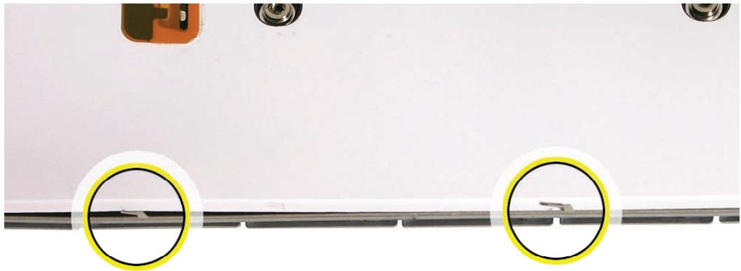
2. Guide the keyboard's flex cable through the slot in the top case, as shown. Make sure that it does not catch or bend behind the keyboard.
