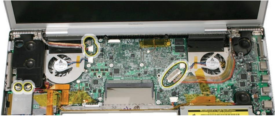
3. Remove the four clutch spring end cap screws, two each side.
