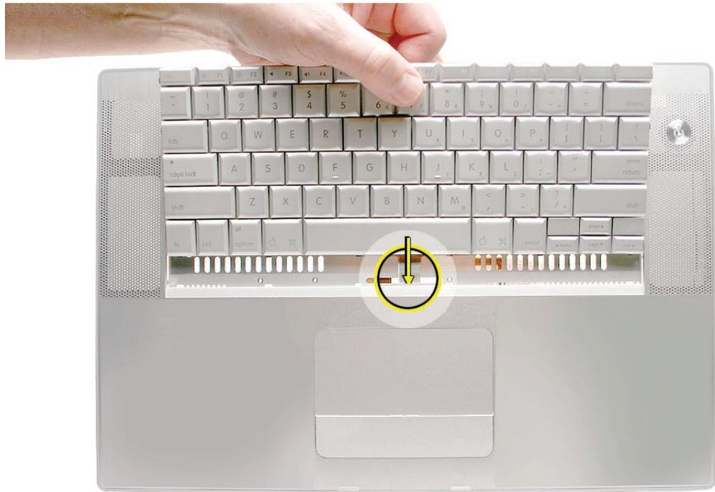
3. Verify that the small cable routes through the small slot, as shown.
