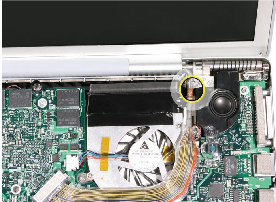
4. Verify that the EMI gasket is on the camera cable connector.
