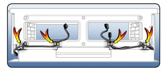
2 Release 4 latches on front fan and slide fan out of cage.
