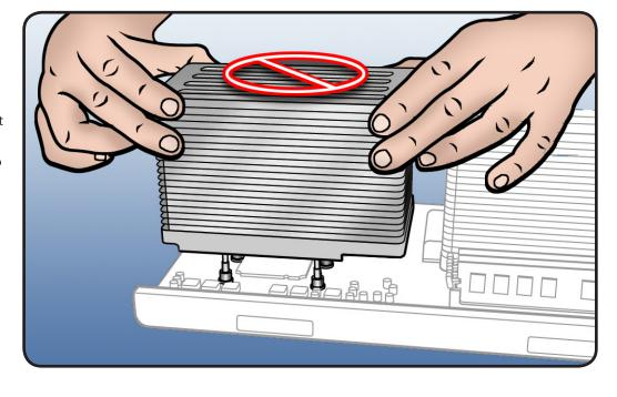
Important: CPU A heatsink (rear) and CPU B heatsink (front) are different parts; they can be identified by their undersides (see illustration). Be sure to install the correct heatsink on each processor.
