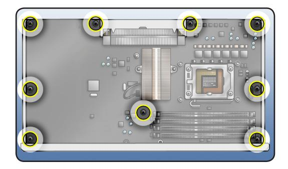
Reassembly Note: If you are installing new processor board, remove protective cap from new board's processor holder and transfer cap to original board's processor holder. Note that processor boards returned to Apple without protective caps may be rejected.
