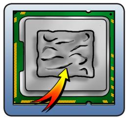
**2** Using syringe of thermal grease included with replacement part, apply narrow bead of grease to processor chip (raised square on top of processor). Apply in pattern illustrated, using approximately 0.2 cc.
