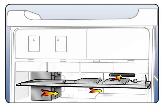
**5** Replace PCI bracket and tighten captive screws.
