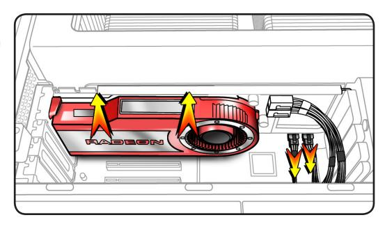
If you are replacing booster cable(s) with new one(s), disconnect cable(s) from card.
