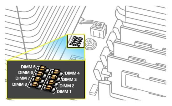
To diagnose memory issues, start up the computer and check the diagnostic memory LEDs. An illuminated, red LED indicates its associated DIMM may be poorly seated or failed.
