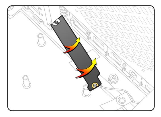
2 Replace antenna board mounting screw.
