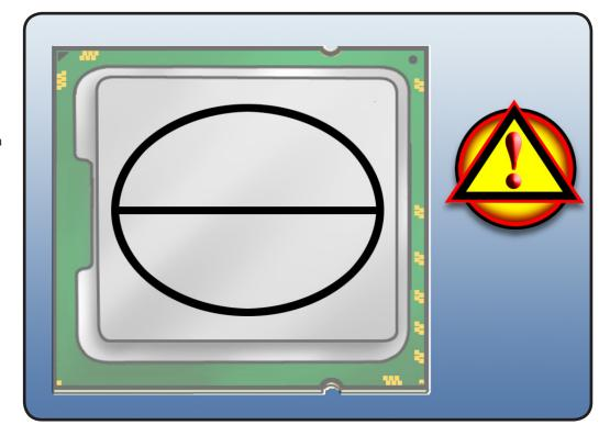
Align processor notches with tabs on processor holder, as shown. Then lower processor straight down onto connector.
