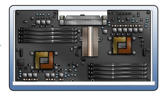
Important: Every time you remove a processor heatsink, you must replace the thermal grease on the processor below it. See "Processor Heatsink, 8 Core."
