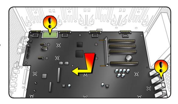
Note: If you are replacing backplane board with a new board, transfer back ports EMI shield from original board to replacement board. Also transfer PCI cards and AirPort card (if installed). You do not need to transfer Bluetooth card to new board; it comes with Bluetooth card already installed.
