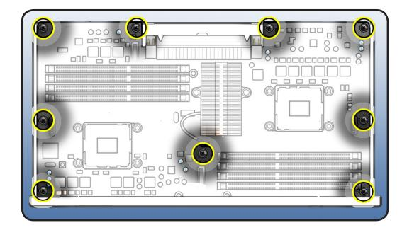
Reassembly Note: If you are installing new processor board, remove protective caps from new board's processor connectors and transfer caps to original board's connectors. Note that processor boards returned to Apple without protective caps may be rejected.
