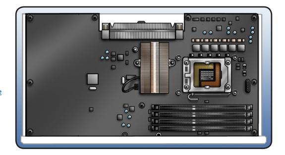
Important: Every time you remove a processor heatsink, you must replace the thermal grease on the processor below it. See "Processor Heatsink, Quad Core."
