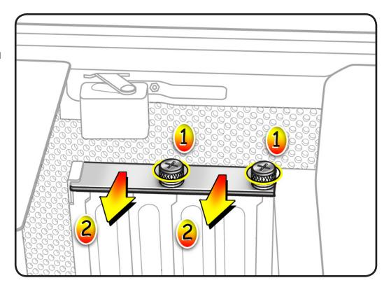
Reassembly Note: Slide bracket under circled tab before securing screws.
