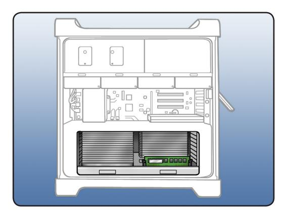
Note: Processor tray includes processor heatsink(s), processor(s), DIMMs, processor board, and processor tray support plate.
