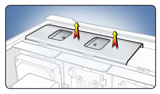
Disconnect optical drive cable from drive(s) and remove carrier.
