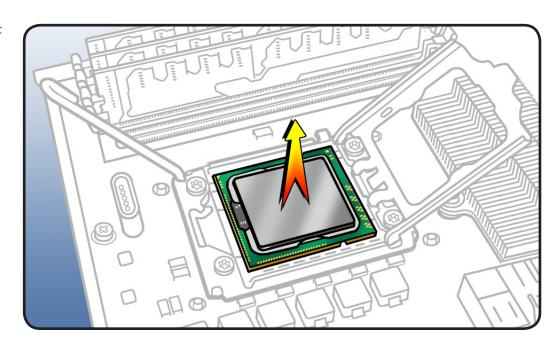
**Important:** Do not touch components on processor top or bottom. Hold processor only by the edges.
