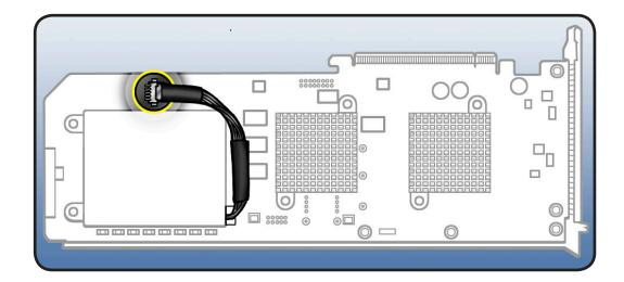
Remove 3 screws and lift battery from card.
