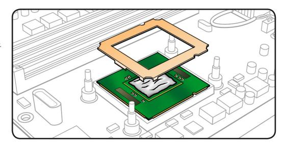
Important: Do not touch components on processor top or bottom. Hold processor only by the edges.
