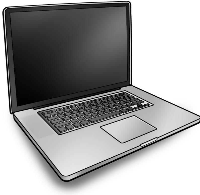
The MacBook Pro (17-inch, Early 2009) computer features both the NVIDIA GeForce 9400M integrated graphics processor and a high-performance NVIDIA 9600M GT graphics processor, Multi-Touch trackpad, and aluminum body. Refer to more features below.
