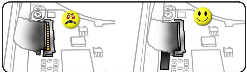
**Replacement Caution:** To prevent no video or a short to the logic board, be sure to place EMI gasket on camera cable—positioned precisely where shown—**after** cable is fully connected to logic board and shim is in place.
