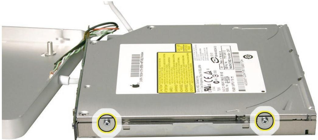
13. Lift the top of the drive enclosure, pivoting the right edge up while sliding it sideways left and downward to disengage the left edge.
