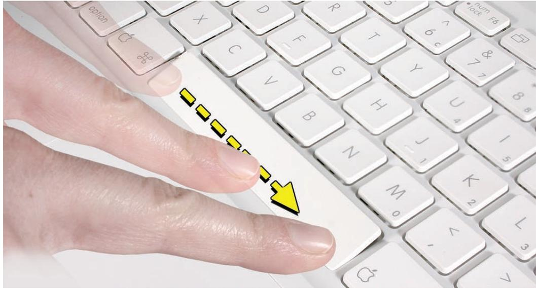
13. Press along the top of the Space bar to secure it to the top stabilizer bar. (Listen for the keycap clicking into place.)
