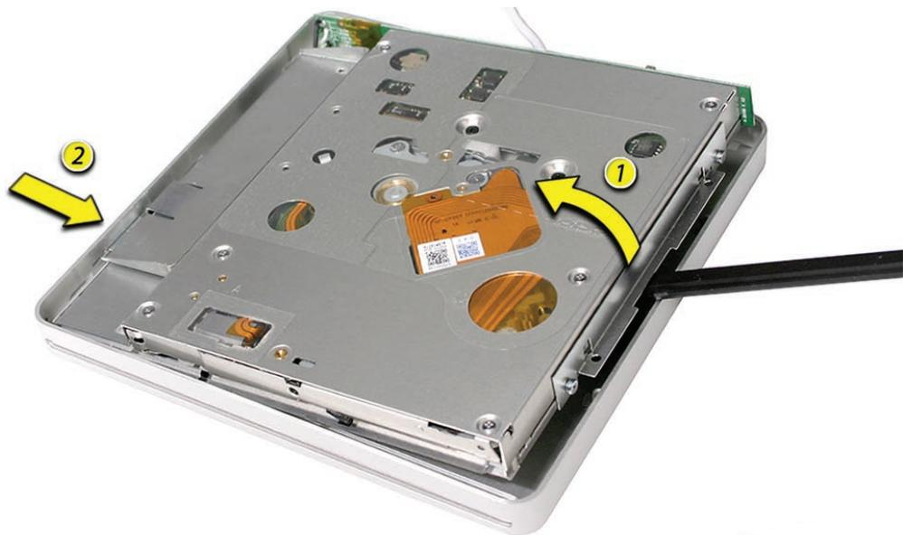
7. Locate the controller board and cable leading to the external USB cable (see inset below). Since the cable remains connected during this procedure, be careful not to pull or stress the cable connections. Always keep the controller board within an inch or so of the outer case.
