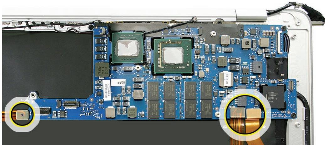
**Very Important:** Before installing a new thermal module or reinstalling the original one, you must clean the old thermal paste from the chips on the logic board, then reapply paste or utilize new paste on the replacement thermal module. See **How to Replace the Thermal Paste** section of the Thermal Module section preceding this one.
