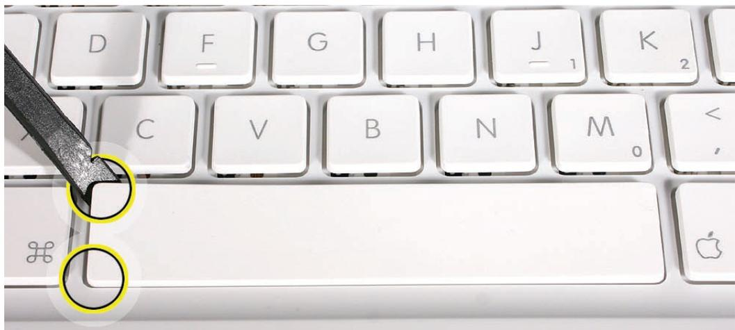
2. Because adhesive is used under the top case, closely inspect the case for any adhesive that may have built up under the keycap. Lift away any built-up adhesive using fine-point tweezers.
