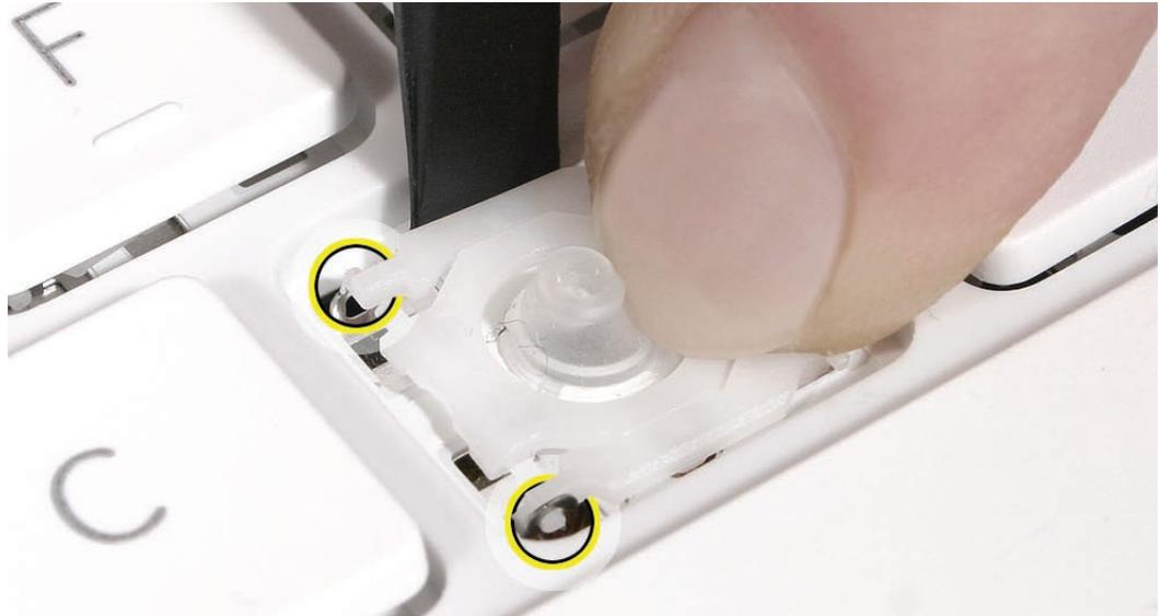
8. With the scissor pins inserted, use a black stick to raise and lower the scissor mechanism to make sure it moves freely.
