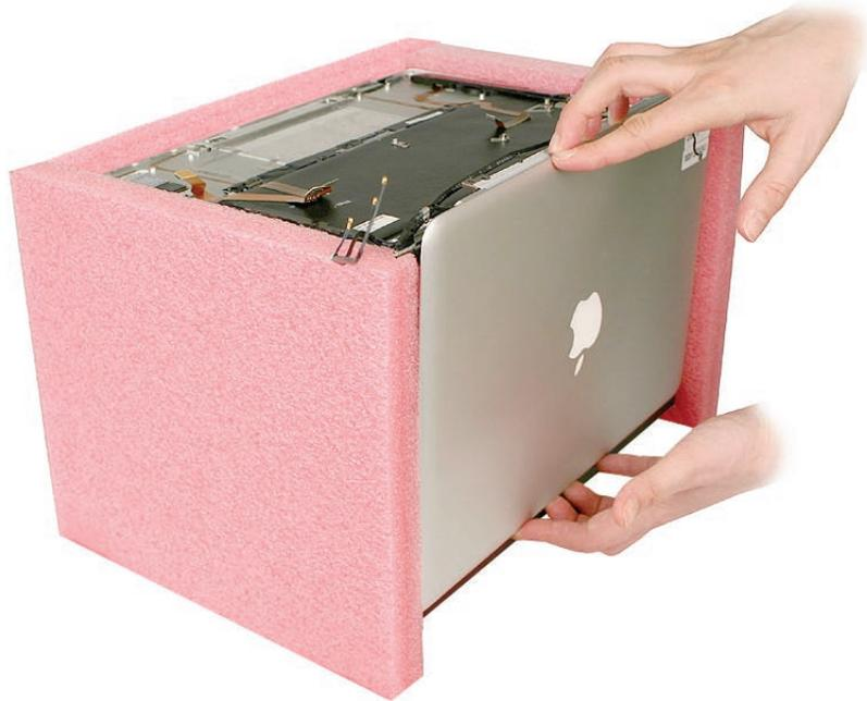
2. If necessary, slide the antenna assembly a millimeter or two to the left or right to fully align the holes.
