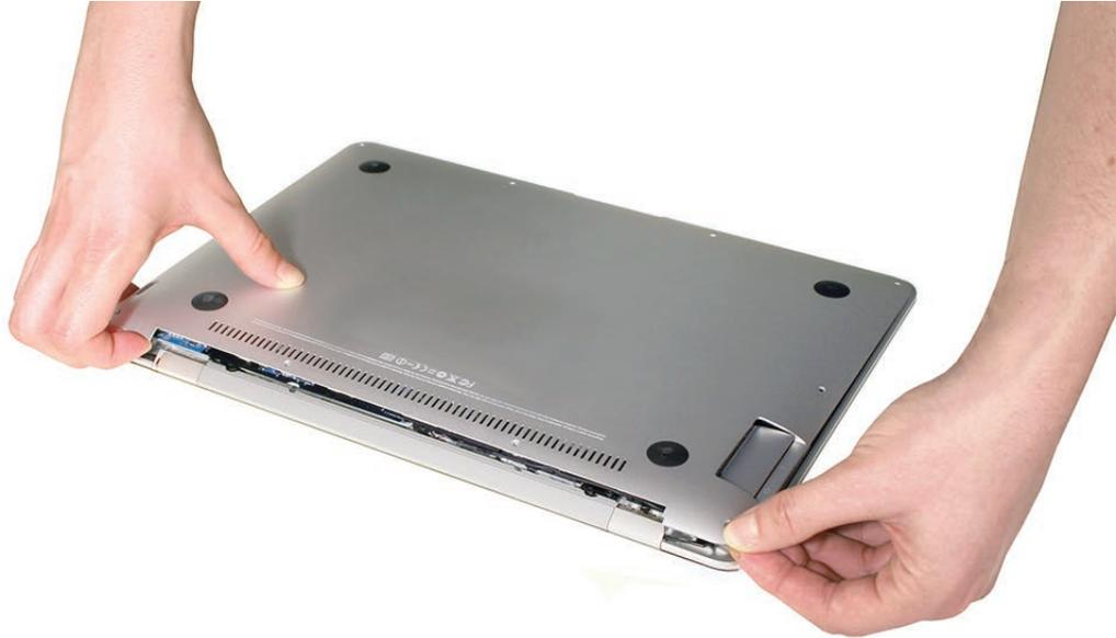
3. Pivot the rear edge upward a few inches to a 30° angle. At that same angle, pull the bottom case outward from the front edge of the top case to preserve the integrity of the front clips.
