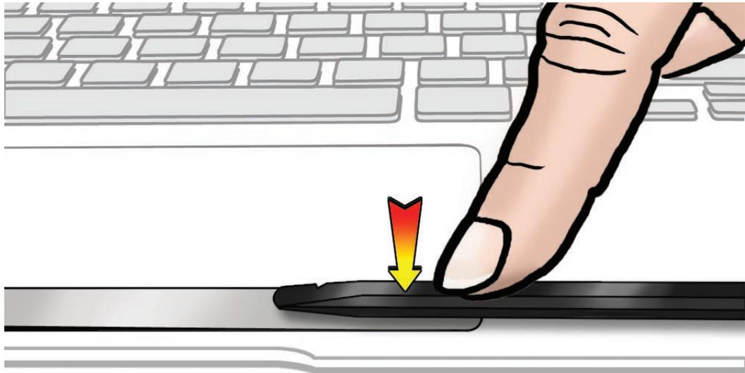
4. If any of the above steps do not register a click, follow instructions below to install a shim into the channel on the underside of the trackpad button.
