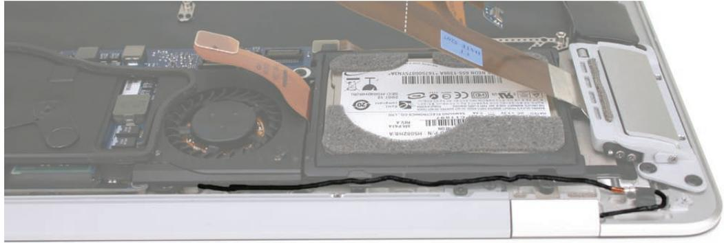
**Note:** Notice two black plastic cosmetic pieces designed to prevent screws and cabling from being visible through vent holes in the bottom case—one molded to fit the edge of the fan and a smaller piece molded to fit the hard drive frame. You will remove them in this procedure.
