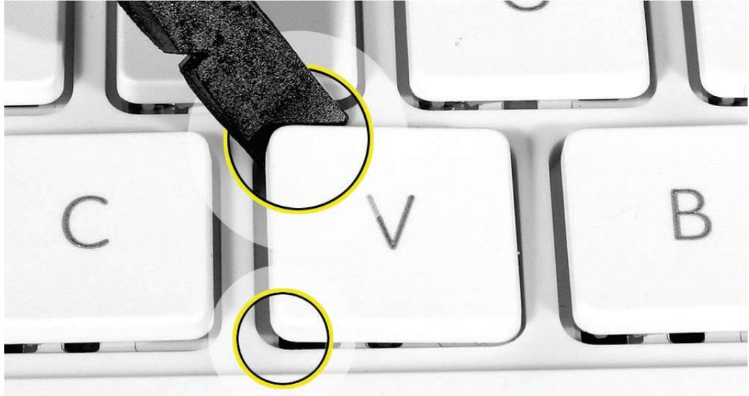
2. Because adhesive is used under the top case, closely inspect the case for any adhesive that may have built up under the keycap. Lift away any built-up adhesive using a black stick or fine-point tweezers.
