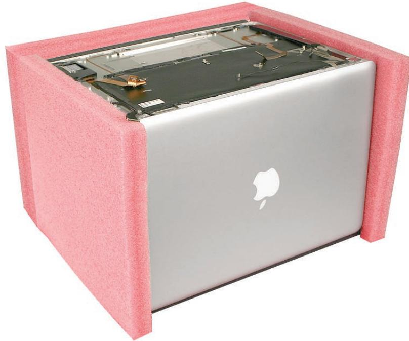
2. Carefully lift the AirPort/Bluetooth antenna cable from the top case, pulling up slowly from the display side to the AirPort/Bluetooth card side to preserve the adhesive.
