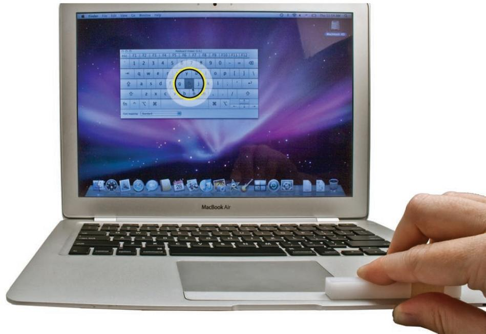
8. Place computer on a flat surface in standard operating position and test the trackpad button feel and functionality with both the flat plastic tool and your thumb.
