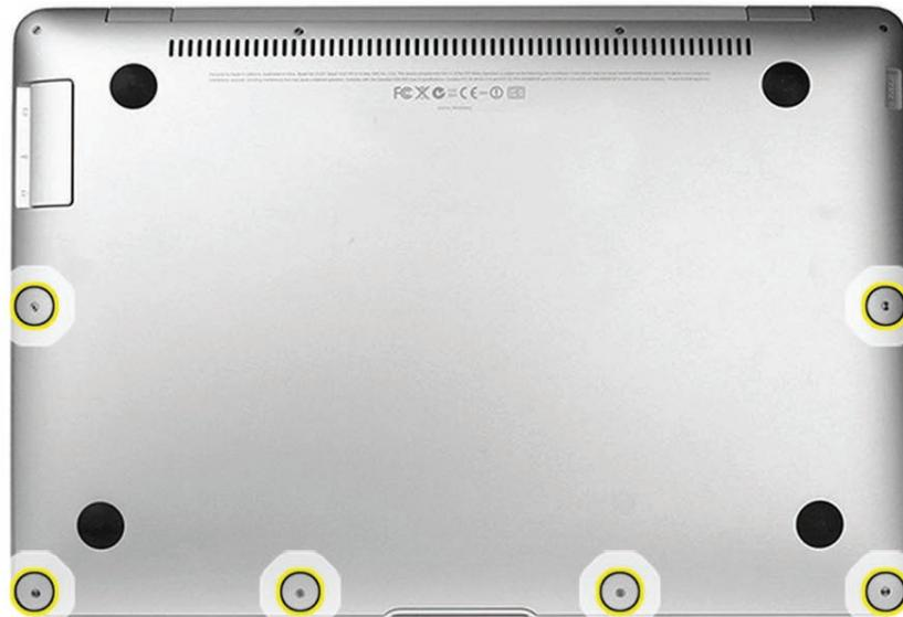
2. When reinstalling the new shoulder screws, make sure the head of the screw sits flush with the bottom case after installation.
