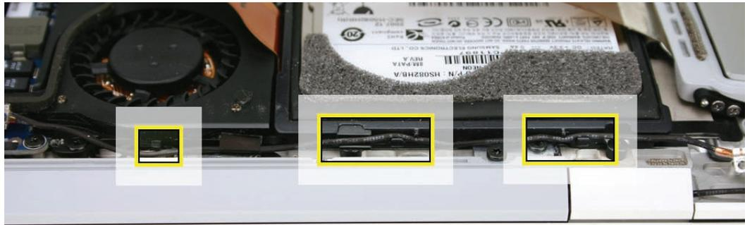
13. Carefully extract the microphone cable from the routing clips on the hard drive frame. Because it is delicate, take great care not to pinch or pull this cable.
