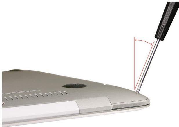
2. Insert ten #000 Phillips screws in the following order, paying close attention to the angle. If a particular screw does not seem to mate easily with its screw boss, set that screw aside and try another of the same size. It should take little effort to screw it in.
