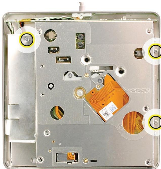
5. Note the tab on the lower left of the drive casing which fits into a recessed slit in the outer enclosure (shown in left blowout area below.) Then, on the opposite side of the drive, look for the indentation in the center of the right edge of the drive (highlighted below on right).
