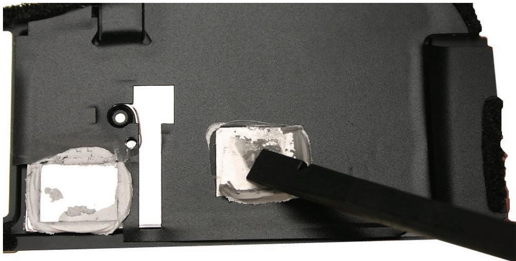
3. Use an alcohol wipe to completely clean the residual thermal paste from the two chips on the logic board and the two pads on the heatsink.
