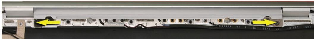
3. Install four identical Torx T6 clutch screws first, and then install the remaining 13 identical Phillips screws.
