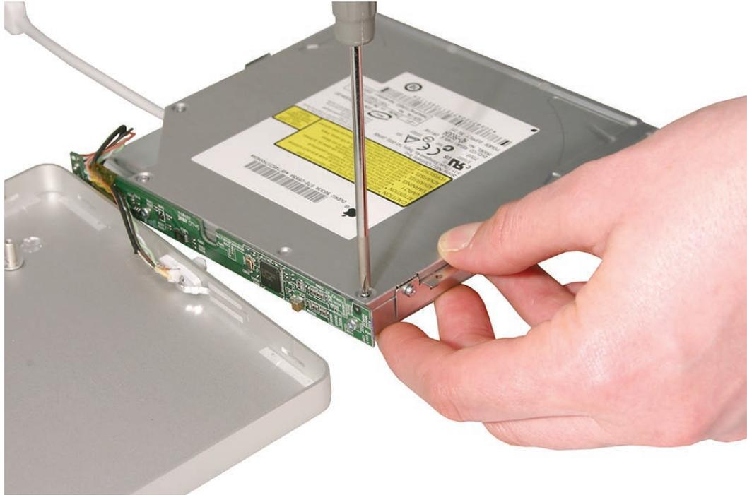
11. Remove the four small Phillips screws shown below from the top of the drive.
