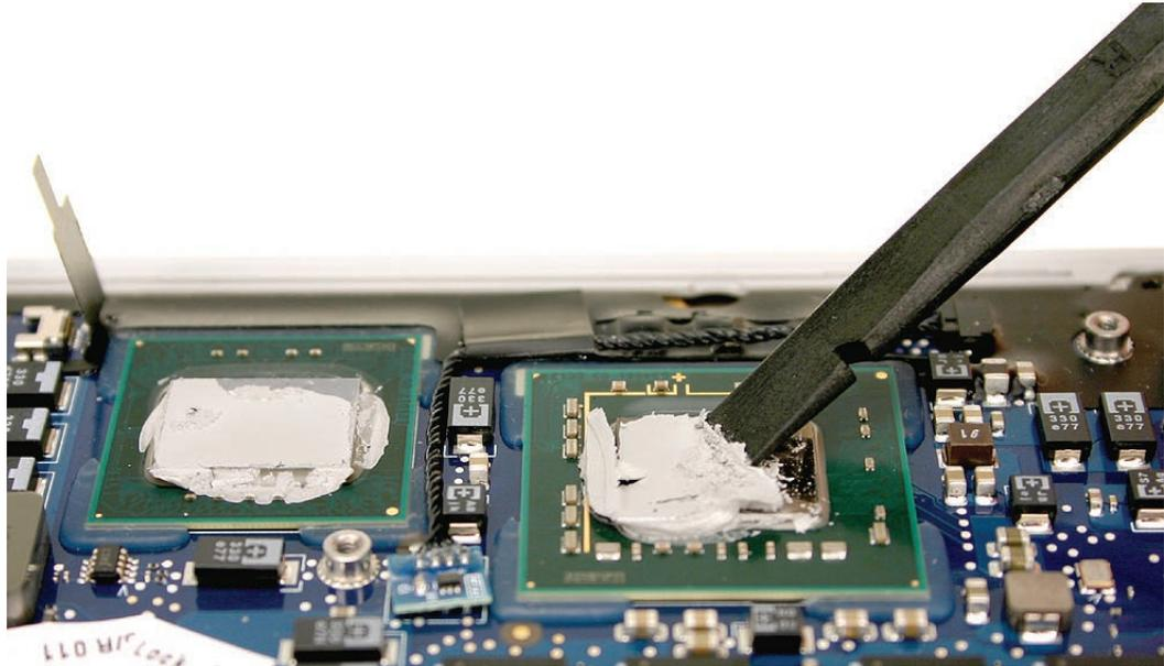
2. Use a black stick to remove thermal paste from the two mating pads on the under side of the thermal module.
