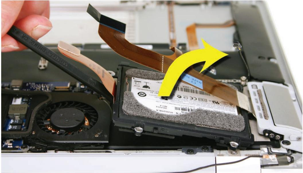
18. Remove the hard drive assembly at an angle, out from under the port hatch assembly flex cable, taking care not to bend or strain the cable.
