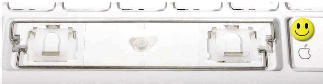
10. Determine which is the top of the Space bar keycap by checking the clips on the inner plane. The top of the keycap has the row of clips that extend closest to the sides of the keycap. These top clips most closely match the longest stabilizer bar at the top of the keycap well.
