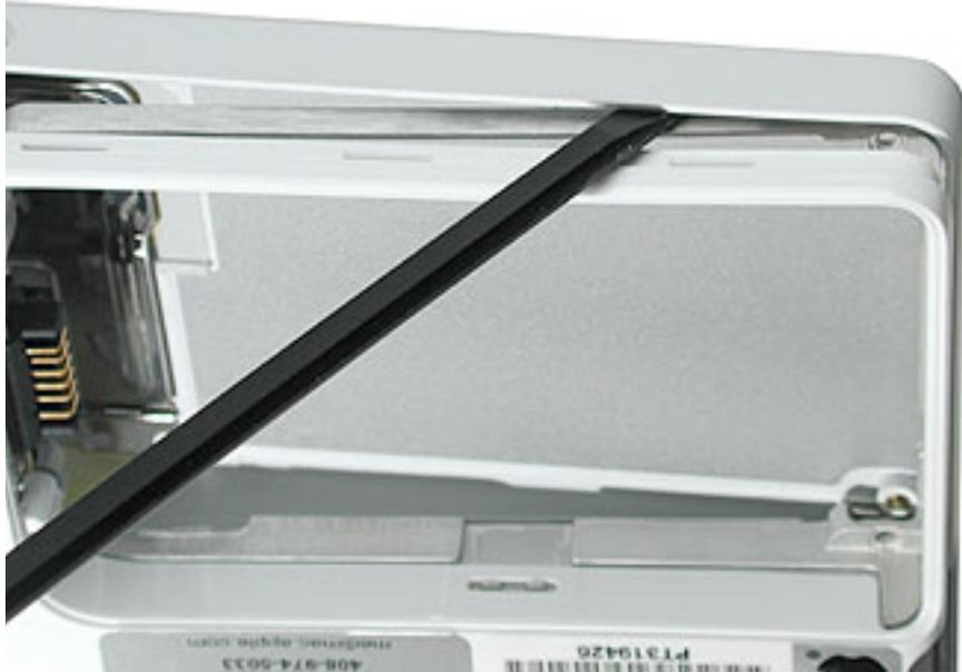
12. With most of the top case loosened, tilt up the corner of the top case that fits over the DC connector.
