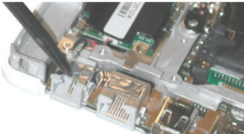
3. Lift up the modem sleeve and disconnect the RJ11 modem cable from the modem board.
