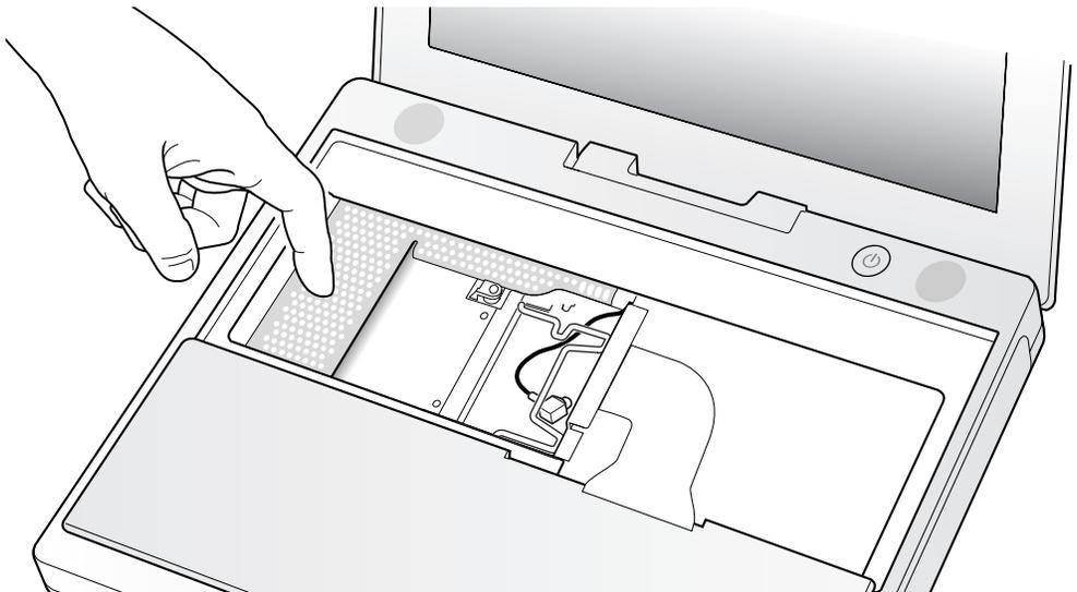
2. Unlatch the flexible wire holder that secures the card.
