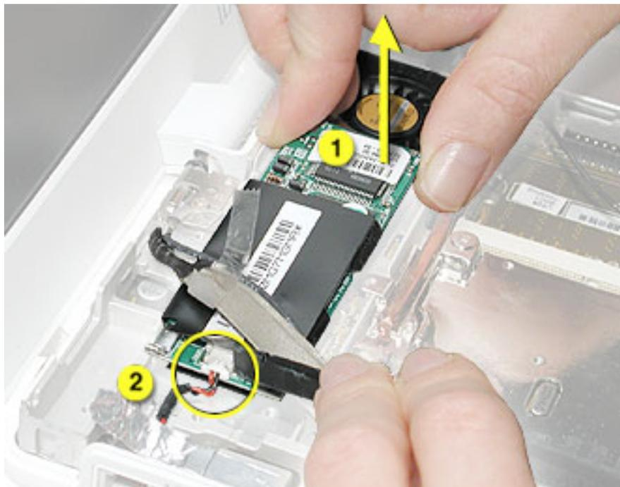
5. Install the replacement modem, and reassemble and test the computer.
