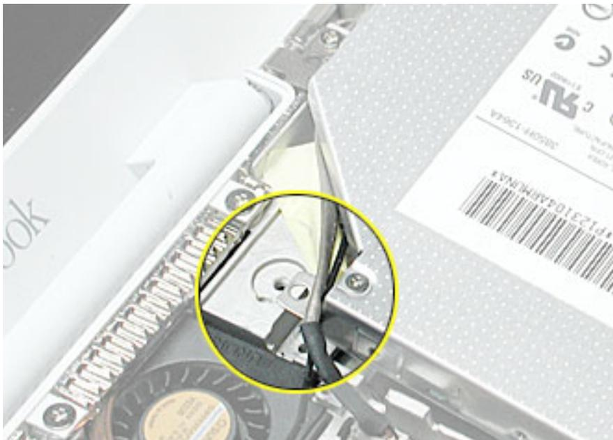
5. Remove the two screws holding the cable bracket to the optical drive.
