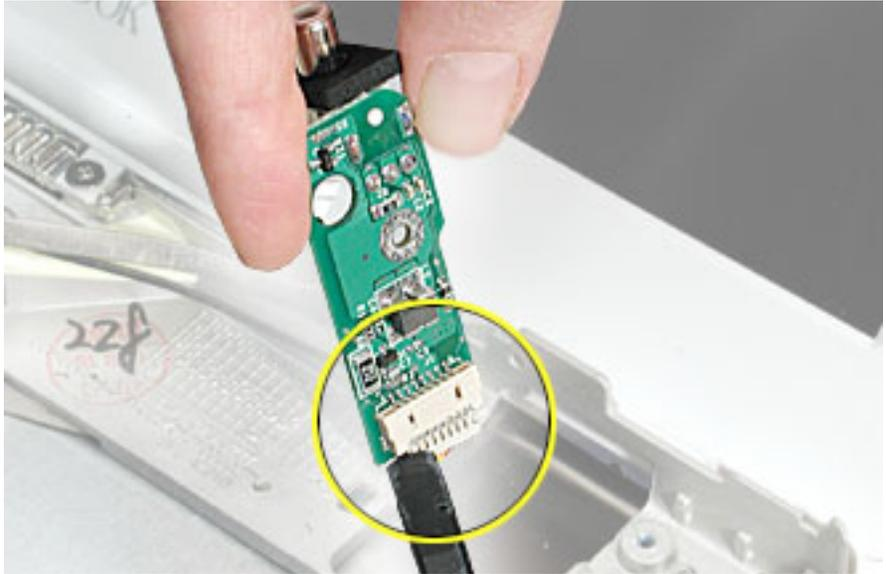
3. Remove the DC board from the computer assembly.
