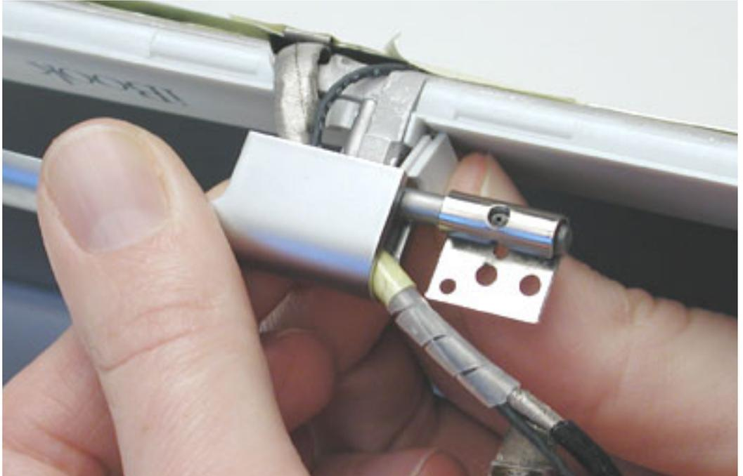
Make sure the clutch cap on each side of the clutch cover is firmly seated before installing the two screws.
