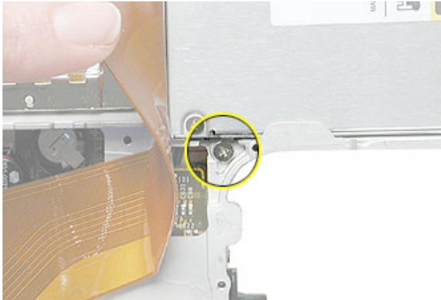
4. **Warning: Handle the optical drive at the sides only. Do not touch or press anywhere else on the drive.**
