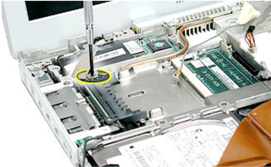
4. Peel the tape off of the optical drive, and disconnect the flat backlight cable from the logic board.
