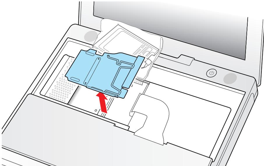
11. Locate the keyboard cable connector.
