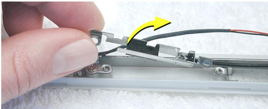
10. Unwrap the tape that secures the AirPort Card antenna to the cable bundle.
