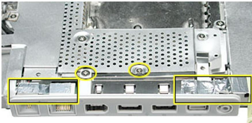
2. Tilt down the I/O bezel and remove it from the computer frame.
