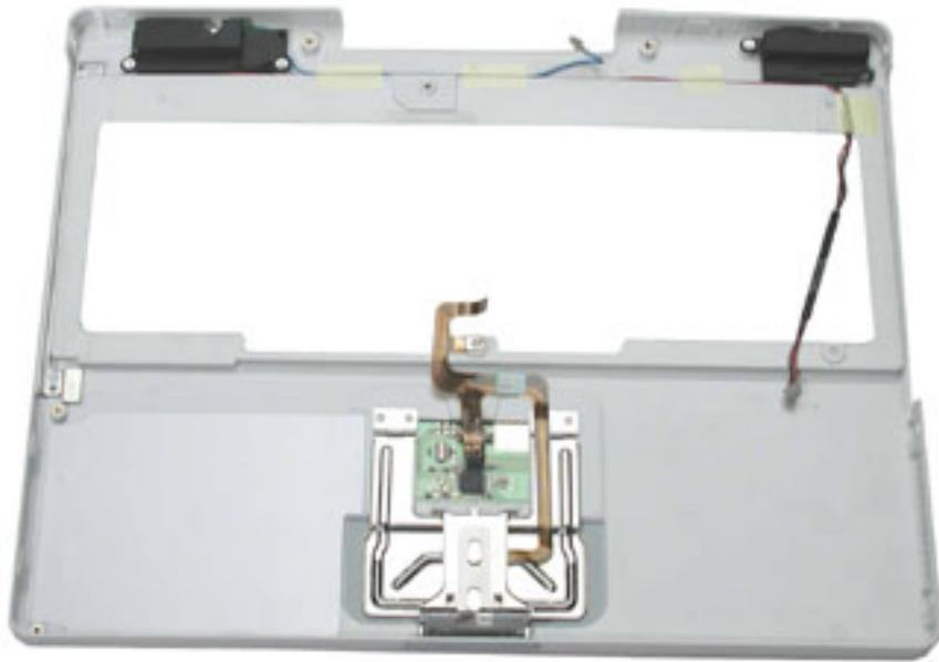
19. Install the replacement top case, and reassemble and test the computer.
