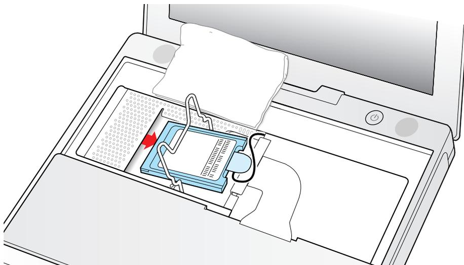
8. If an AirPort Card is not installed, unlatch the flexible wire holder to release the AirPort Card antenna cable.
