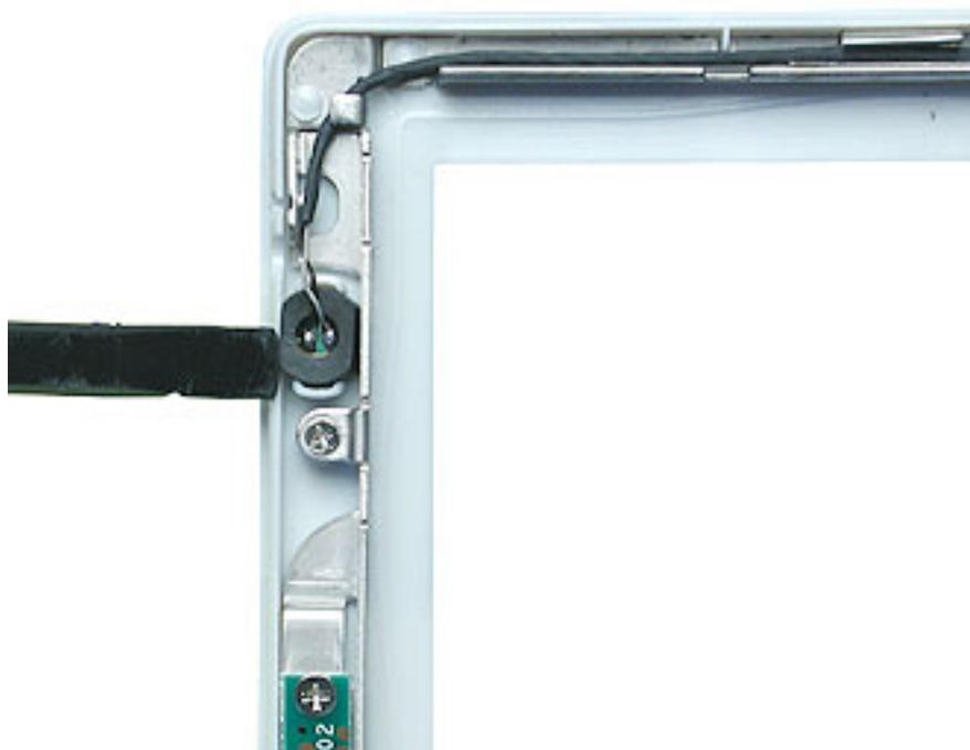
3. Working around the perimeter of the bezel, pull up the microphone cable from the cable channel, being careful not to strain any other cables.
