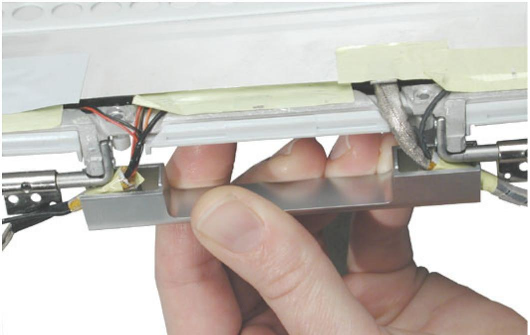
**Replacement Note:** When installing the replacement clutch cover, hold the cables and clutch cap in place as you slide the clutch cover over them.
