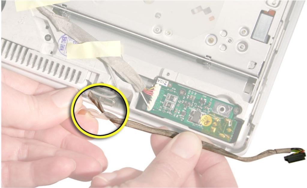
5. Make sure the tubing covers the cable where it exits the display.
