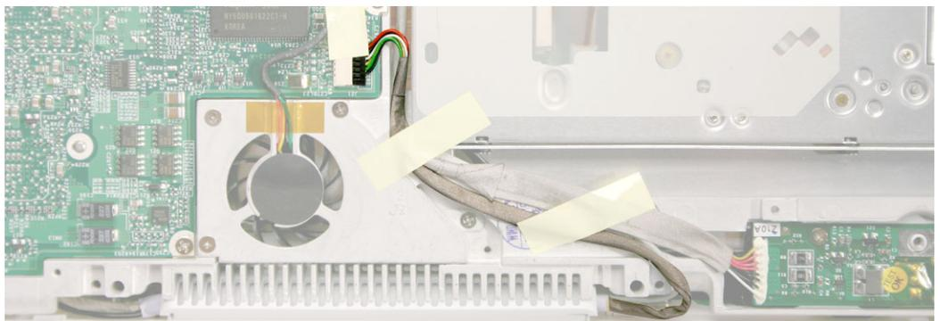
3. Release the cable from the channel in the frame.
