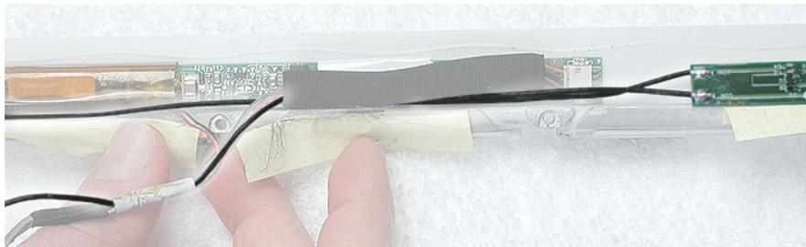
8. On the left side of the bezel, remove the two 3-mm long Phillips screws at the antenna receptor.
