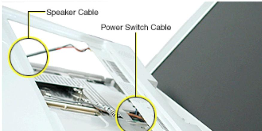
14. With the top case loosened, note how the speaker cable is routed.
