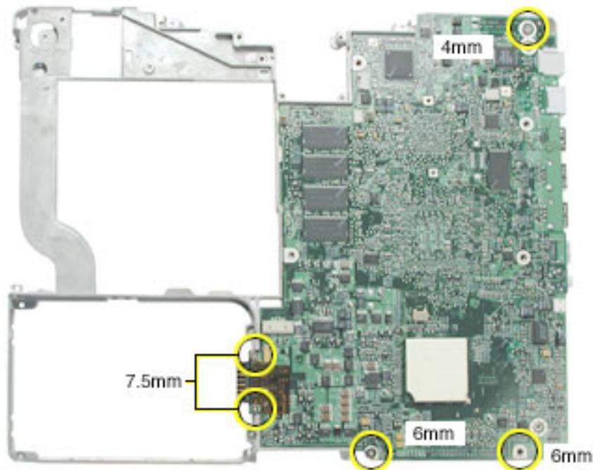
8. **Warning:** Flexing the logic board can break solder joints to components. To prevent damage, do not flex the board.
