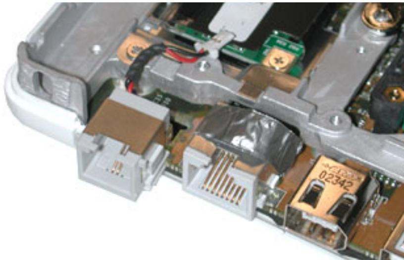
5. Install the replacement RJ11 modem cable, and reassemble and test the computer.
