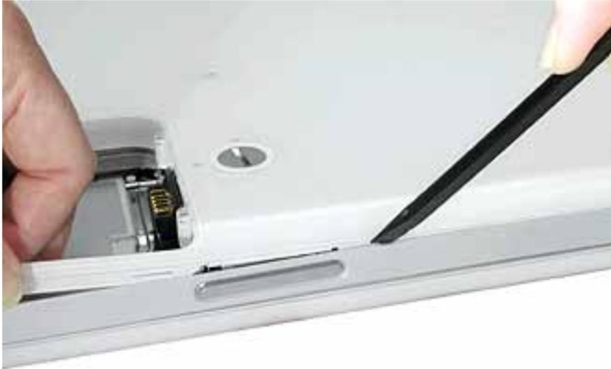
10. The bottom case fits snugly. Use moderate force to remove the remaining tabs from the slots.
