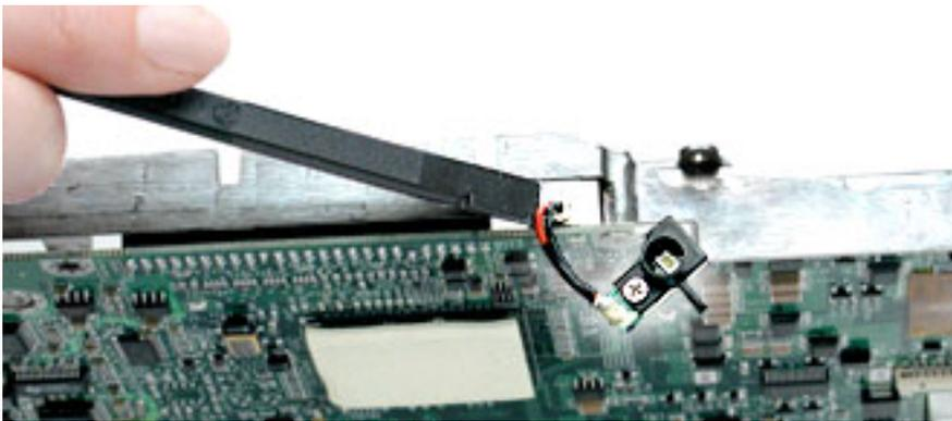
3. Remove the screw from the reset button board, and disconnect the connector from the logic board.
