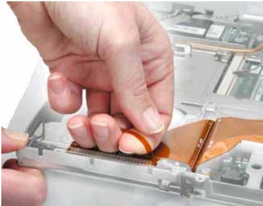
3. Lift up the fabric tape to release the microphone cable.
