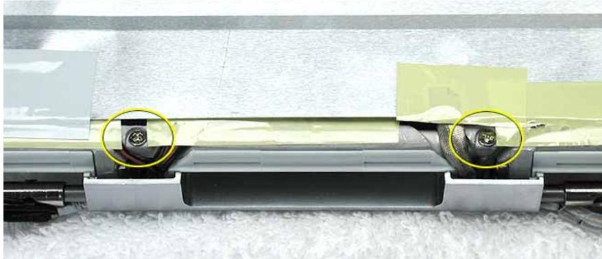
6. Tilt up the display assembly and pull straight down on the display clutch cover.
