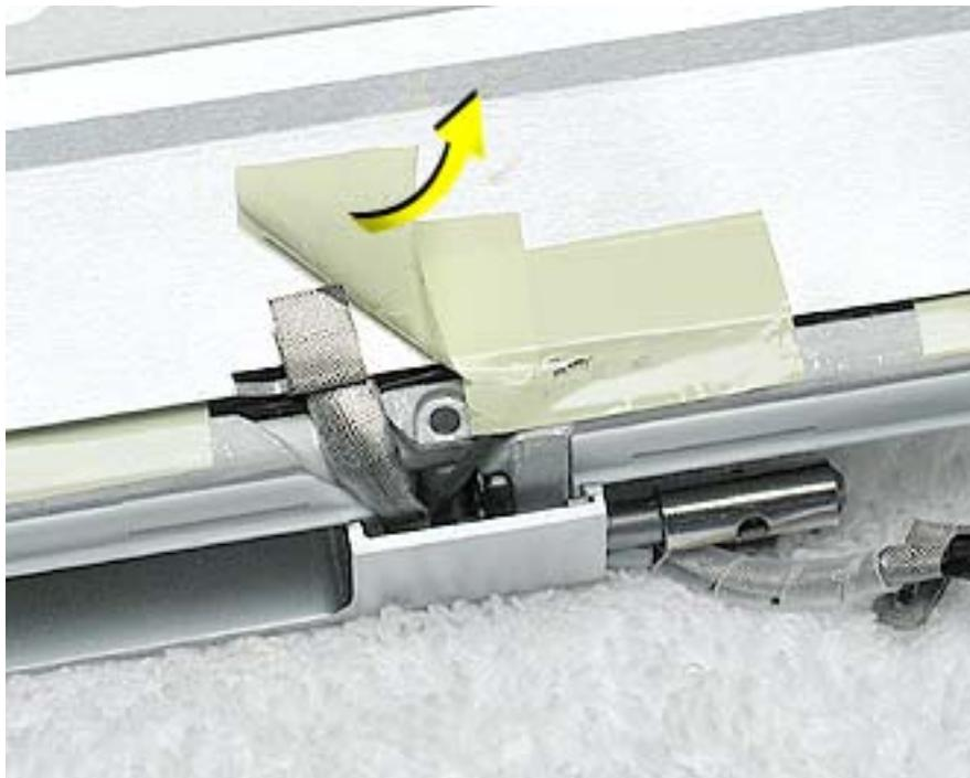
10. Loosen the remaining tape that secures the shield to the assembly. Remove the shield.
