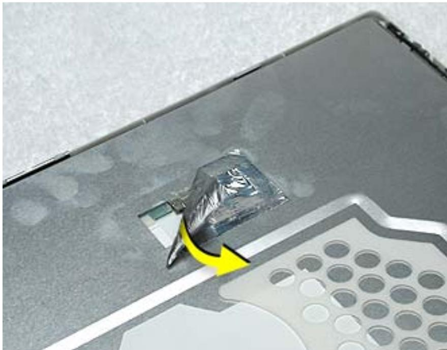
8. Peel up the tape if it covers the two screws at the clutch. Remove the two 11-mm long Phillips screws.
