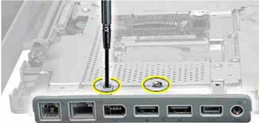
2. Tilt down the I/O bezel and remove it from the computer frame.
