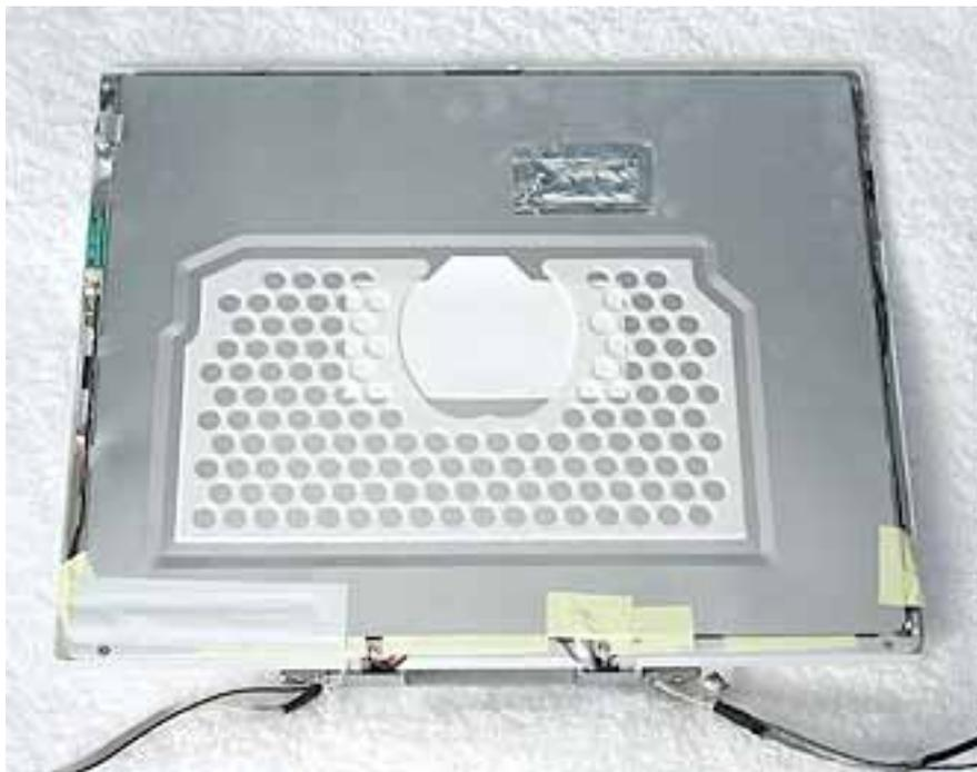
5. Peel up the tape if it covers the two screws at the clutch. Remove the two 11-mm long Phillips screws.
