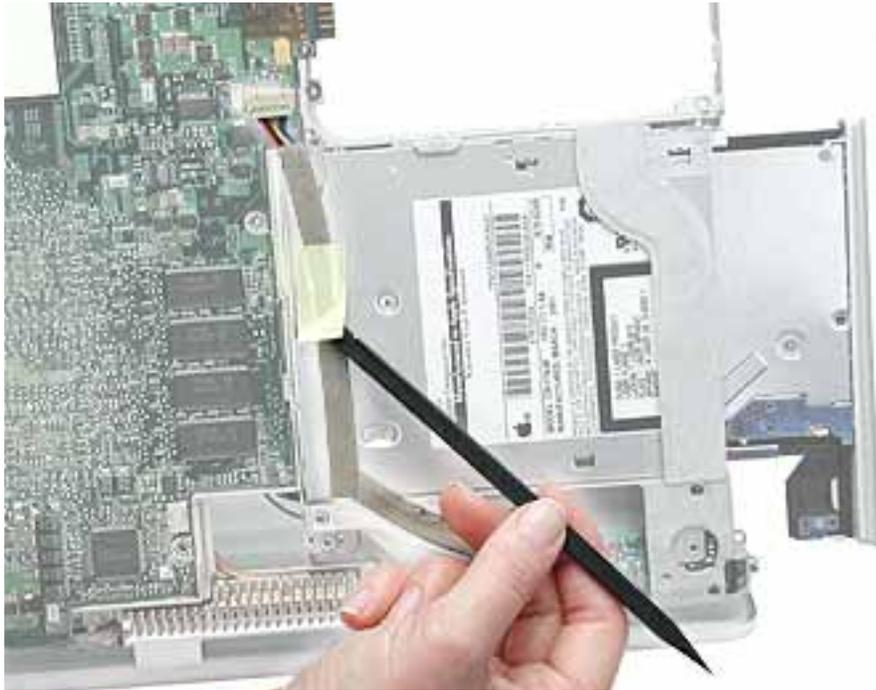
4. Tilt back the computer, and on the other side of the optical drive, loosen the tape holding the backlight cable to the optical drive. Do not disconnect the backlight cable.
