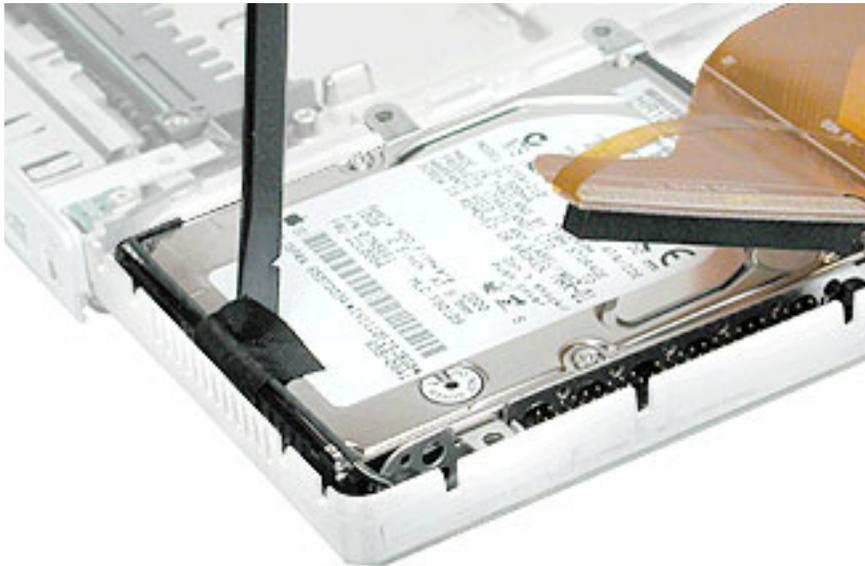
4. From the corner bracket, tilt the hard drive, and slide it out from under the microphone cable.
