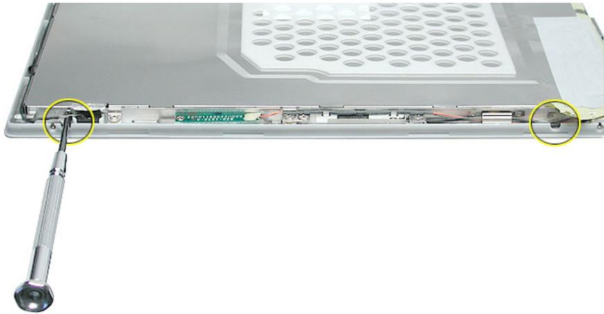
7. Peel up the foil tape that holds the LCD cable to the LCD shield.
