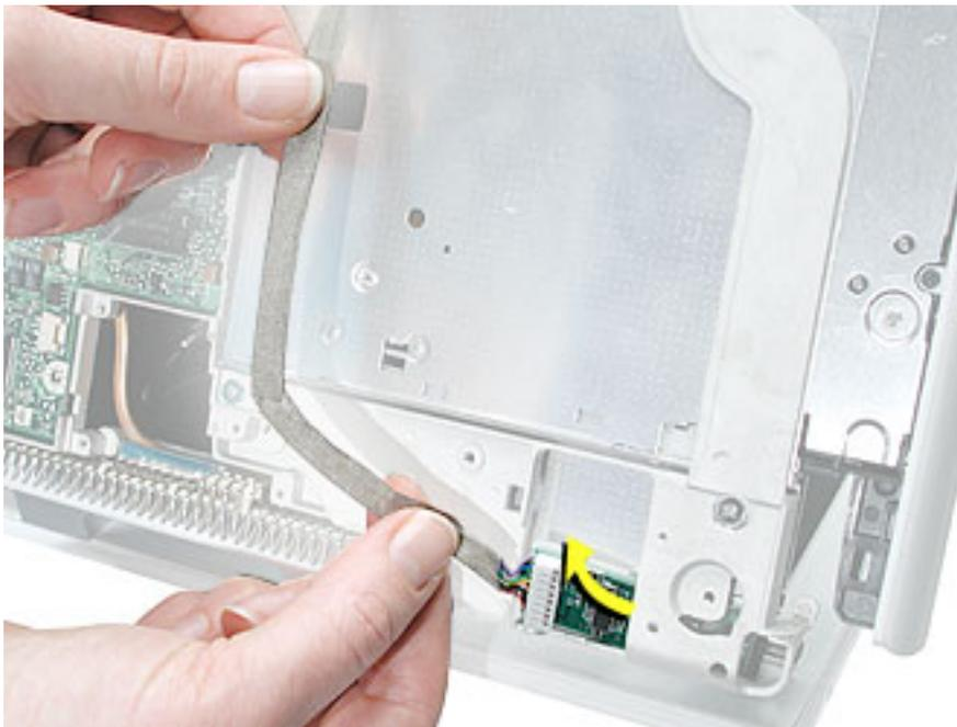
5. Install the replacement DC board, and reassemble and test the computer.
