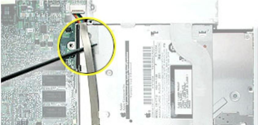
3. Tilt up the computer and note the routing of the flat power cable across the underside of the inner frame.
