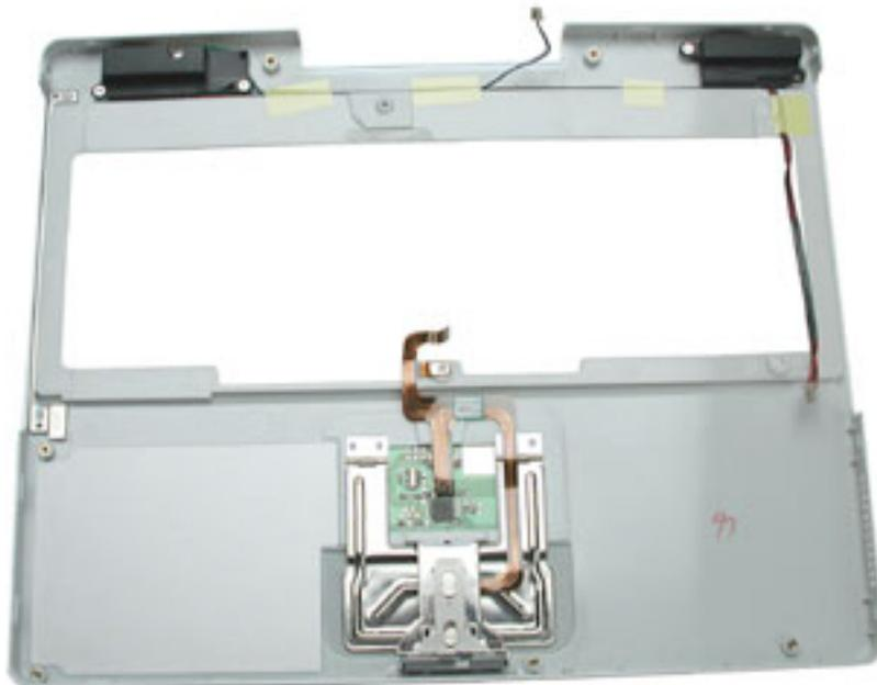
14. Install the replacement top case, and reassemble and test the computer.
