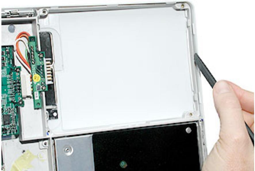
7. **Warning: The top case is connected to the computer assembly with delicate cables. Do not remove the top case until the cables are disconnected (see the next steps).**
