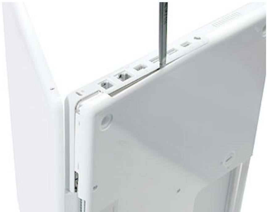
11. The bottom case fits snugly. Use moderate force to remove the tabs from the slots.
