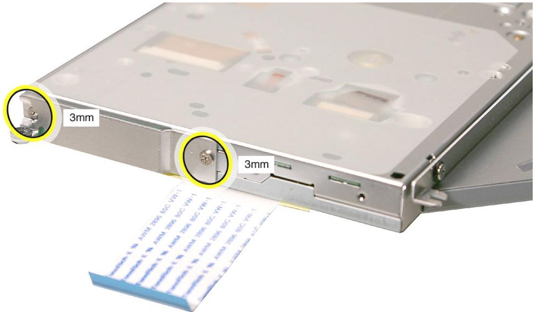
8. Peel off the tape from the optical drive, and disconnect the ribbon cable.
