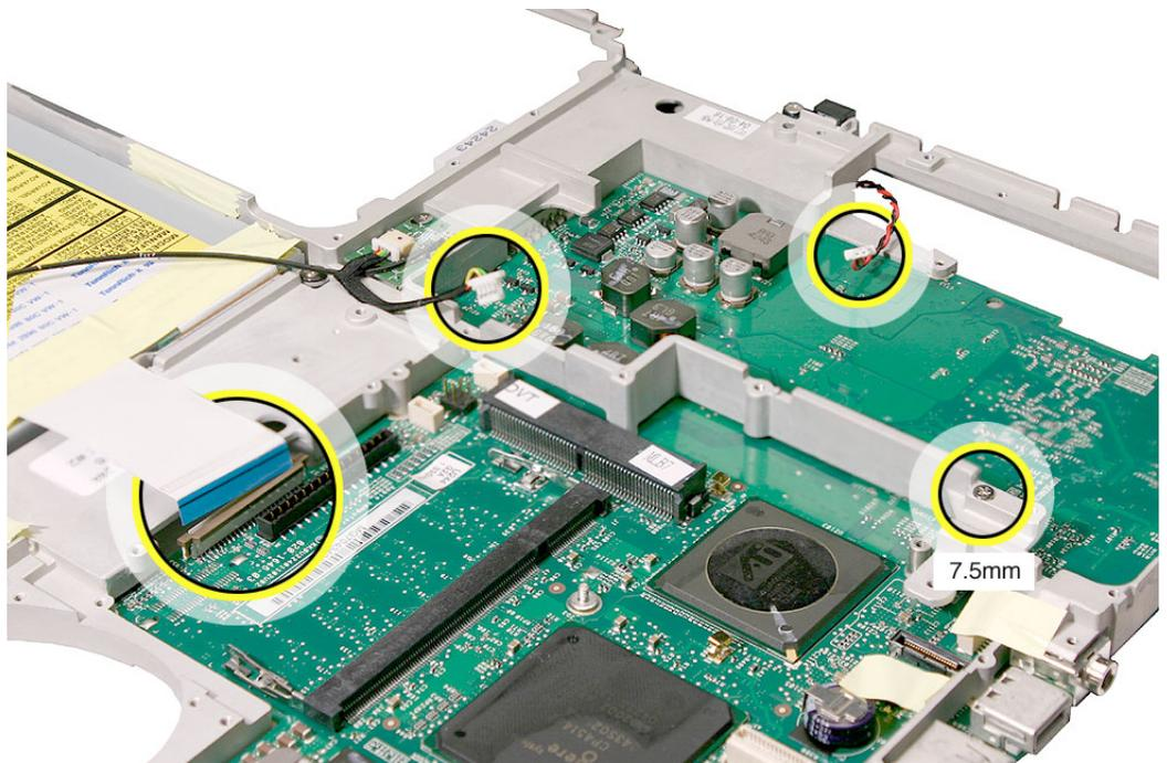
3. Turn over the frame, and remove the following from the logic board:
