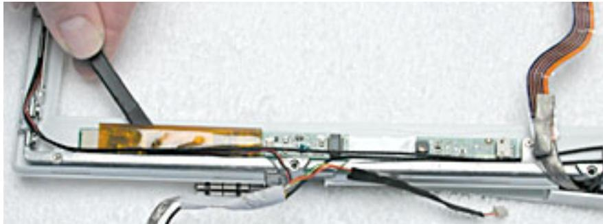
**Replacement Note:** The inverter board is held to the bezel assembly with double-sided tape on each end of the board. Use new double-sided tape when installing the replacement inverter board.
