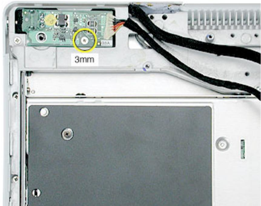
5. Tilt up the DC-in board, and pivot it out of the frame.
