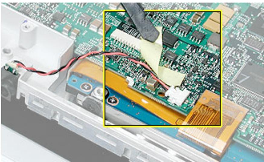
4. Turn over the computer and remove the single screw from the sleep light holder and frame.
