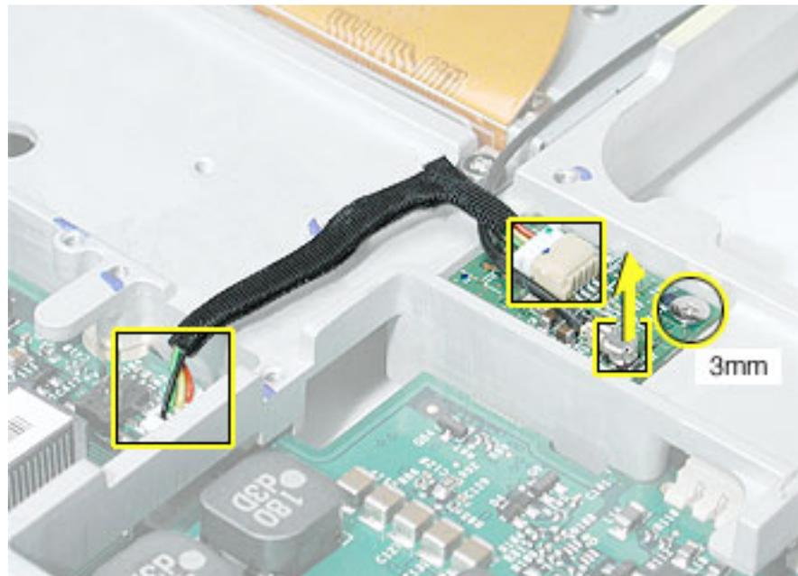
4. Install the replacement Bluetooth board and antenna, and reassemble and test the computer.
