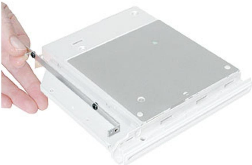
11. With the pointed end of a black stick, press the three tabs, and tilt the bezel up and off of the drive.
