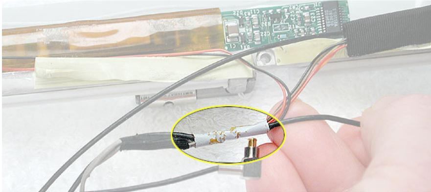
12. Use a black stick to lift out the cables from the channels.
