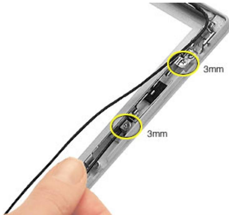
8. Tilt up the antenna receptor to remove it from the bezel assembly.
