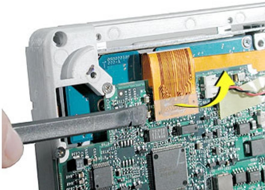
4. Remove the four identical screws at the hard drive bracket.
