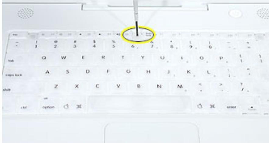
3. Release the keyboard by pulling down on the keyboard release tabs (located to the left of the F1 and F12 keys), then lift the top portion of the keyboard up slightly, and toward the display.
