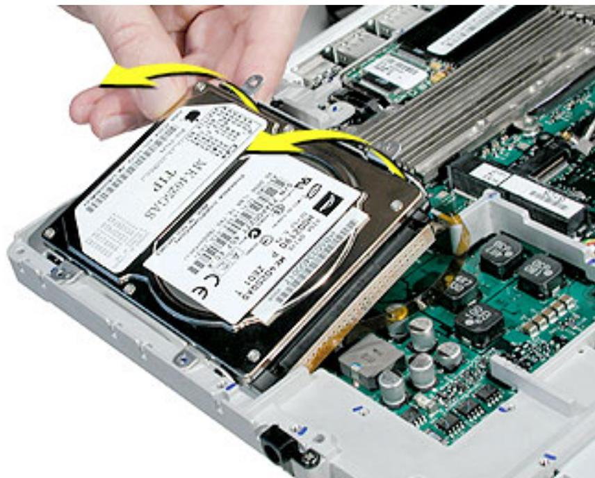
6. Route the end of the hard drive cable through the opening in the computer frame.
