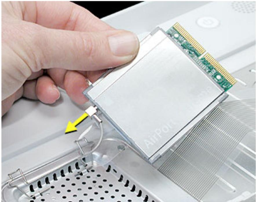
5. Install the replacement AirPort Extreme Card into the slot.
