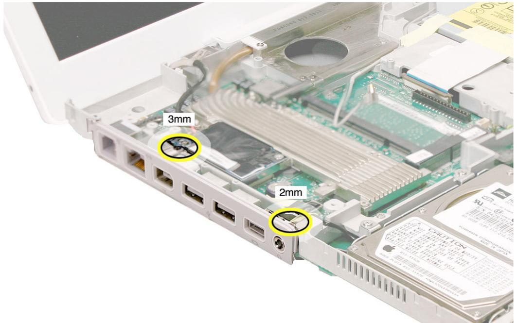
2. Remove the I/O bezel from the computer frame.
