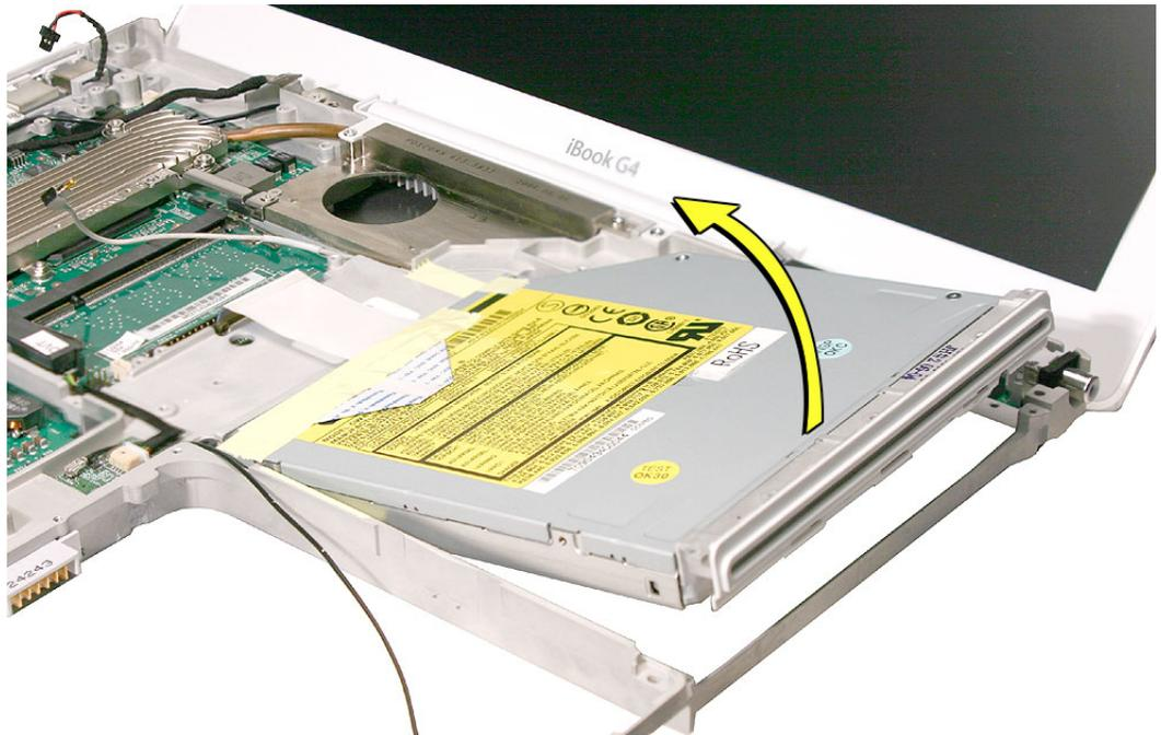
6. Remove the two identical screws holding the cable bracket to the optical drive.
