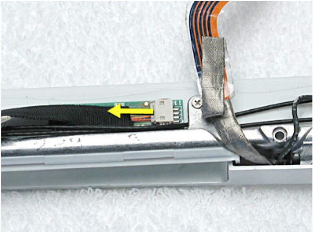
2. **Replacement Note:** Note the position of the inverter board and cables for the installation of the replacement inverter board.
