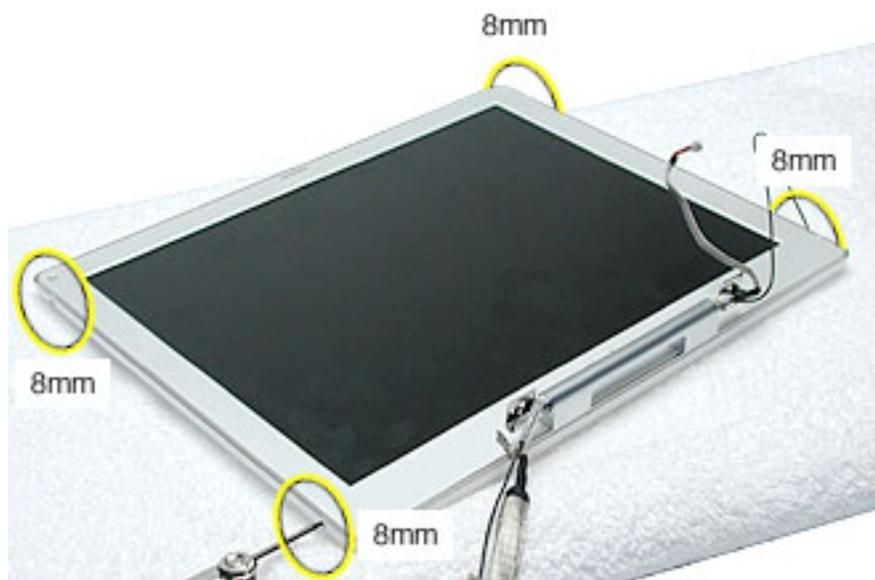
2. Using a black stick, pry up the bezel from the display housing. Carefully work the black stick around the outer perimeter and corners of the bezel.
