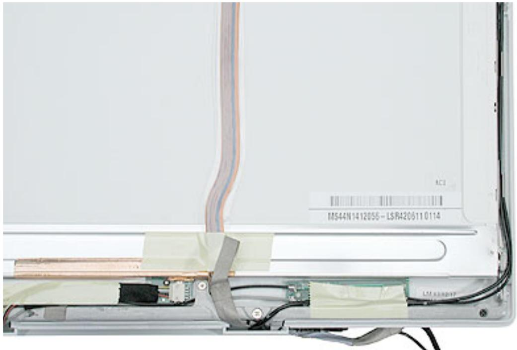
13. **Warning: When lifting the LCD panel, be careful not to strain the inverter cable.**
