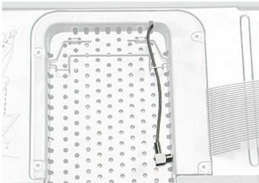
9. Lift the RAM shield out of the computer.
