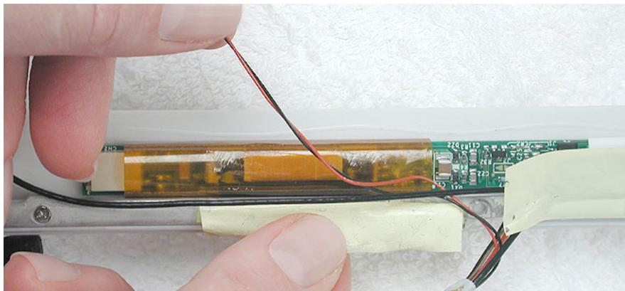
4. **Warning:** When removing the tape that bundles the reed switch cable assembly to the AirPort antenna cable, be careful not to strain or pinch the cables.
