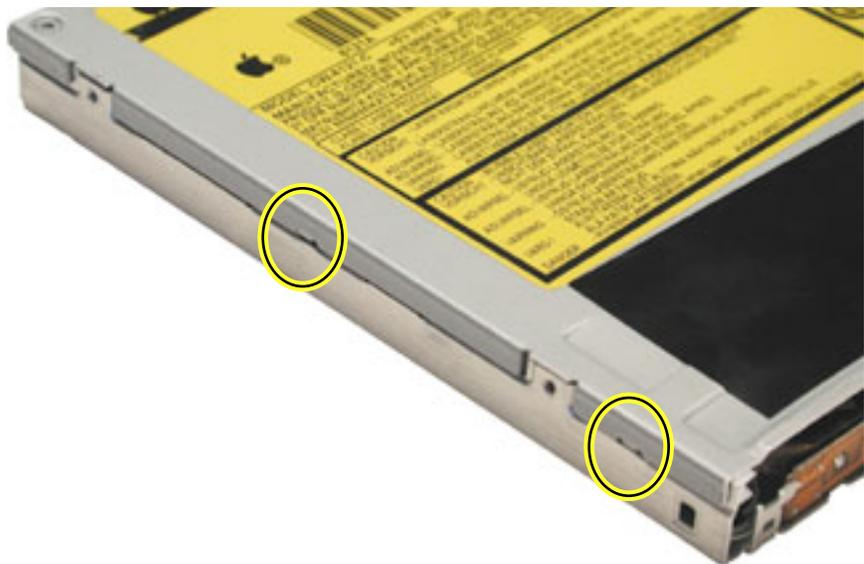
6. Replace the four screws. If applicable, install the brackets, cable, and faceplate back on the drive before returning the old drive.
