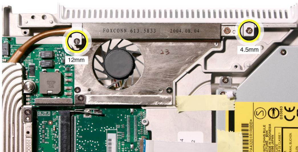
2. Remove the vent cover from the computer assembly.
