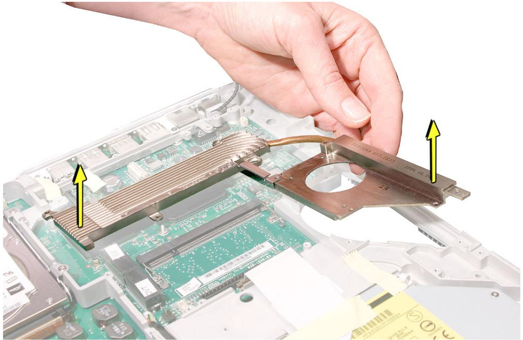
3. Turn over the heatsink and note the placement of the thermal pads.
