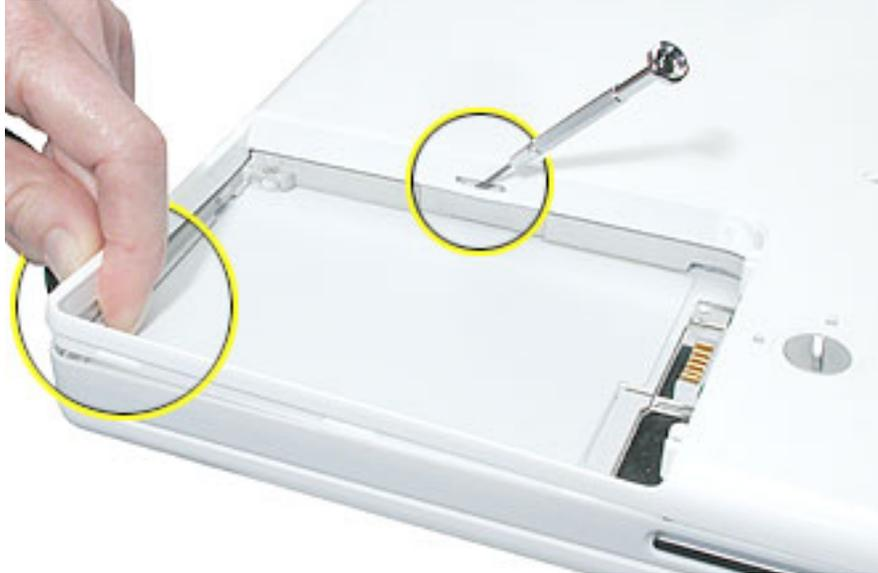
13. Loosen the tabs from the slot load area last.
