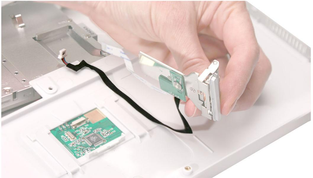
6. Install the replacement display latch by tilting it onto the trackpad assembly, pressing the latch button, and feeding the latch into the latch opening in the top case. Test that the latch button works easily.
