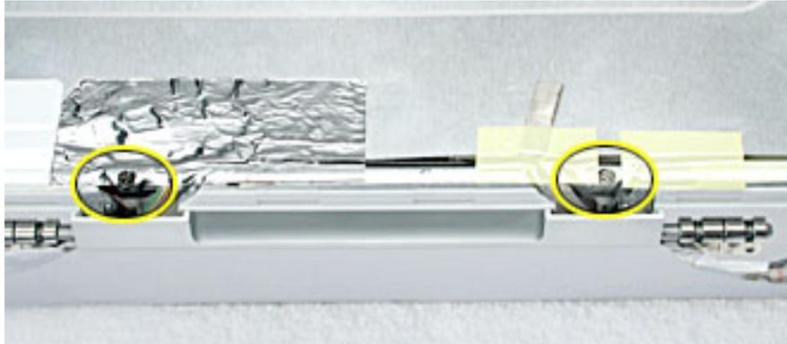
**Note:** The positioning of the tape on the shield might differ among computer models.
