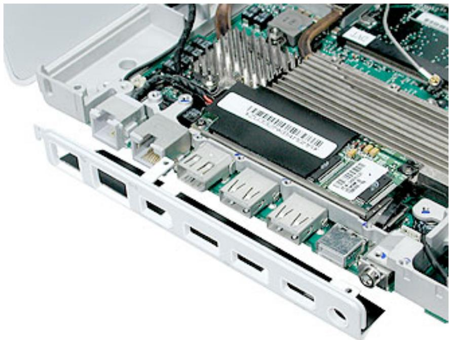
3. Install the replacement I/O bezel, and reassemble and test the computer.
