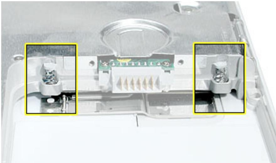
5. Install the replacement bottom shield, and reassemble and test the computer.
