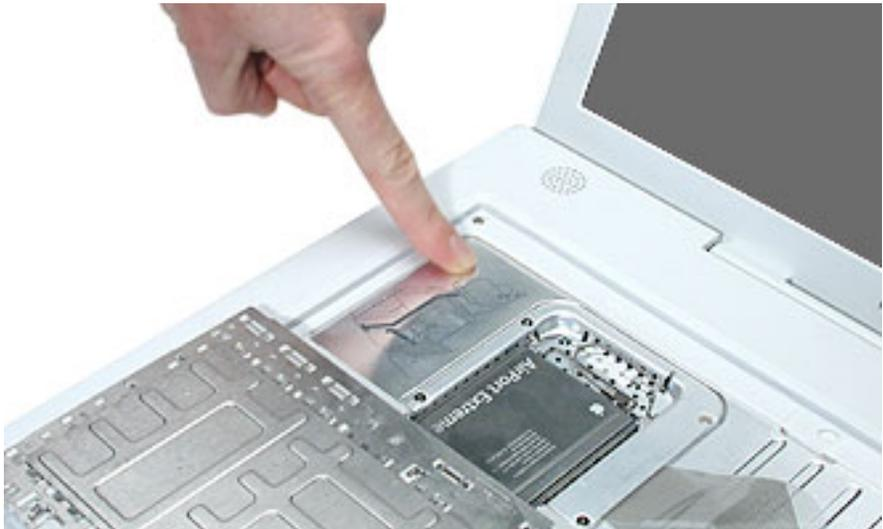
6. For the installed AirPort Extreme Card, unlatch the flexible wire bracket that secures the card.
