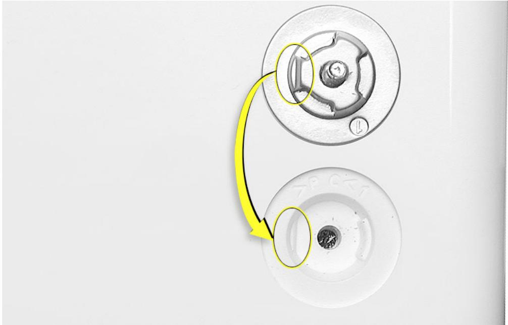
2. With the socket sitting flat in the bottom case, install the screw.
