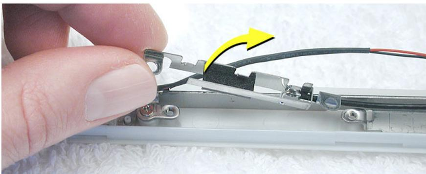
11. Unwrap the tape that secures the AirPort antenna cable to the cable bundle.
