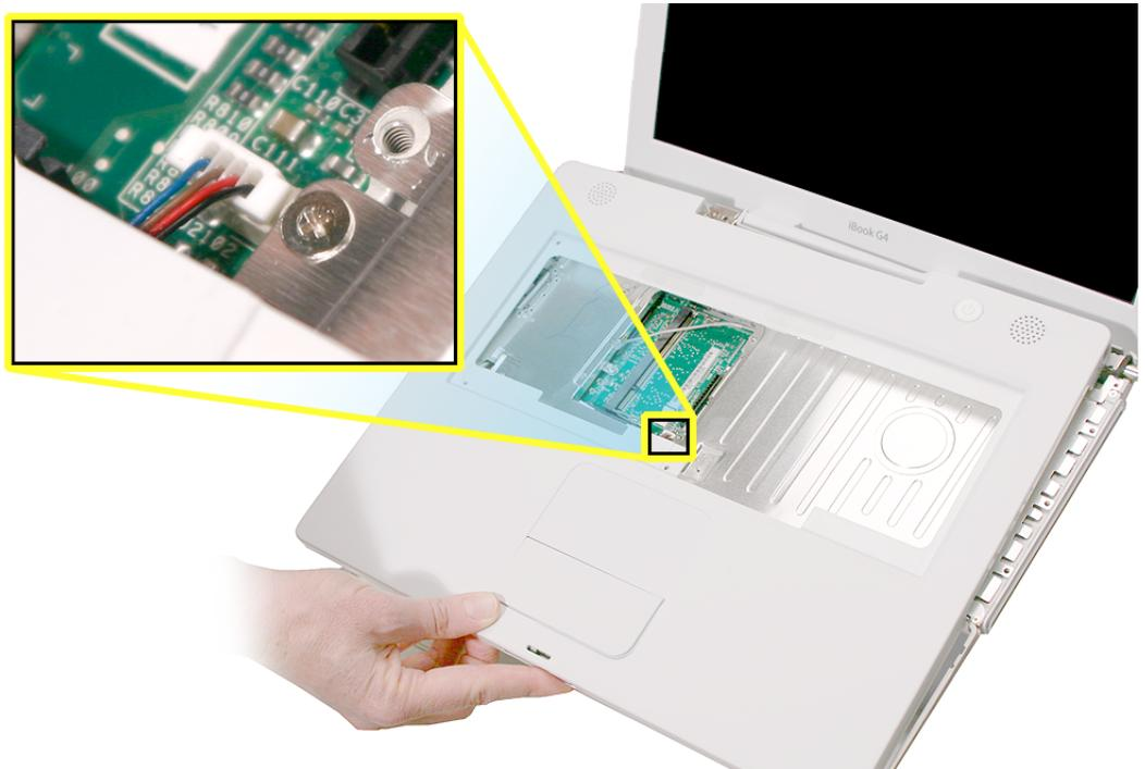
8. With the speaker cable and power cable still attached, carefully reposition the top case so you can access the two remaining cables.
