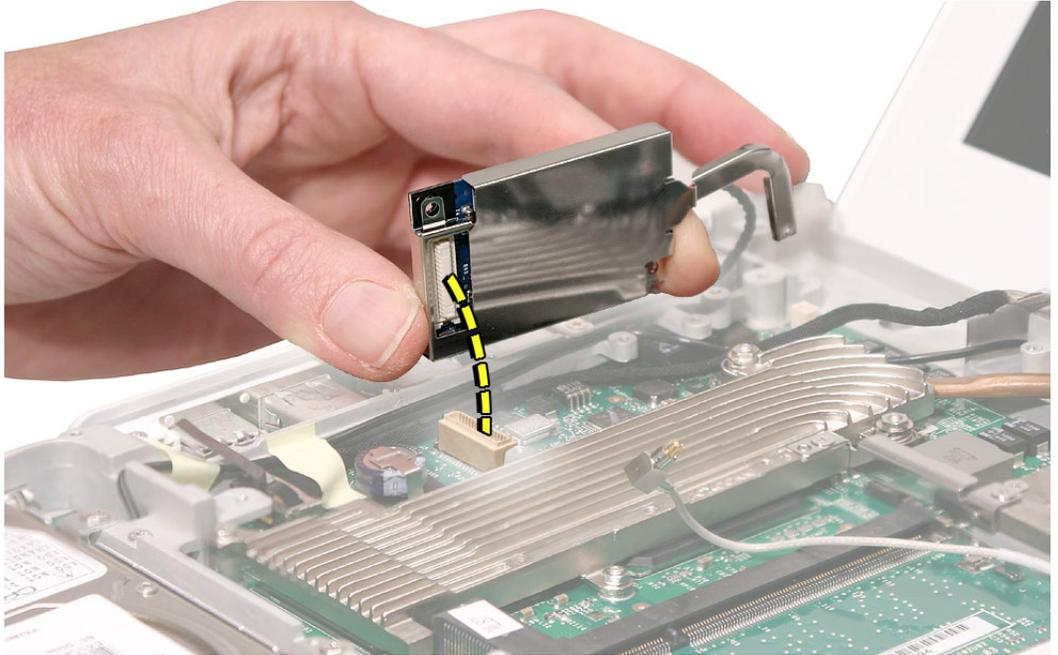
5. Disconnect the cable from the end of the modem board.
