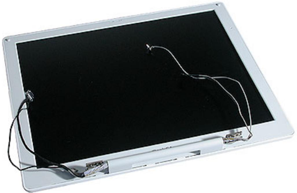
**Replacement Note:** As you reassemble the computer, make sure cables are secure. Check that the microphone cable is routed as shown.
