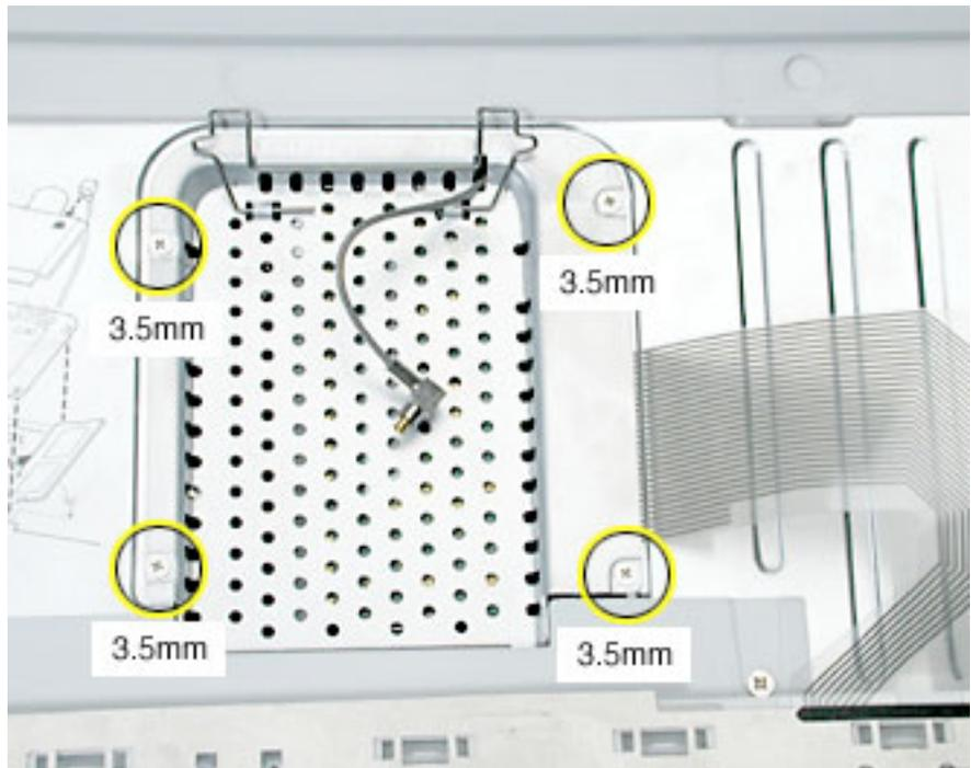
**Replacement Note:** Note the routing of the AirPort antenna cable. When reinstalling the RAM shield, make sure the antenna cable is routed as shown if there is no AirPort Extreme Card.
