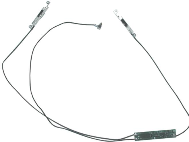
14. Install the replacement antenna board, and reassemble and test the computer.
