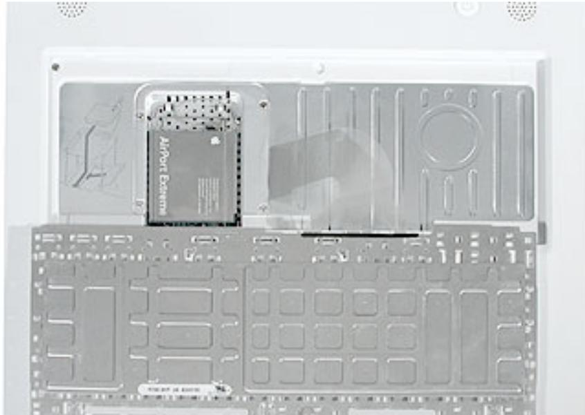
**Note:** If no replacement AirPort Extreme Card is to be installed, the antenna cable should be routed as shown.
