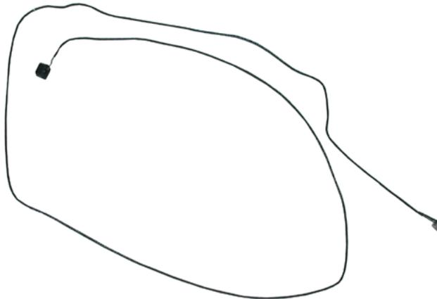
7. Install the replacement microphone cable, and reassemble and test the computer.
