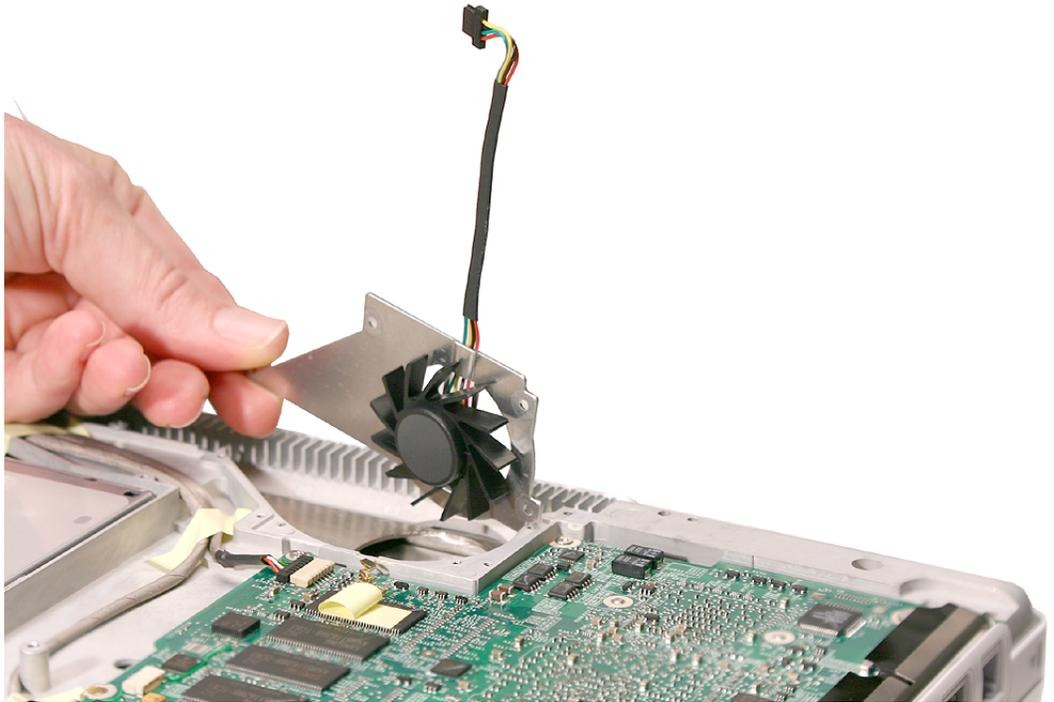
5. Install the replacement fan, and reassemble and test the computer.
