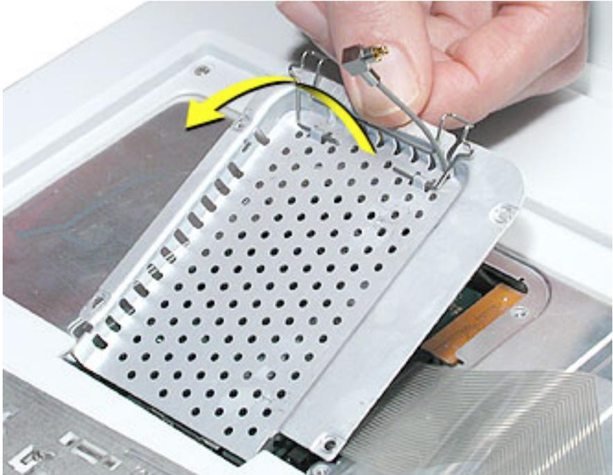
11. Locate the keyboard cable connector.
