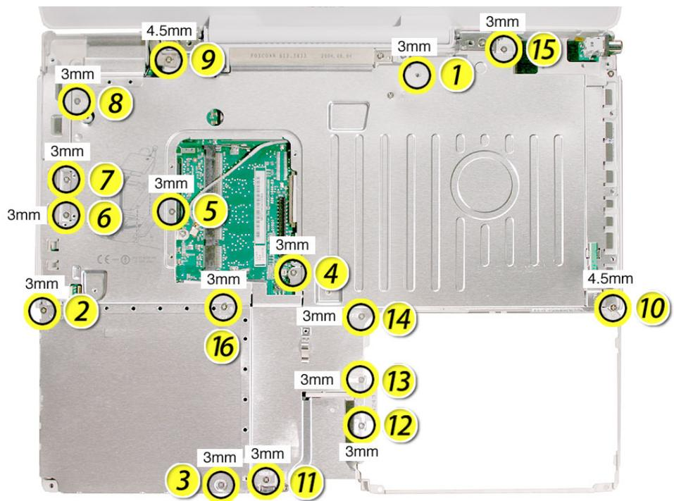
**Replacement Note:** The longest screw at the top shield secures the LVDS cable to the shield and frame.
