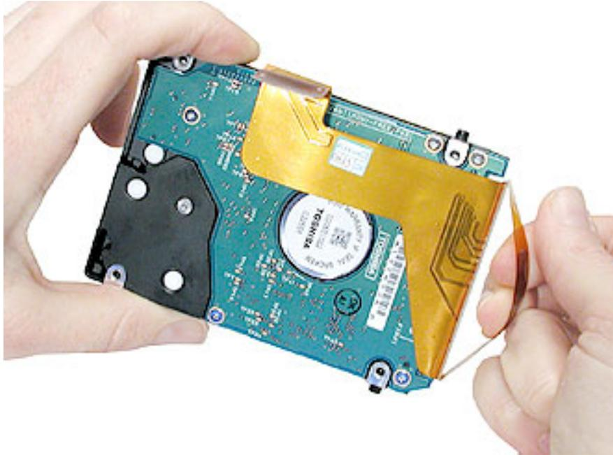
9. Remove the four black Torx T8 screws from the ends of the hard drive, and transfer the screws to the replacement drive.
