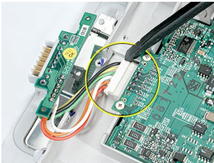
3. Install the replacement battery transfer board, and reassemble and test the computer.
