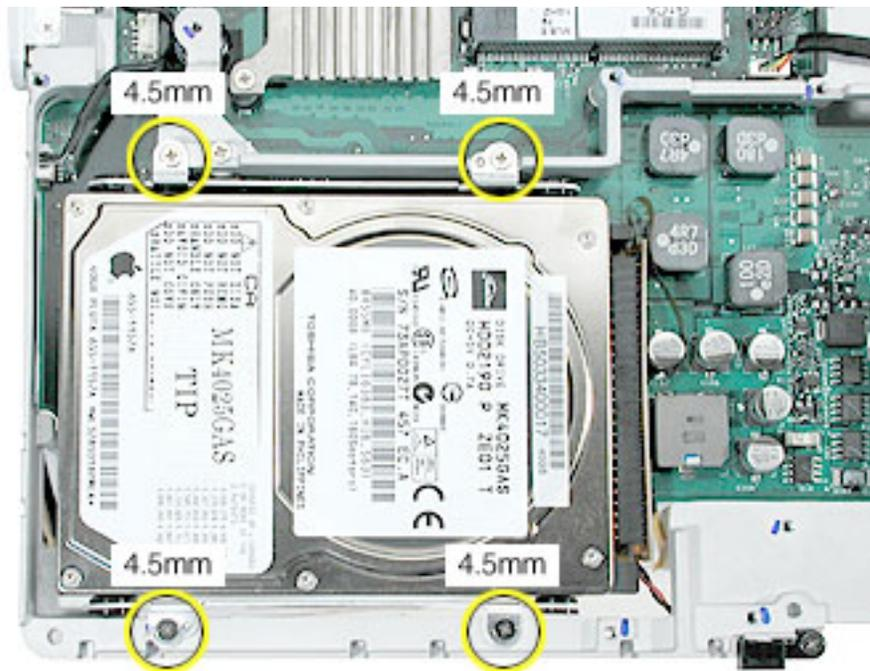
5. From the bracket side, tilt up the hard drive, and hold it by the sides of the drive.
