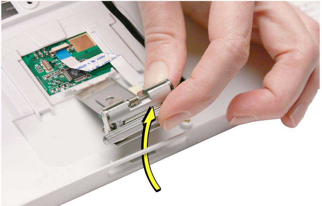
5. Carefully peel up the trackpad cable from the top case.
