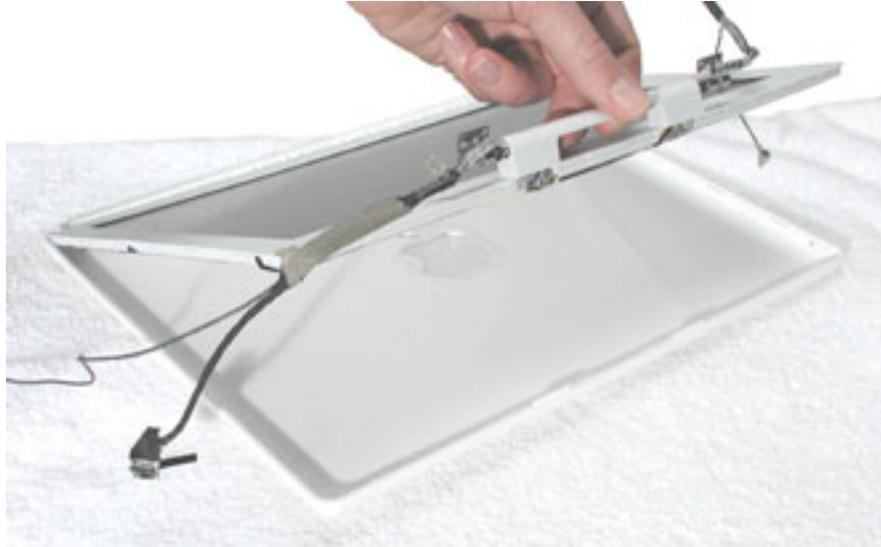
4. Place the display assembly face down on a soft cloth.
