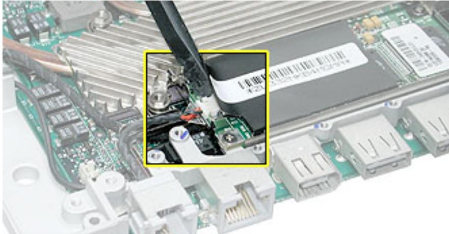
2. Guide the cable up through the metal channel.
