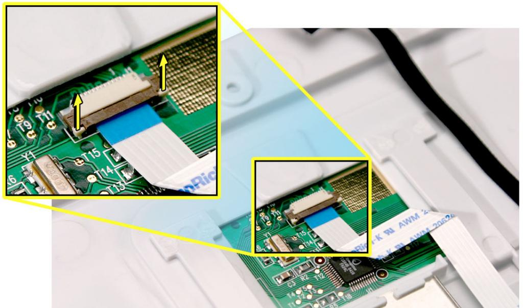
3. With the locking connector tilted up, slide out the trackpad cable.
